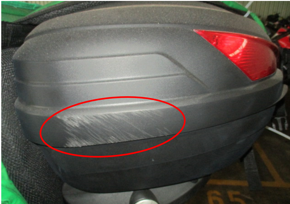
Photo 12 shows the top box of the Motorcycle that had sustained damages of grazing nature as a result of the accident (circled).
