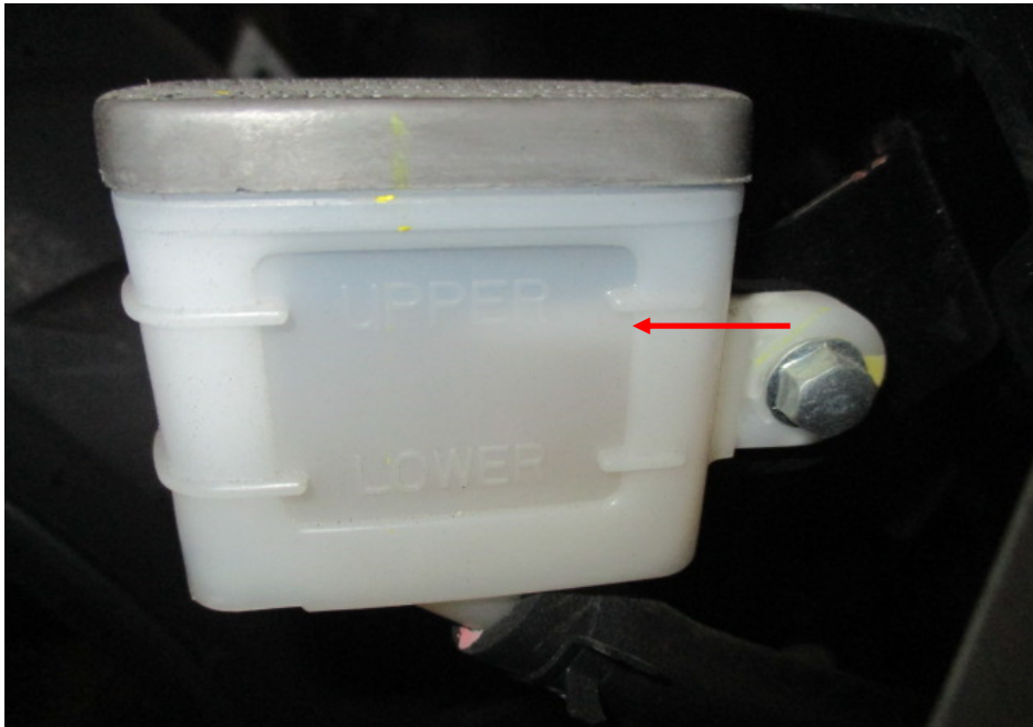
Photo 26 shows the brake fluid reservoir for the rear brake of the Motorcycle. The brake fluid was observed to be of sufficient level (arrowed) and without contamination for operational purposes.
