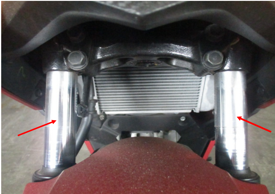
Photo 19 shows the front fork (arrowed) of the Motorcycle. The front fork and fork bracket of the Motorcycle were both found to be intact and undamaged. Turning the Motorcycle's handle bar towards the left and right did not produce any abnormal free play. The steering system of the Motorcycle was in serviceable condition at the time of our inspection.
