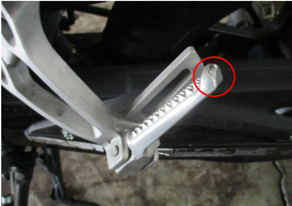
Photo 10 shows a closer view of the left pillion foot peg which was amongst the body parts of the Motorcycle that had sustained damages of grazing nature as a result of the accident (circled).
