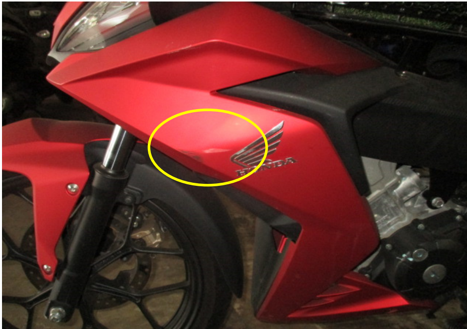
Photo 6 shows a closer view of the left cowling (circled) which was amongst the body parts of the Motorcycle that had sustained damage as a result of the accident.
