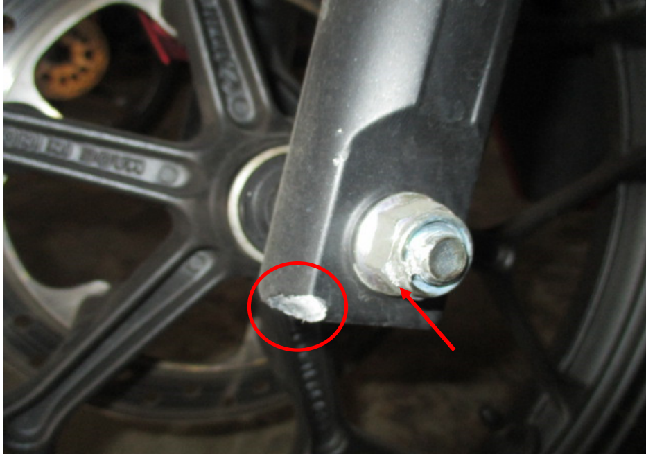
Photo 4 shows a close up view of the left front fork outer tube (circled) and front wheel axle nut (arrowed) which were amongst the body parts at the front of the Motorcycle that had sustained damage as a result of the accident.
