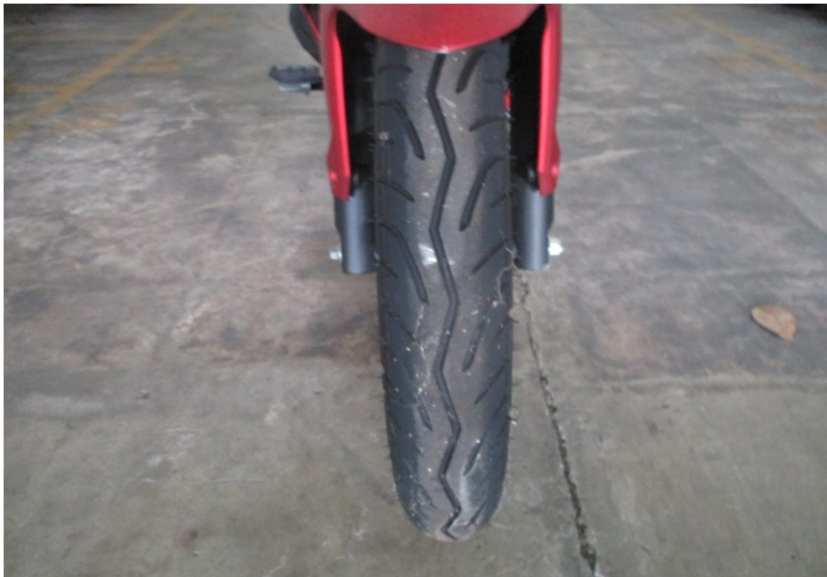
Photo 13 shows the front tyre of the Motorcycle at the time of our inspection. The front tyre was observed to be in serviceable condition with remaining tread depth of approximately 4mm. The pattern of the tread was also clearly visible. There was no tear, burst mark(s) and/or punctured hole(s) on the sidewalls as well as across the tread of the front tyre.
