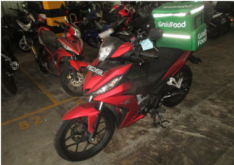
Photo 3 shows a general view of the left body of the Motorcycle at the time of our inspection. The Motorcycle was observed to have sustained damages along its left body. Amongst the body parts that were found to have been damaged include its left front fork outer tube, front wheel axle nut, left cowling, clutch lever, left side mirror, gear shift pedal, left front footrest, left pillion foot peg, top box rack and top box, amongst others.
