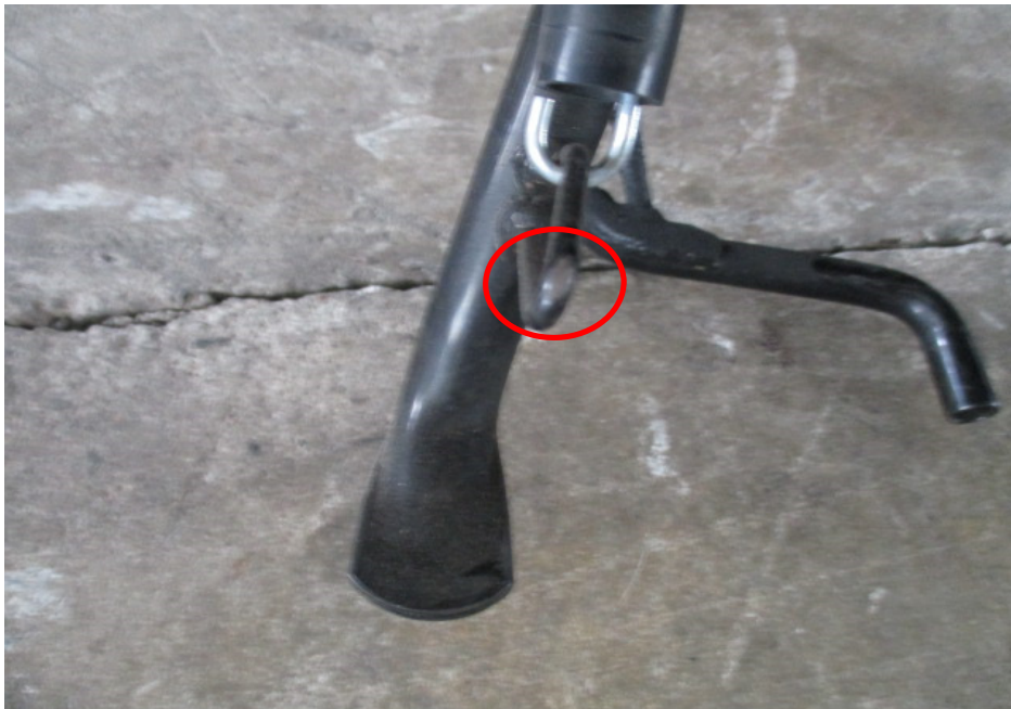
Photo 5 shows a closer view of the side stand (circled) which was amongst the body parts of the Motorcycle that had sustained damage as a result of the accident.
