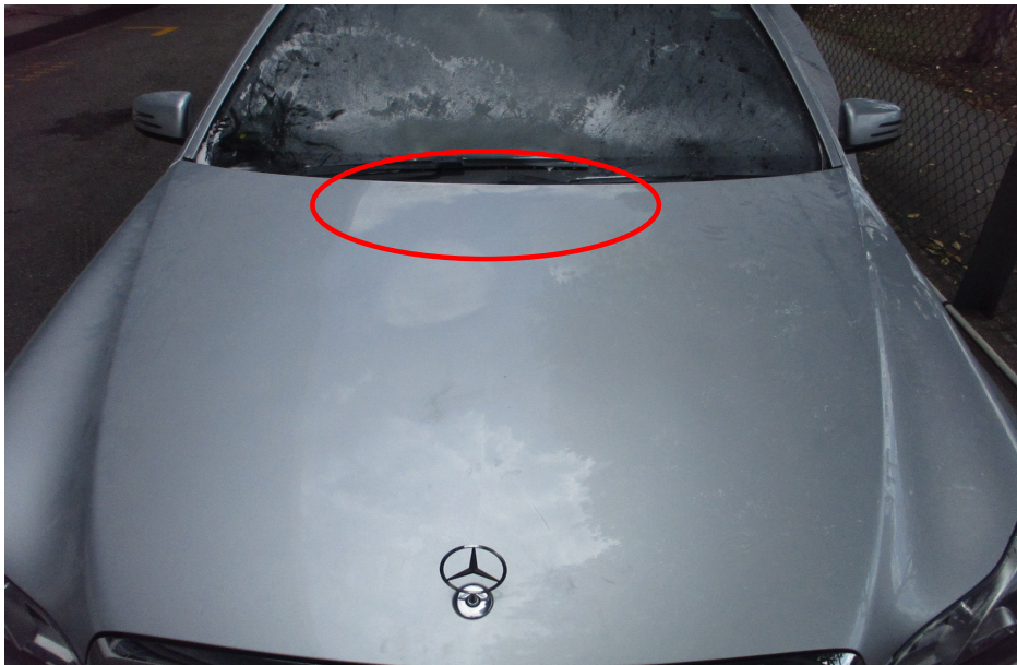
Photo 7 shows the burn pattern and whitish burn marks that were found on the rear centre portion of the front bonnet of the Insured Vehicle (circled). Such whitish burn marks are a result of exposure to prolonged heat intensity, which may indicate where the fire had started. Rust would also begin to develop on these areas soon after the fire.
