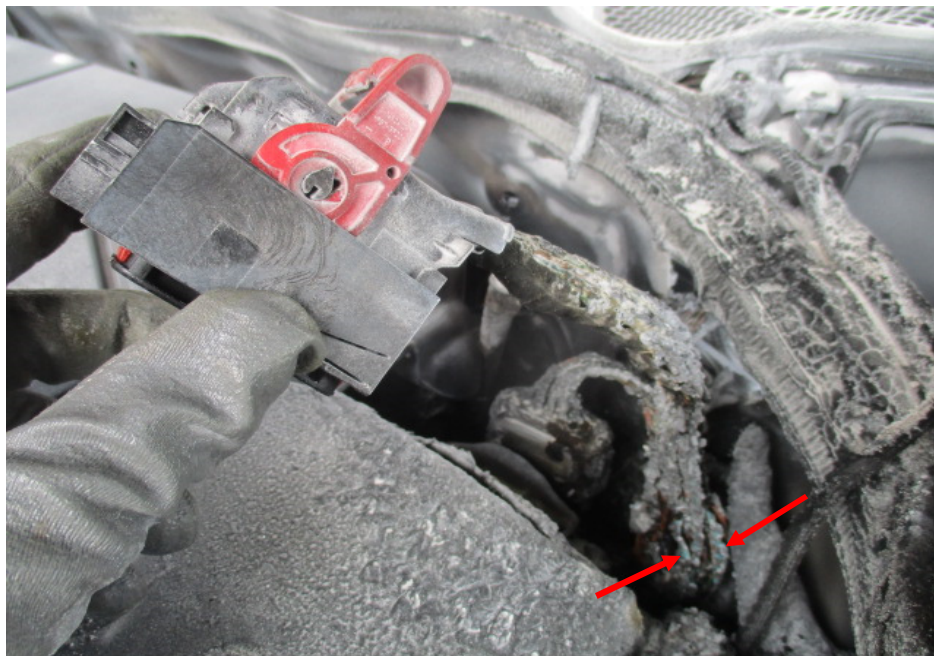
Photo 12 shows a closer view of the greenish residue on the wirings leading from the wiring harness of the Insured Vehicle (red arrows). The presence of such greenish residue suggests occurrence of an electrical short circuit.
