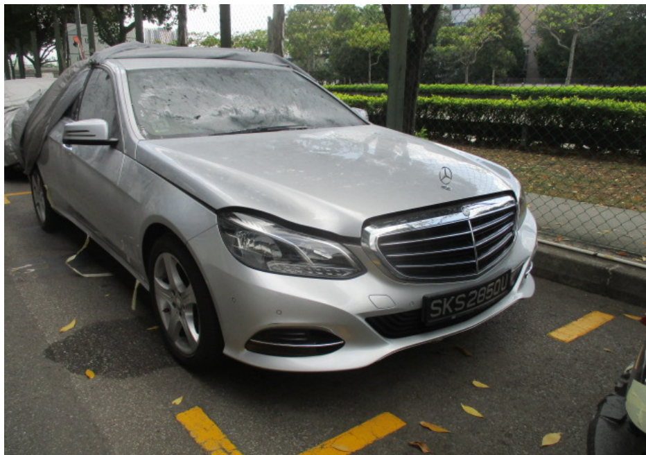
Photo 2 shows the general view of the right front portion of the Insured Vehicle at the time of our inspection. The exterior body of the Insured Vehicle had sustained visible fire damage. This included its front windscreen and front bonnet.
