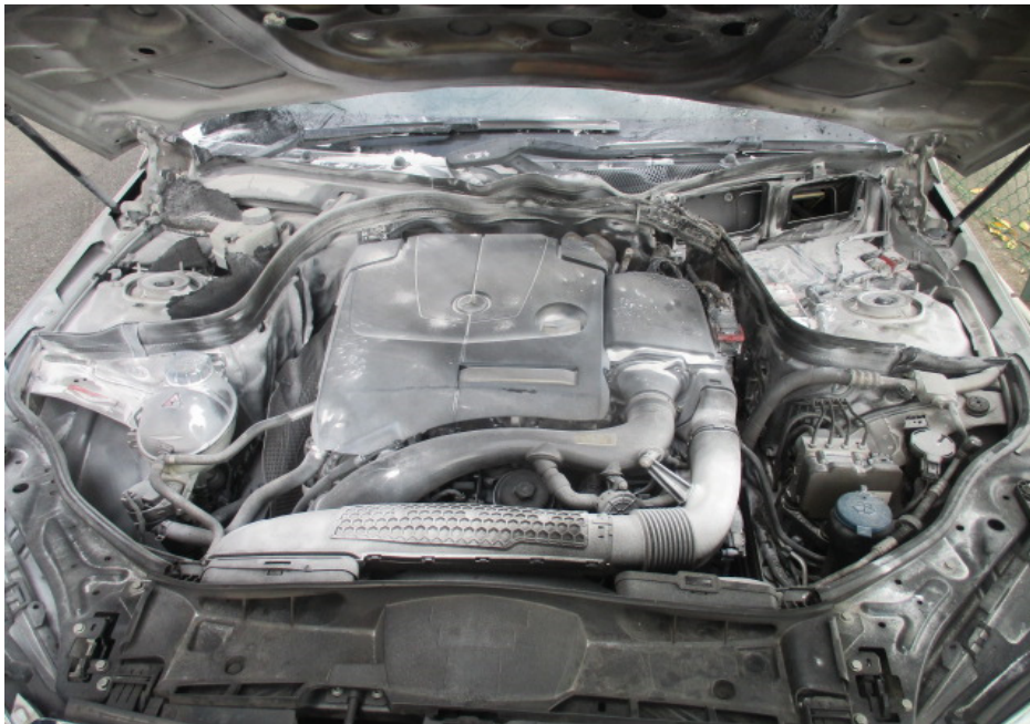
Photo 6 shows a general view of the engine compartment of the Insured Vehicle at the time of our inspection. Some of the components inside the engine compartment were found to be severely burnt and/or melted as a result of the fire.
