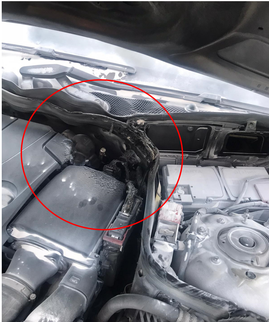
Photo 16 shows the Insured Vehicle at the incident scene after the fire was extinguished. In general, the information that could be gathered from these photographs had corresponded to the events that were related to us by Mr Lingam. The burn pattern and concentration of fire extinguisher residue observed at the rear centre portion of the engine compartment (circled) is an indication that the fire had started from the rear centre portion of the engine compartment.
