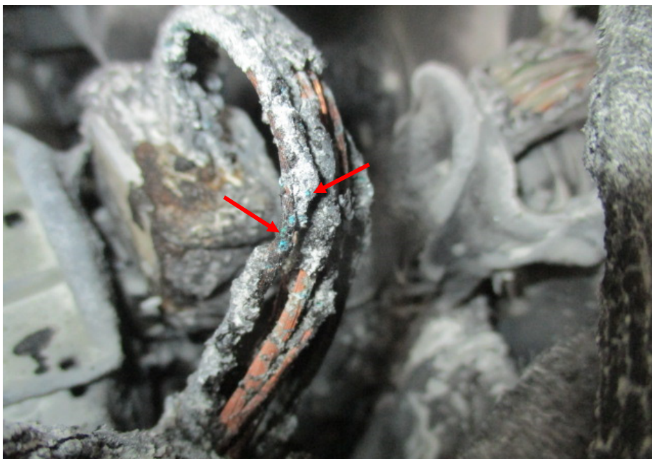
Photo 14 shows a close up view of the greenish residue on the wirings leading from the disconnected wiring harness of the Insured Vehicle (red arrows). The presence of such greenish residue suggests occurrence of an electrical short circuit.
