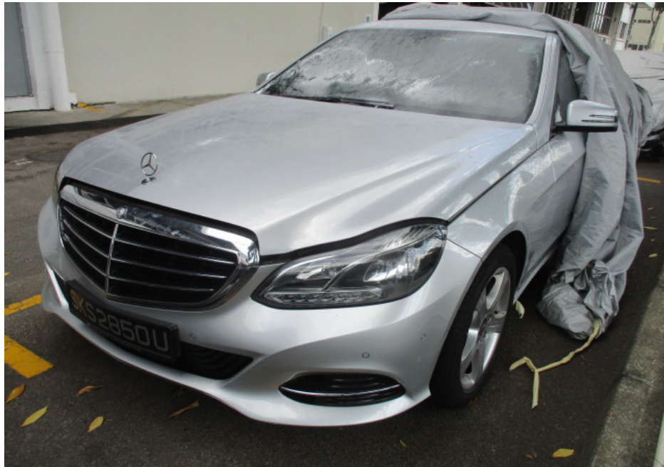
Photo 3 shows the general view of the left front portion of the Insured Vehicle at the time of our inspection. The exterior body of the Insured Vehicle had sustained visible fire damage. This included its front windscreen and front bonnet.
