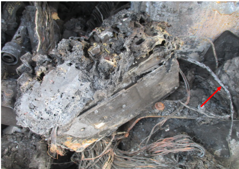
Photo 10 shows a closer view of the burnt wirings leading from the battery around the left portion of the engine compartment, which is in the immediate vicinity where the fire to the Insured Vehicle had likely started. We noticed greenish residue on several stretches of burnt wirings (arrowed). The presence of greenish residue indicates internal heating of copper wires, a sign of an electrical short circuit occurring. The greenish residue is normally left behind from oxidation as a result of chemical reaction involving the copper wires.
