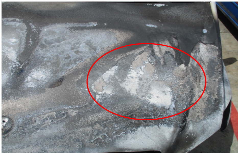
Photo 7 shows the burn pattern and whitish burn marks that were found on the left portion of the front bonnet of the Insured Vehicle (circled). Such whitish burn marks are a result of exposure to prolonged heat intensity, which may indicate where the fire had started. Rust would also begin to develop on these areas soon after the fire.
