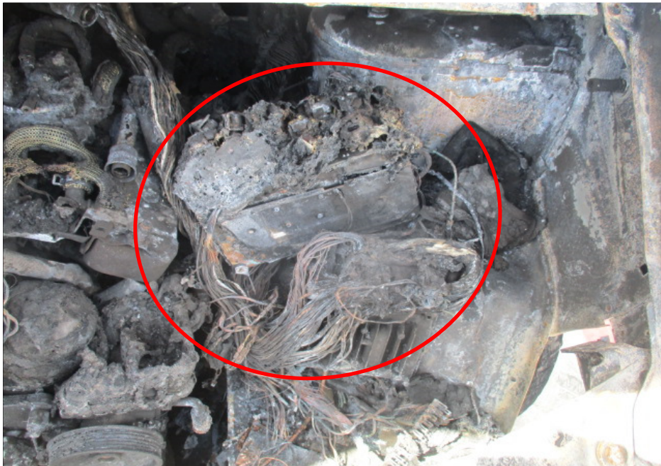
Photo 9 shows the burnt wirings leading from the battery around the left portion of the engine compartment (circled), which is in the immediate vicinity where the fire to the Insured Vehicle had likely started.
