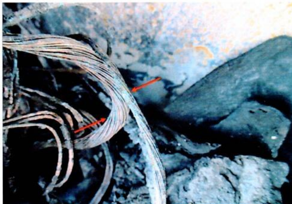
Photo 12 shows a close up view of the greenish residue found on several stretches of burnt wirings leading from the battery (red arrows). The presence of such greenish residue suggests occurrence of an electrical short circuit.
