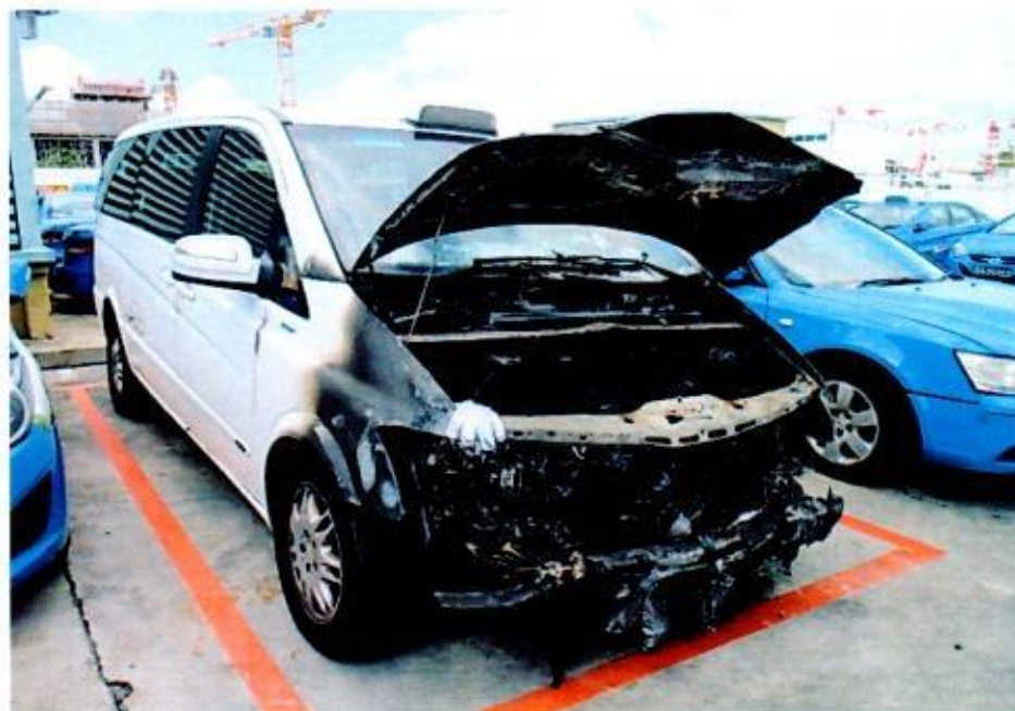
Photo 2 shows the general view of the right portion of the Insured Vehicle at the time of our inspection. The exterior body of the Insured Vehicle had sustained visible fire damage. This included its front windscreen, front bonnet, front bumper, right front panel and right headlight.
