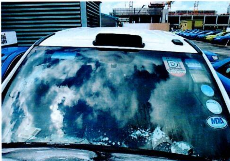
Photo 4 shows a closer view of the front windscreen of the Insured Vehicle at the time of our inspection. The front windscreen had sustained significant fire damage.
