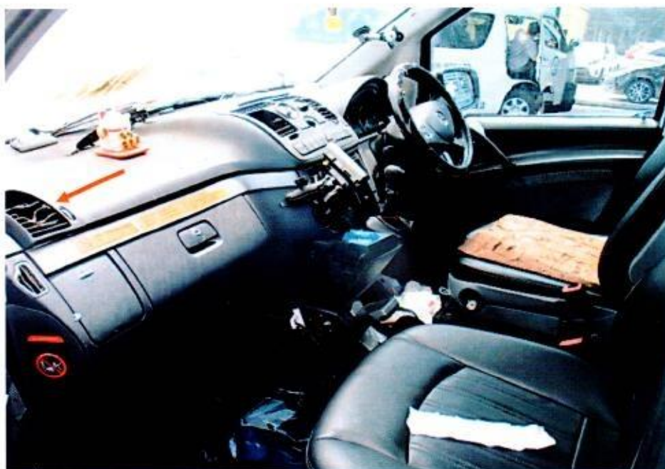
Photo 6 shows the interior compartment of the Insured Vehicle, which was observed to be slightly affected by the fire (arrowed).
