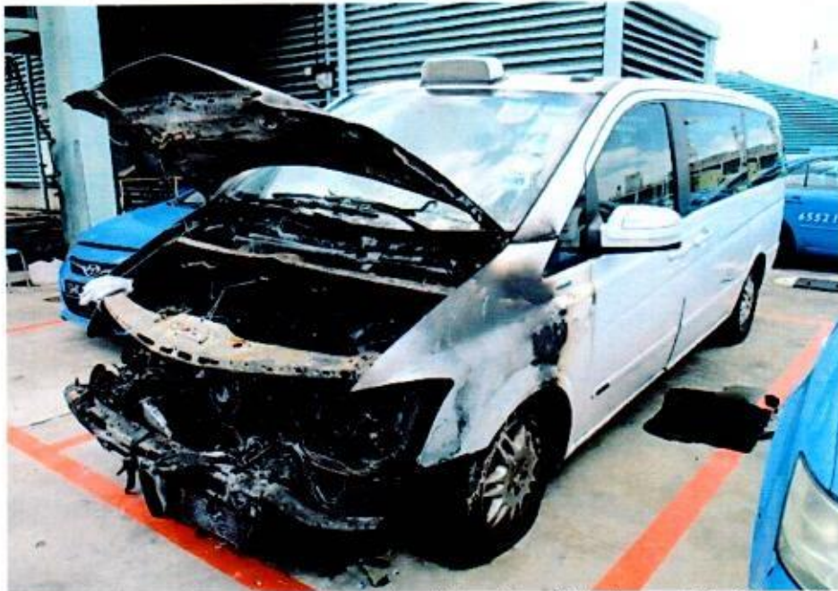
Photo 3 shows the general view of the left portion of the Insured Vehicle at the time of our inspection. The exterior body of the Insured Vehicle had sustained visible fire damage. This included its front windscreen, front bonnet, left headlight, front bumper, left front panel, left front wheel rim and left front tyre.
