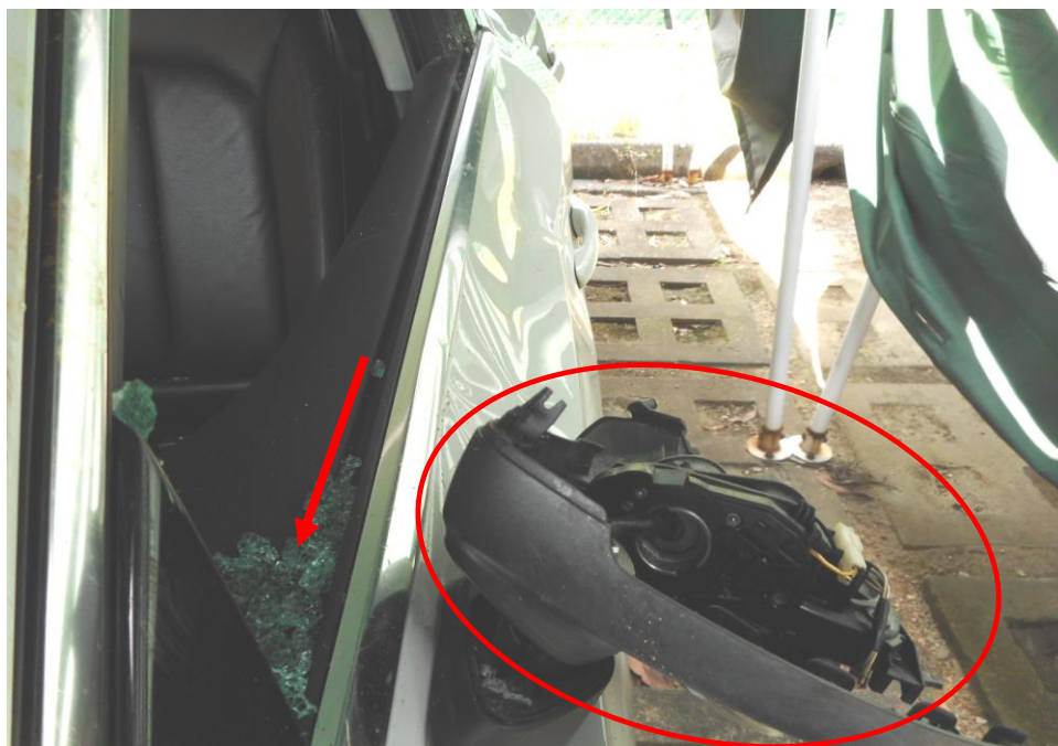
Photo 14 shows a close up view of the left rear view mirror (circled) and the left side windscreen (arrowed) of the Insured Vehicle upon our inspection. The severe damages on the left rear view mirror and windscreen correlate with Mr Maung's statement in which the Insured Vehicle was hit by a fallen tree branch.
