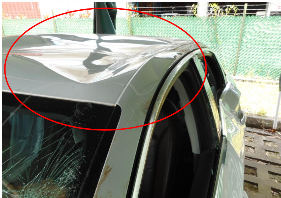
Photo 13 shows a close up view of the roof of the Insured Vehicle upon our inspection. The severe damages on the roof correlate with Mr Maung's statement in which the Insured Vehicle was hit by a fallen tree branch.
