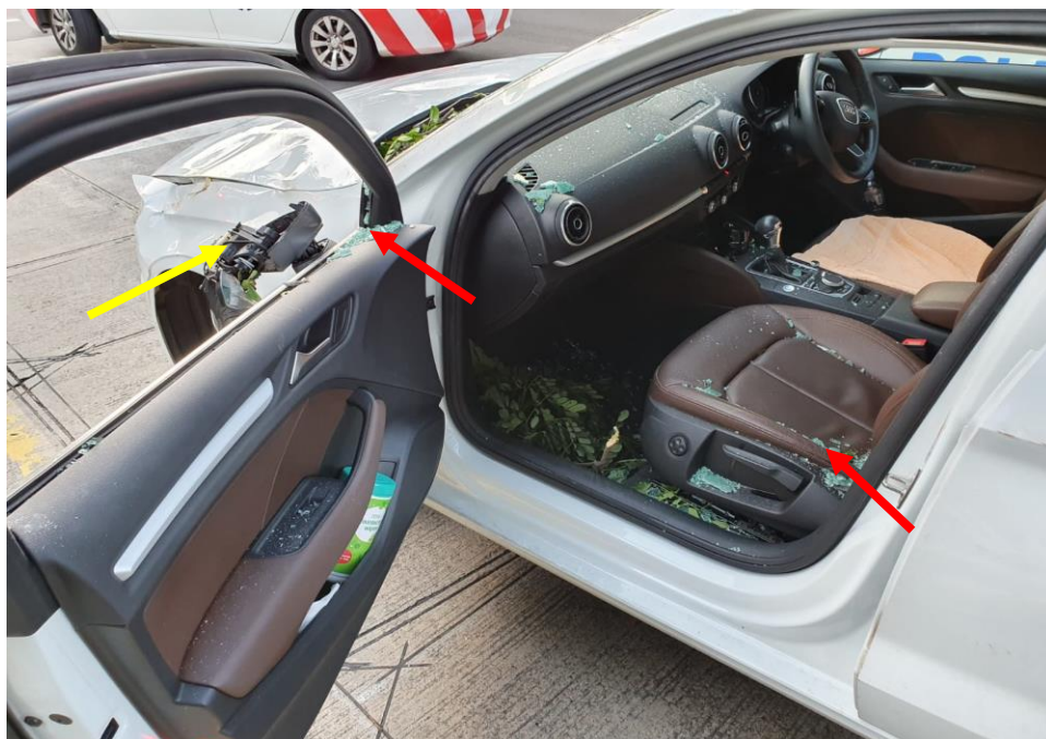
Photo 9 shows the shattered front and left side windscreen (red arrow) and the left rear view mirror (yellow arrow) due to the impact of the fallen tree branch (as seen from the interior of the Insured Vehicle).
