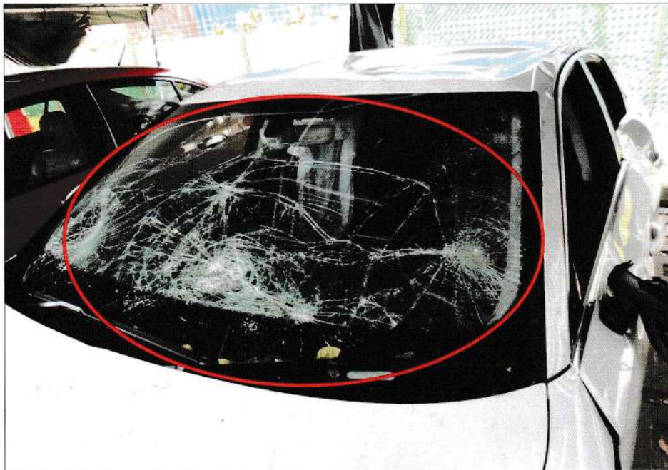
Photo 12 shows the front view of the Insured Vehicle upon our inspection. The severe damages on the front windscreen (circled) correlates with Mr Maung's statement in which the Insured Vehicle was hit by a fallen tree branch.
