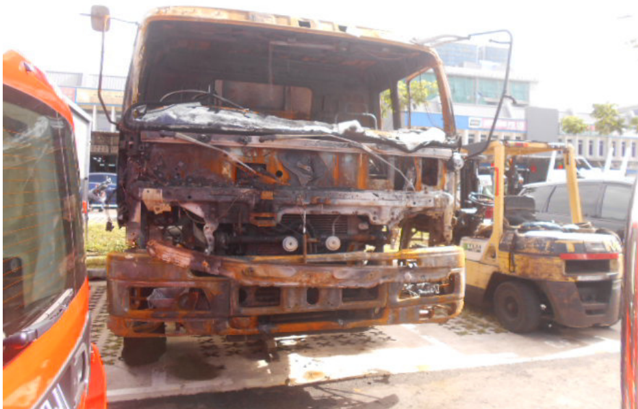
Photo 1 shows a general view of the front body of the Insured Vehicle at the time of inspection. The Insured Vehicle was observed to have sustained extensive fire damage at its frontal portion. The body panels at the frontal portion and the undercarriage components at the front underside were found to have been burnt to char.
