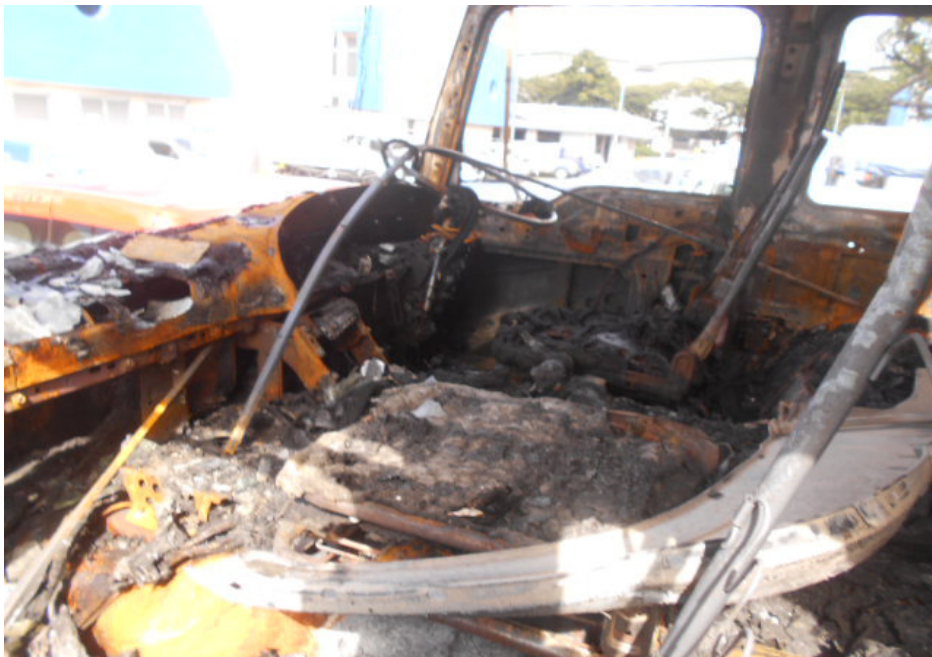
Photo 3 shows the interior compartment of the Insured Vehicle. All the parts inside the interior compartment were found to be burnt and/or melted. Its front seats, rear seats, roof upholstery, carpet and various trims were all burnt and/or melted as a result of the fire.
