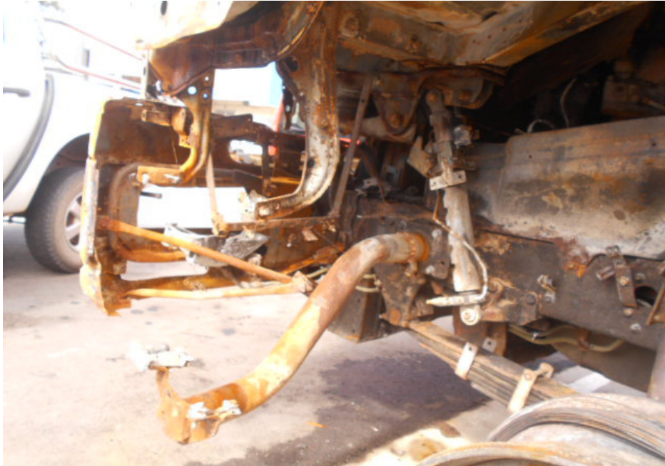
Photo 4 shows the underside of the Insured Vehicle, at its front left area. The various undercarriage components at the front underside of the Insured Vehicle were observed to be affected. This had included components of the braking system and steering system.
