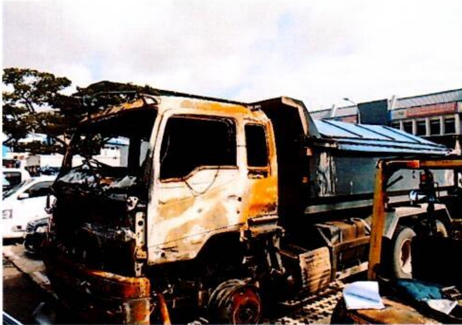
Photo 2 shows a general view of the front left body of the Insured Vehicle at the time of inspection. The Insured Vehicle was observed to have sustained extensive fire damage at its frontal portion. The body panels at the frontal portion were found to have been burnt to char.
