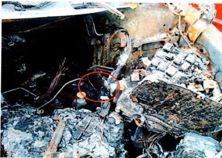
Photo 11 shows a closer view the greenish residue on several stretches of burnt wirings at the rear left portion of the engine compartment (circled), a sign of an electrical short circuit occurring. The greenish residue is normally left behind from oxidation as a result of chemical reaction involving the copper wires.
