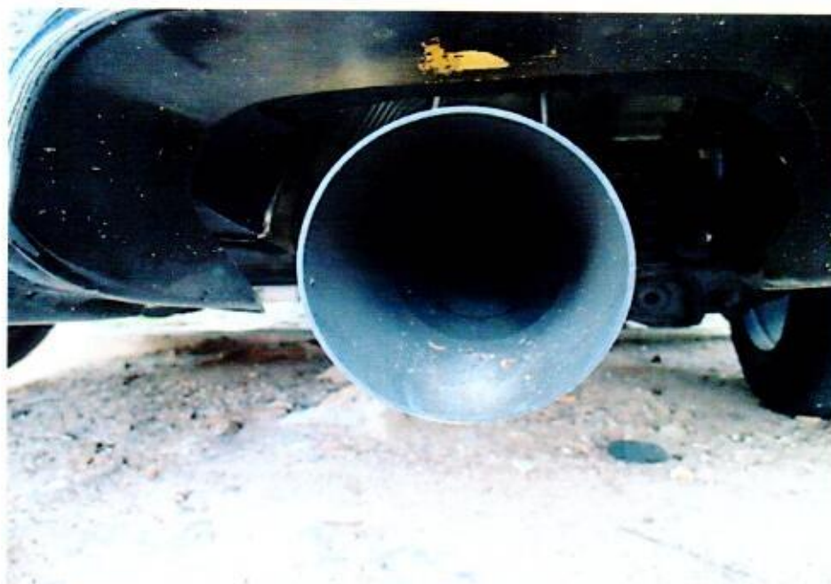
Photo 7 shows a front view of the non-standard rear exhaust muffler that was found to be fitted on the Insured Vehicle at the time of our inspection.
