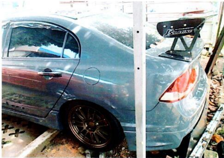
Photo 1 shows the rear left view of the Insured Vehicle. The rear portion of the Insured Vehicle was observed to be relatively unaffected by the fire.
