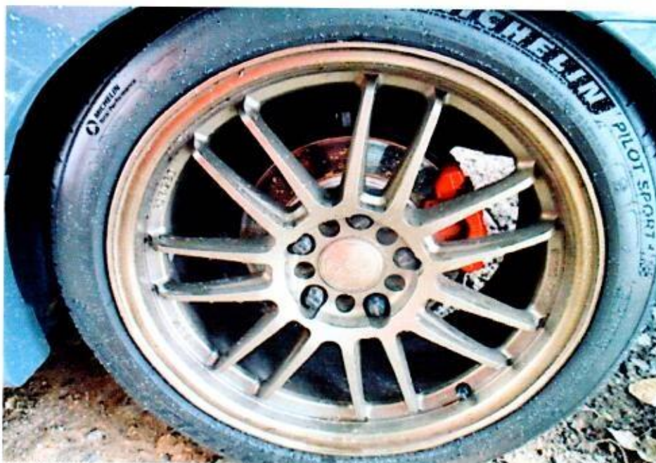
Photo 9 shows the non-standard rim found to be fitted on the Insured Vehicle at the time of our inspection. The 17- inch alloy rims fitted on the Insured Vehicle were not the standard type for the Insured Vehicle.
