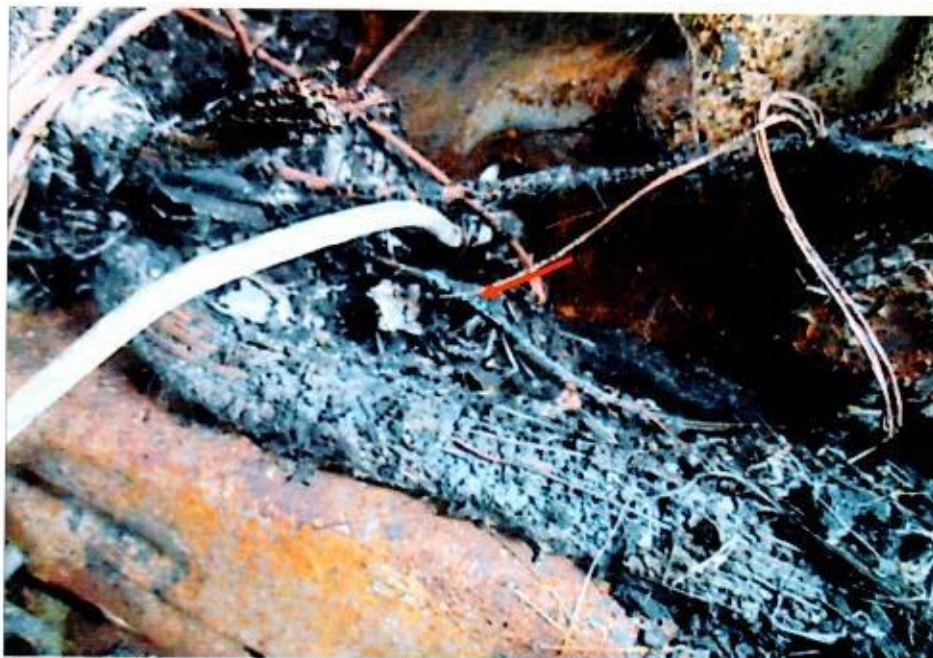
Photo 12 shows a close up view of the greenish residue on the wirings at the rear portion of the engine compartment (arrowed). The presence of such greenish residue suggests occurrence of an electrical short circuit.
