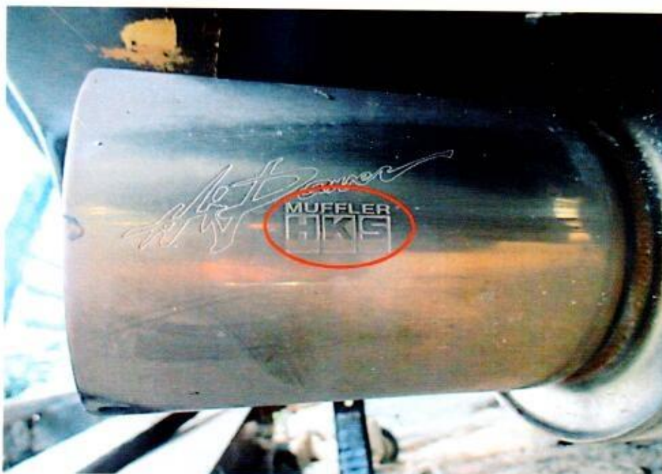
Photo 8 shows a close up right side view of the non-standard rear exhaust muffler that was found to be fitted on the Insured Vehicle at the time of our inspection. The brand of the rear exhaust muffler was 'HKS' (circled).
