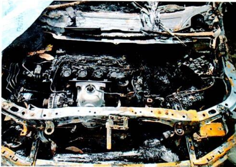
Photo 5 shows a general view of the engine compartment of the Insured Vehicle at the time of our inspection. Most of the components inside the engine compartment were found to be severely burnt and/or melted as a result of the fire.
