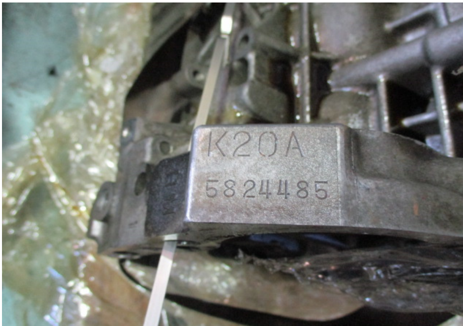
Photo 4 shows the engine number engraved on the housing of the Honda engine that I had inspected. The engine number was K20A5824485.
