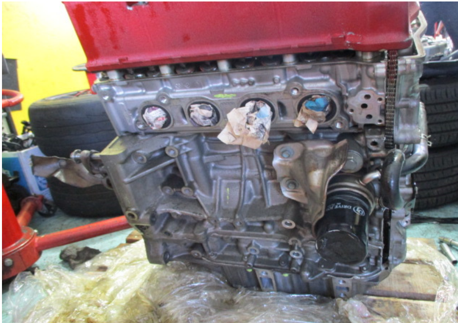
Photo 3 shows a closer view of the Honda engine that I had inspected. My visual examination of the engine housing revealed the housing to be of serviceable/satisfactory condition. There was no crack and/or hole observed on the engine housing.
