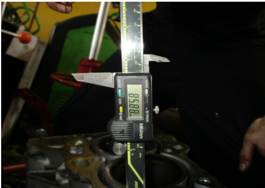
Photo 14 shows the stroke measurement of cylinder 2, which was recorded to be 85.88mm.
