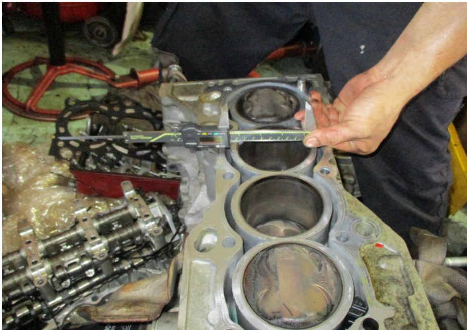
Photo 15 shows measurement being carried out to the bore of cylinder 3 of the Honda engine. The bore and stroke measurements of the Honda engine were carried out using a digital Vernier Caliper.
