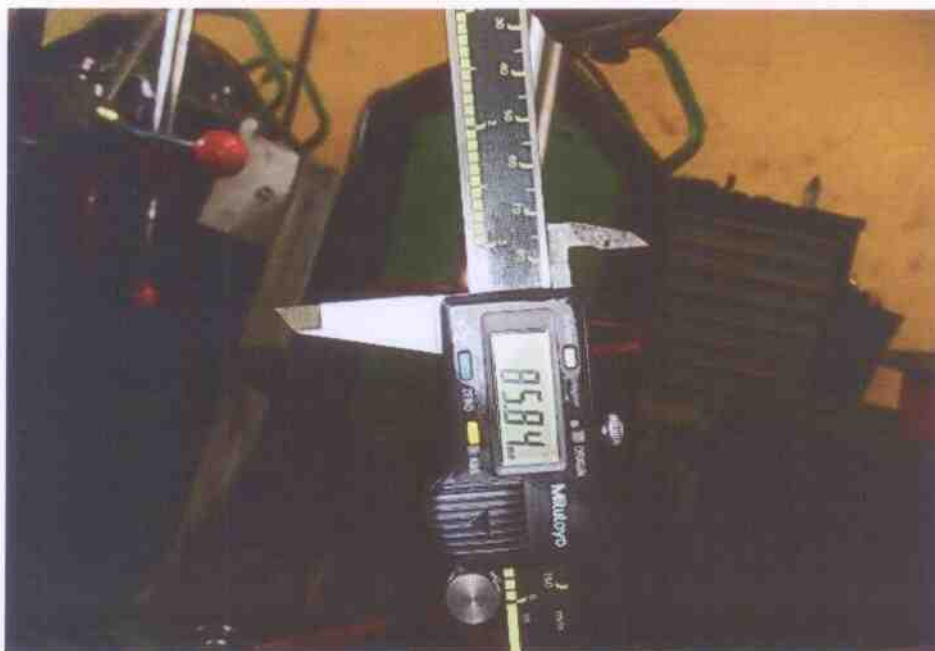
Photo 22 shows the stroke measurement of cylinder 4, which was recorded to be 85.84mm.
