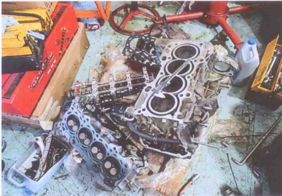
Photo 5 shows the top block of the Honda engine separated from its bottom block. This was to enable me to carry out measurements of its cylinders, in particular the bore and stroke measurements of each cylinder, which typically can be used to determine the engine displacement or more commonly referred to as engine cc.
