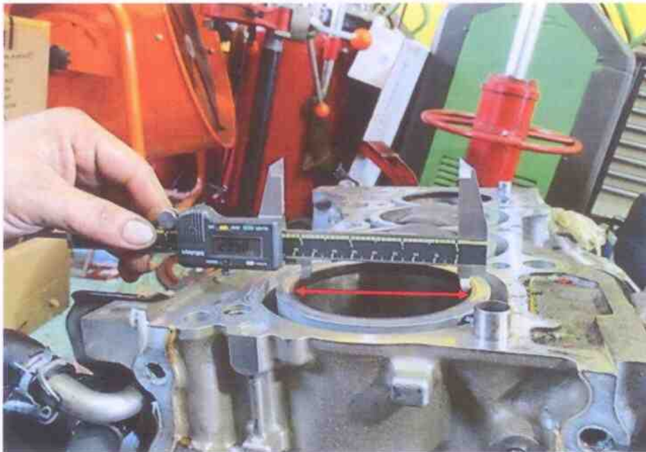
Photo 7 shows measurement being carried out to the bore (arrowed) of cylinder 1 of the Honda engine. The measurements were carried out using a digital Vernier Caliper that was calibrated before the start of the measurements.
