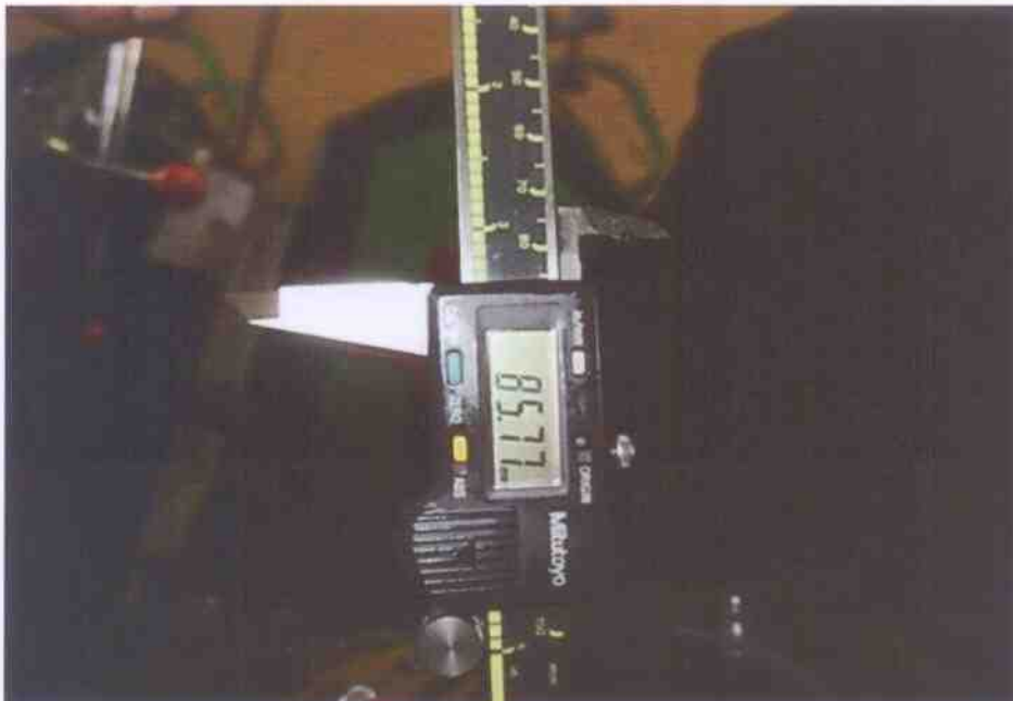
Photo 18 shows the stroke measurement of cylinder 3, which was recorded to be 85.77mm.
