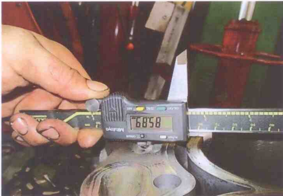
Photo 20 shows the bore measurement of cylinder 4, which was recorded to be 85.89mm.
