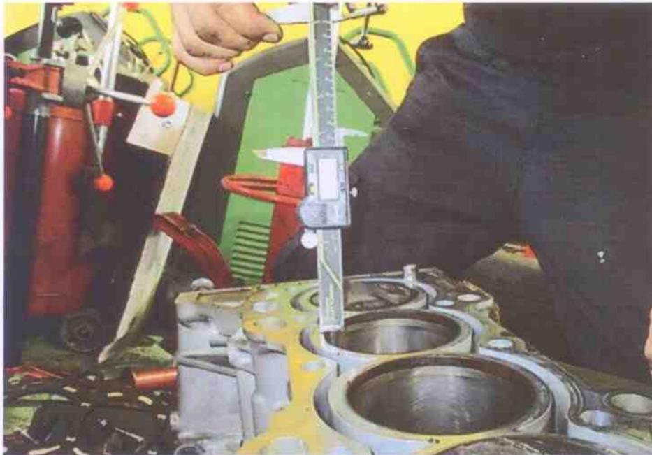
Photo 17 shows measurement of the stroke for cylinder 3 of the Honda engine that I had inspected. The bore and stroke measurements of the Honda engine were carried out using a digital Vernier Caliper that was calibrated before the start of measurements.
