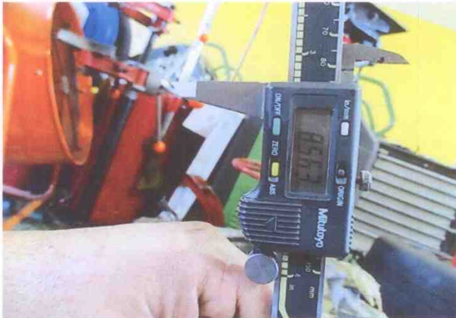
Photo 11 shows the stroke measurement of cylinder 1, which was recorded to be 85.63mm.
