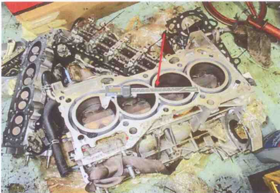
Photo 6 shows the bottom block of the Honda engine and the digital Vernier Caliper (arrowed) that was used to measure the bore and stroke measurements of each cylinder, which typically can be used to determine the engine displacement or more commonly referred to as engine cc. The digital Vernier Caliper was calibrated before the start of the measurements.
