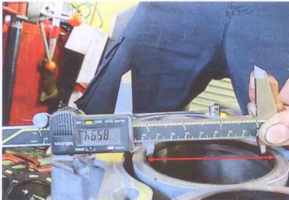
Photo 16 shows measurement being carried out to the bore (arrowed) of cylinder 3 of the Honda engine. The bore measurement of cylinder 3 was recorded to be 85.94mm.
