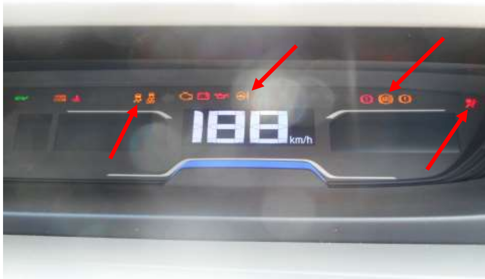
Photo 22 shows the warning light for Anti-Lock Brake System (ABS), Traction Control (TC), Supplemental Restraint System (SRS) and Electric Power Steering System (EPS) appearing on the instrument panel of the Motor Car during the self-test of its various electronic operating systems when its engine was cranked.
