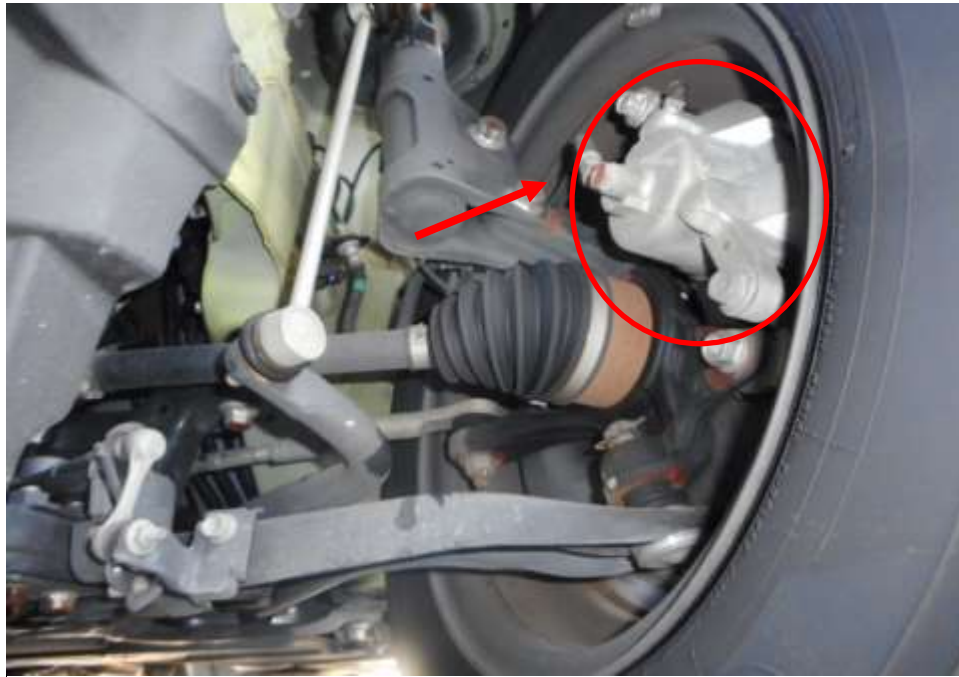
Photo 20 shows the brake hose/pipe (arrowed) at the front left wheel of the Motor Car. No leakage of brake fluid was observed. Visual examination of the various components of the braking system like the brake caliper (circled), brake booster, brake pedal etc had revealed all to be intact and without visible damage at the time of accident. There was also no sign of fluid stain(s) observed on the various undercarriage components.
