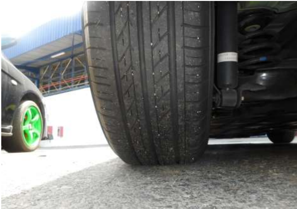
Photo 8 shows the condition of the rear left tyres of the Motor Car, which was observed to be in serviceable condition with remaining tread depth of approximately 4mm. The tyres, which were wrapped around standard alloy wheel rim, were also observed to be sufficiently inflated for vehicular operation. There was also no damage found on all 4 alloy wheel rims of the Motor Car.
