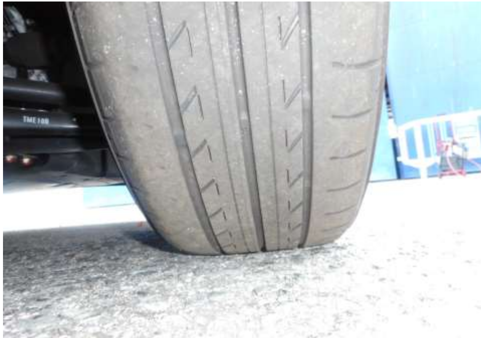
Photo 6 shows the condition of the front right tyre of the Motor Car, which was observed to be in serviceable condition with remaining tread depth of approximately 3.3mm. The tyre, which was wrapped around standard alloy wheel rim, was also observed to be sufficiently inflated for vehicular operation. There was no tear, cut or burst mark(s) on the outer and the inner sidewalls as well as across the tread of the 4 tyres that were fitted on the Motor Car.
