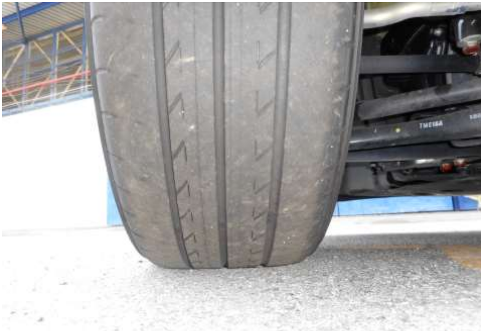
Photo 9 shows the condition of the rear right tyres of the Motor Car, which were observed to be in serviceable condition with remaining, tread depth of approximately 2.9mm. There was also no tear, cut or burst mark(s) on the outer and the inner sidewalls as well as across the tread of the 4 tyres that were fitted on the Motor Car.
