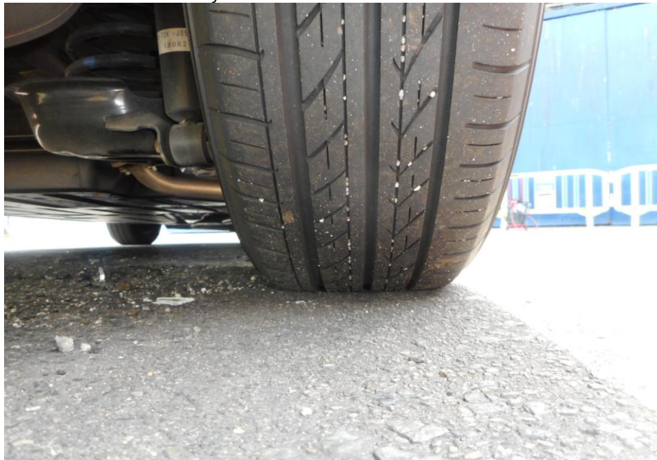
Photo 7 shows the condition of the rear right tyre of the Motor Car, which was observed to be in serviceable condition with remaining tread depth of approximately 5.1mm. The tyre, which was wrapped around standard alloy wheel rim, was also observed to be sufficiently inflated for vehicular operation.
