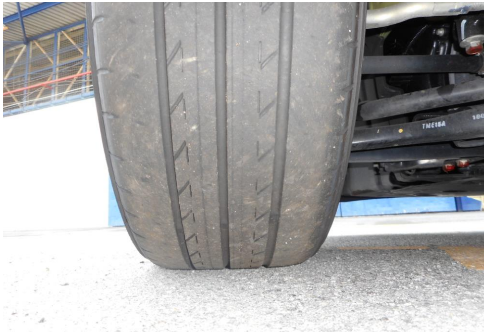
Photo 9 shows the condition of the rear right tyres of the Motor Car, which were observed to be in serviceable condition with remaining, tread depth of approximately 2.9mm. There was also no tear, cut or burst mark(s) on the outer and the inner sidewalls as well as across the tread of the 4 tyres that were fitted on the Motor Car.
