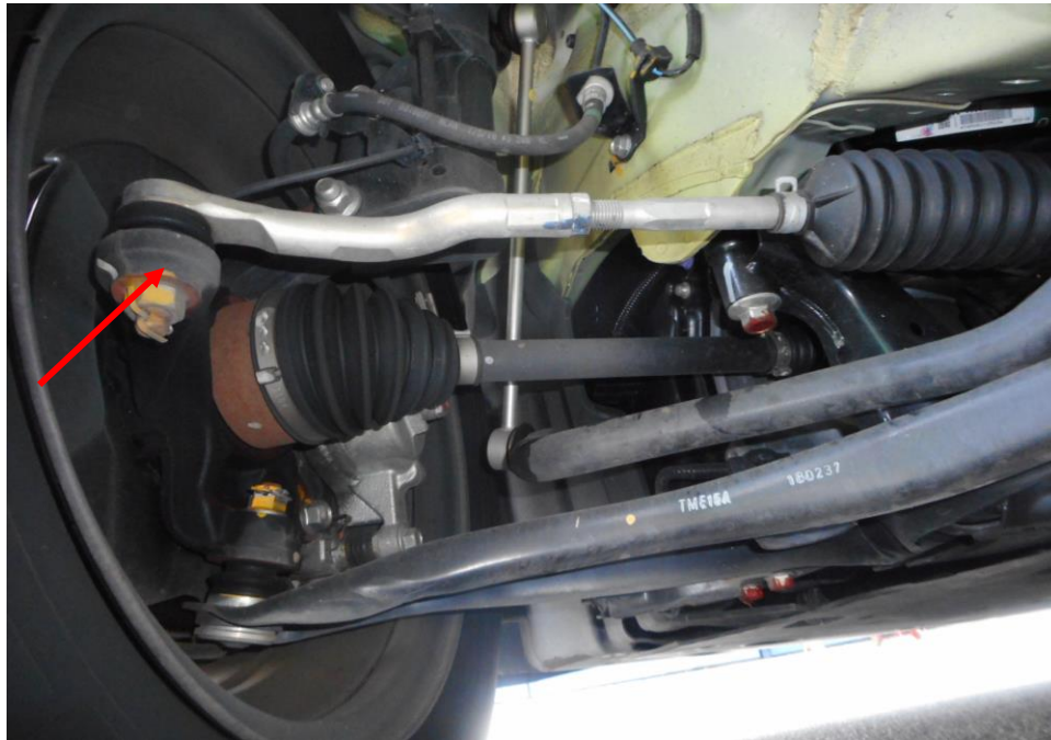
Photo 16 shows the various undercarriage components at the front left wheel of the Motor Car, in particular the steering tie rod end (arrowed). The various Undercarriage components of the Motor Car were all found to be intact without any visible damage. There was also no sign of fluid stain(s) observed on the various undercarriage components.
