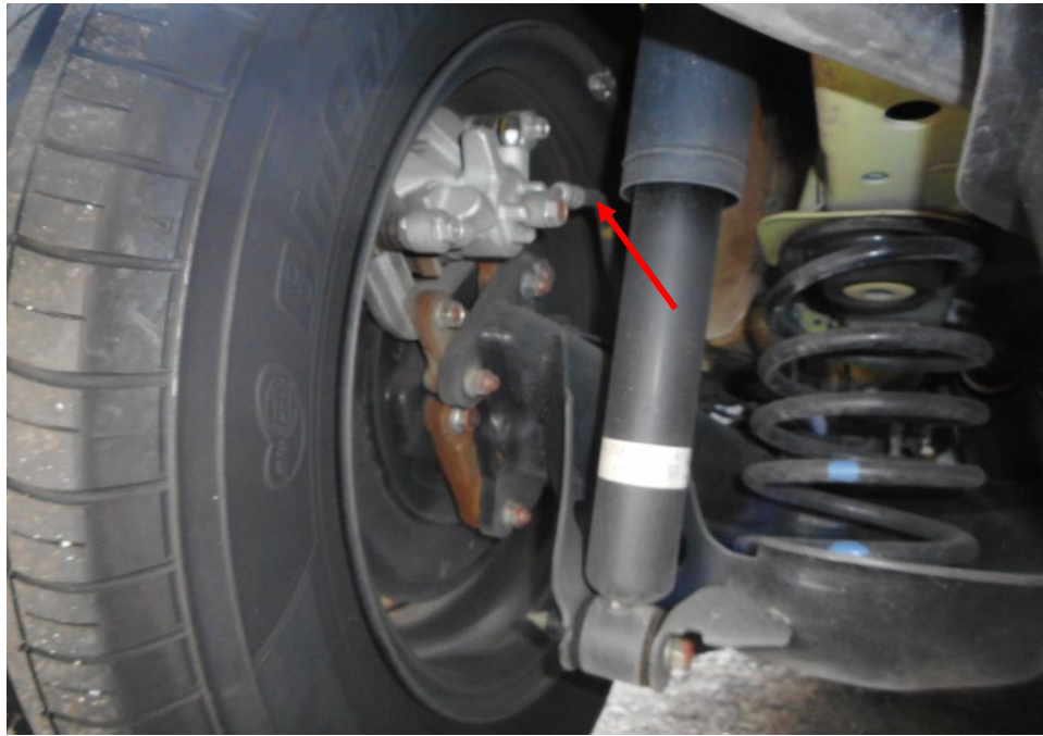
Photo 18 shows the brake pipe (arrowed) at the rear left wheel of the Motor Car. I did not observe any leakage of brake fluid at the time of my inspection of the Motor Car. My static tests of the Motor Car's braking system, along with my visual examination of the various mechanical components in the braking system had indicated that there was no internal leakage of pressure/vacuum. Hence the braking system of the Motor Car was likely to be in serviceable condition at the material time of accident.
