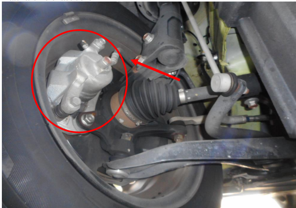
Photo 19 shows the brake hose/pipe (arrowed) at the front right wheel of the Motor Car. No leakage of brake fluid was observed. Visual examination of the various components of the braking system like the brake caliper (circled), brake booster, brake pedal etc had revealed all to be intact and without visible damage at the time of accident. There was also no sign of fluid stain(s) observed on the various undercarriage components.
