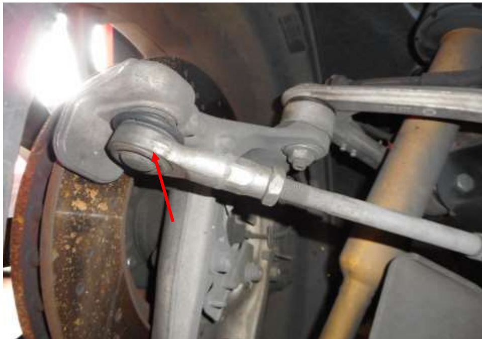
Photo 25 shows the various undercarriage components at the front right wheel of the Motor Car, in particular the steering tie rod end (arrowed). The various steering components were all found to be intact, suggesting that the steering system of the Motor Car was likely to be in serviceable condition at the material time of accident. There was also no sign of fluid stain(s) observed on the various undercarriage components.
