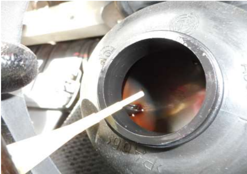
Photo 23 shows the power steering dip stick of the Motor Car at the time of my inspection. The power steering fluid was observed to be of lower level but sufficient for operating purposes.
