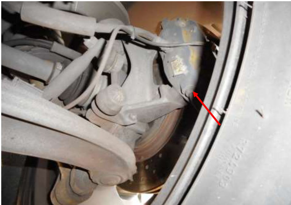
Photo 27 shows the brake pipe (arrowed) at the rear right wheel of the Motor Car. I did not observe any leakage of brake fluid at the time of my inspection of the Motor Car. My static tests of the Motor Car's braking system, along with my visual examination of the various mechanical components in the braking system, had indicated that there was no internal leakage of pressure/vacuum. Hence the braking system of the Motor Car was likely to be in serviceable condition at the material time of accident.
