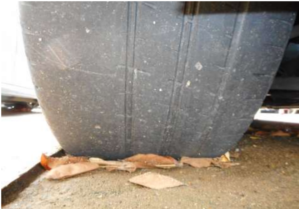
Photo 15 shows the condition of the rear left tyres of the Motor Car, which was observed to be in unserviceable condition with remaining tread depth of approximately 1.1mm which has exceeded the minimum legal limit. The tyres, which were wrapped around standard alloy wheel rim. There was no damage found on all 4 alloy wheel rims of the Motor Car.
