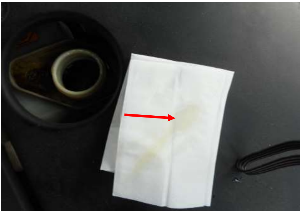
Photo 20 shows the brake fluid reservoir of the Motor Car at the time of my inspection. The brake fluid was observed to be of sufficient level and without any visible contamination (arrowed).
