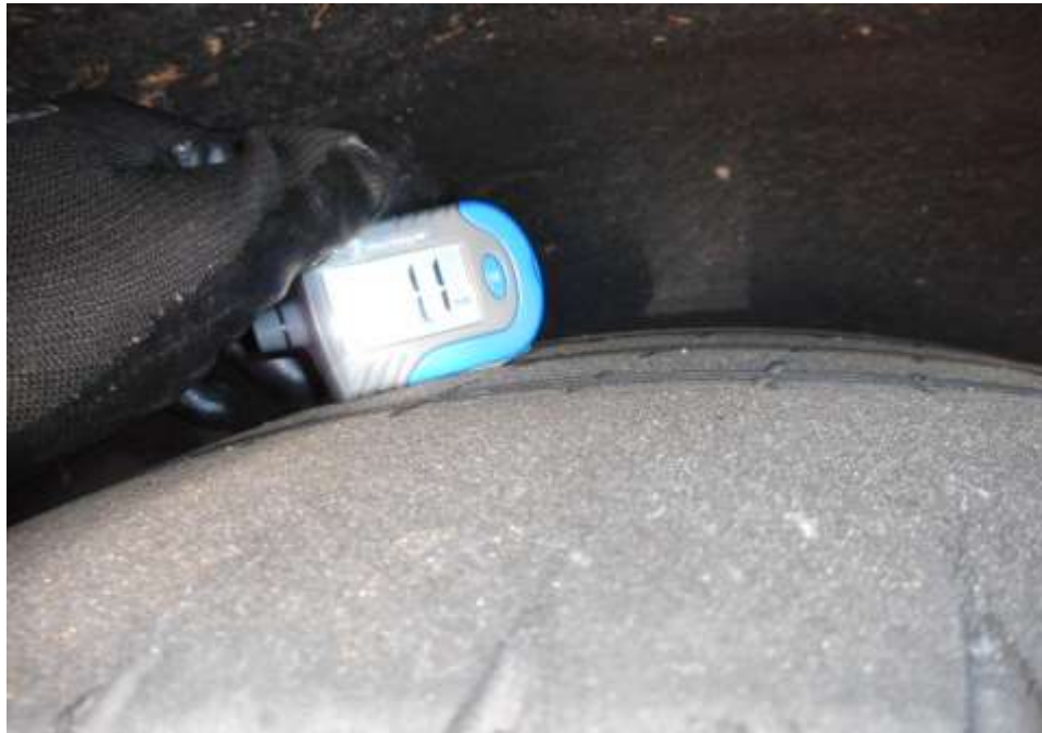
Photo 16 shows the condition of the rear left tyres of the Motor Car, which was observed to be in unserviceable condition with remaining tread depth of approximately 1.1mm which has exceeded the minimum legal limit.
