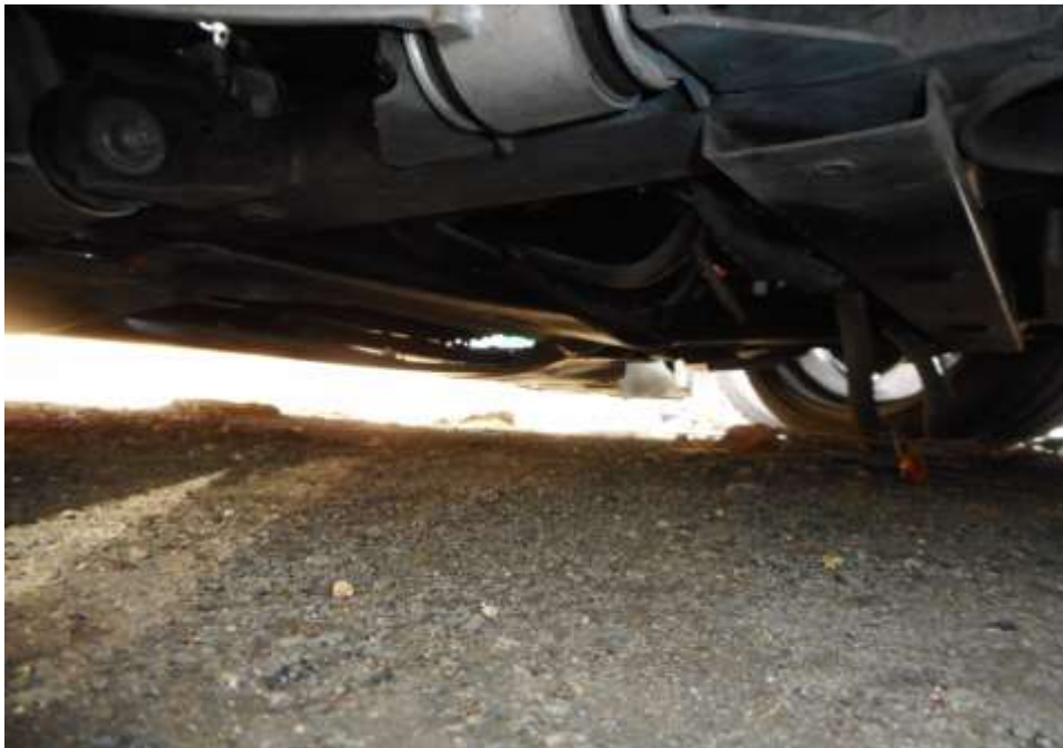
Photo 24 shows the undercarriage of the Motor Car, at the area where the engine housing and transmission housing are located. . I did not find any sign(s) or indication(s) of fluid leak and/or fluid stain(s) on the underside of the Motor Car.
