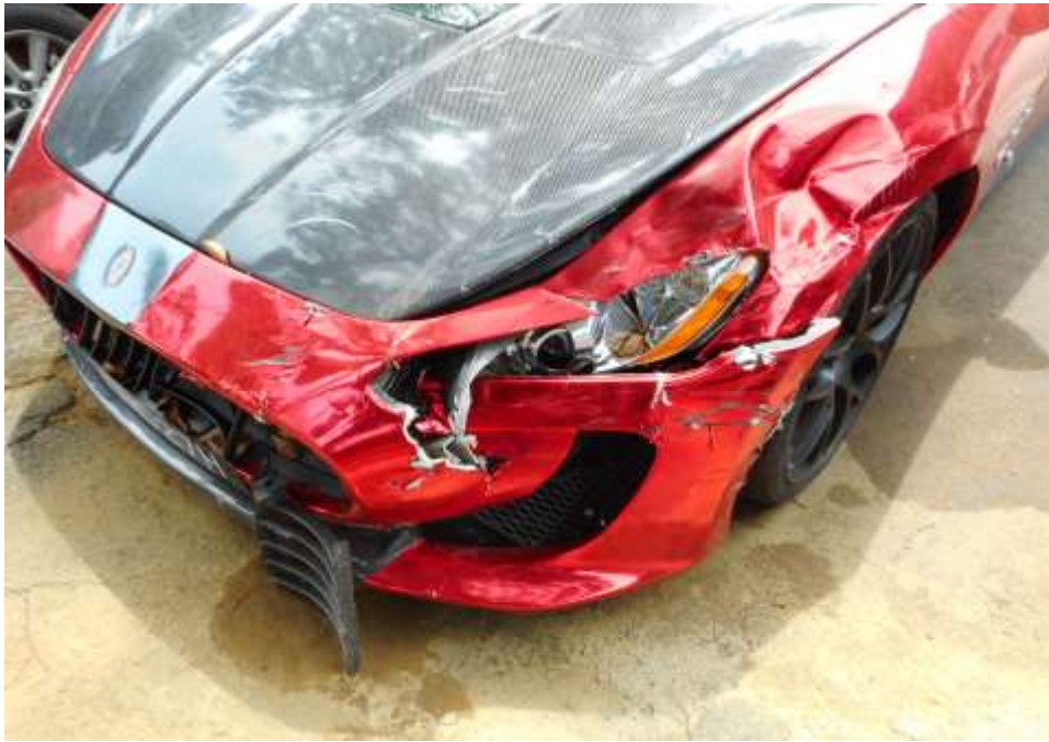
Photo 4 shows a general view of the Motor Car's frontal portion at the time of my inspection. Its front bonnet, front bumper, front grille, front left headlamp, front left fender and left rear view mirror were damage at the time of my inspection.
