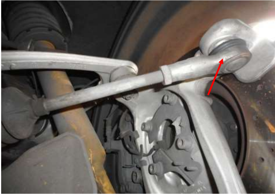
Photo 26 shows the various undercarriage components at the front left wheel of the Motor Car, in particular the steering tie rod end (arrowed). The various Undercarriage components of the Motor Car were all found to be intact without any visible damage. There was also no sign of fluid stain(s) observed on the various undercarriage components.
