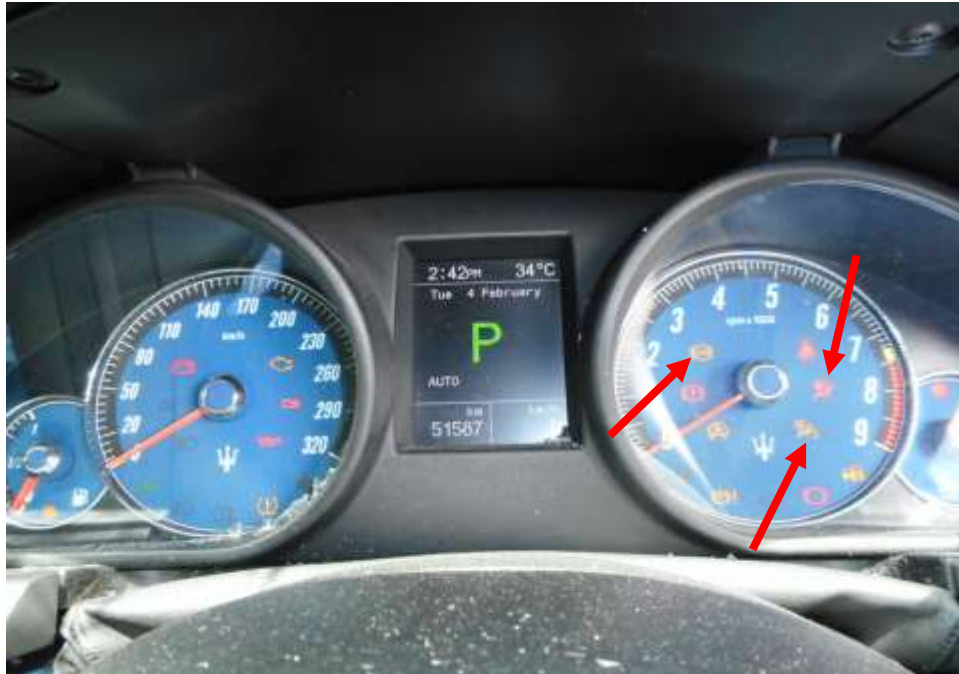
Photo 33 shows the warning light for Anti-Lock Brake System (ABS) and Supplemental Restraint System (SRS) and Traction Control System (TC) appearing on the instrument panel of the Motor Car during the self-test of its various electronic operating systems when its engine was cranked.
