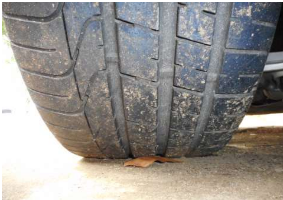
Photo 17 shows the condition of the rear right tyres of the Motor Car, which were observed to be in serviceable condition with remaining, tread depth of approximately 5mm. There was also no tear, cut or burst mark(s) on the outer and the inner sidewalls as well as across the tread of the 4 tyres that were fitted on the Motor Car.
