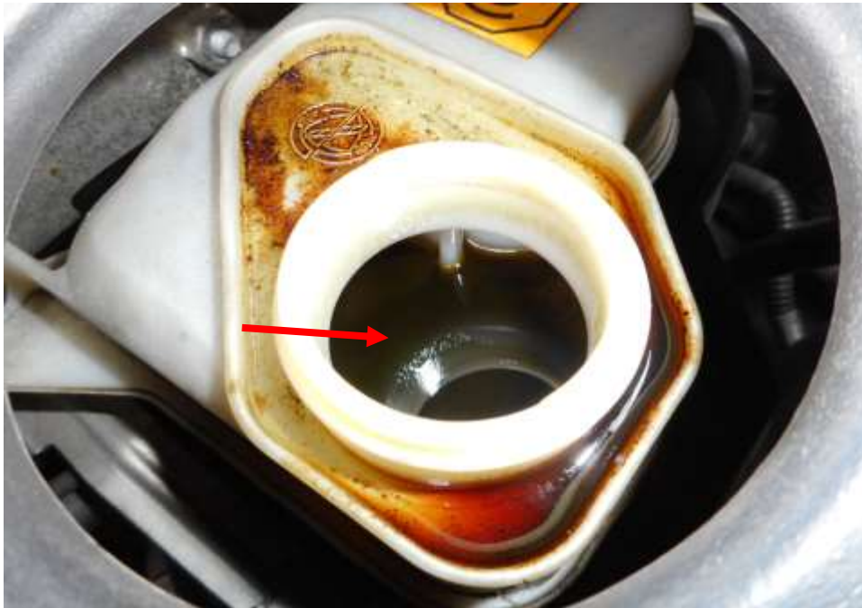
Photo 19 shows the brake fluid reservoir of the Motor Car at the time of my inspection. The brake fluid was observed to be of sufficient level (arrowed) and without any visible contamination.
