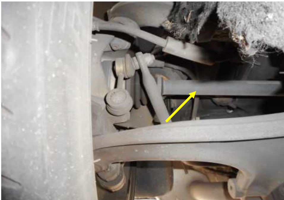
Photo 31 shows the various undercarriage components at the rear left wheel of the Motor Car. The drive shaft (yellow arrow) was found to be intact and there was no sign of fluid stain(s) observed on the various undercarriage components.
