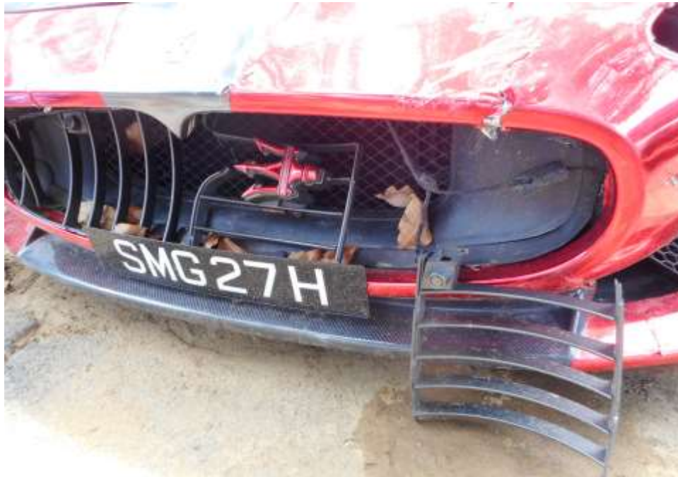
Photo 6 shows a close up view of the Motor Car's frontal portion at the time of my inspection. Its front grille was damage at the time of my inspection.
