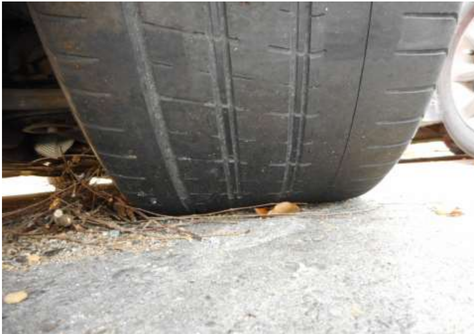
Photo 14 shows the condition of the rear right tyre of the Motor Car, which was observed to be in serviceable condition with remaining tread depth of approximately 1.9mm. The tyre, which was wrapped around standard alloy wheel rim, was also observed to be sufficiently inflated for vehicular operation.
