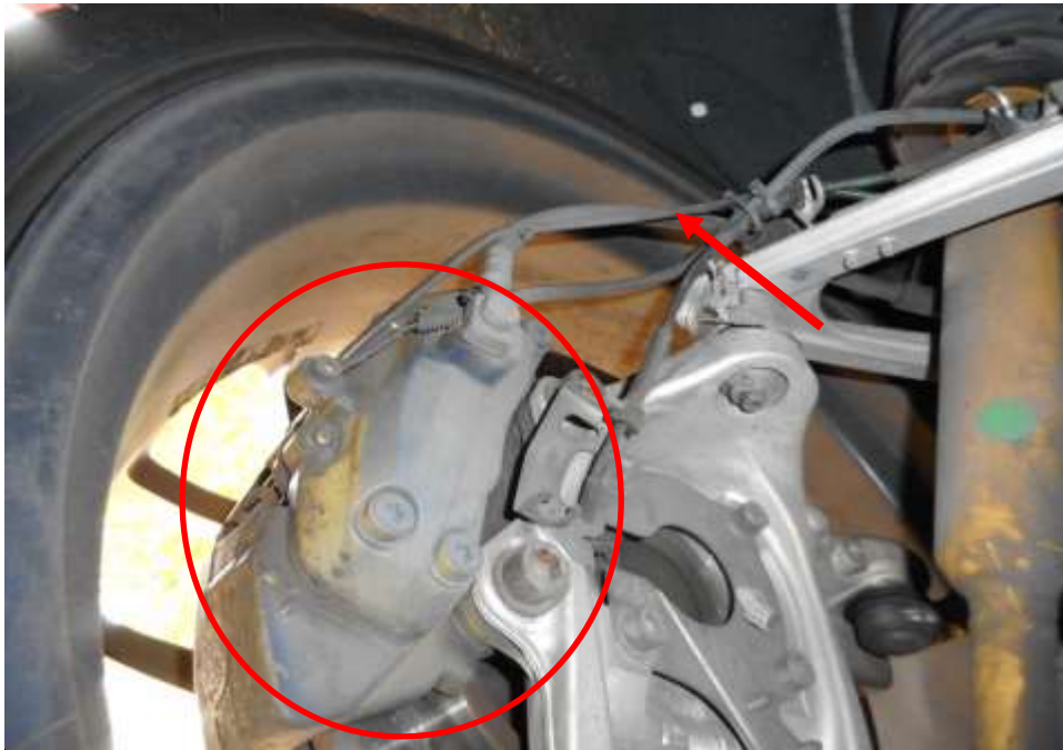
Photo 30 shows the brake hose/pipe (arrowed) at the front left wheel of the Motor Car. No leakage of brake fluid was observed. Visual examination of the various components of the braking system like the brake caliper (circled), brake booster, brake pedal etc had revealed all to be intact and without visible damage at the time of accident. There was also no sign of fluid stain(s) observed on the various undercarriage components.
