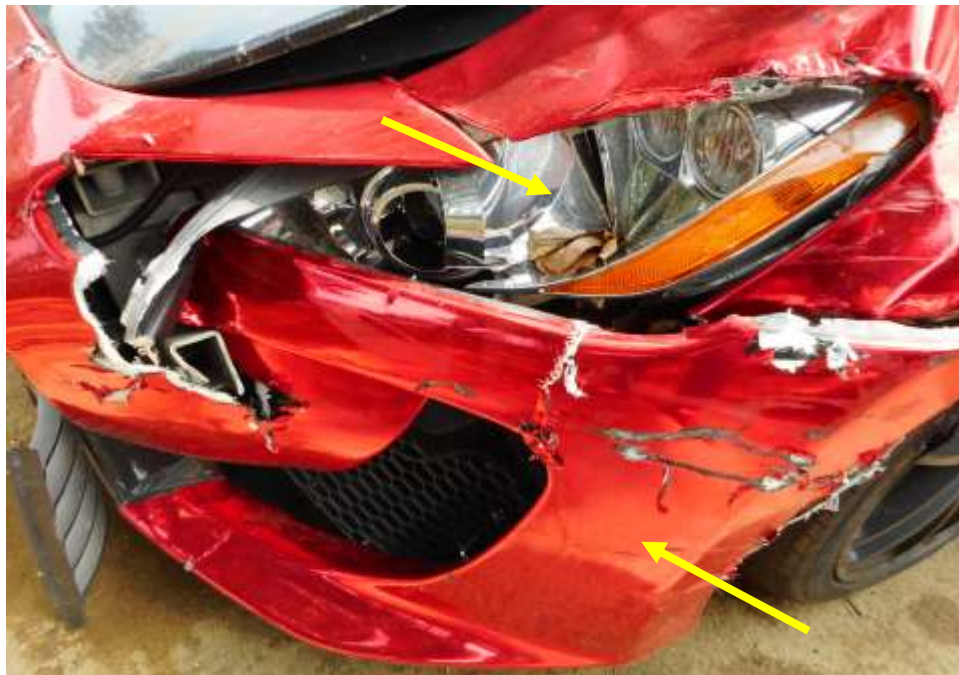
Photo 7 shows a close up view of the Motor Car's frontal portion at the time of my inspection. Its front bumper (arrowed) and front left headlamp (arrowed) were damage at the time of my inspection.
