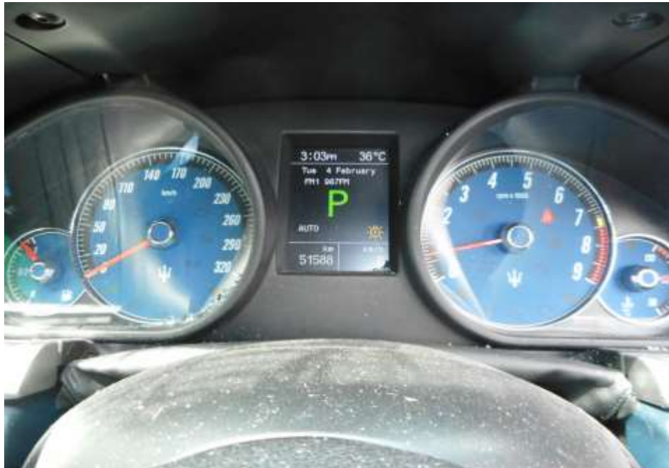
Photo 34 shows no warning lights illuminated on the instrument panel of the Motor Car after the engine was cranked. This would suggest that there was no abnormality to the various electronic operating systems of the Motor Car, like the ABS, SRS and TC.
