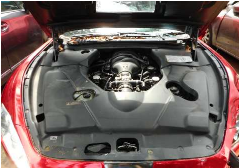
Photo 18 shows a general view of the Motor Car's engine compartment, which was accessed by lifting the front cabin of the Motor Car. The various parts and components inside the engine compartment were unaffected by the accident. There was also no sign(s) or indication(s) of fresh fluid leakage and/or fluid stain within the engine compartment
