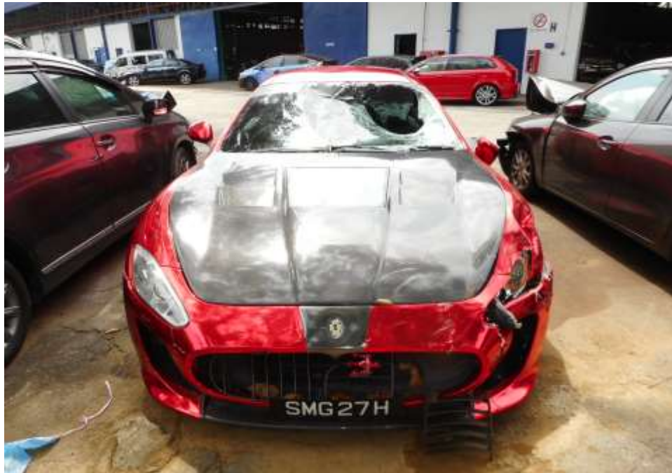
Photo 2 shows a general view of the Motor Car's frontal portion at the time of my inspection. It appeared to have sustained moderate damage at its frontal portion. Its front windscreen, front bonnet, front bumper, front grille, front left headlamp, front left fender and left rear view mirror were damage at the time of my inspection.
