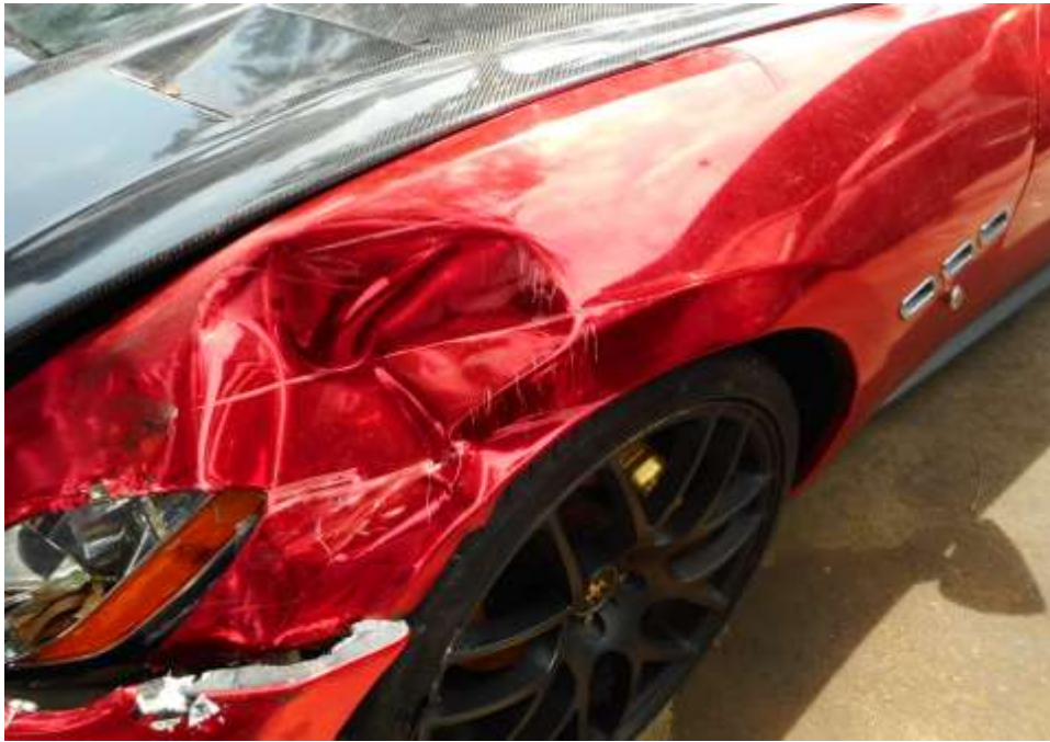
Photo 8 shows a close up view of the Motor Car's frontal portion at the time of my inspection. Its front left fender was damage at the time of my inspection.
