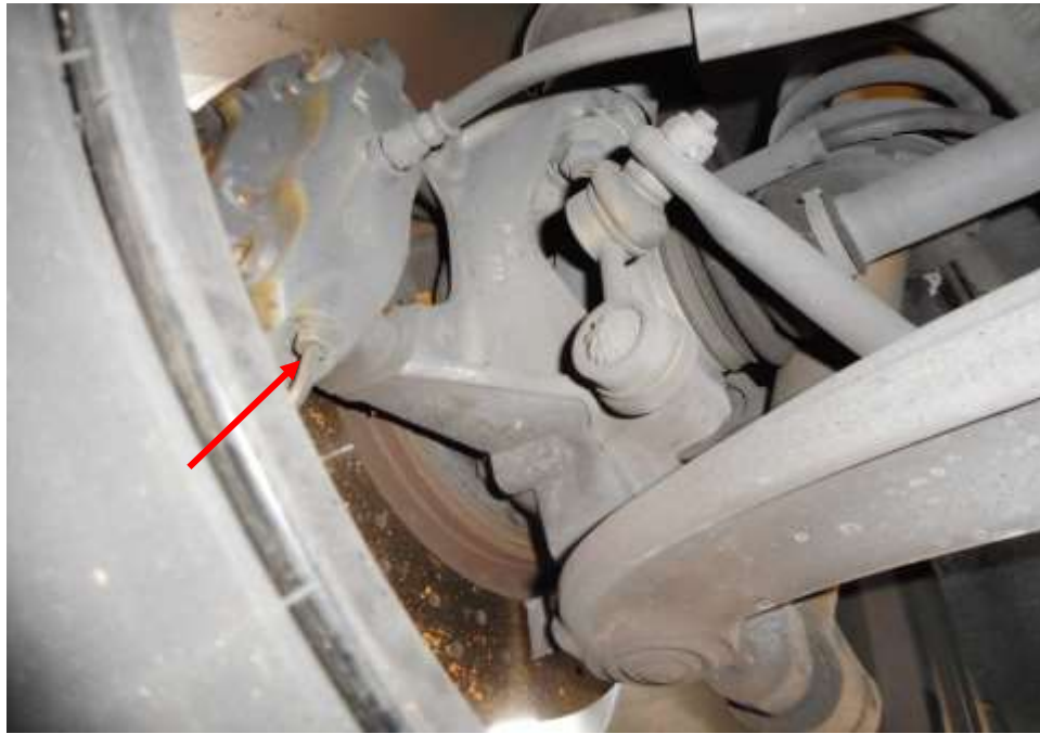
Photo 28 shows the brake pipe (arrowed) at the rear left wheel of the Motor Car. I did not observe any leakage of brake fluid at the time of my inspection of the Motor Car. My static tests of the Motor Car's braking system, along with my visual examination of the various mechanical components in the braking system had indicated that there was no internal leakage of pressure/vacuum. Hence the braking system of the Motor Car was likely to be in serviceable condition at the material time of accident.
