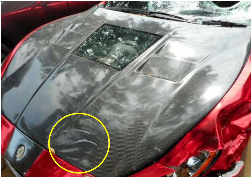
Photo 5 shows a close up view of the Motor Car's frontal portion at the time of my inspection. Its front bonnet (circled) was damage at the time of my inspection.
