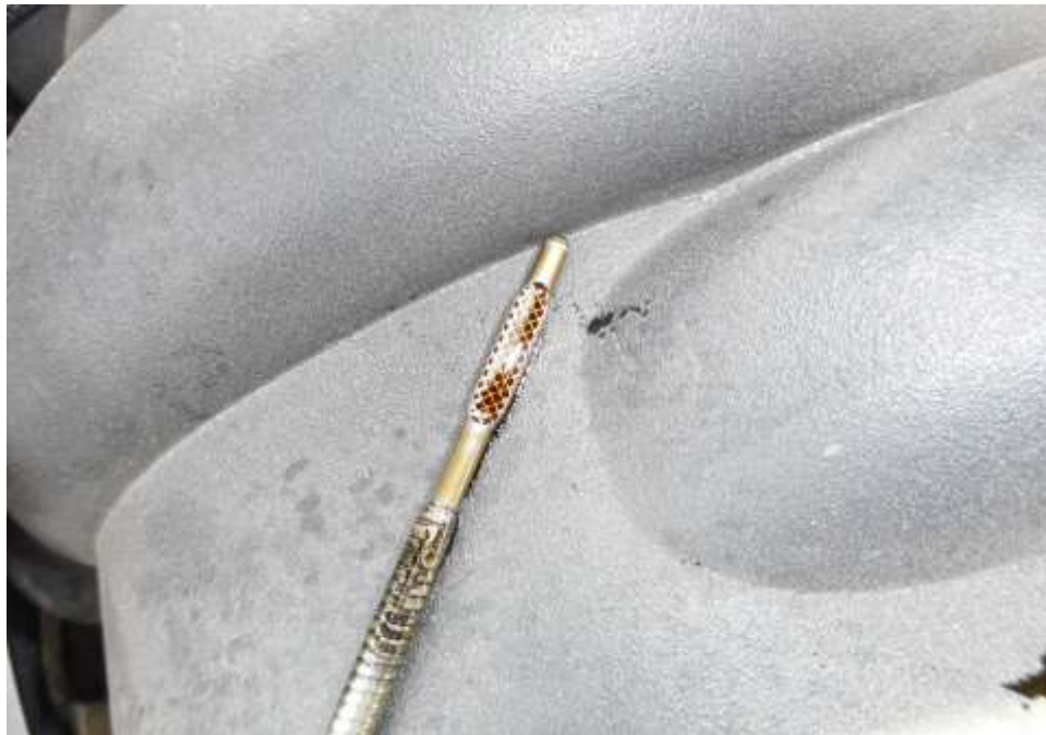
Photo 22 shows the engine oil dip stick of the Motor Car at the time of my inspection. The engine oil was observed to be of sufficient level and without any visible contamination.
