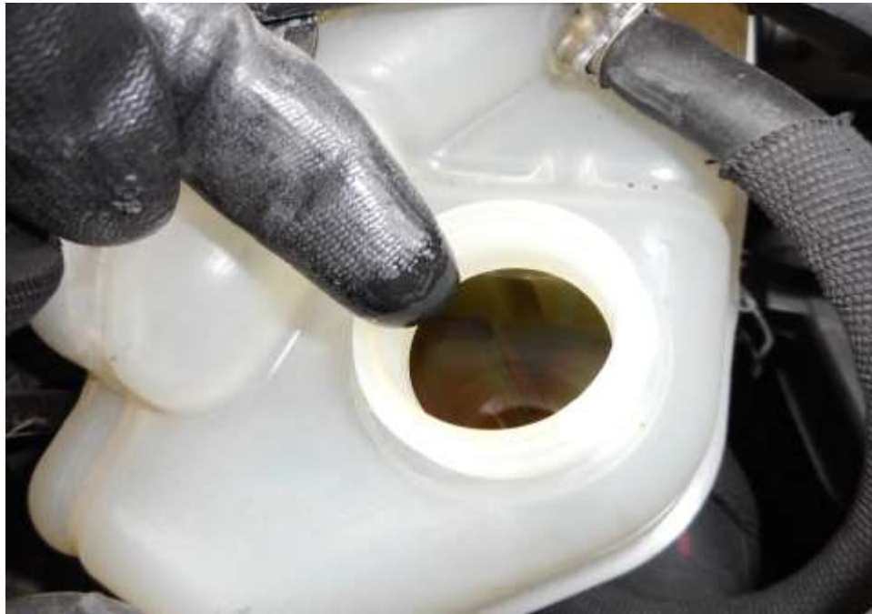
Photo 21 shows the engine coolant reservoir of the Motor Car at the time of my inspection. The engine coolant was observed to be of sufficient level and without any visible contamination.
