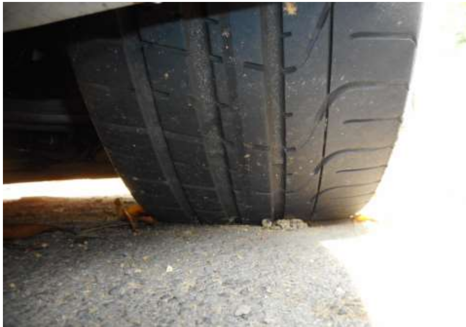
Photo 13 shows the condition of the front right tyre of the Motor Car, which was observed to be in serviceable condition with remaining tread depth of approximately 4.8mm. The tyre, which was wrapped around standard alloy wheel rim, was also observed to be sufficiently inflated for vehicular operation. There was no tear, cut or burst mark(s) on the outer and the inner sidewalls as well as across the tread of the 4 tyres that were fitted on the Motor Car.
