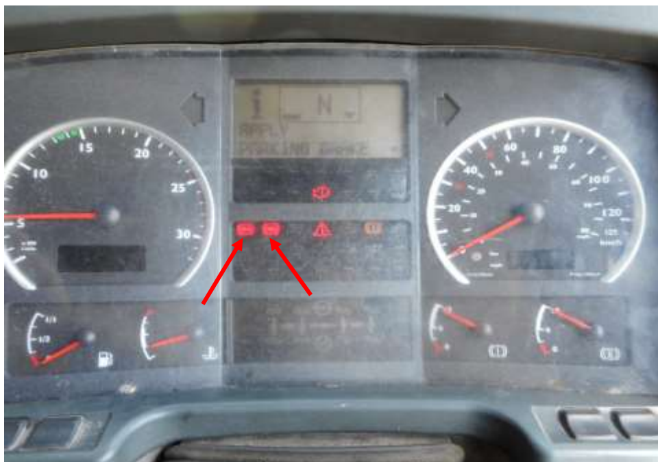
Photo 21 shows warning lights of the Anti-Lock Brake System (ABS) and Traction Control (TC) (arrowed) remained illuminated on the instrument panel of the Motor Trailer after the engine was cranked. This due a fault in the electrical system of the Motor Trailer.
