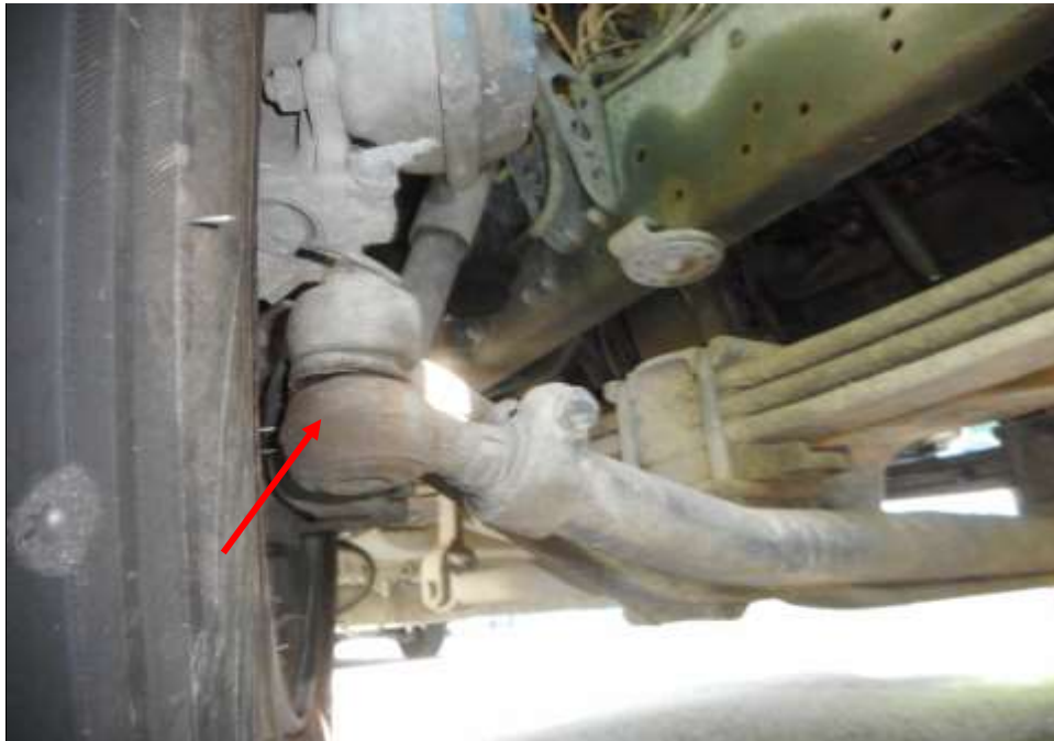
Photo 25 shows the various undercarriage components at the front left wheel of the Motor Trailer, in particular the steering tie rod end (arrowed). The various undercarriage components of the Motor Trailer were all found to be intact without any visible damage. There was also no sign of fluid stain(s) observed on the various undercarriage components.
