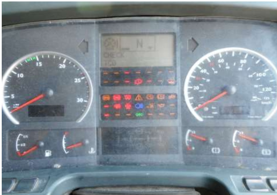
Photo 20 shows the warning light for Anti-Lock Brake System (ABS) and Traction Control (TC) appearing on the instrument panel of the Motor Trailer during the self-test of its various electronic operating systems when its engine was cranked.
