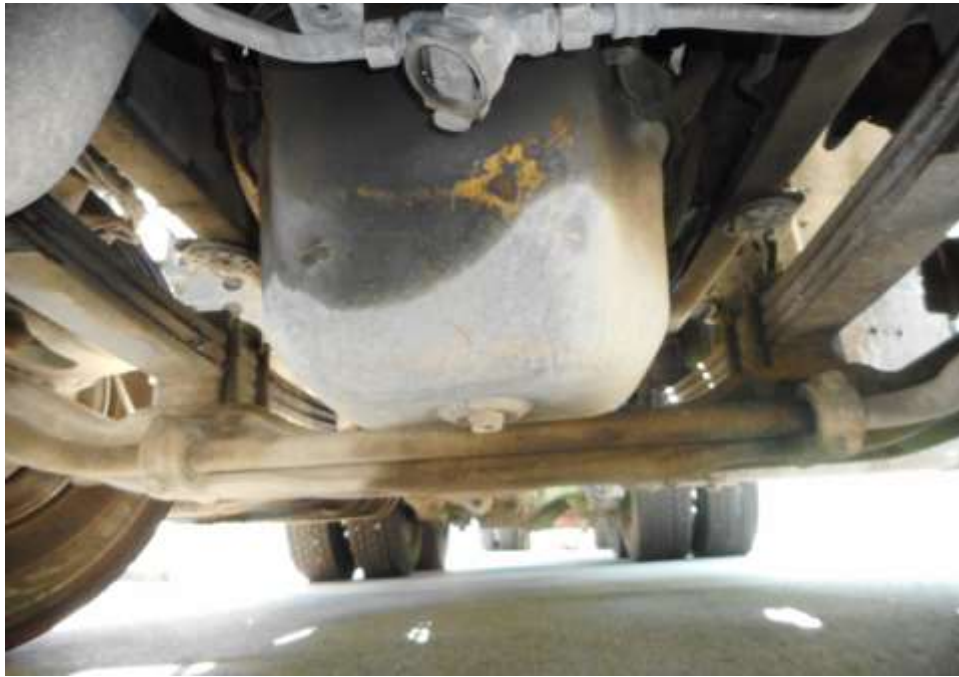
Photo 18 shows the undercarriage of the Motor Trailer, at the area where the engine housing located. I did not find any sign(s) or indication(s) of fluid leak, or fluid stain(s) was observed on the underside of the Motor Trailer.
