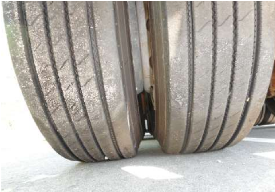
Photo 15 shows the condition of the left tyres of the trailer, which was observed to be in serviceable condition with remaining tread depth of approximately 12.5mm. The tyres, which were wrapped around standard steel wheel rim, were also observed to be sufficiently inflated for vehicular operation. There was also no damage found on all 22 steel wheel rims of the Motor Trailer.
