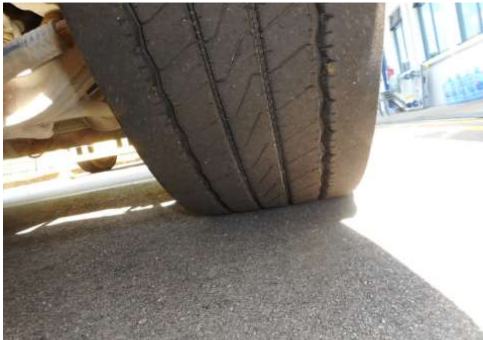
Photo 10 shows the condition of the front right tyre of the Motor Trailer, which was observed to be in serviceable condition with remaining tread depth of approximately 9.7 mm. The tyre, which was wrapped around standard steel wheel rim, was also observed to be sufficiently inflated for vehicular operation. There was no tear, cut or burst mark(s) on the outer and the inner sidewalls as well as across the tread of the 22 tyres that were fitted on the Motor Trailer.
