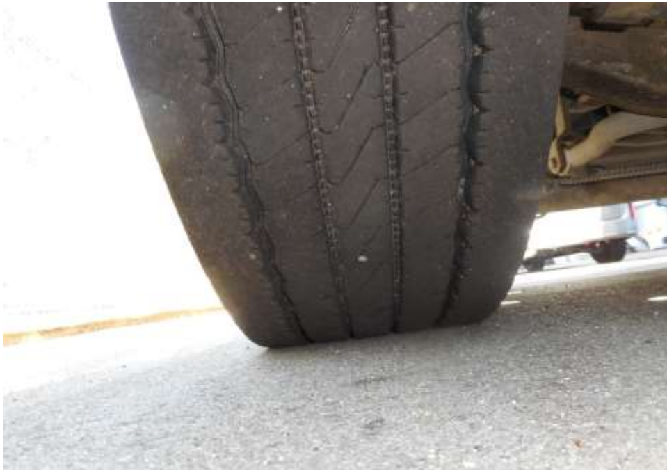
Photo 13 shows the condition of the front left tyres of the Motor Trailer, which were observed to be in serviceable condition with remaining tread depth of approximately 9.7mm. There was also no tear, cut or burst mark(s) on the outer and the inner sidewalls as well as across the tread of the 6 tyres that were fitted on the Motor Trailer.
