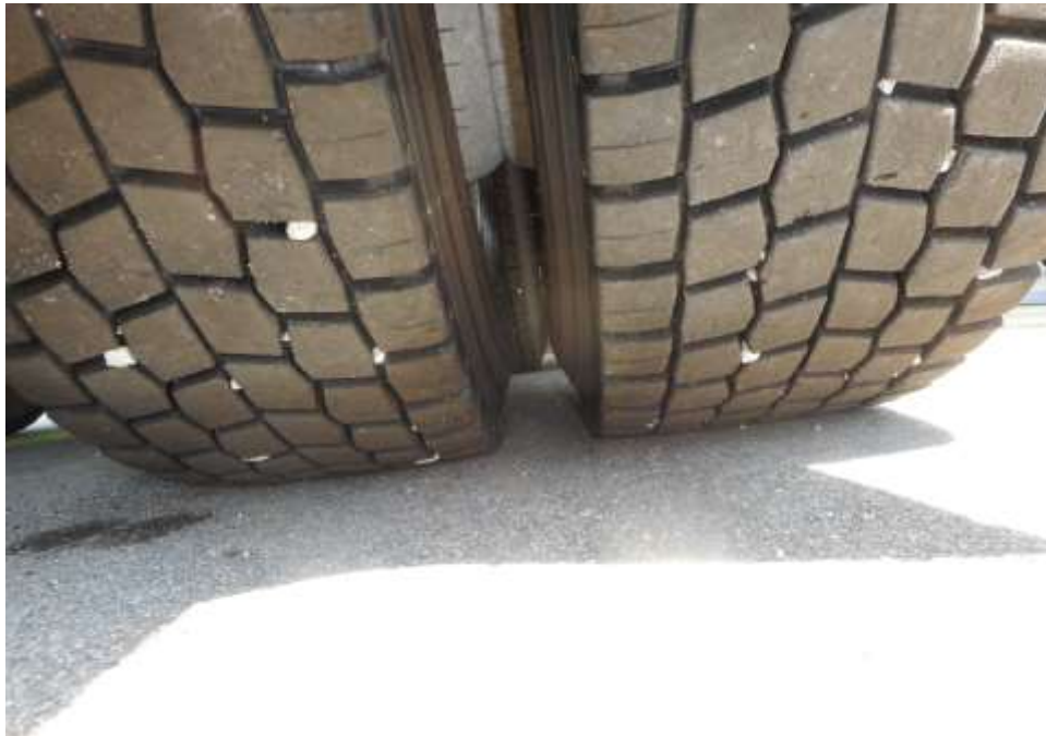
Photo 11 shows the condition of the rear right tyre of the Motor Trailer, which was observed to be in serviceable condition with remaining tread depth of approximately 12.3mm. The tyre, which was wrapped around standard steel wheel rim, was also observed to be sufficiently inflated for vehicular operation.
