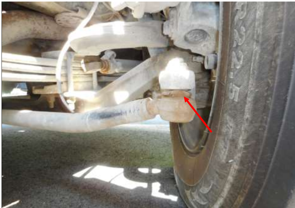
Photo 24 shows the various undercarriage components at the front right wheel of the Motor Trailer, in particular the steering tie rod end (arrowed). The various steering components were all found to be intact, suggesting that the steering system of the Motor Trailer was likely to be in serviceable condition at the material time of accident. There was also no sign of fluid stain(s) observed on the various undercarriage components.
