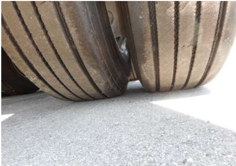
Photo 14 shows the condition of the right tyres of the trailer, which was observed to be in serviceable condition with remaining, tread depth of approximately 12.1mm. The tyre, which was wrapped around standard steel wheel rim, was also observed to be sufficiently inflated for vehicular operation.
