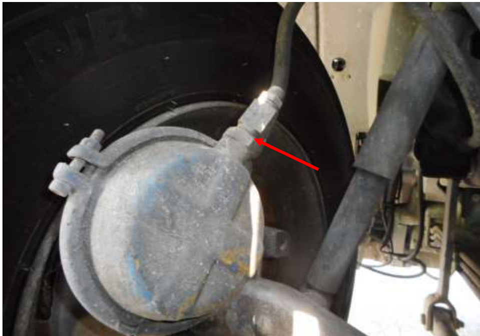
Photo 22 shows the brake pipe (arrowed) at the front left wheel of the Motor Trailer. I did not observe any leakage of brake fluid at the time of my inspection of the Motor Trailer. My static tests of the Motor Trailer's braking system, along with my visual examination of the various mechanical components in the braking system had indicated that there was no internal leakage of pressure/vacuum. Hence the braking system of the Motor Trailer was likely to be in serviceable condition at the material time of accident.
