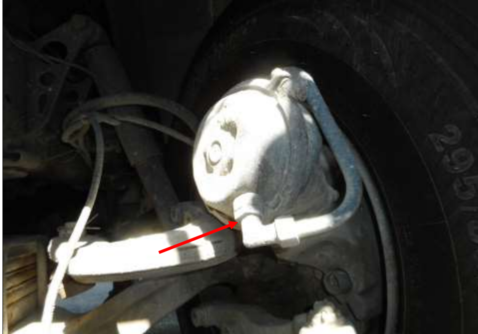
Photo 21 shows the brake pipe (arrowed) at the front right wheel of the Motor Trailer. I did not observe any leakage of brake fluid at the time of my inspection of the Motor Trailer. My static tests of the Motor Trailer's braking system, along with my visual examination of the various mechanical components in the braking system, had indicated that there was no internal leakage of pressure/vacuum. Hence the braking system of the Motor Trailer was likely to be in serviceable condition at the material time of accident.
