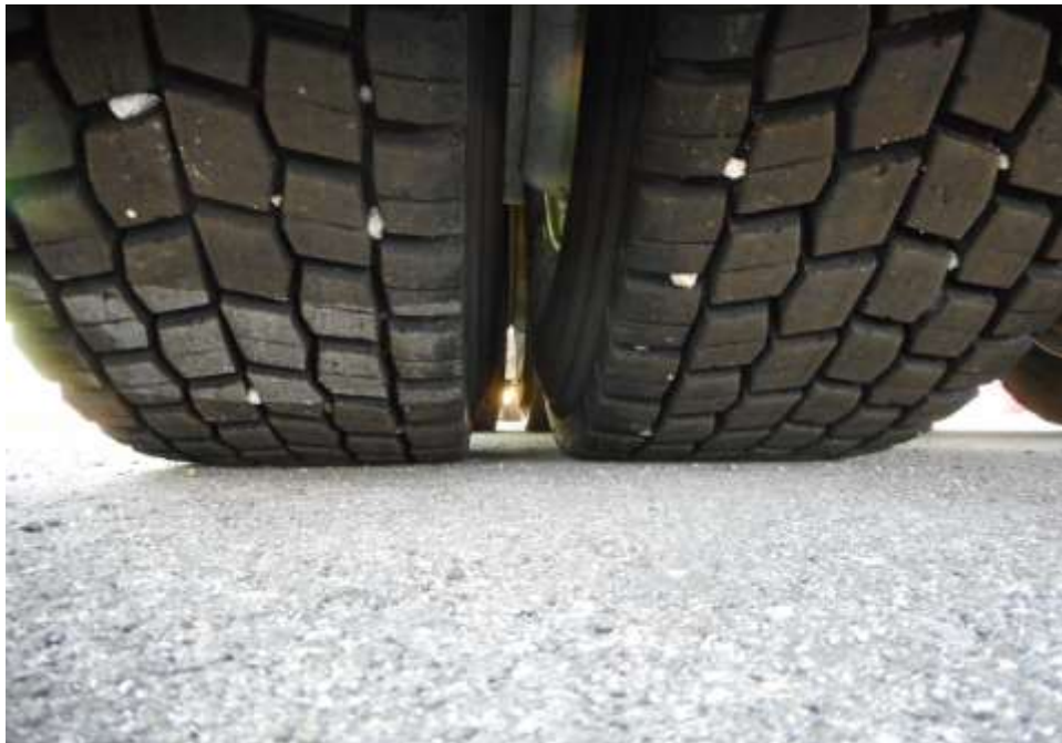
Photo 12 shows the condition of the rear left tyres of the Motor Trailer, which was observed to be in serviceable condition with remaining tread depth of approximately 10.2mm. The tyres, which were wrapped around standard steel wheel rim, were also observed to be sufficiently inflated for vehicular operation. There was also no damage found on all 6 steel wheel rims of the Motor Trailer.
