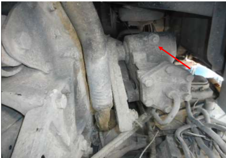
Photo 26 shows the steering box component (arrowed) at the undercarriage of the Motor Trailer was found to be intact without any visible damage. There was also no sign of fluid stain(s) observed on the various undercarriage components.
