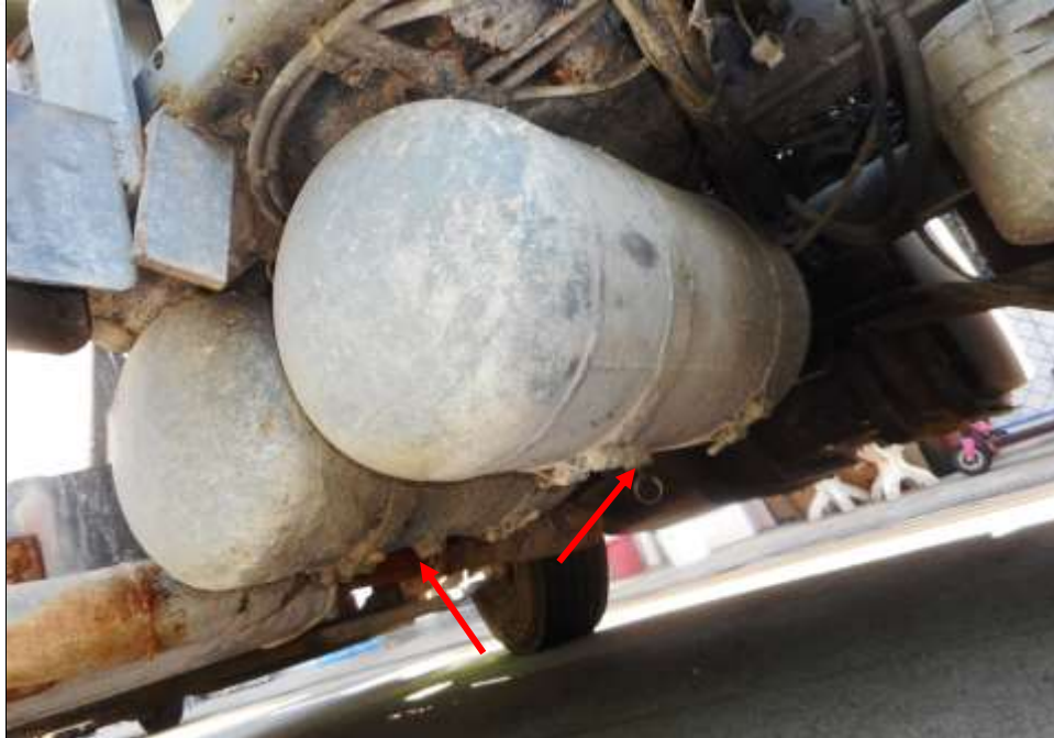
Photo 23 shows the air brake cylinders (arrowed) at the undercarriage of the Motor Trailer. I did not observe any leakage of air brake fluid at the time of my inspection of the Motor Trailer. My static tests of the Motor Trailer's braking system, along with my visual examination of the various mechanical components in the braking system had indicated that there was no internal leakage of pressure/vacuum. Hence the braking system of the Motor Trailer was likely to be in serviceable condition at the material time of accident.
