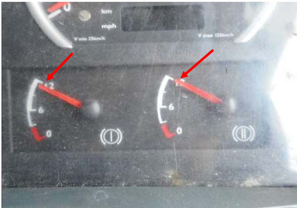
Photo 17 shows the air in the air brake cylinders of the Motor Trailer at the time of my inspection. The air in the cylinder was observed to be of sufficient level & serviceable at the time of the accident.
