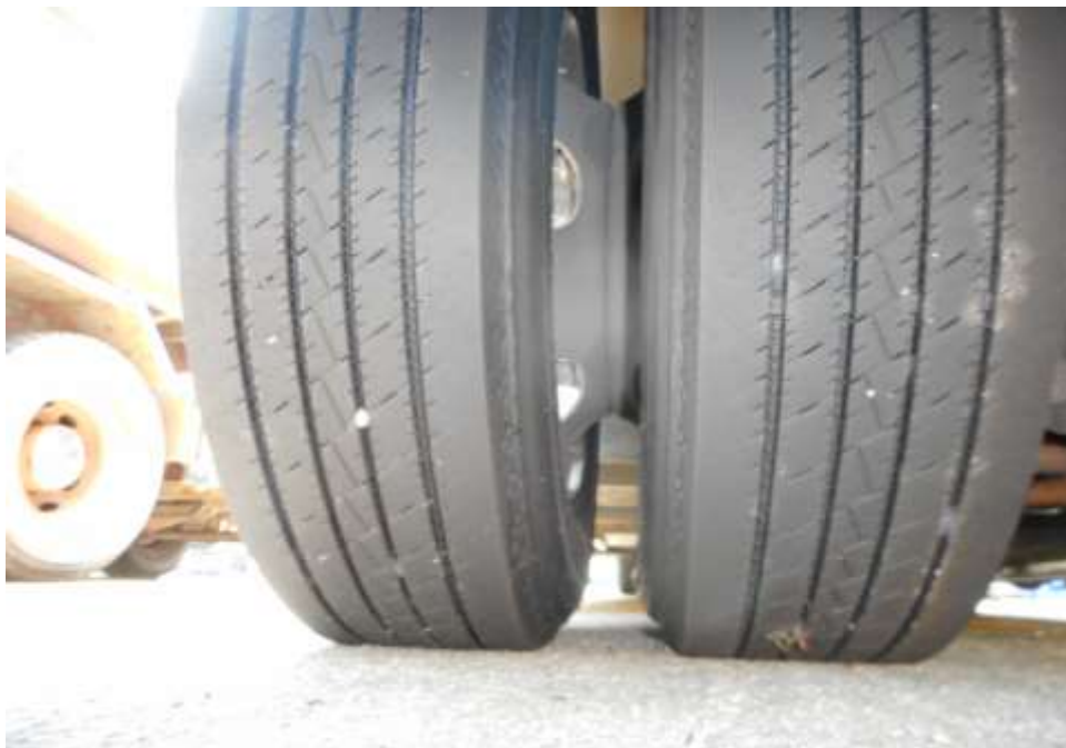
Photo 11 shows the condition of the rear left tyres of the Motor Bus, which was observed to be in serviceable condition with remaining tread depth of approximately 4.9mm. The tyres, which were wrapped around standard steel wheel rim, were also observed to be sufficiently inflated for vehicular operation. There was also no damage found on all 6 steel wheel rims of the Motor Bus.
