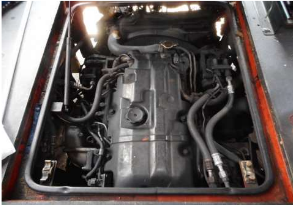
Photo 13 shows a general view of the Motor Bus's engine compartment, which was accessed by lifting the front cabin of the Motor Bus. The various parts and components inside the engine compartment were unaffected by the accident. There was also no sign(s) or indication(s) of fresh fluid leakage and/or fluid stain within the engine compartment
