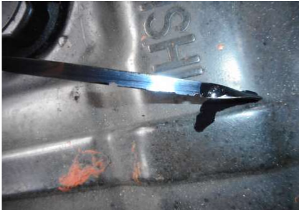
Photo 16 shows the engine oil level display of the Motor Bus at the time of my inspection. The engine oil was observed to be of sufficient level.
