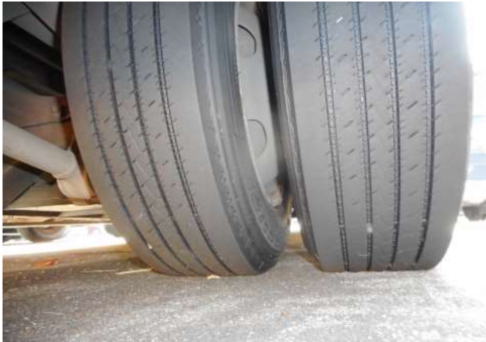
Photo 10 shows the condition of the rear right tyre of the Motor Bus, which was observed to be in serviceable condition with remaining tread depth of approximately 5.6mm. The tyre, which was wrapped around standard steel wheel rim, was also observed to be sufficiently inflated for vehicular operation.
