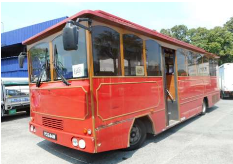
Photo 25 shows the front left of the steering wheel of the Motor Bus turned to its full right. During my steering system test, I did not experience any abnormal free play and/or resistance when I had turned the steering wheel towards full left and full right. This would suggest that the steering system of the Motor Bus was likely to be in serviceable condition at the material time of accident.
