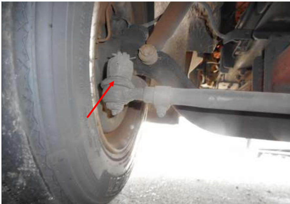
Photo 23 shows the various undercarriage components at the front left wheel of the Motor Bus, in particular the steering tie rod end (arrowed). The various undercarriage components of the Motor Bus were all found to be intact without any visible damage. There was also no sign of fluid stain(s) observed on the various undercarriage components.
