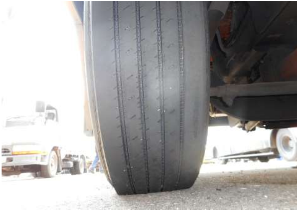
Photo 12 shows the condition of the front left tyres of the Motor Bus, which were observed to be in serviceable condition with remaining tread depth of approximately 5.4mm. There was also no tear, cut or burst mark(s) on the outer and the inner sidewalls as well as across the tread of the 6 tyres that were fitted on the Motor Bus.
