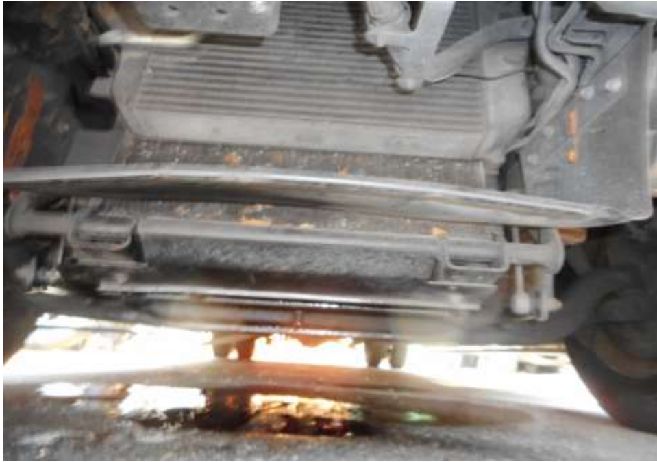
Photo 17 shows the undercarriage of the Motor Bus, at the area where the engine housing located. I did not find any sign(s) or indication(s) of fluid leak and/or fluid stain(s) on the underside of the Motor Bus.
