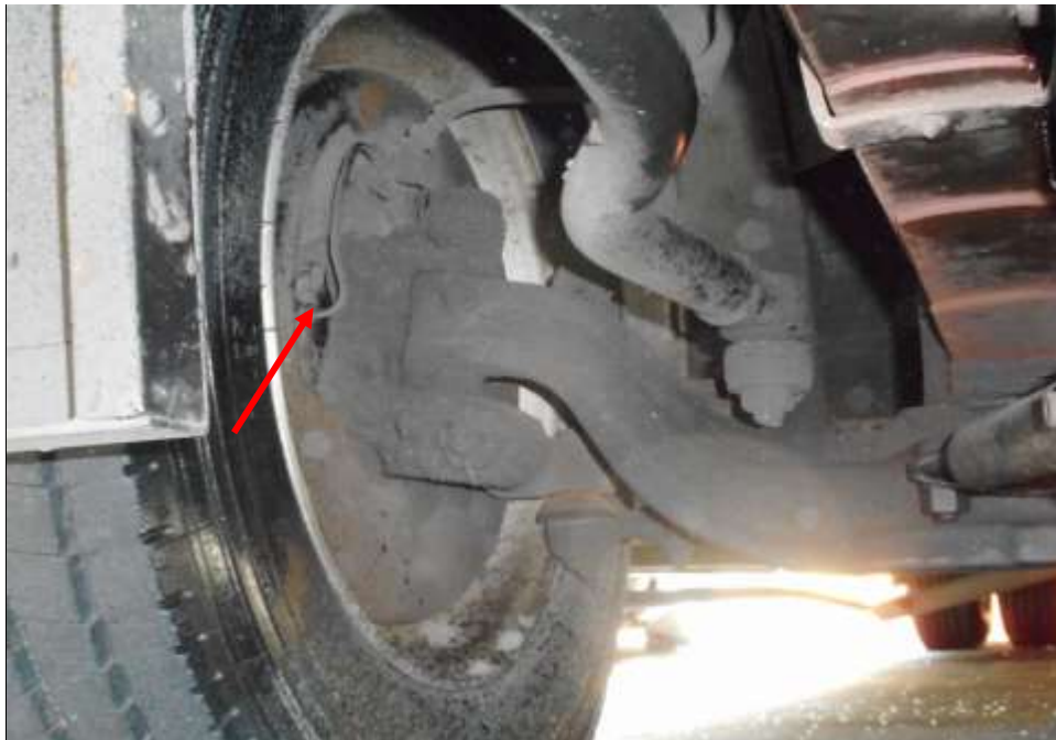
Photo 21 shows the brake pipe (arrowed) at the front right wheel of the Motor Bus. I did not observe any leakage of brake fluid at the time of my inspection of the Motor Bus. My static tests of the Motor Bus's braking system, along with my visual examination of the various mechanical components in the braking system had indicated that there was no internal leakage of pressure/vacuum. Hence the braking system of the Motor Bus was likely to be in serviceable condition at the material time of accident.
