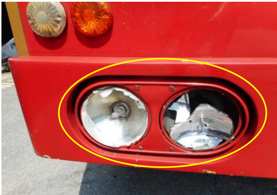
Photo 5 shows the close up view of the Motor Bus front body at the time of my inspection. The Motor Bus was observed to have sustained damage at its front right head lamp (circled), as a result of the accident.
