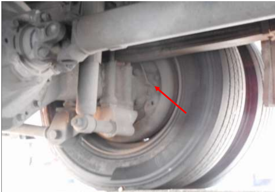
Photo 19 shows the brake pipe (arrowed) at the rear left wheel of the Motor Bus. I did not observe any leakage of brake fluid at the time of my inspection of the Motor Bus. My static tests of the Motor Bus's braking system, along with my visual examination of the various mechanical components in the braking system, had indicated that there was no internal leakage of pressure/vacuum. Hence the braking system of the Motor Bus was likely to be in serviceable condition at the material time of accident.
