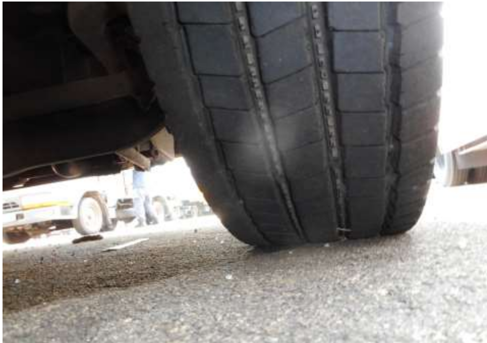
Photo 9 shows the condition of the front right tyre of the Motor Bus, which was observed to be in serviceable condition with remaining tread depth of approximately 10.3 mm. The tyre, which was wrapped around standard steel wheel rim, was also observed to be sufficiently inflated for vehicular operation. There was no tear, cut or burst mark(s) on the outer and the inner sidewalls as well as across the tread of the 6 tyres that were fitted on the Motor Bus.
