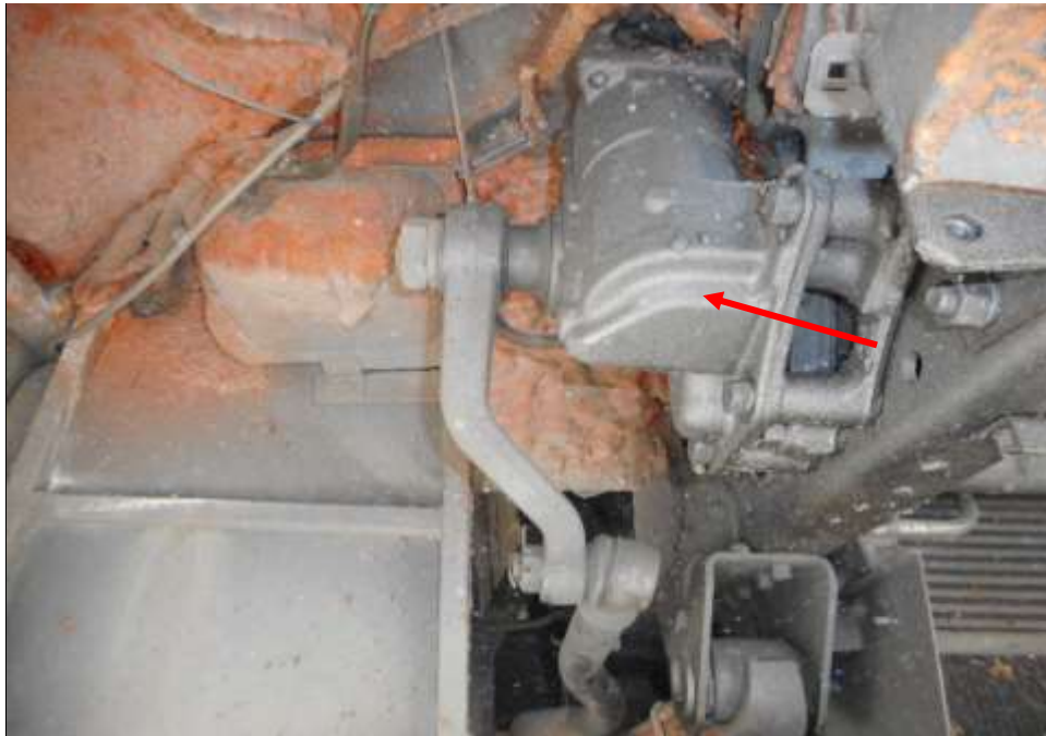
Photo 24 shows the steering box component (arrowed) at the undercarriage of the Motor Bus was found to be intact without any visible damage. There was also no sign of fluid stain(s) observed on the various undercarriage components.
