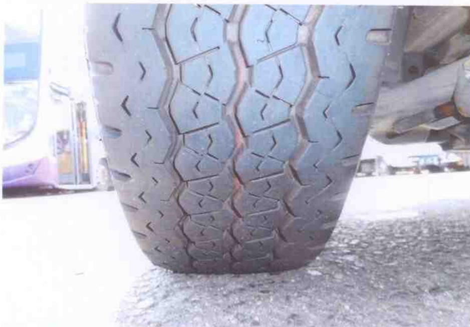
Photo 11 shows the condition of the front left tyre of the Motor Lorry, which observed to be in serviceable condition with remaining tread depth of approximately 5mm. The tyre, which was wrapped around standard alloy wheel rim, was also observed to be sufficiently inflated for vehicular operation.
