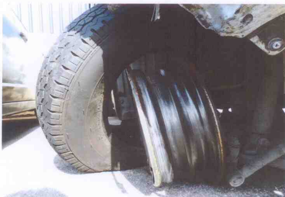
Photo 8 shows the condition of the front right tyre and rims of the Motor Lorry, which was observed to have been dislodged as a result of the accident. The remaining tread depth of approximately 7.3mm. The tyre was wrapped around standard alloy wheel rim.
