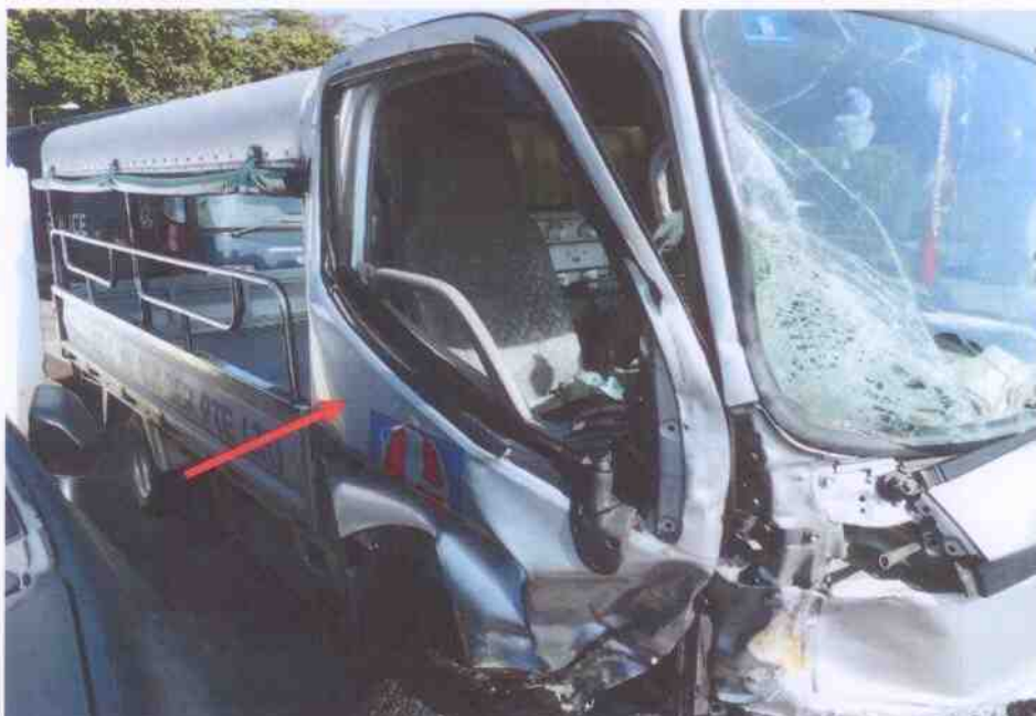
Photo 5 shows the close up view of the right portion of the Motor Lorry at the time of our inspection. Its right door was damaged as a result of the accident.
