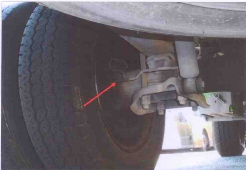
Photo 18 shows the various undercarriage components at the rear left wheel of the Motor Lorry, in particular the brake hose and drum brake (arrowed). The various undercarriage components of the Motor Lorry were all found to be intact without any visible damage. There was also no sign of fluid stain(s) observed on the various undercarriage components.
