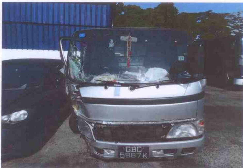
Photo 2 shows a general view of the front portion of the Motor Lorry. Its front windscreen, front bumper, front right head lamp and its right doors as a result of the accident.
