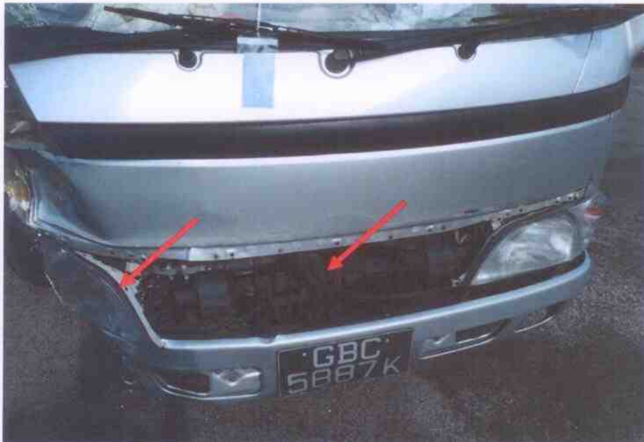
Photo 4 shows the close up view of the front portion of the Motor Lorry at the time of our inspection. Its front bumper and left head lamp (arrowed) was damaged as a result of the accident.
