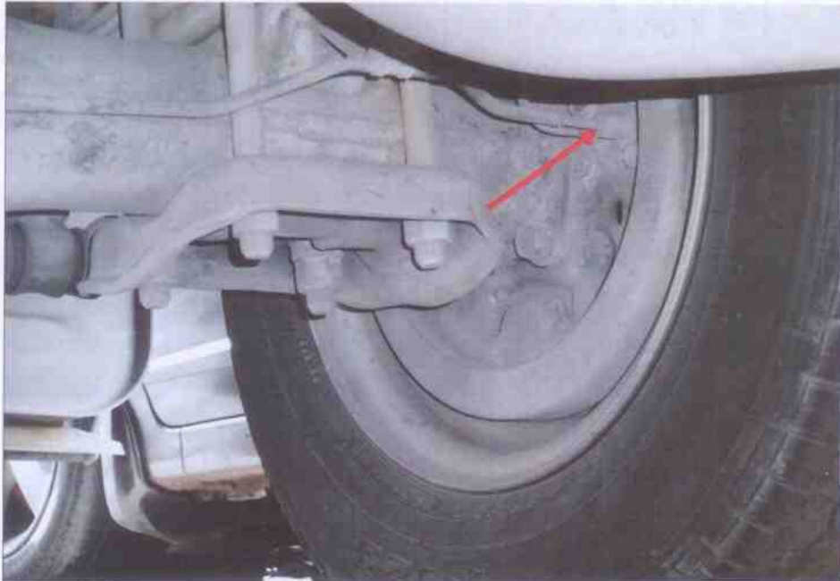
Photo 17 shows the various undercarriage components at the rear right wheel of the Motor Lorry, in particular the brake hose and drum brake (arrowed). The various undercarriage components of the Motor Lorry were all found to be intact without any visible damage. There was also no sign of fluid stain(s) observed on the various undercarriage components.
