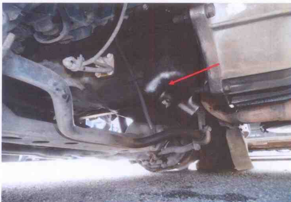
Photo 13 shows the undercarriage of the engine of the Motor Lorry at the time of our inspection. There was also no sign(s) or indication(s) of fresh fluid leakage and/or fluid stain within the engine area.
