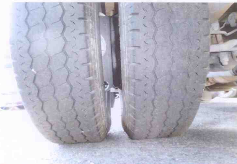
Photo 10 shows the condition of the front left tyre of the Motor Lorry, which observed to be in serviceable condition with remaining tread depth of approximately 2.4mm. The tyre, which was wrapped around standard alloy wheel rim, was also observed to be sufficiently inflated for vehicular operation.
