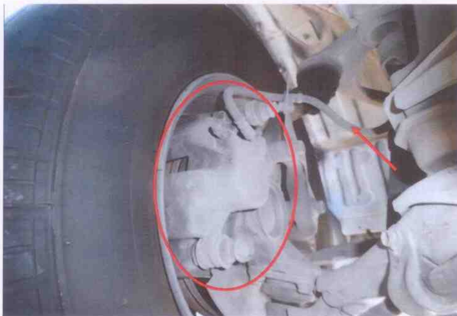
Photo 16 shows the various undercarriage components at the front left wheel of the Motor Lorry, in particular the brake hose and caliper (arrowed). The various undercarriage components of the Motor Lorry were all found to be intact without any visible damage. There was also no sign of fluid stain(s) observed on the various undercarriage components.
