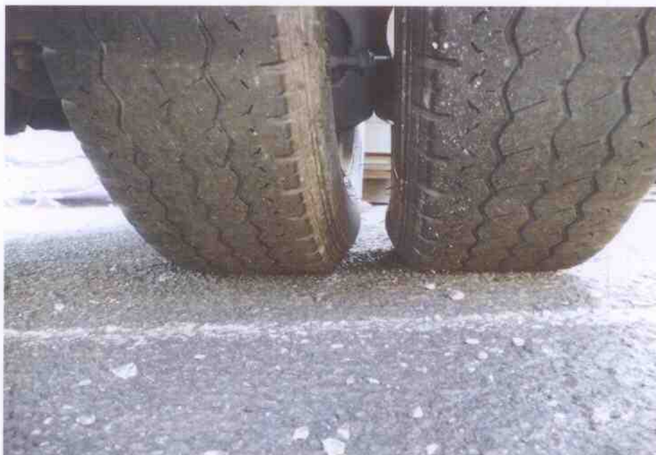
Photo 9 shows the condition of the rear right tyre of the Motor Lorry, which observed to be in serviceable condition with remaining tread depth of approximately 2.3mm. The tyre, which was wrapped around standard alloy wheel rim, was also observed to be sufficiently inflated for vehicular operation.
