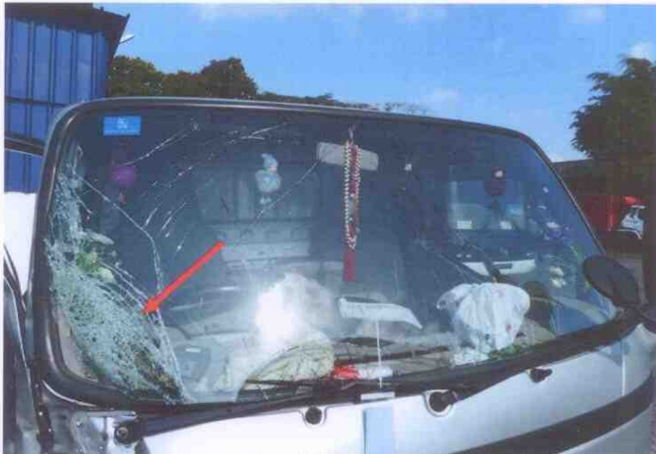
Photo 3 shows the close up view of the front portion of the Motor Lorry at the time of our inspection. Its front windscreen (arrowed) was damaged as a result of the accident.
