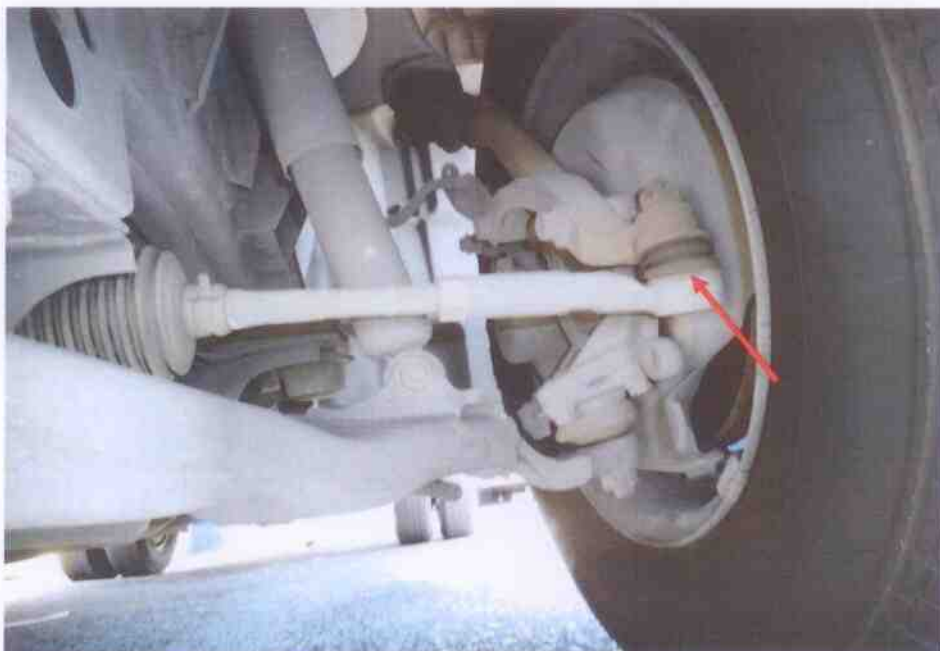
Photo 15 shows the various undercarriage components at the front left wheel of the Motor Lorry, in particular the steering tie rod end and ball joints (arrowed). The various undercarriage components of the Motor Lorry were all found to be intact without any visible damage. There was also no sign of fluid stain(s) observed on the various undercarriage components.
