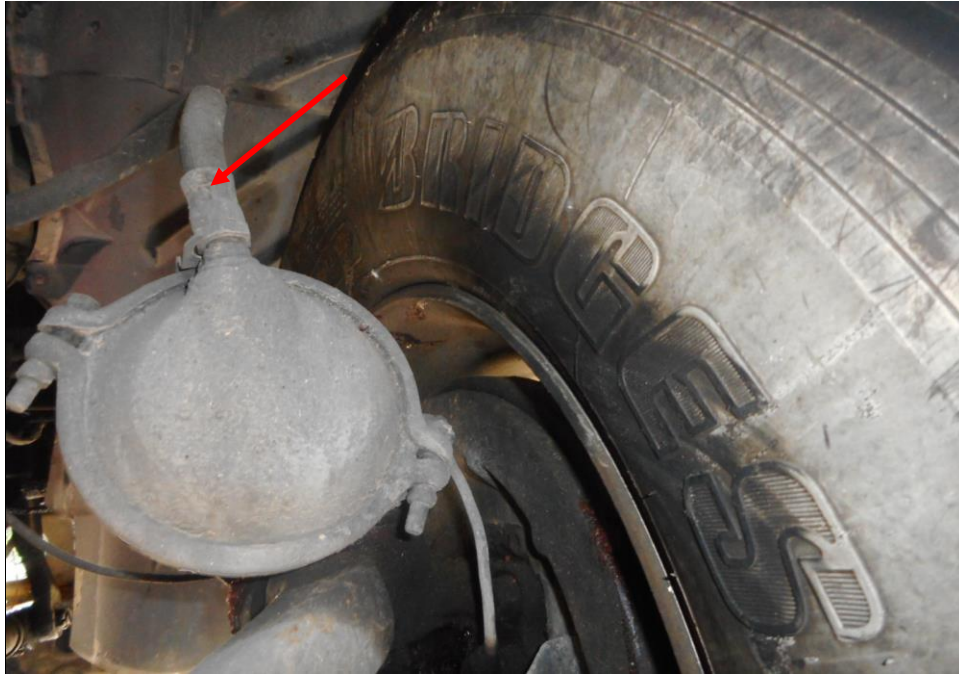
Photo 24 shows the brake pipe (arrowed) at the front right wheel of the Motor Trailer. I did not observe any leakage of brake fluid at the time of my inspection of the Motor Trailer. My visual examination of the various mechanical components in the braking system, had indicated that there was no internal leakage of pressure/vacuum and were generally intact to suggest that its braking system was in serviceable condition at the material time of accident.
