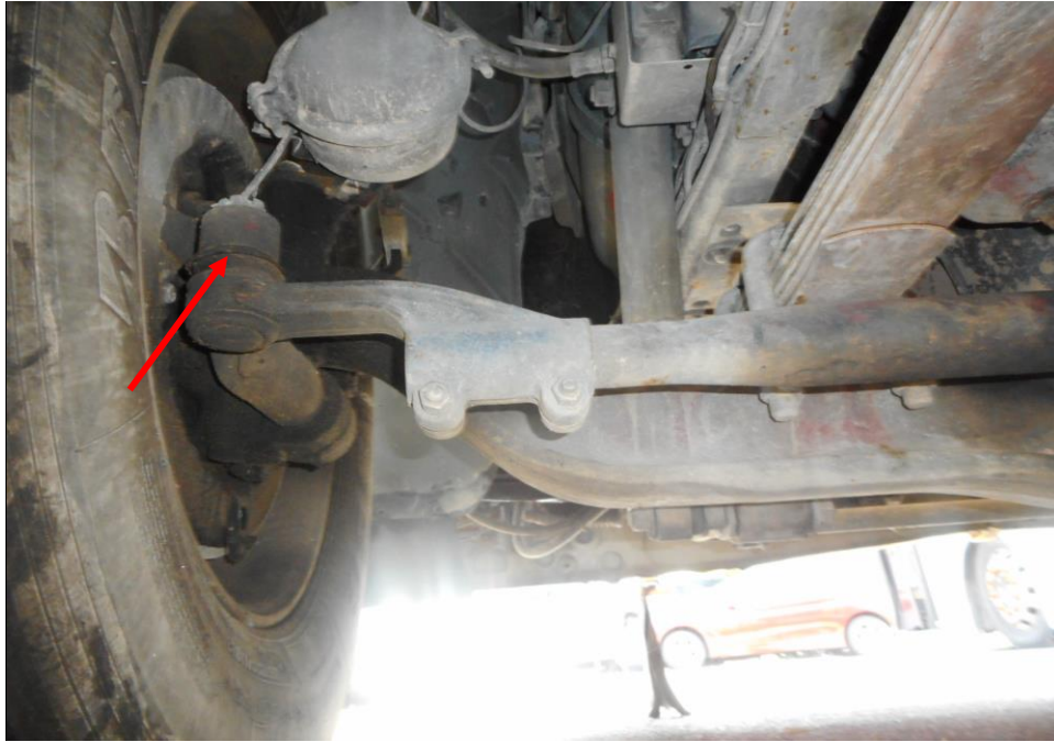
Photo 21 shows the various undercarriage components at the front left wheel of the Motor Trailer, in particular the steering tie rod end (arrowed). The various undercarriage components of the Motor Trailer were all found to be intact without any visible damage. There was also no sign of fluid stain(s) observed on the various undercarriage components to indicate that the Motor Trailer's steering system was in serviceable condition.
