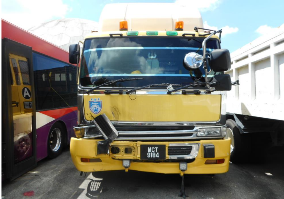
Photo 1 shows a general view of the front body of the Motor Trailer at the time of my inspection. The Motor Trailer was observed to sustain damage at its front portion. Its front body panel & front right headlamp was damaged.
