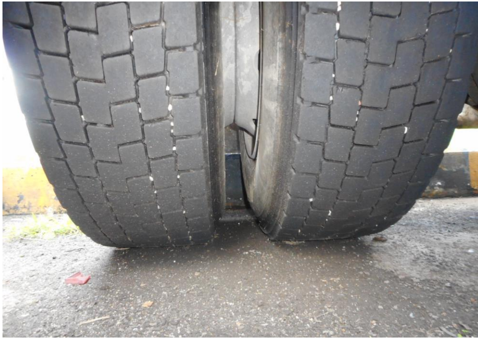
Photo 11 shows the condition of the rear right tyre of the Motor Trailer, which was observed to be in serviceable condition with remaining tread depth of approximately 9mm. The tyre, which was wrapped around standard steel wheel rim, was also observed to be sufficiently inflated for vehicular operation.
