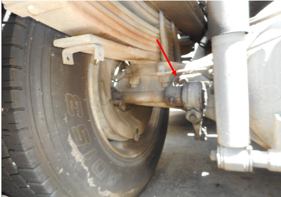
Photo 22 shows the brake pipe (arrowed) at the rear right wheel of the Motor Trailer. I did not observe any leakage of brake fluid at the time of my inspection of the Motor Trailer. My visual examination of the various mechanical components in the braking system, had indicated that there was no internal leakage of pressure/vacuum and were generally intact to suggest that its braking system was in serviceable condition at the material time of accident.
