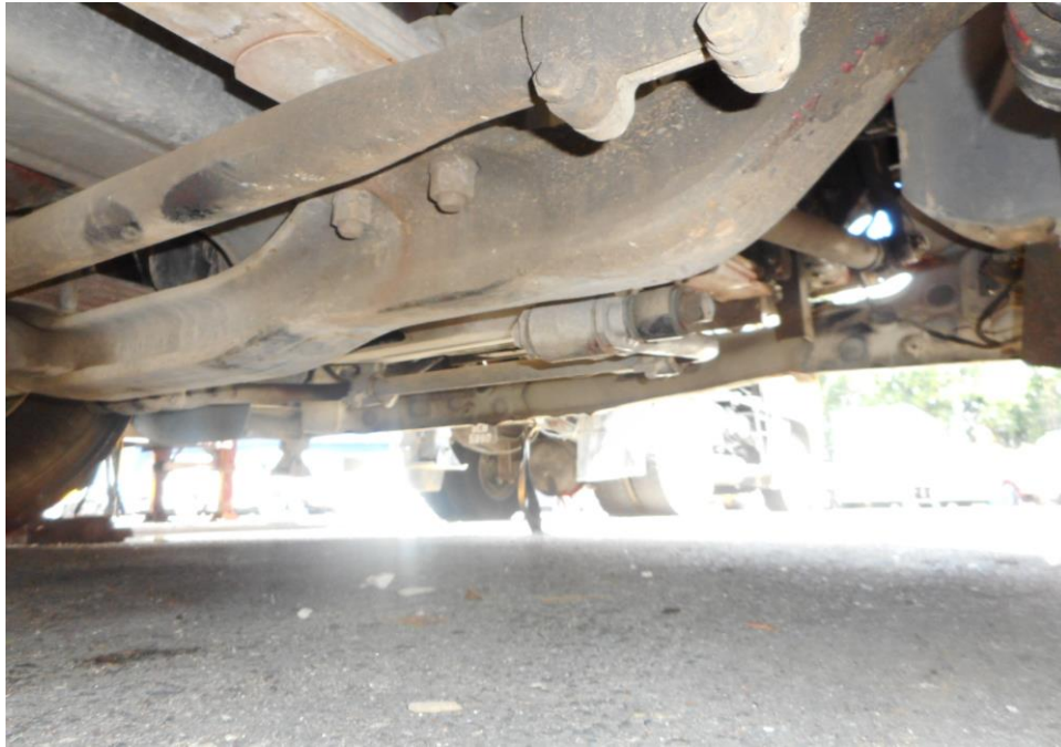
Photo 16 shows the undercarriage of the Motor Trailer, at the area where the engine housing located. I did not find any sign(s) or indication(s) of fluid leak, or fluid stain(s) was observed on the underside of the Motor Trailer.
