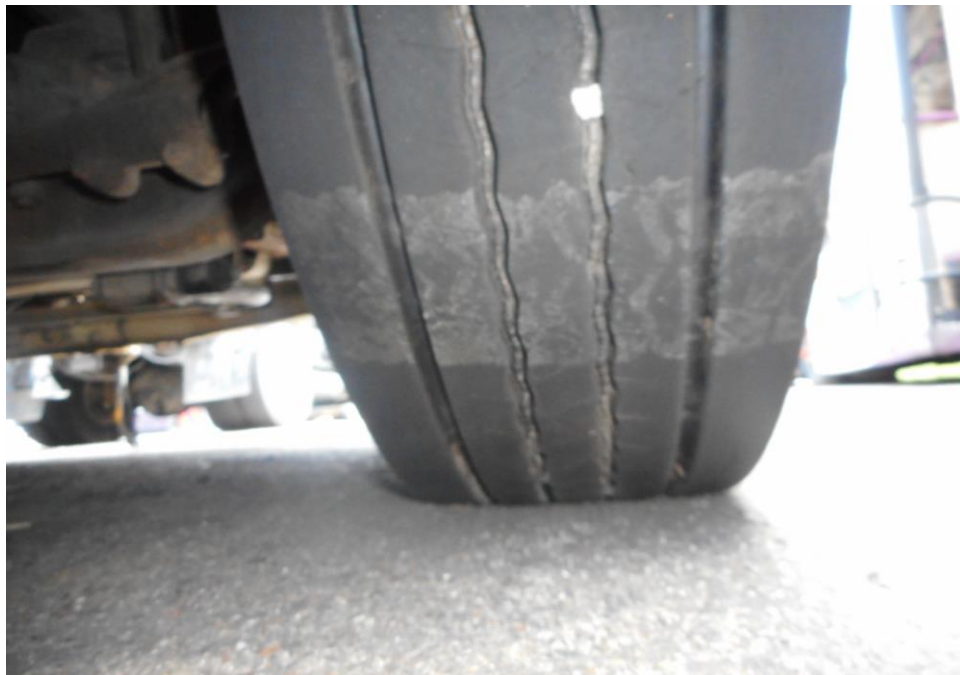
Photo 10 shows the condition of the front right tyre of the Motor Trailer, which was observed to be in serviceable condition with remaining tread depth of approximately 11mm. The tyre, which was wrapped around standard steel wheel rim, was also observed to be sufficiently inflated for vehicular operation. There was no tear, cut or burst mark(s) on the outer and the inner sidewalls as well as across the tread of the 22 tyres that were fitted on the Motor Trailer.
