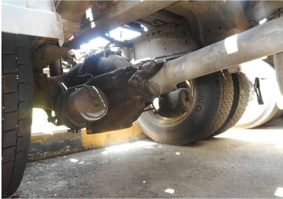
Photo 18 shows the undercarriage of the Motor Trailer, at the area where the rear differential housing located. I did not find any sign(s) or indication(s) of fluid leak, or fluid stain(s) was observed on the underside of the Motor Trailer.
