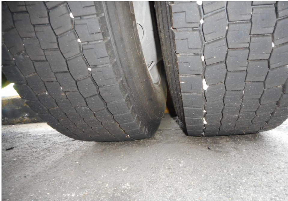
Photo 12 shows the condition of the rear left tyres of the Motor Trailer, which was observed to be in serviceable condition with remaining tread depth of approximately 10.9mm. The tyres, which were wrapped around standard steel wheel rim, were also observed to be sufficiently inflated for vehicular operation. There was also no damage found on all 6 steel wheel rims of the Motor Trailer.
