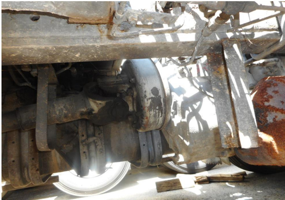
Photo 17 shows the undercarriage of the Motor Trailer, at the area where the transmission housing located. I did not find any sign(s) or indication(s) of fluid leak, or fluid stain(s) was observed on the underside of the Motor Trailer.
