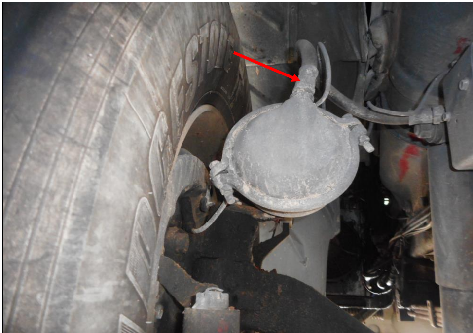
Photo 25 shows the brake pipe (arrowed) at the front left wheel of the Motor Trailer. I did not observe any leakage of brake fluid at the time of my inspection of the Motor Trailer. My visual examination of the various mechanical components in the braking system, had indicated that there was no internal leakage of pressure/vacuum and were generally intact to suggest that its braking system was in serviceable condition at the material time of accident.
