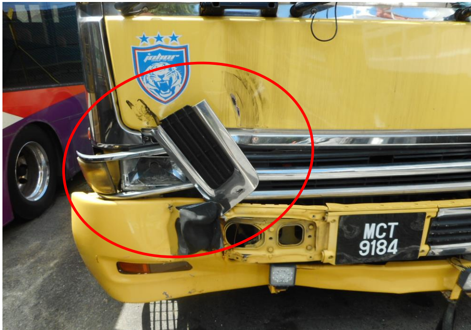
Photo 2 shows a close up view of the front body of the Motor Trailer at the time of my inspection. The Motor Trailer was observed to sustain damage at its front portion. Its front body panel & front right headlamp (circled) was damaged.
