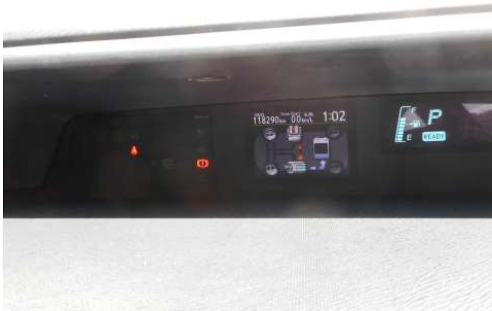
Photo 26 shows no warning lights illuminated on the instrument panel of the Motor Car after the engine was cranked. This would suggest that there was no abnormality to the various electronic operating systems of the Motor Car, like the ABS, EPS SRS and TC etc.
