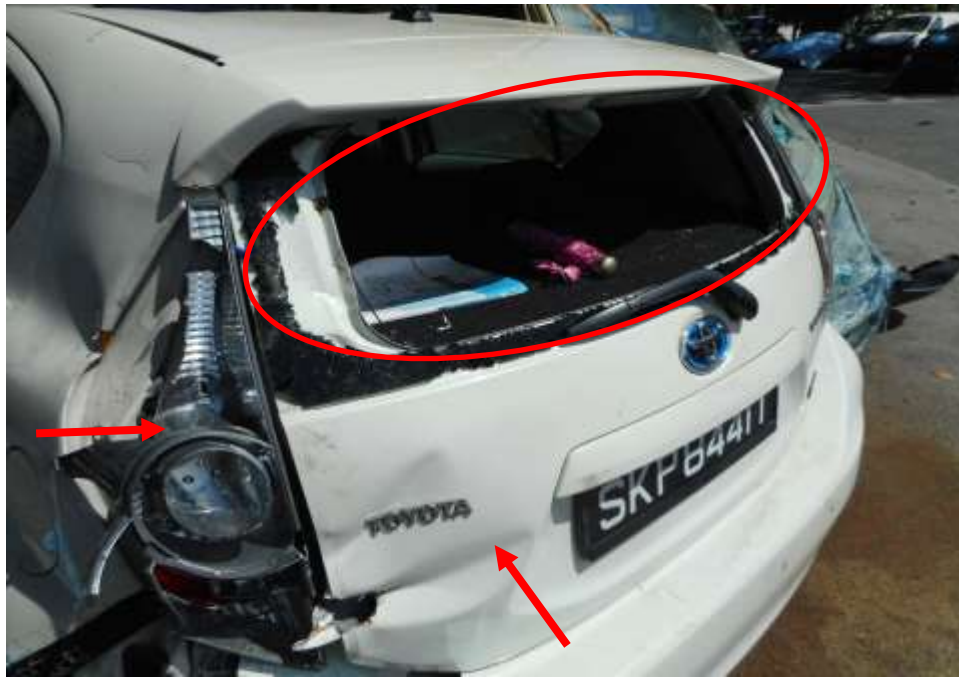
Photo 4 shows a close up view of the Motor Car's rear portion at the time of my inspection. The rear and rear left portion of the Motor Car was observed to sustain major damage. Its rear windscreen (circled), rear bonnet, and its rear left headlamp (arrowed) were damaged as a result of the accident.
