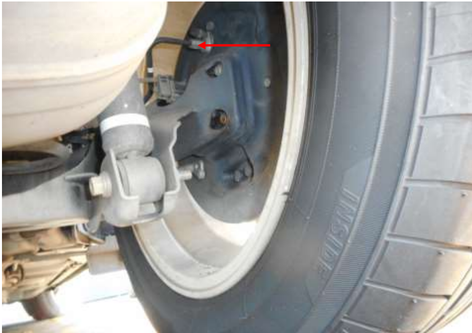
Photo 22 shows the brake hose/pipe (arrowed) at the rear right wheel of the Motor Car. No leakage of brake fluid was observed. Visual examination of the various components of the braking system like the drum brake, brake booster, brake pedal etc had revealed all to be intact and without visible damage.
