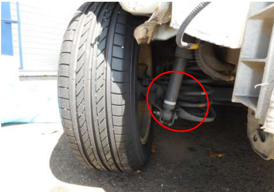
Photo 23 shows the general view of the Motor Car's rear axle at the time of my inspection. The rear axle (circled) of the Motor Car was observed to sustain damaged and shifted out of position as a result of the accident.
