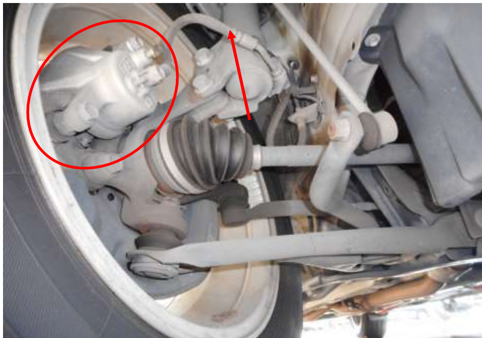
Photo 19 shows the brake hose/pipe (arrowed) at the front right wheel of the Motor Car. I did not observe any leakage of brake fluid at the time of my inspection of the Motor Car. Static tests of the Motor Car's braking system had indicated that there was no internal leakage of pressure/vacuum. The undercarriage components of the Motor Car were also all found to be intact and without any visible damage.
