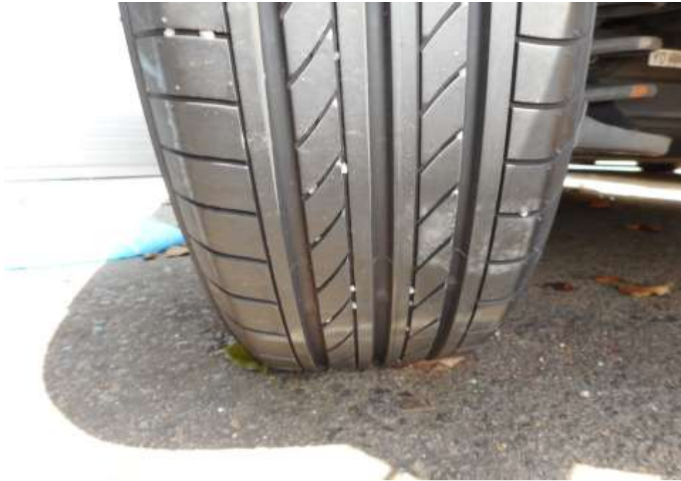
Photo 10 shows the condition of the rear left tyre of the Motor Car, which was observed to be in serviceable condition with remaining tread depth of approximately 5.9mm. The tyre, which was wrapped around alloy wheel rim, was also observed to be sufficiently inflated for vehicular operation. The 4 tyres of the Motor Car were wrapped around standard alloy wheel rims.
