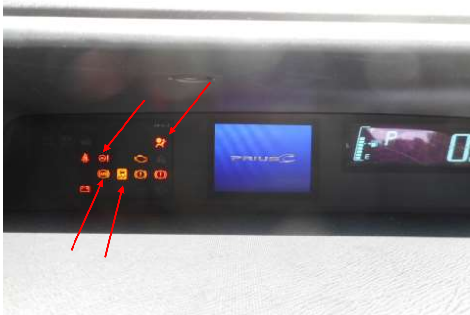
Photo 25 shows the warning light for Anti-Lock Brake System (ABS), Electric Power Steering System (EPS) Supplemental Restraint System (SRS) and Traction Control (TC) appearing on the instrument panel of the Motor Car during the self-test of its various electronic operating systems when its engine was cranked.
