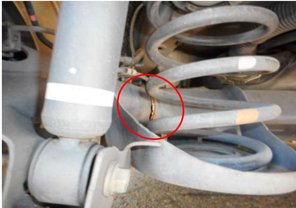
Photo 24 shows the close up view of the Motor Car's rear axle at the time of my inspection. The rear axle (circled) of the Motor Car was observed to sustain damaged and shifted out of position as a result of the accident.
