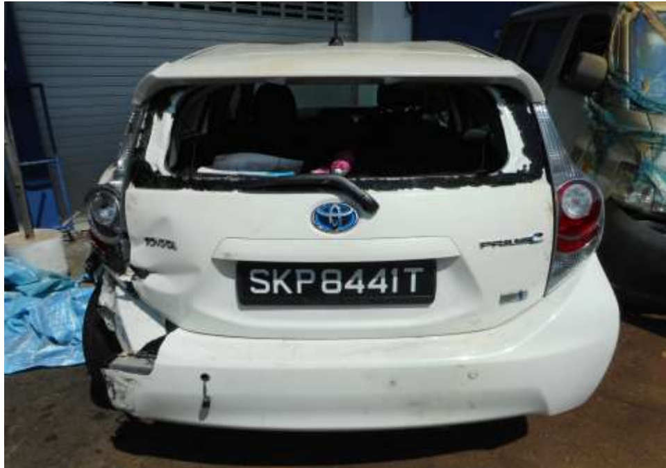
Photo 2 shows a general view of the Motor Car's rear portion at the time of my inspection. The rear and rear left portion of the Motor Car was observed to sustain major damage. Its rear windscreen, rear bonnet, rear bumper, rear left body panel and its rear left headlamp was damaged at the time of my inspection.
