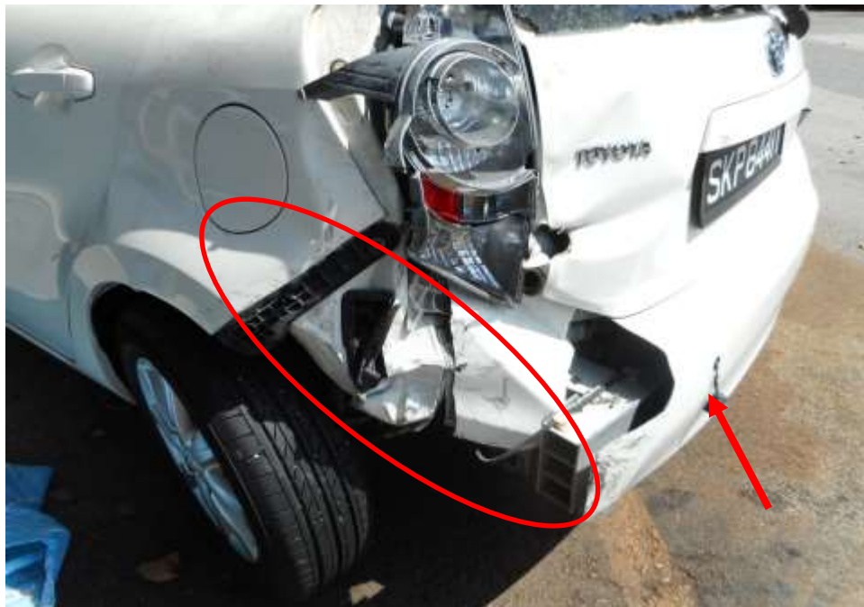
Photo 5 shows a close up view of the Motor Car's left portion at the time of my inspection. The rear portion of the Motor Car was observed to sustain moderate damage at its rear left portion. Its rear bumper (arrowed) and rear left body panel (circled) was damaged as a result of the accident.
