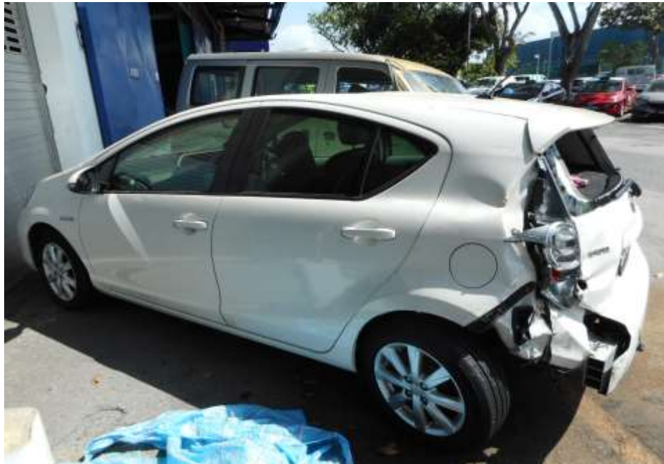
Photo 3 shows a general view of the Motor Car's left portion at the time of my inspection. The rear and rear left portion of the Motor Car was observed to sustain major damage. Its rear windscreen, rear bonnet, rear bumper, rear left body panel and its rear left headlamp was damaged at the time of my inspection.
