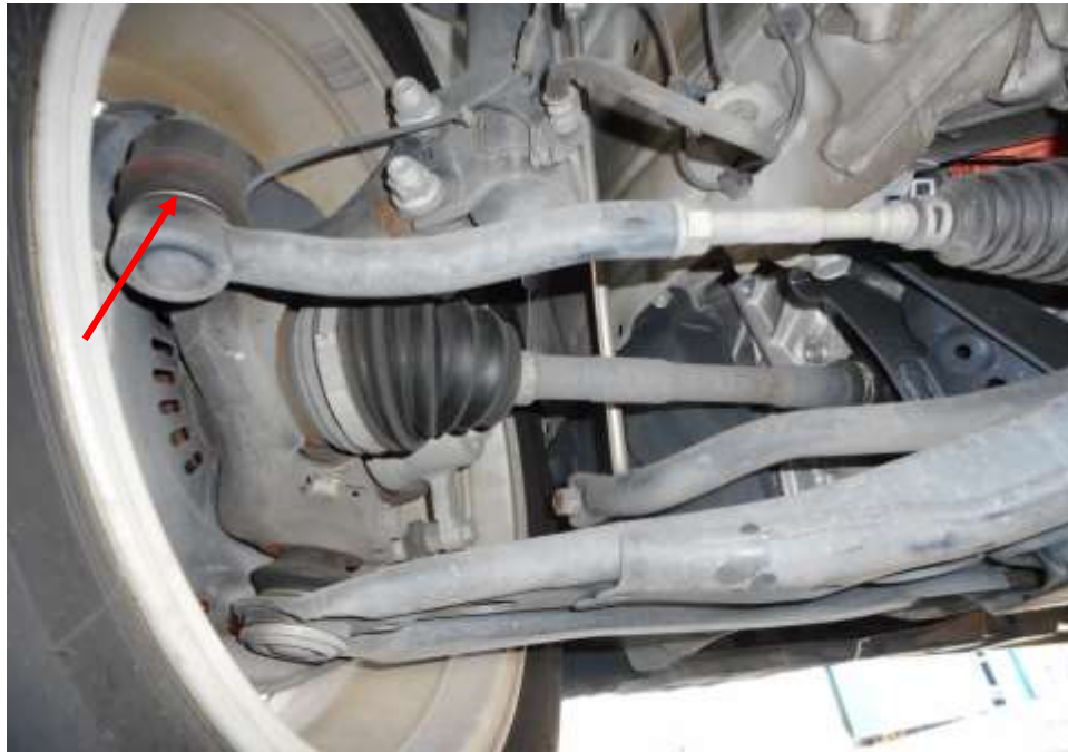
Photo 18 shows the various undercarriage components at the front left wheel of the Motor Car, which had included the steering tie rod (red arrow). The various undercarriage components of the Motor Car were all found to be intact without any visible damage.
