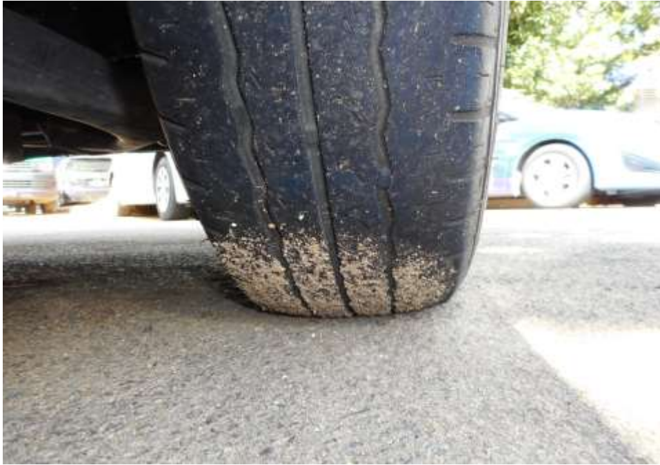
Photo 8 shows the condition of the front right tyre of the Motor Van, which was observed to be in serviceable condition with remaining tread depth of approximately 3.9mm. The tyre, which was wrapped around standard steel wheel rim, was also observed to be sufficiently inflated for vehicular operation. There was no tear, cut or burst mark(s) on the outer and the inner sidewalls as well as across the tread of the 4 tyres that were fitted on the Motor Van.
