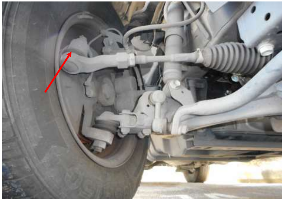
Photo 17 shows the various undercarriage components at the front right wheel of the Motor Van, in particular the steering tie rod end (arrowed). The various steering components were all found to be intact, suggesting that the steering system of the Motor Van was likely to be in serviceable condition at the material time of accident. There was also no sign of fluid stain(s) observed on the various undercarriage components.
