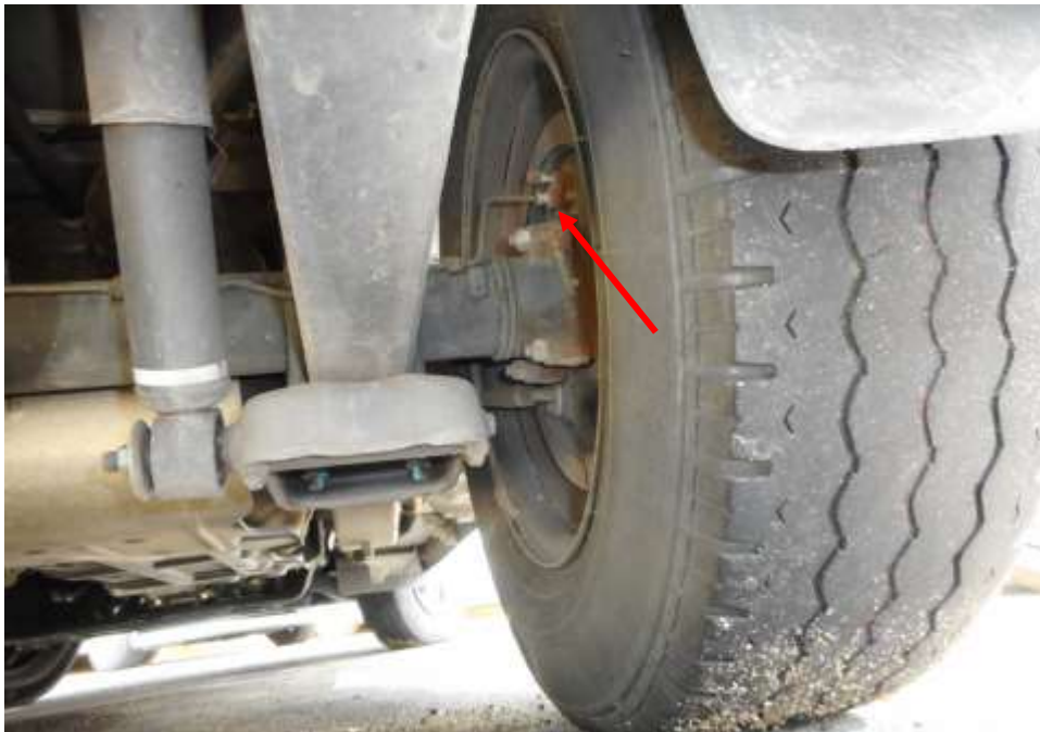
Photo 19 shows the brake pipe (arrowed) at the rear right wheel of the Motor Van. I did not observe any leakage of brake fluid at the time of my inspection of the Motor Van. My static tests of the Motor Van's braking system, along with my visual examination of the various mechanical components in the braking system, had indicated that there was no internal leakage of pressure/vacuum. Hence the braking system of the Motor Van was likely to be in serviceable condition at the material time of accident.
