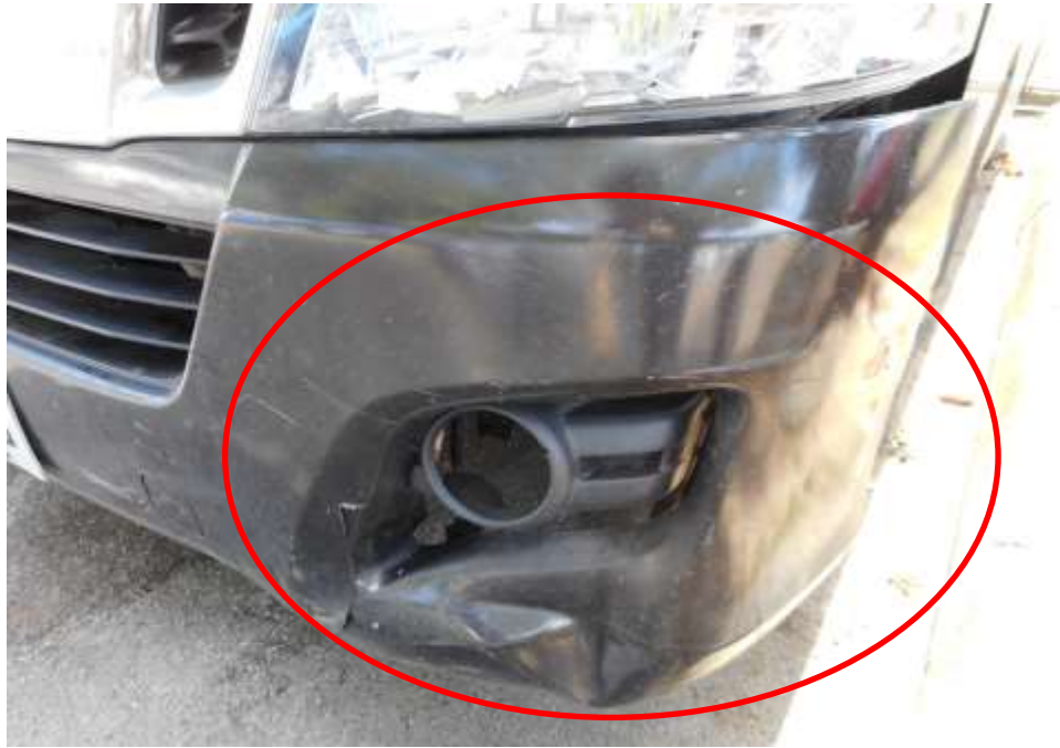
Photo 4 shows a close up view of the Motor Van's frontal portion at the time of my inspection. It appeared to have sustained damage at its frontal portion. Its front bumper (circled) was damaged at the time of my inspection as a result of the accident.
