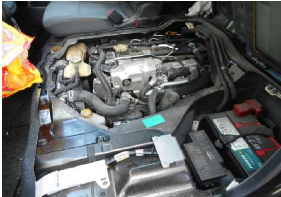
Photo 12 shows a general view of the Motor Van's engine compartment, which was accessed by lifting the front cabin of the Motor Van. The various parts and components inside the engine compartment were unaffected by the accident. There was also no sign(s) or indication(s) of fresh fluid leakage and/or fluid stain within the engine compartment
