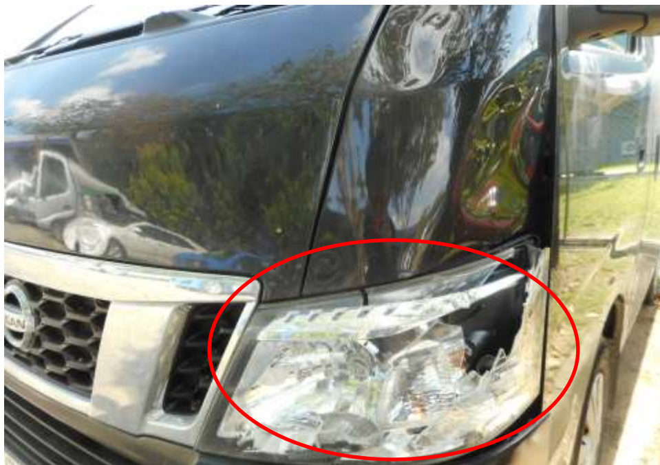
Photo 3 shows a close up view of the Motor Van's frontal portion at the time of my inspection. It appeared to have sustained damage at its frontal portion. Its front left head lamp (circled) was damage at the time of my inspection as a result of the accident.
