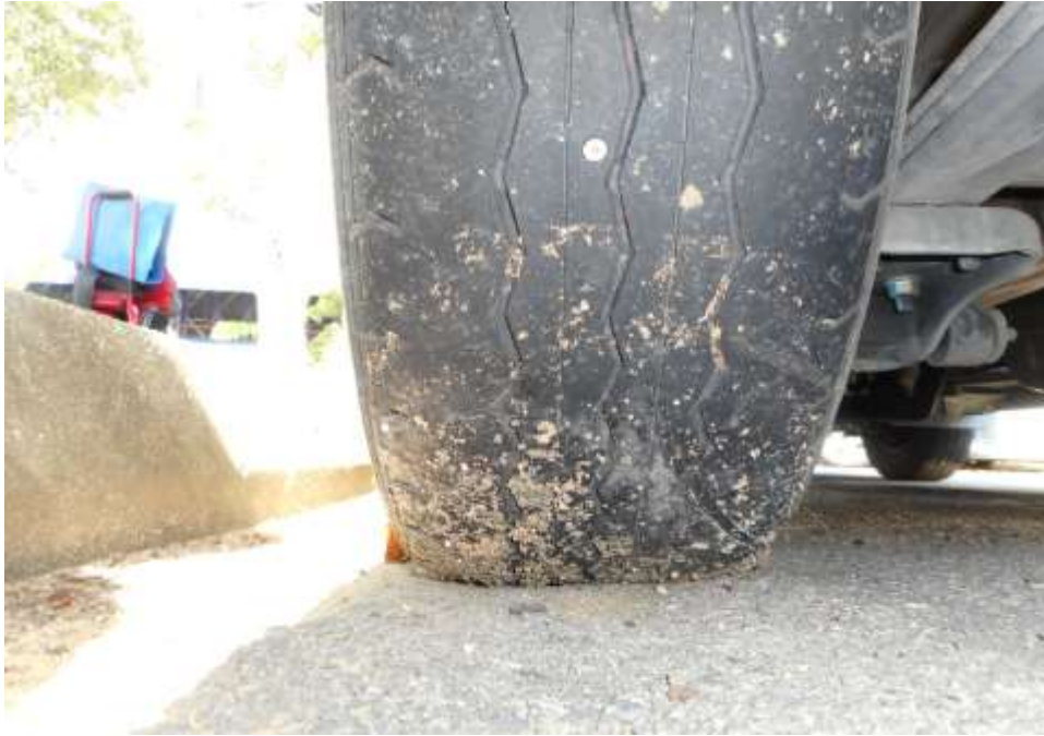
Photo 10 shows the condition of the rear left tyres of the Motor Van, which was observed to be in serviceable condition with remaining tread depth of approximately 2.7mm. The tyres, which were wrapped around standard steel wheel rim, were also observed to be sufficiently inflated for vehicular operation. There was also no damage found on all 4 steel wheel rims of the Motor Van.
