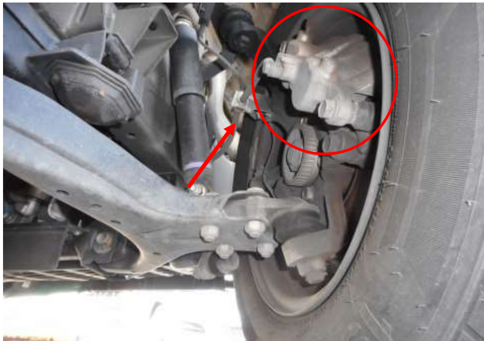
Photo 21 shows the brake hose/pipe (arrowed) at the front right wheel of the Motor Van. No leakage of brake fluid was observed. Visual examination of the various components of the braking system like the brake caliper (circled), brake booster, brake pedal etc had revealed all to be intact and without visible damage at the time of accident. There was also no sign of fluid stain(s) observed on the various undercarriage components.
