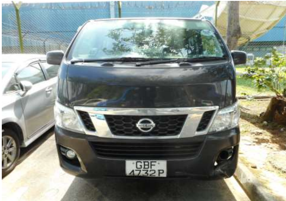
Photo 2 shows a general view of the Motor Van's frontal portion at the time of my inspection. It appeared to have sustained damage at its frontal portion. Its front bumper and front left head lamp were damage at the time of my inspection.
