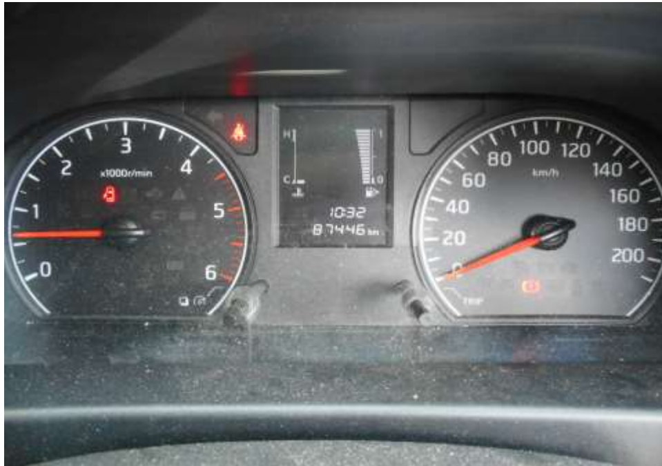
Photo 25 shows no warning lights illuminated on the instrument panel of the Motor Van after the engine was cranked. This would suggest that there was no abnormality to the electronic operating system of the Motor Van, like the ABS and SRS etc.
