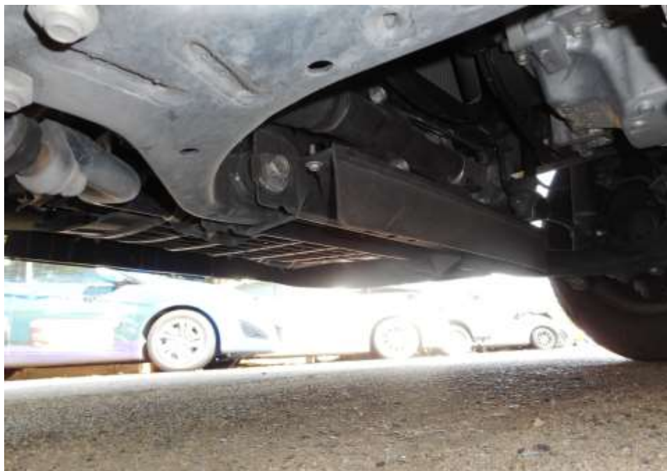
Photo 16 shows the undercarriage of the Motor Van, at the area where the engine housing and transmission housing are located. . I did not find any sign(s) or indication(s) of fluid leak and/or fluid stain(s) on the underside of the Motor Van.
