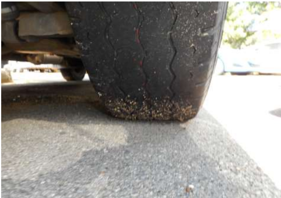
Photo 9 shows the condition of the rear right tyre of the Motor Van, which was observed to be in serviceable condition with remaining tread depth of approximately 2.4mm. The tyre, which was wrapped around standard steel wheel rim, it was observed to be sufficiently inflated for vehicular operation.
