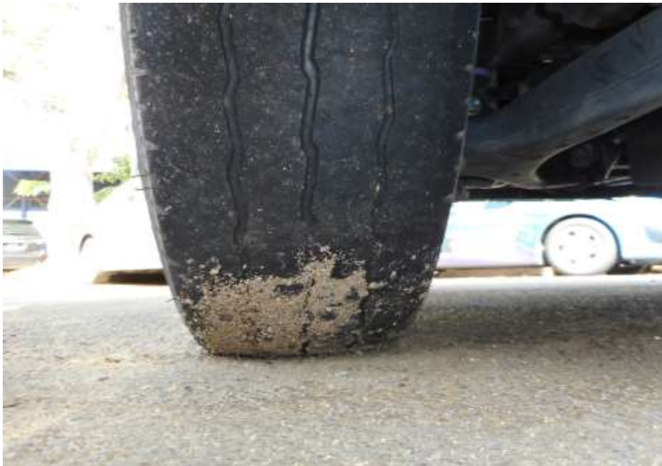
Photo 11 shows the condition of the rear right tyres of the Motor Van, which were observed to be in serviceable condition with remaining, tread depth of approximately 2.1mm. There was also no tear, cut or burst mark(s) on the outer and the inner sidewalls as well as across the tread of the 4 tyres that were fitted on the Motor Van.
