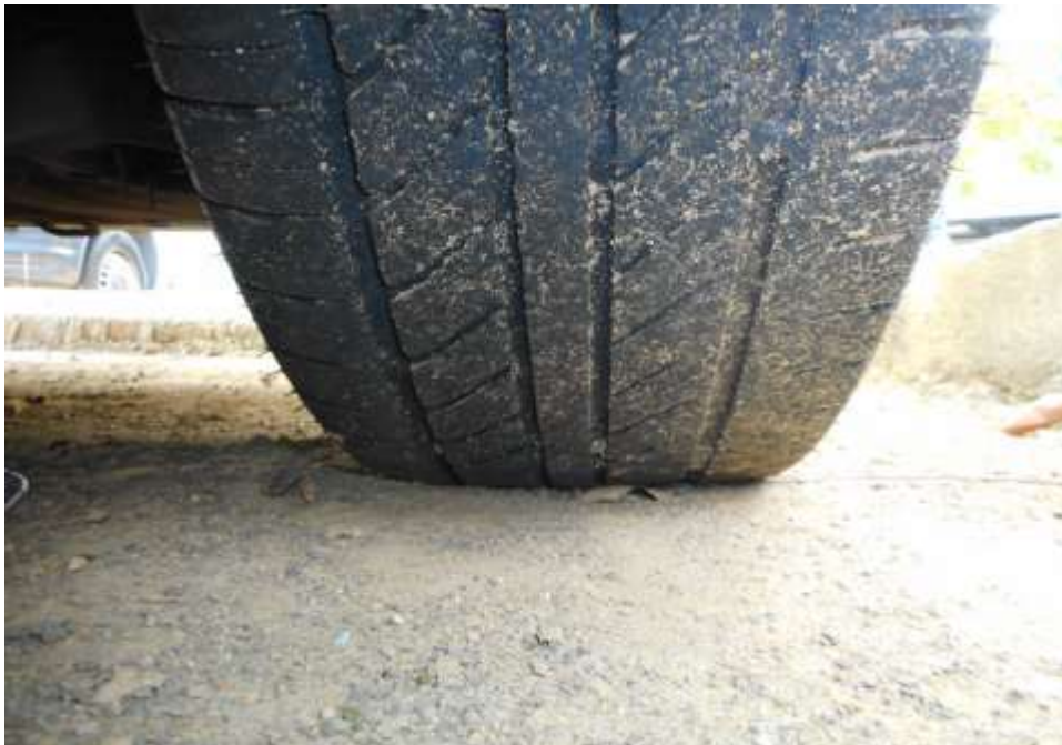
Photo 9 shows the condition of the rear left tyres of the Motor Taxi, which was observed to be in serviceable condition with remaining tread depth of approximately 6.8mm. The tyres, which were wrapped around standard alloy wheel rim, were also observed to be sufficiently inflated for vehicular operation. There was also no damage found on all 4 alloy wheel rims of the Motor Taxi.
