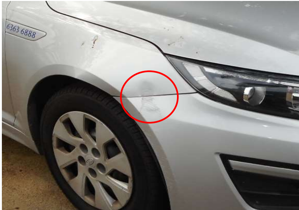
Photo 4 shows a close up view of the right body of the Motor Taxi at the time of my inspection. The Motor Taxi was observed to visually sustain damage at its front right bumper and fender portion (circled).
