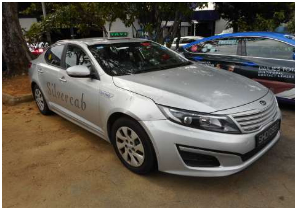
Photo 3 shows a general view of the right body of the Motor Taxi at the time of my inspection. The Motor Taxi was observed to visually sustain damage at its front right bumper and fender portion.
