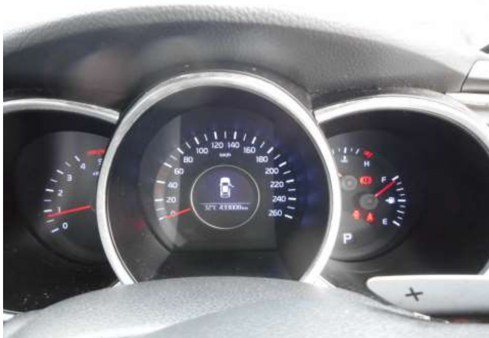
Photo 24 shows no warning lights illuminated on the instrument panel of the Motor Taxi after the engine was cranked. This would suggest that there was no abnormality to the various electronic operating systems of the Motor Taxi, like the ABS, SRS and EPS.
