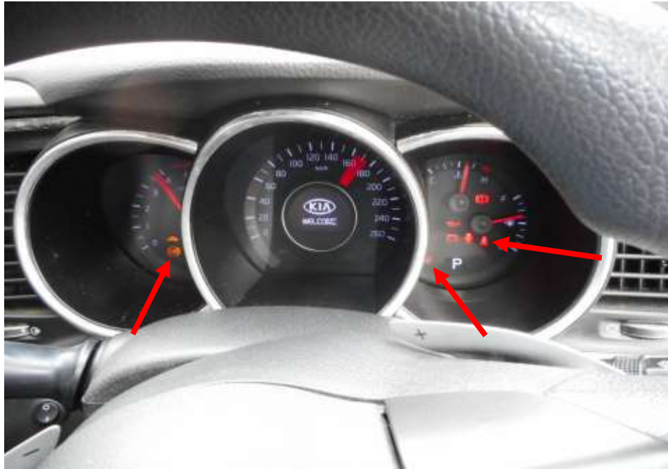
Photo 23 shows the warning light for Anti-Lock Brake System (ABS), Supplemental Restraint System (SRS) and Electric Power Steering System (EPS) appearing on the instrument panel of the Motor Taxi during the self-test of its various electronic operating systems when its engine was cranked.
