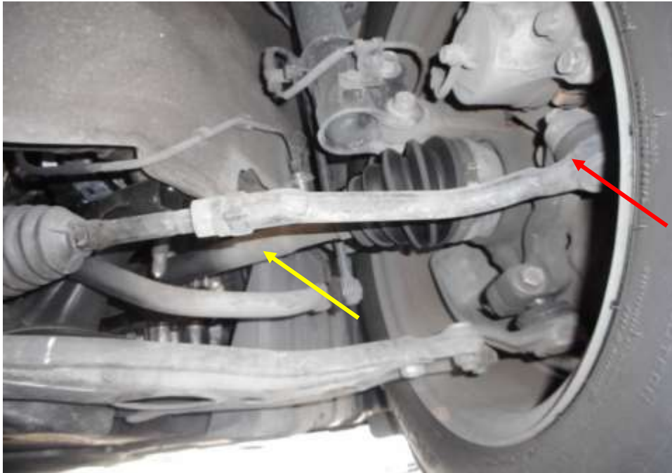
Photo 16 shows the various undercarriage components at the front right wheel of the Motor Taxi, in particular the steering tie rod end (arrowed) and drive shaft (yellow arrow). The various steering components were all found to be intact, suggesting that the steering system of the Motor Taxi was likely to be in serviceable condition at the material time of accident. There was also no sign of fluid stain(s) observed on the various undercarriage components.
