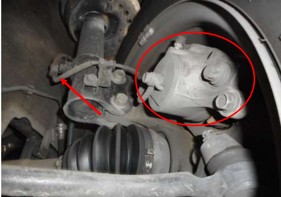
Photo 20 shows the brake hose/pipe (arrowed) at the front right wheel of the Motor Taxi. No leakage of brake fluid was observed. Visual examination of the various components of the braking system like the brake caliper (circled), brake booster, brake pedal etc had revealed all to be intact and without visible damage at the time of accident. There was also no sign of fluid stain(s) observed on the various undercarriage components.
