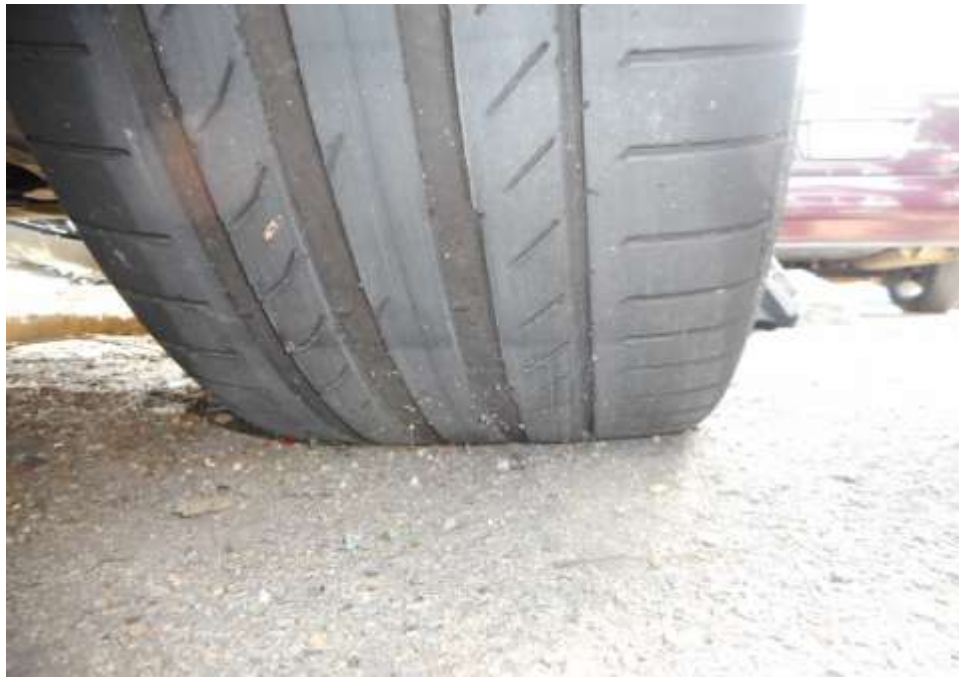
Photo 5 shows the condition of the front right tyre of the Motor Car, which was observed to be in serviceable condition with remaining tread depth of approximately 2.8mm. The tyre, which was wrapped around alloy wheel rim, was also observed to be sufficiently inflated for vehicular operation.
