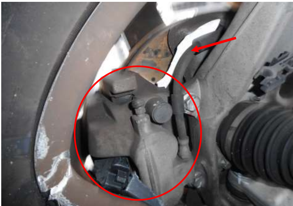
Photo 14 shows the brake hose/pipe (arrowed) at the front left wheel of the Motor Car. No leakage of brake fluid was observed. Visual examination of the various components of the braking system like the brake caliper (circled), brake booster, brake pedal etc had revealed all to be intact and without visible damage at the time of accident. There was also no sign of fluid stain(s) observed on the various undercarriage components.
