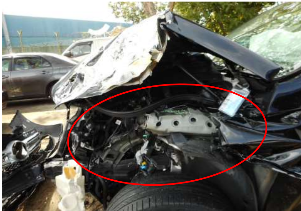
Photo 4 shows a close up view of the Motor Car's engine compartment at the time of my inspection. Due to the induced impact of the accident, the Motor Car's engine system, ignition system, cooling system (circled) and various components in the engine compartments were also damaged as a result of the accident.
