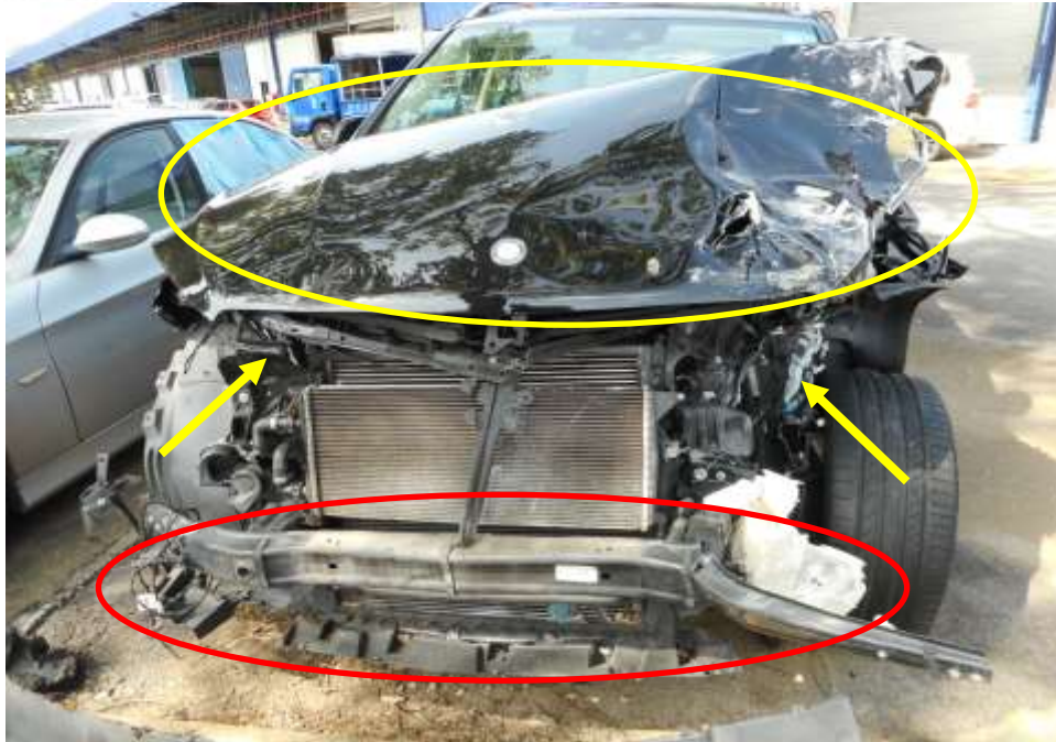
Photo 3 shows the close up view of the Motor Car's front body at the time of my inspection. The Motor car was observed to have sustained damage at its front portion. Its front bonnet (red circle), front bumper (red circle) and both front headlamp (yellow arrow) was amongst the body parts and various components in the engine compartments were also damaged as a result of the accident.
