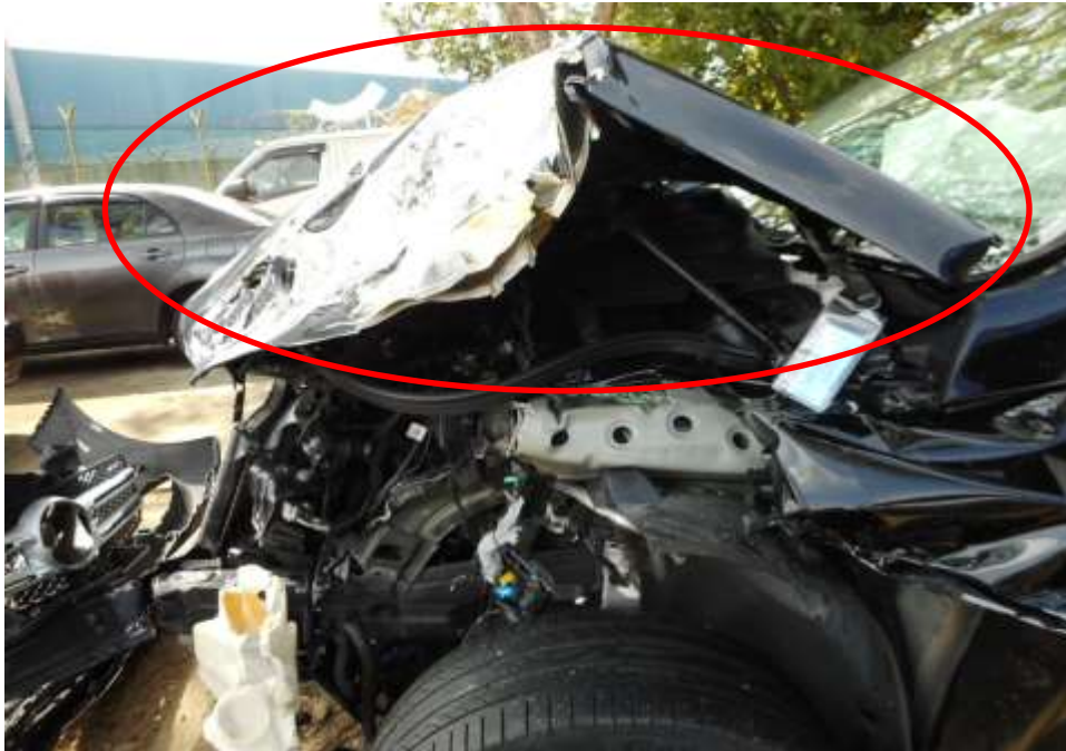
Photo 10 shows a close up view of the damaged front bonnet lock mechanism and the structure of the engine compartment of the Motor Car at the time of my inspection resulting it unable to open a result of the accident. (circled) (Unable to open)
