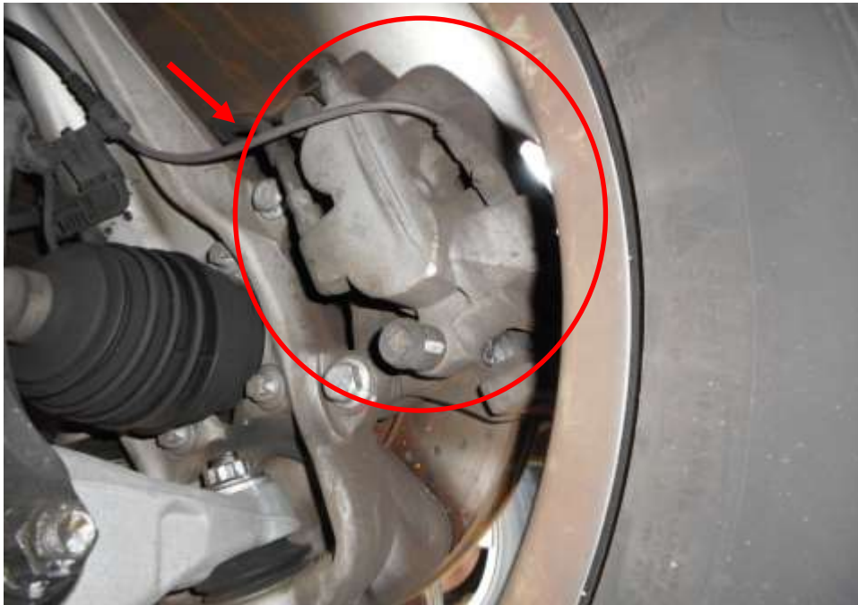
Photo 13 shows the brake hose/pipe (arrowed) at the front right wheel of the Motor Car. No leakage of brake fluid was observed. Visual examination of the various components of the braking system like the brake caliper (circled), brake booster, brake pedal etc had revealed all to be intact and without visible damage at the time of accident. There was also no sign of fluid stain(s) observed on the various undercarriage components.
