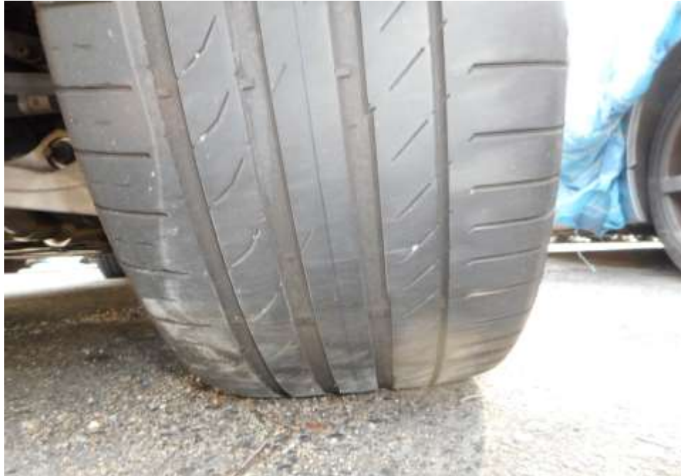
Photo 6 shows the condition of the rear right tyre of the Motor Car, which was observed to be in serviceable condition with remaining tread depth of approximately 3.1mm. The tyre was also observed to be sufficiently inflated for vehicular operation with no tear, cut or burst mark(s).
