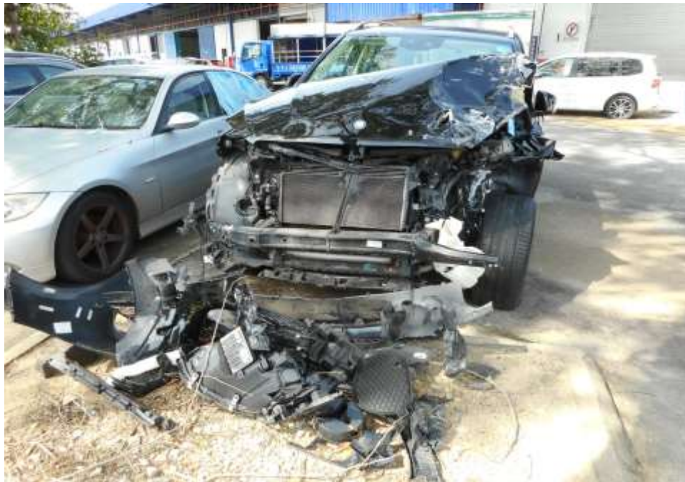
Photo 2 shows a general view of the Motor Car's front body at the time of my inspection. The Motor car was observed to have sustained damage at its front portion. Its front bonnet, front bumper and both front headlamp was amongst the body parts and various components in the engine compartments were also damaged as a result of the accident. The Supplemental Restraint System (SRS) was activated as a result of the accident.
