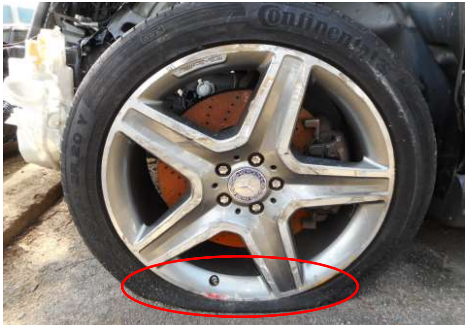
Photo 8 shows the condition of the front left tyre of the Motor Car, the rim was observed to be damaged (circled) as a result of the accident and the tyre was observed to be in deflated condition due to the air leakage from the damaged rim. The remaining tread depth of the tyre was approximately 3.4mm. There was also no tear, cut or burst mark(s) on the outer and the inner sidewalls as well as across the tread of the Motor Car's 4 tyres.
