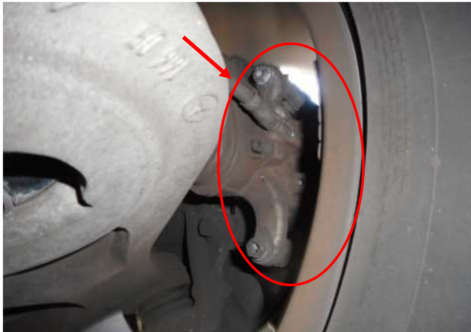
Photo 12 shows the brake caliper (circled) brake hose/pipe (arrowed) at the rear right wheel of the Motor Car and it was observed to be intact
