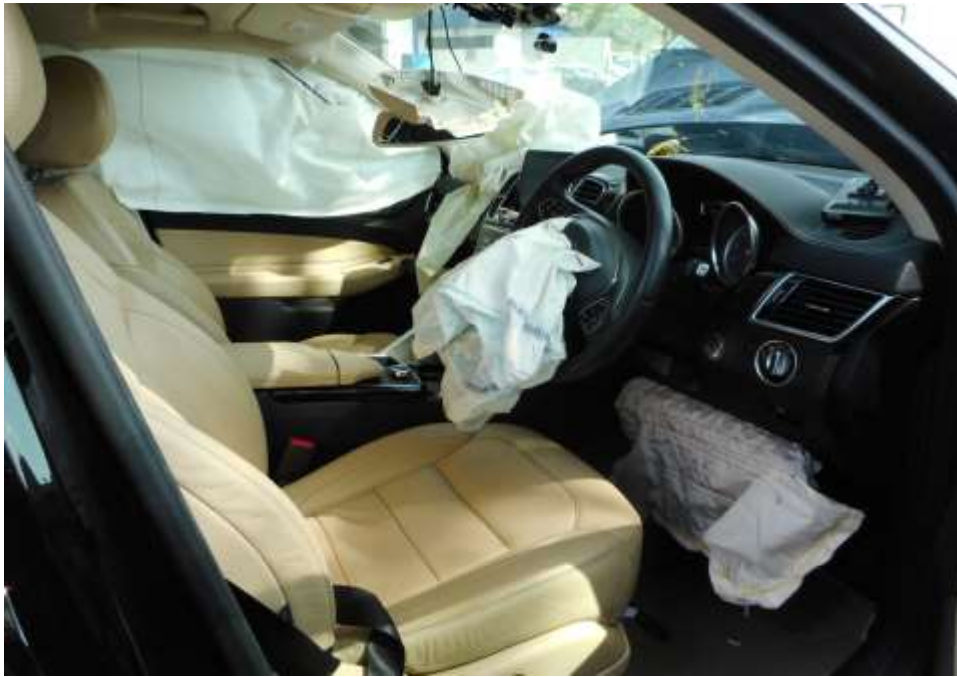
Photo 9 shows the deployment of the Supplemental Restraint System (SRS) airbag (arrowed) in the Motor Car as a result of the accident.
