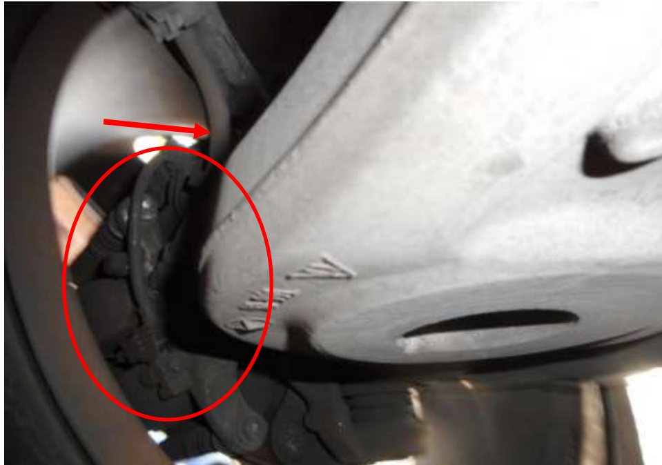
Photo 11 shows the brake caliper (circled) and brake hose/pipe (arrowed) at the rear left wheel of the Motor Car and it was observed to be intact
