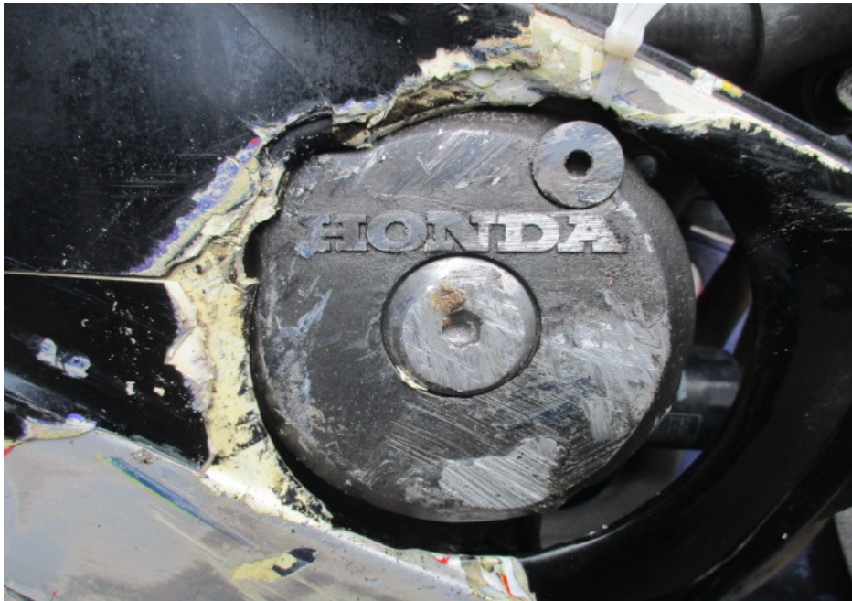
Photo 20 shows the right side of the engine of the Motorcycle at the time of our inspection. The various right engine components had sustained damage of grazing nature as a result of the accident however the engine components were still intact. There was also no fluid leak and/or fluid stain found around the right engine area of the Motorcycle.
