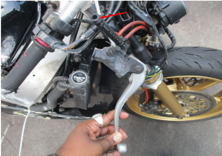
Photo 28 shows the front brake lever of the Motorcycle. However we observed that the front brake reservoir was missing as a result of the accident (arrowed). Therefore we were unable to conduct any static brake test on the front braking system of the Motorcycle.
