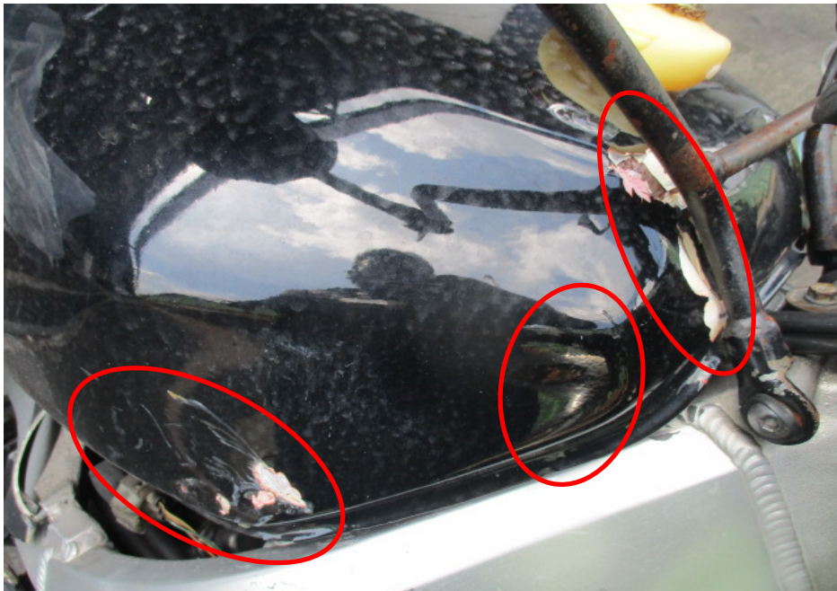
Photo 6 shows a closer view of the dented petrol tank, which was amongst the body parts of the Motorcycle that had sustained damage as a result of the accident.
