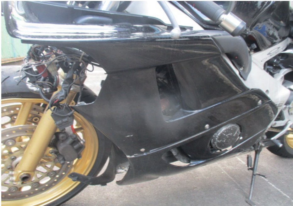
Photo 9 shows a closer view of the left cowling which was amongst the body parts at the front body of the Motorcycle that had sustained damages as a result of the accident.
