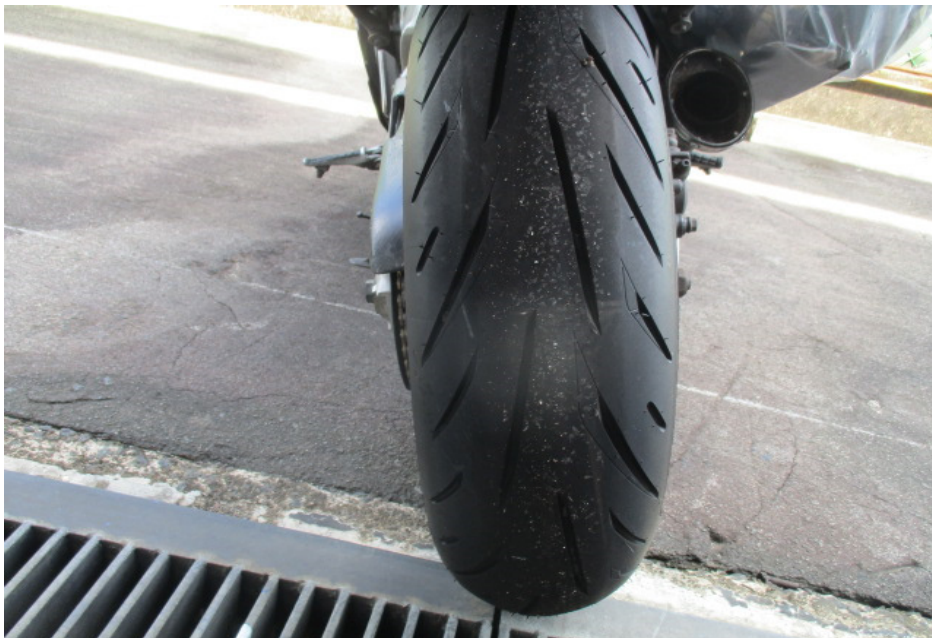
Photo 18 shows the condition of the Motorcycle's rear tyre. The rear tyre was observed to be in serviceable condition with remaining tread depth of approximately 4mm. The tyre was also observed to be sufficiently inflated for vehicular operation. We did not observe any tear, burst mark(s) and/or punctured hole(s) on the sidewalls as well as across the tread of the rear tyre.
