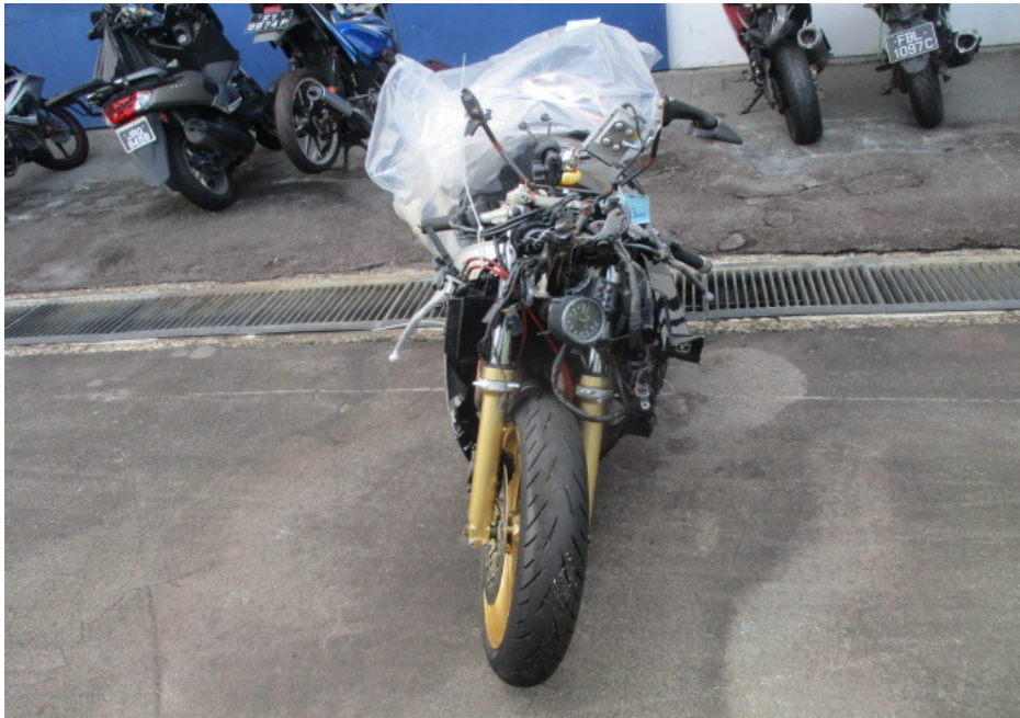
Photo 3 shows a general view of the frontal portion of the Motorcycle at the time of our inspection. The Motorcycle had sustained damages all around. Body parts that were found to have been damaged include its headlight assembly, speedometer, side mirrors, clutch lever, front brake lever, right side frame, petrol tank, rear brake pedal, right front footrest, exhaust muffler and rear side covers, amongst others.
