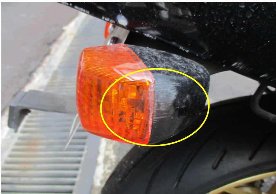
Photo 16 shows the damaged right rear signal lamp (circled) of the Motorcycle as a result of the accident.
