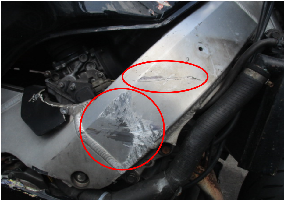
Photo 7 shows the damaged right side frame (circled) of the Motorcycle. The damage sustained at the side frame of the Motorcycle was mainly of grazing nature.
