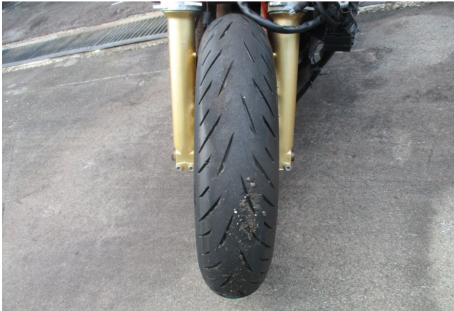
Photo 17 shows the front tyre of the Motorcycle at the time of our inspection. The front tyre was observed to be in serviceable condition with remaining tread depth of approximately 4mm. The pattern of the tread was also clearly visible. There was no tear, burst mark(s) and/or punctured hole(s) on the sidewalls as well as across the tread of the front tyre.
