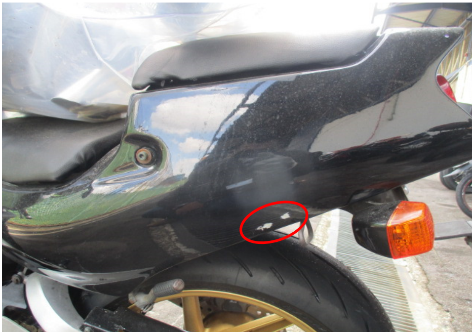
Photo 12 shows the right rear cover (circled) which was amongst the body parts at the rear body of the Motorcycle that had sustained damages as a result of the accident.
