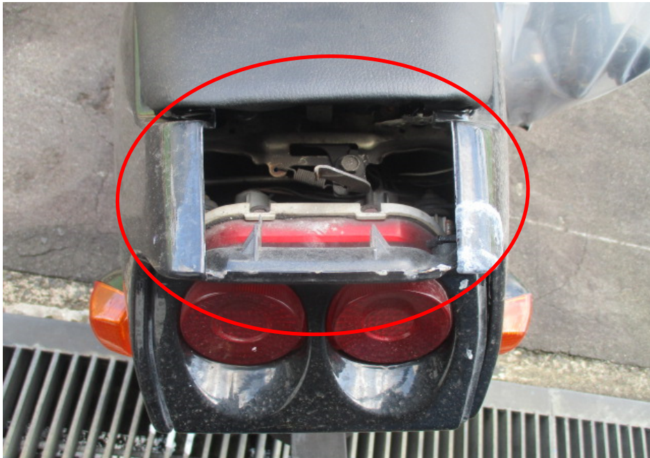
Photo 15 shows the damaged rear cover (circled) of the Motorcycle as a result of the accident.
