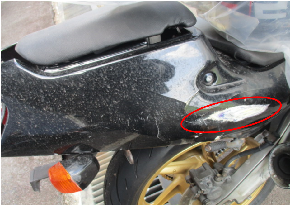
Photo 11 shows the right rear cover (circled) which was amongst the body parts at the rear body of the Motorcycle that had sustained damages as a result of the accident.
