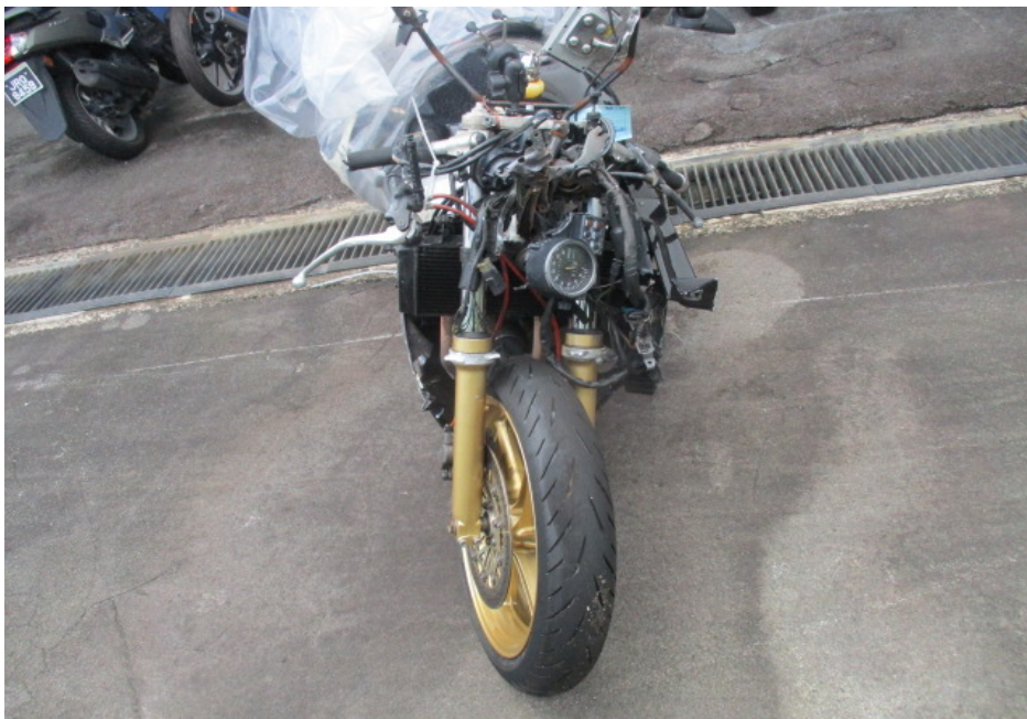
Photo 25 shows the front wheel of the Motorcycle turned towards its full left. Turning the Motorcycle's handle bar towards the left and right did not produce any abnormal free play and/or resistance. This would indicate that the steering system of the Motorcycle was in serviceable condition at the time of our inspection.
