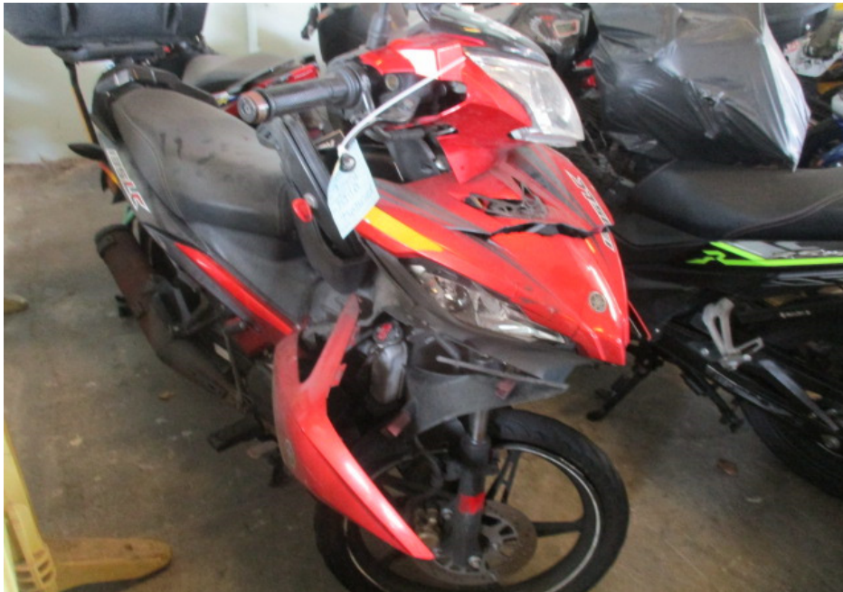
Photo 3 shows a general view of the right front body of the Motorcycle at the time of our inspection. The Motorcycle had sustained damages at its frontal portion. Body parts that were found to have been damaged include its headlight assembly, front cowlings, front fork assembly, side cowlings, side mirrors, front brake lever, right handlebar end, left handlebar grip and top box, amongst others.
