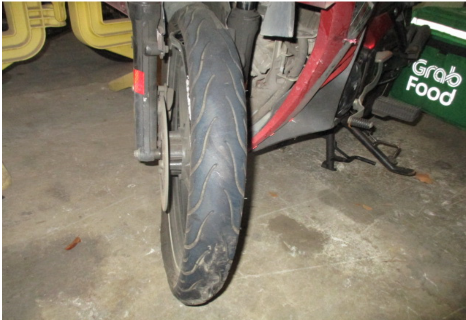
Photo 13 shows the punctured front tyre of the Motorcycle most likely as a result of the accident at the time of our inspection. The front tyre was observed to be in serviceable condition with remaining tread depth of approximately 3mm. The pattern of the tread was also clearly visible. There was no tear, burst mark(s) and/or punctured hole(s) on the sidewalls as well as across the tread of the front tyre.
