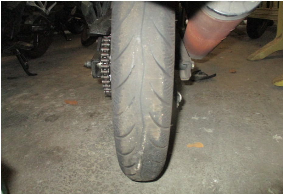
Photo 14 shows the condition of the Motorcycle's rear tyre. The rear tyre was observed to be in serviceable condition with remaining tread depth of approximately 3mm. The tyre was also observed to be sufficiently inflated for vehicular operation. We did not observe any tear, burst mark(s) and/or punctured hole(s) on the sidewalls as well as across the tread of the rear tyre.
