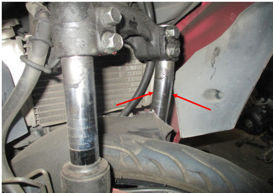
Photo 19 shows the front forks of the Motorcycle. The front left fork (arrowed) was observed to be bent inwards as a result of the accident. We were hence not able to conduct any tests on the steering system of the Motorcycle.
