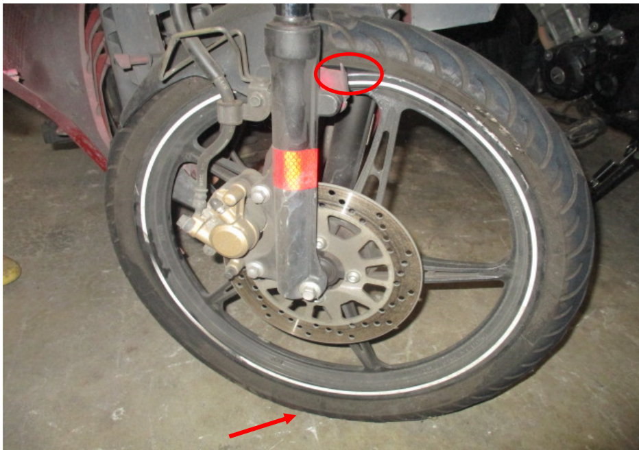
Photo 12 shows the bent front wheel rim (circled) and deflated front tyre (arrowed) of the Motorcycle as a result of the accident at the time of our inspection.
