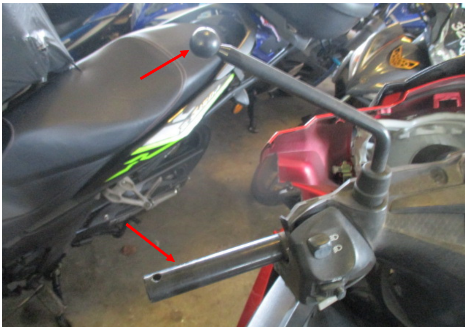
Photo 10 shows a closer view of the missing left side mirror and left handlebar grip (arrowed), which were amongst the body parts of the Motorcycle that had sustained damage as a result of the accident (circled).
