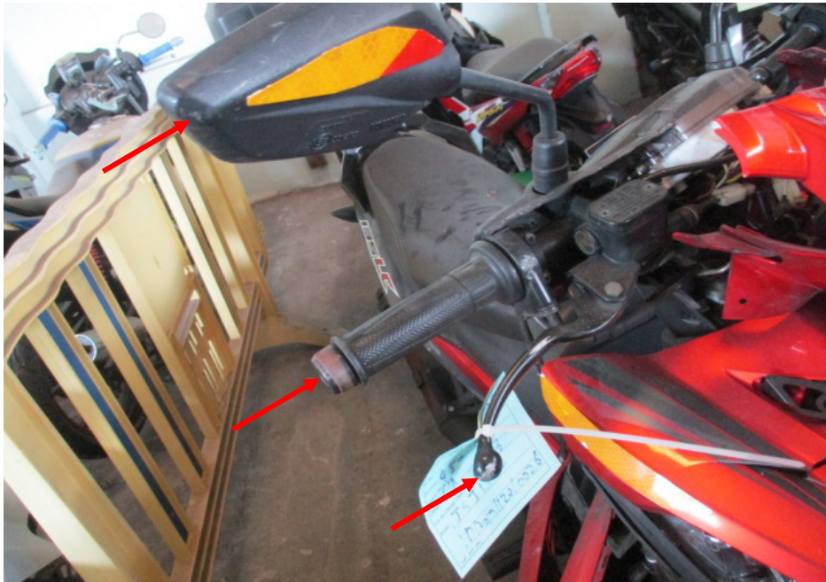
Photo 5 shows a closer view of the front brake lever, right side mirror and right handlebar end (arrowed) of the Motorcycle. These parts were amongst the body parts of the Motorcycle which were damaged as a result of the accident.
