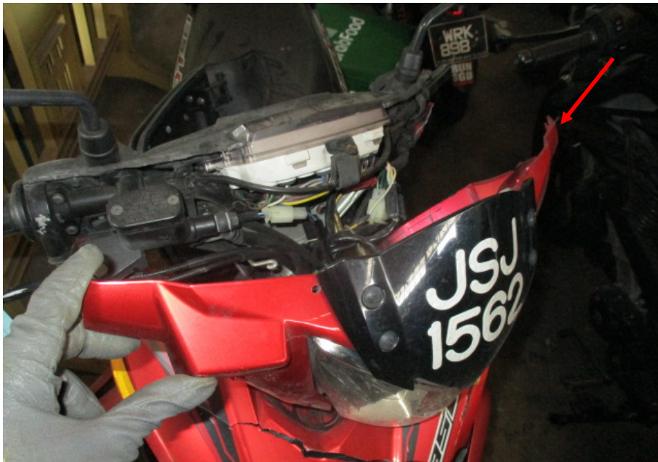
Photo 4 shows a closer view of the headlight assembly which was amongst the body parts at the front body of the Motorcycle that had sustained damages as a result of the accident (arrowed).
