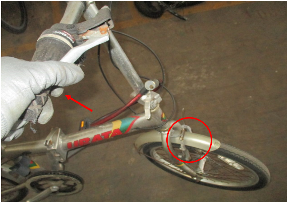
Photo 20 shows a static brake test conducted on the Bicycle's front brake. There was some resistance felt upon pressing the right hand brake lever (arrowed). It also shows that the front brake clamps responded to the gripping action (circled) after depressing the right hand brake lever.
