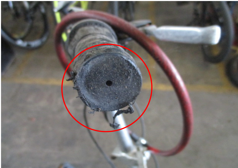
Photo 7 shows the damaged right handlebar grip (circled) of the Bicycle at the time of our inspection.
