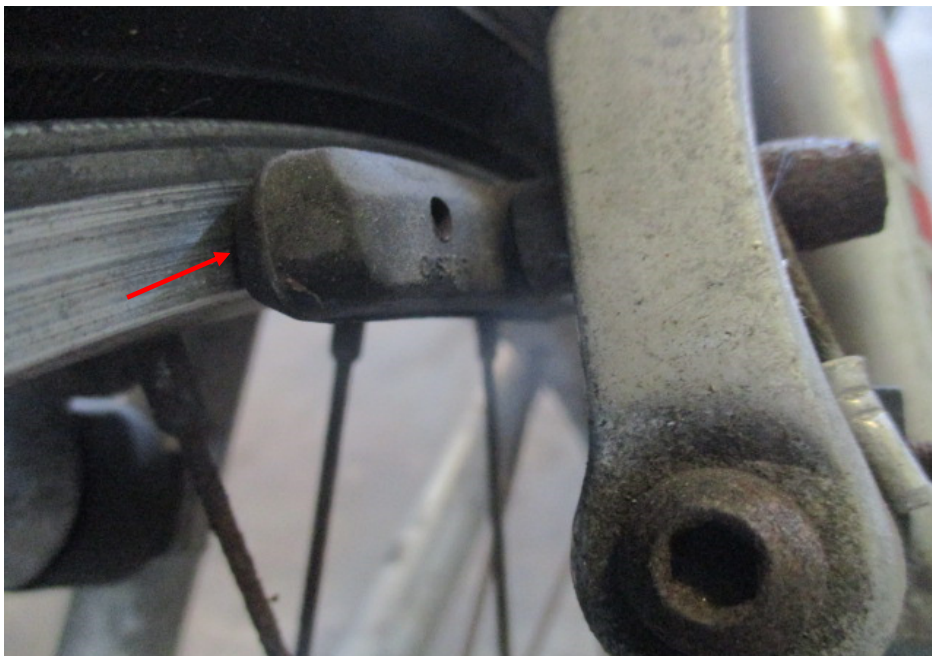
Photo 23 shows a close up view of the rear brake clamps responding to the gripping action. The rubber brake blocks pressed against the rear wheel rim upon depressing the left hand brake lever (arrowed). This had appeared to indicate that the rear brake was in serviceable condition.
