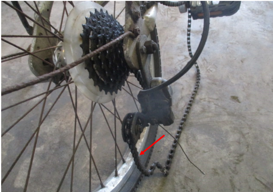
Photo 16 shows a closer view of the dislodged chain from the gear train of the Bicycle, most likely as a result of the accident. It was found to be adequately lubricated for operating purposes (arrowed).
