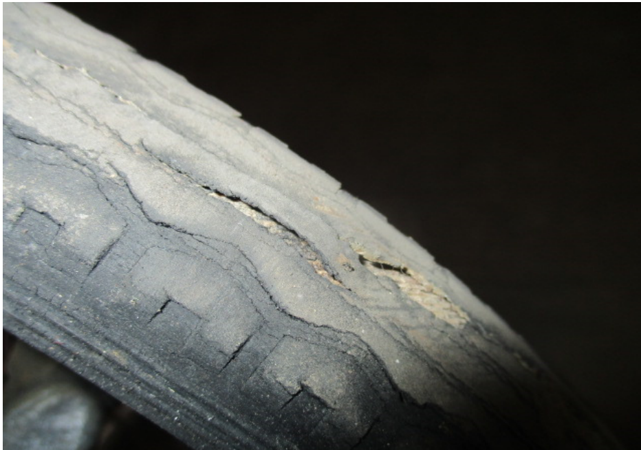
Photo 13 shows a closer view of the cut/tear on the tread area of the front tyre of the Bicycle observed upon our inspection.
