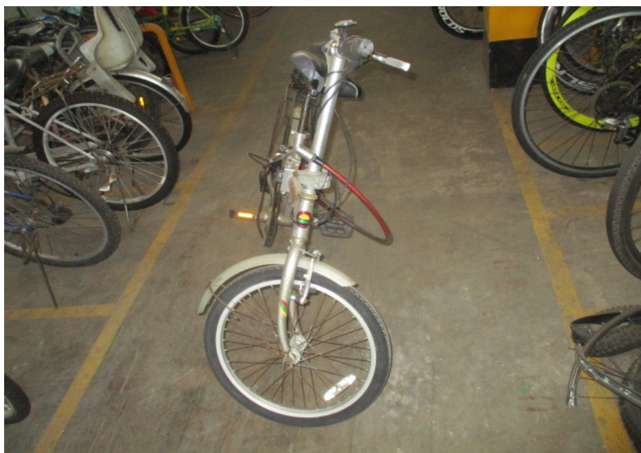
Photo 19 shows the front wheel of the Bicycle turned towards its full left. Turning the Bicycle's handle bar towards the left did not produce any abnormal free play and/or resistance. This would indicate that the steering system of the Bicycle was in serviceable condition at the time of our inspection.
