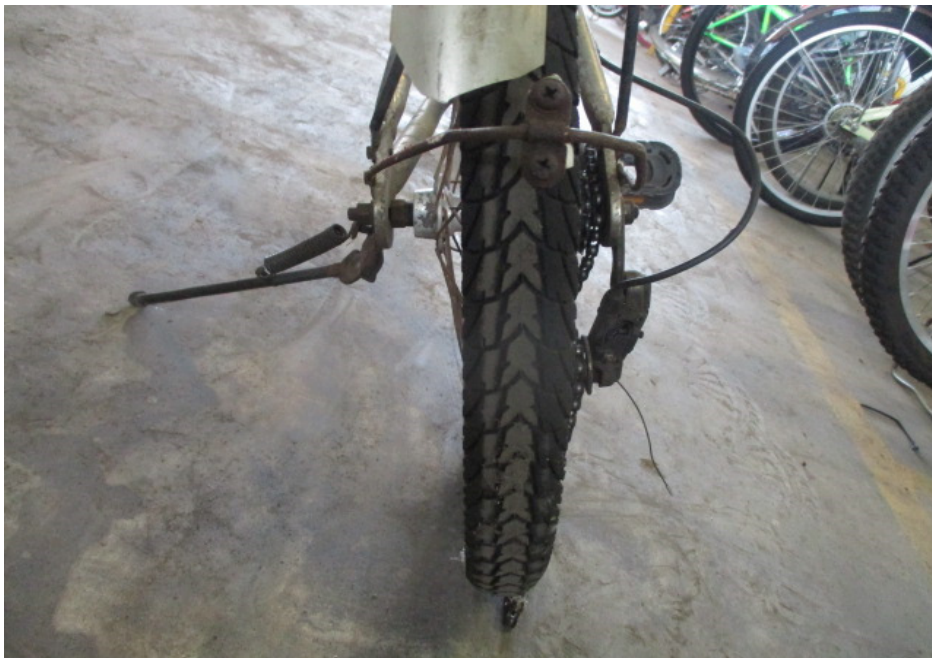
Photo 14 shows the rear tyre of the Motorcycle. The pattern of the tread was clearly visible. There was no tear, burst mark(s) and/or punctured hole(s) on the sidewalls as well as across the tread of the rear tyre. However the rear tyre was observed to be deflated.
