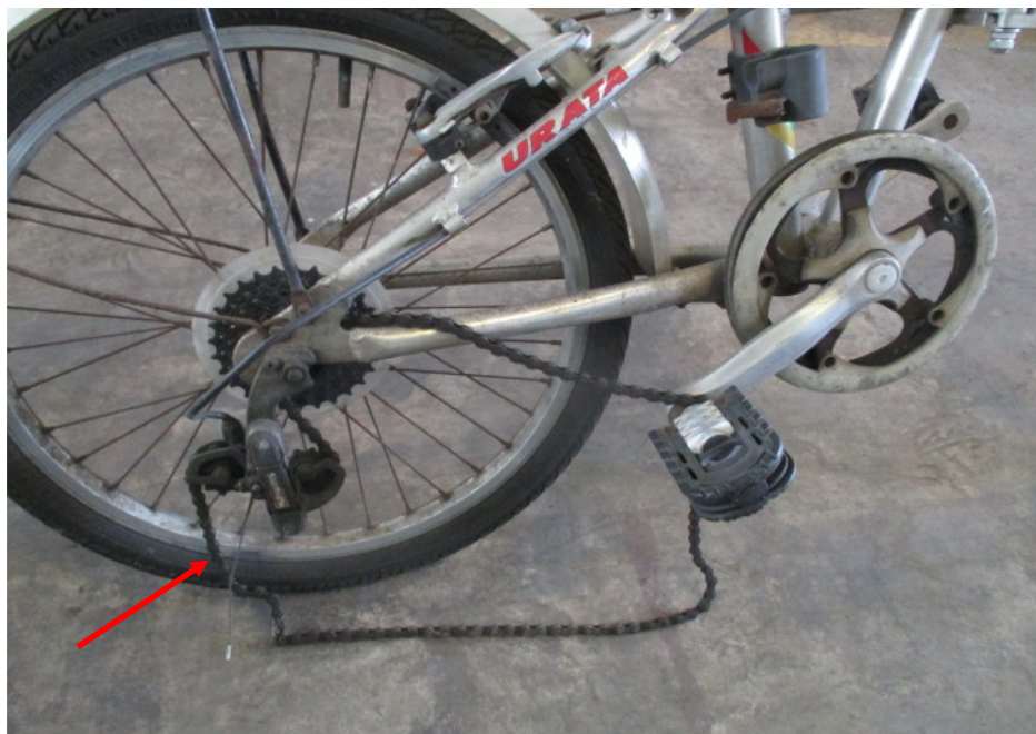
Photo 15 shows the general view of the gear train of the Bicycle, which was observed to be intact with no misalignment. It was also adequately lubricated for operating purposes. However the chain was observed to be dislodged from the gear train most likely as a result of the accident (arrowed).
