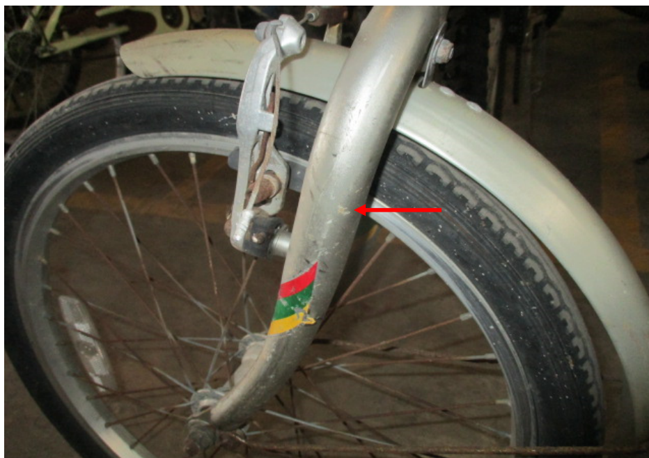
Photo 6 shows the damages of grazing nature sustained to the front left fork (arrowed) of the Bicycle at the time of our inspection.
