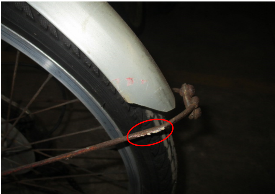
Photo 10 shows the damages of grazing nature on the rear mudguard (circled) of the Bicycle at the time of our inspection.
