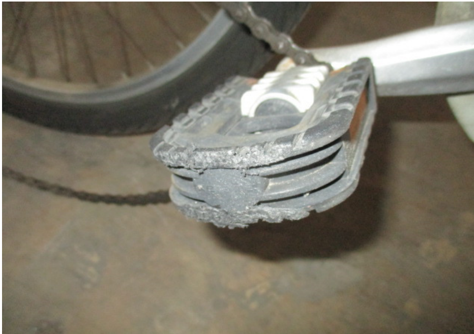
Photo 9 shows the damaged right pedal of the Bicycle at the time of our inspection.
