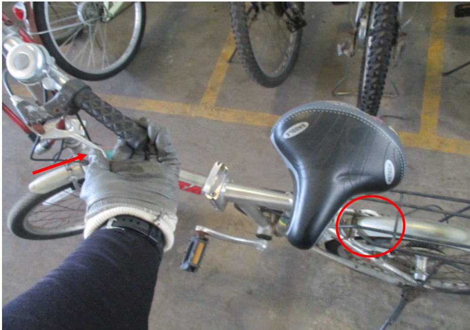
Photo 22 shows a static brake test conducted on the Bicycle's rear brake. There was some resistance felt upon pressing the left hand brake lever (arrowed). It also shows that the rear brake clamps responded to the gripping action (circled) after depressing the left hand brake lever.
