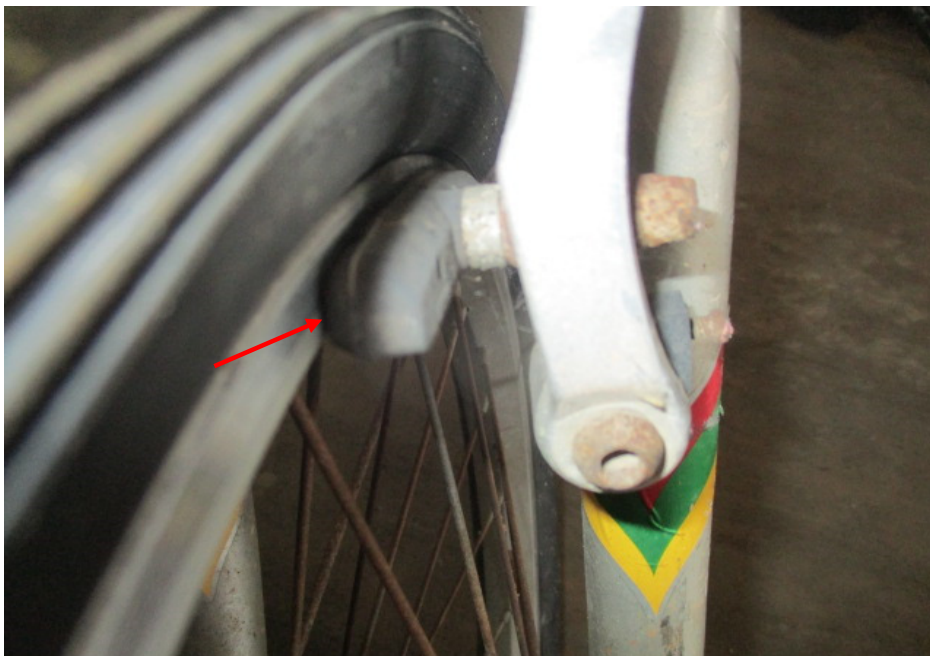
Photo 21 shows a close up view of the front brake clamps responding to the gripping action. The rubber brake blocks pressed against the front wheel rim upon depressing the right hand brake lever (arrowed). This had appeared to indicate that the front brake was in serviceable condition.
