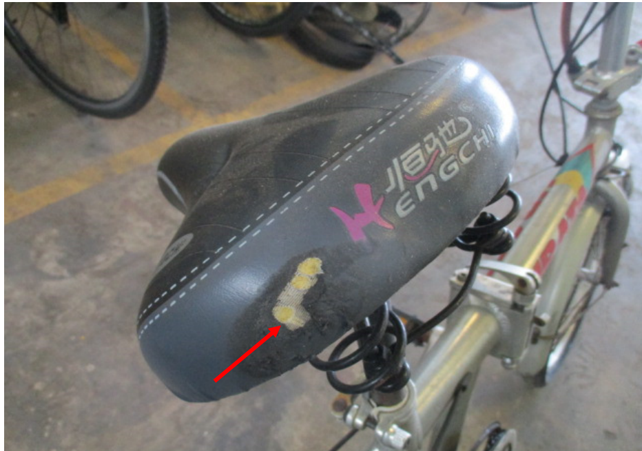
Photo 11 shows a close-up view of the torn seat (arrowed) of the Bicycle as a result of the accident.
