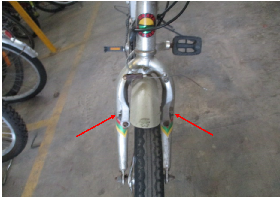
Photo 17 shows the front forks (arrowed) of the Bicycle. The front fork and fork bracket of the Bicycle were both found to be intact and undamaged. Turning the Bicycle's handle bar towards the left and right did not produce any abnormal free play. The steering system of the Bicycle was in serviceable condition at the time of our inspection.
