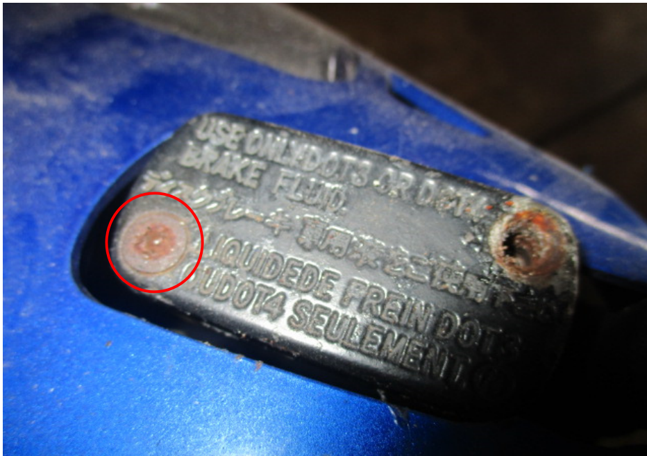
Photo 21 shows the brake fluid reservoir cover for the front brake of the Motorcycle. We were unable to examine whether the brake fluid was of sufficient level and without contamination for operational purposes due to the worn out screw (circled).
