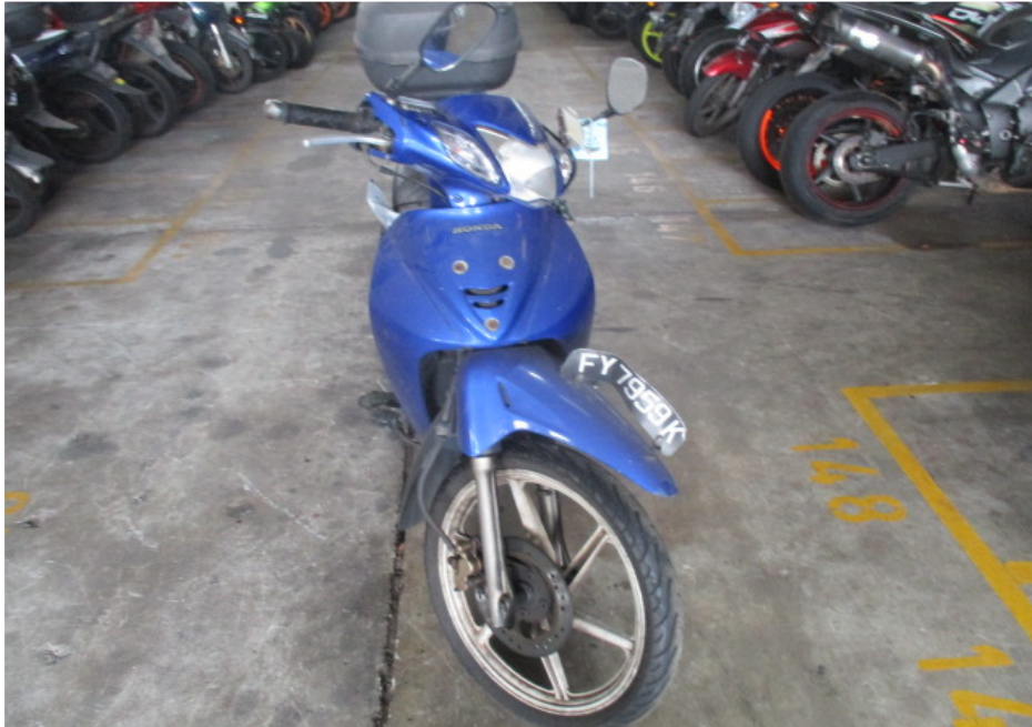
Photo 18 shows the front wheel of the Motorcycle turned towards its full left. Turning the Motorcycle's handle bar towards the left and right did not produce any abnormal free play and/or resistance. This would indicate that the steering system of the Motorcycle was in serviceable condition at the time of our inspection.
