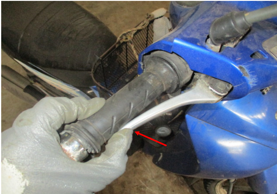
Photo 22 shows the front brake lever being depressed. There was no resistance felt (spongy like feel) upon pressing the front brake lever (arrowed). This would indicate that there may be a leakage of pressure/vacuum in the brake system.
