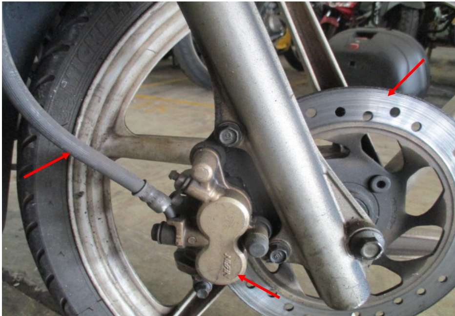
Photo 20 shows a close up view of the front brake caliper, front brake disc and front brake hose (arrowed) of the Motorcycle, which are all part of the components in the hydraulic front brake system of the Motorcycle. Our visual checks of these various components had revealed all to be intact with no visible damage. No leakage of brake fluid was also observed.
