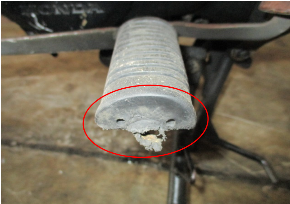
Photo 8 shows a closer view of the left front footrest (circled) which was amongst the body parts of the Motorcycle that had sustained damage as a result of the accident.
