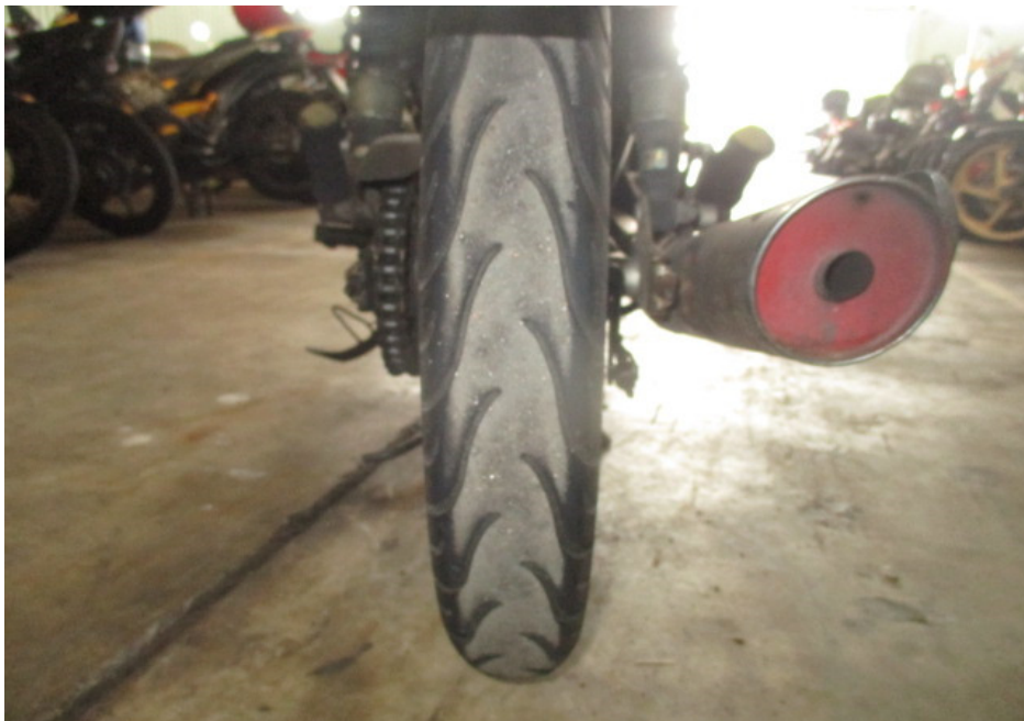
Photo 12 shows the condition of the Motorcycle's rear tyre. The rear tyre was observed to be in serviceable condition with remaining tread depth of approximately 3mm. The tyre was also observed to be sufficiently inflated for vehicular operation. We did not observe any tear, burst mark(s) and/or punctured hole(s) on the sidewalls as well as across the tread of the rear tyre.
