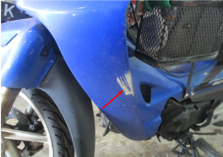
Photo 7 shows a closer view of the left cowling of the Motorcycle that had sustained damage as a result of the accident (arrowed).
