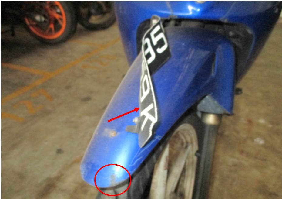
Photo 5 shows a closer view of the front mudguard (circled) and front number plate (arrowed) which were amongst the body parts at the front body of the Motorcycle that had sustained damage as a result of the accident.
