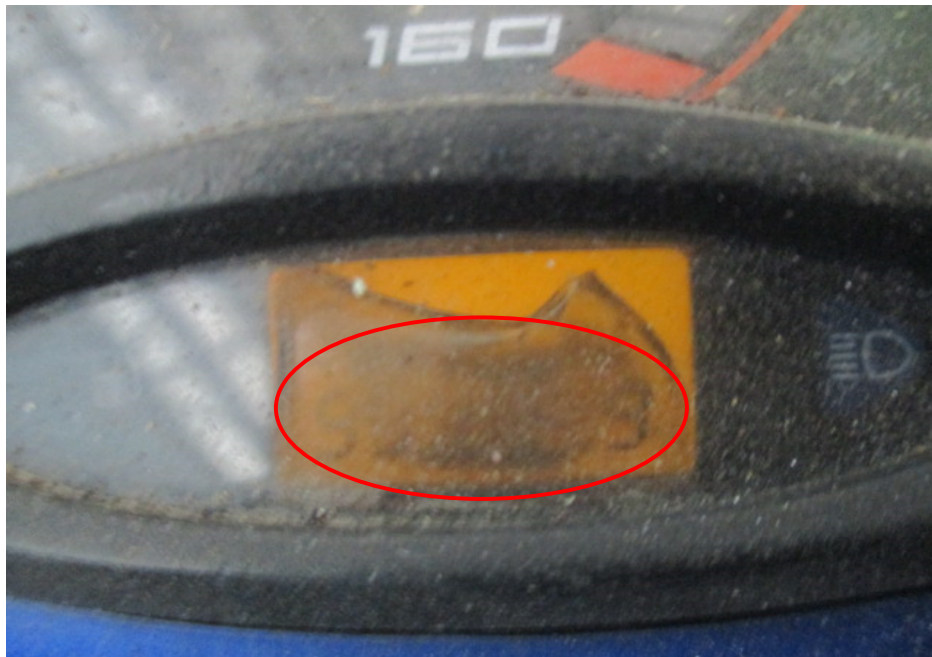
Photo 1 shows the speedometer gauge of the Motorcycle. The mileage of the Motorcycle could not be recorded at the time of our inspection due to a damaged speedometer display (circled).
