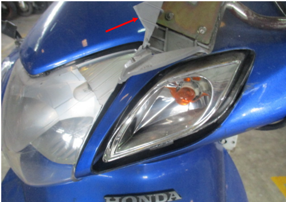
Photo 4 shows a closer view of the headlight assembly and IU Unit (arrowed) which were amongst the body parts at the front body of the Motorcycle that had sustained damage as a result of the accident.
