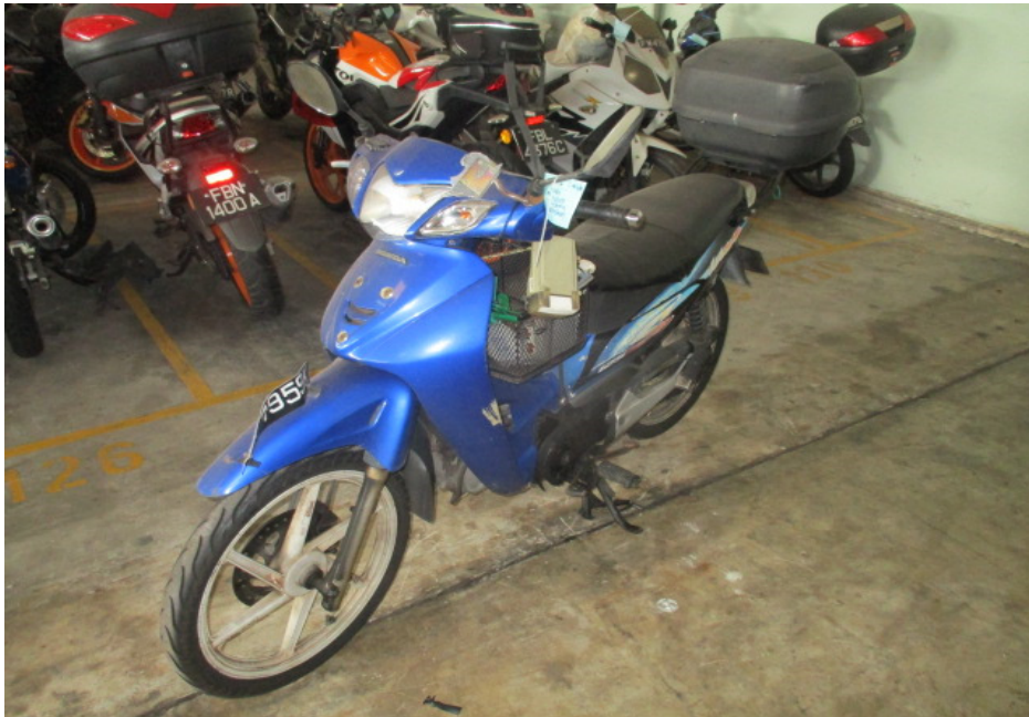
Photo 3 shows a general view of the left front body of the Motorcycle at the time of our inspection. The Motorcycle was observed to have sustained damages all around. Amongst the body parts that were found to have been damaged include its headlight assembly, front mudguard, front number plate, IU unit, left side mirror, left handlebar end, left cowling, left front footrest, exhaust muffler and top box, amongst others.
