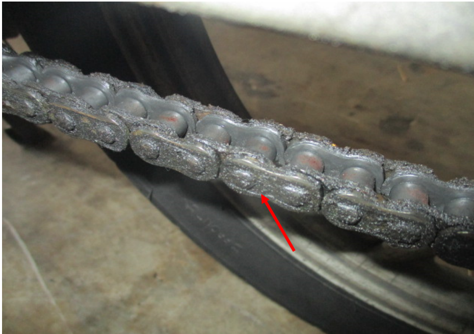
Photo 16 shows a closer view of the gear train (arrowed) of the Motorcycle, which was observed to be intact with no misalignment. It was also adequately lubricated for operating purposes.
