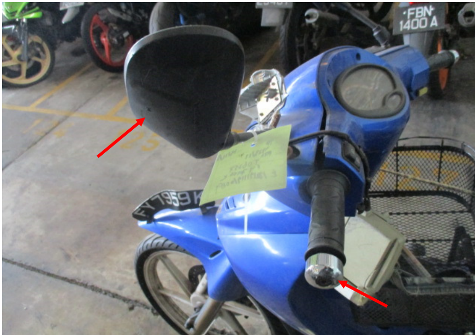
Photo 6 shows a closer view of the left handlebar end as well as the left side mirror (arrowed) which were amongst the body parts of the Motorcycle that had sustained damage as a result of the accident.
