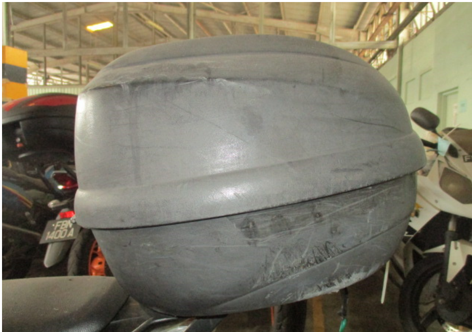
Photo 10 shows the top box of the Motorcycle which was observed to have sustained damages of grazing nature as a result of the accident.
