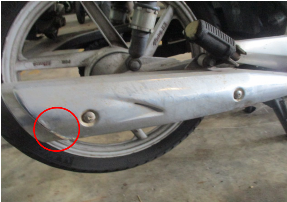
Photo 9 shows a close up view of the exhaust muffler and exhaust muffler heat shield (circled) which were amongst the body parts of the Motorcycle that had sustained damage as a result of the accident.
