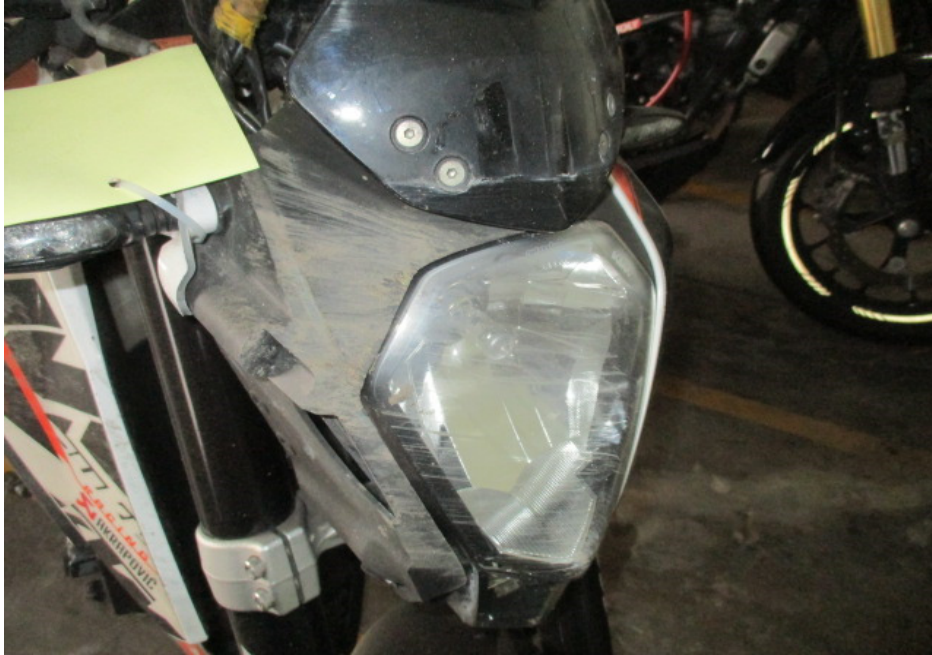
Photo 6 shows a close up view of the head cowl and headlight assembly which were amongst the body parts of the Motorcycle that had sustained damages of grazing nature as a result of the accident.
