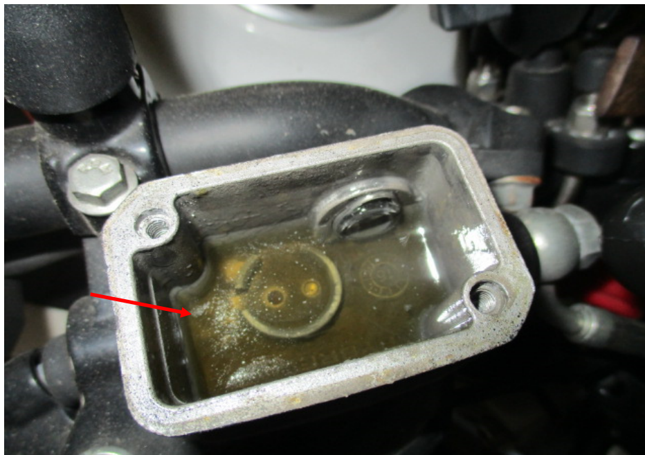
Photo 26 shows the brake fluid reservoir for the front brake of the Motorcycle. The brake fluid was found to be of sufficient level for operating purposes. However the brake fluid was found to be slightly contaminated (arrowed).
