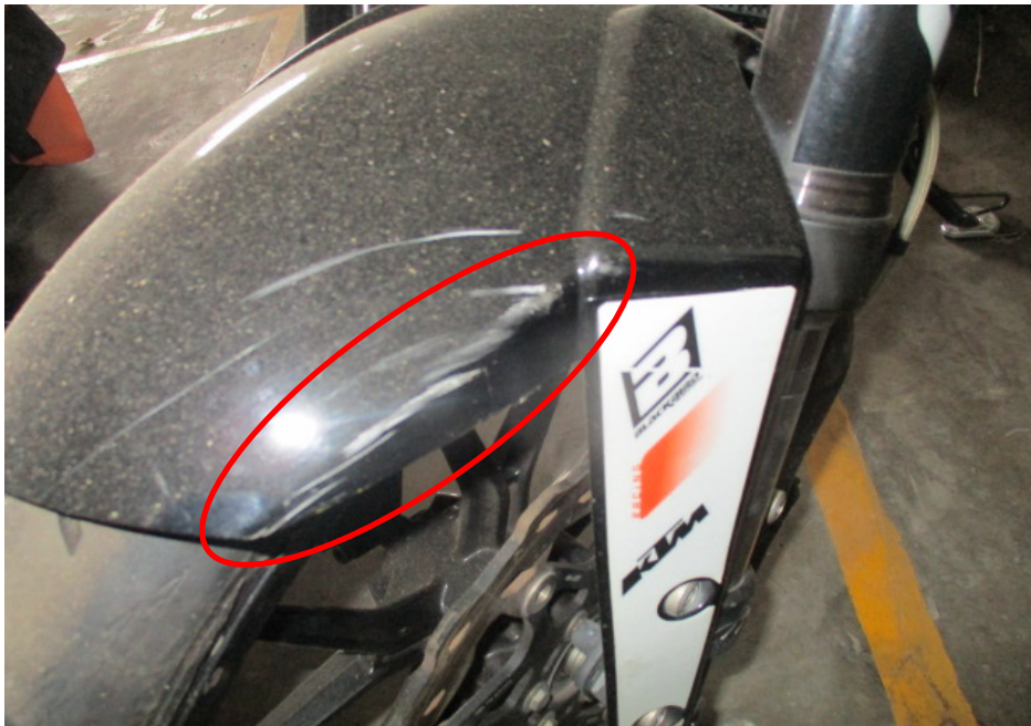
Photo 7 shows a closer view of the front mudguard (circled) which was amongst the body parts at the front body of the Motorcycle that had sustained damage as a result of the accident.
