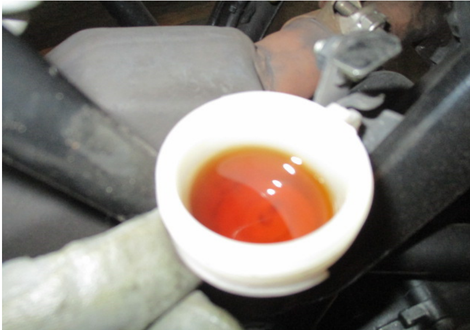
Photo 29 shows the brake fluid reservoir for the rear brake of the Motorcycle. The brake fluid was observed to be of sufficient level and without contamination for operational purposes.
