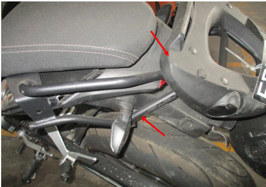
Photo 11 shows the bent top box rack and top box base plate (arrowed) of the Motorcycle as a result of the accident.
