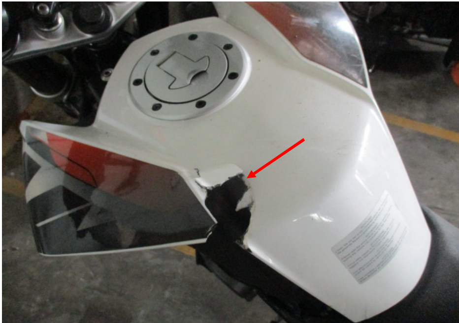
Photo 8 shows a closer view of the cracked fuel tank cover (arrowed) of the Motorcycle as a result of the accident.
