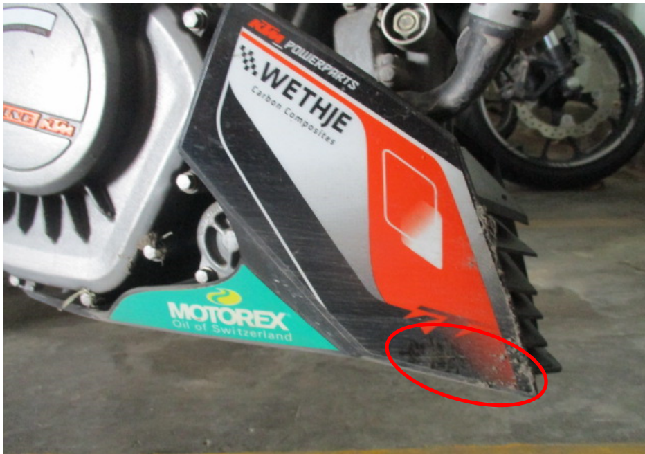
Photo 9 shows a closer view of the belly pan (circled) which was amongst the body parts of the Motorcycle that had sustained damage as a result of the accident.
