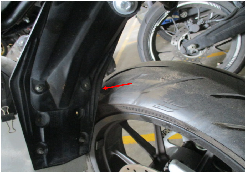
Photo 30 shows the deformed rear mudguard coming into contact with the rear tyre of the Motorcycle as a result of the accident (arrowed), rendering the Motorcycle immobile for the operational test.
