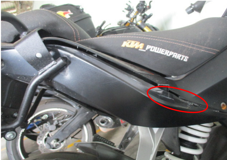
Photo 14 shows a closer view of the cracked right rear side cover (circled) of the Motorcycle as a result of the accident.
