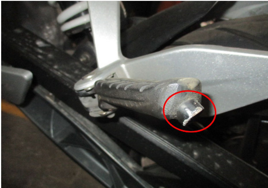
Photo 13 shows a closer view of the broken left pillion foot peg of the Motorcycle (circled) as a result of the accident.
