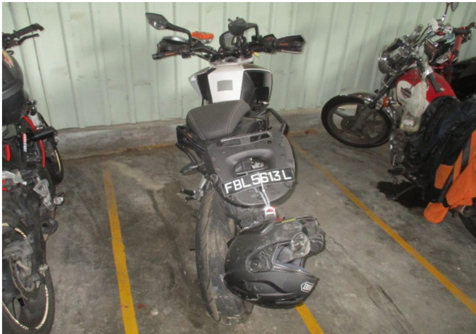
Photo 5 shows a general view of the rear portion of the Motorcycle at the time of our inspection. The Motorcycle was observed to have sustained damages all around. Amongst the body parts that were found to have been damaged include its headlight assembly, head cowl, fuel tank cover, belly pan, rear brake pedal, right front footrest, left pillion foot peg, right rear side cover, top box rack and rear mudguard, amongst others.
