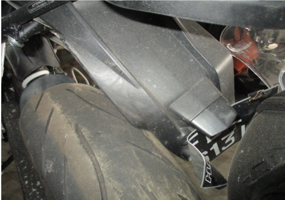
Photo 12 shows a closer view of the deformed rear mudguard and dented rear number plate of the Motorcycle as a result of the accident.
