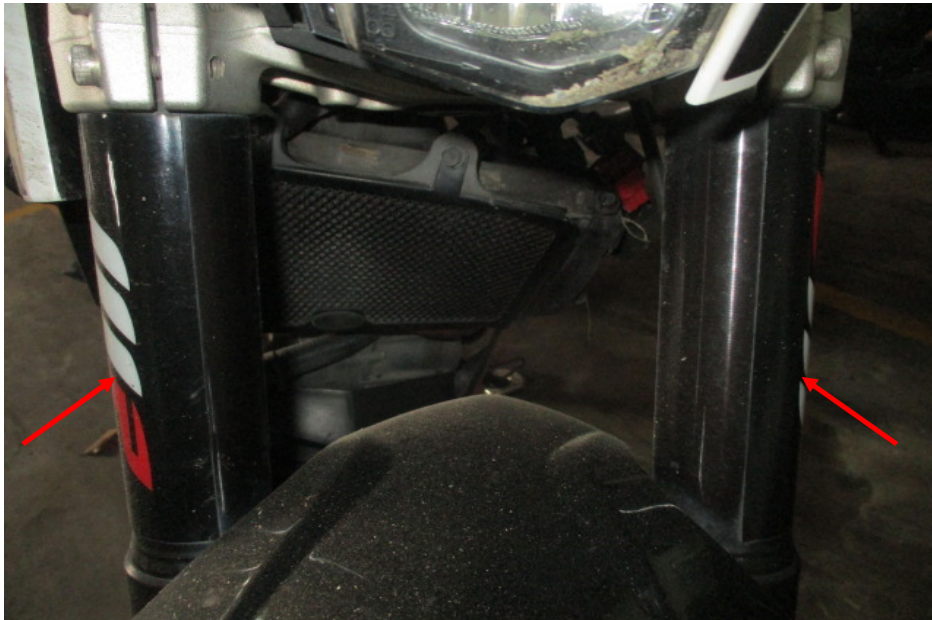
Photo 22 shows the front fork (arrowed) of the Motorcycle. The front fork and fork bracket of the Motorcycle were both found to be intact and undamaged. Turning the Motorcycle's handle bar towards the left and right did not produce any abnormal free play and/or resistance. The steering system of the Motorcycle was in serviceable condition at the time of our inspection.
