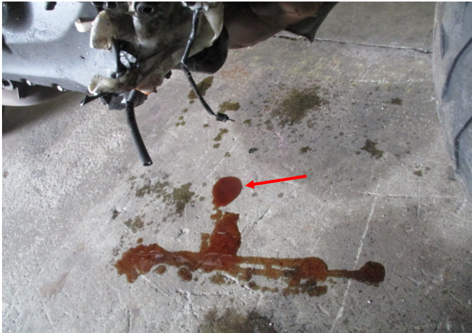
Photo 22 shows wet fluid stains observed on the ground directly below the engine cover of the Motorcycle (arrowed), indicating that a fluid leak had occurred as a result of the accident.
