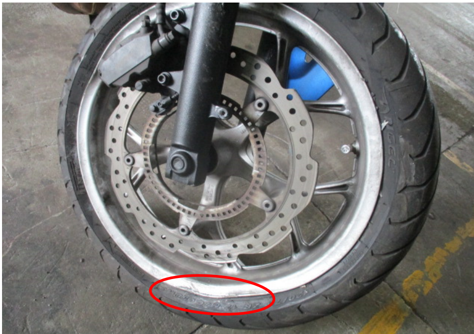
Photo 18 shows the front wheel rim of the Motorcycle at the time of our inspection. Some relatively minor marks of grazing nature were observed on the edges of the front wheel rim (circled), at the right side of the Motorcycle.
