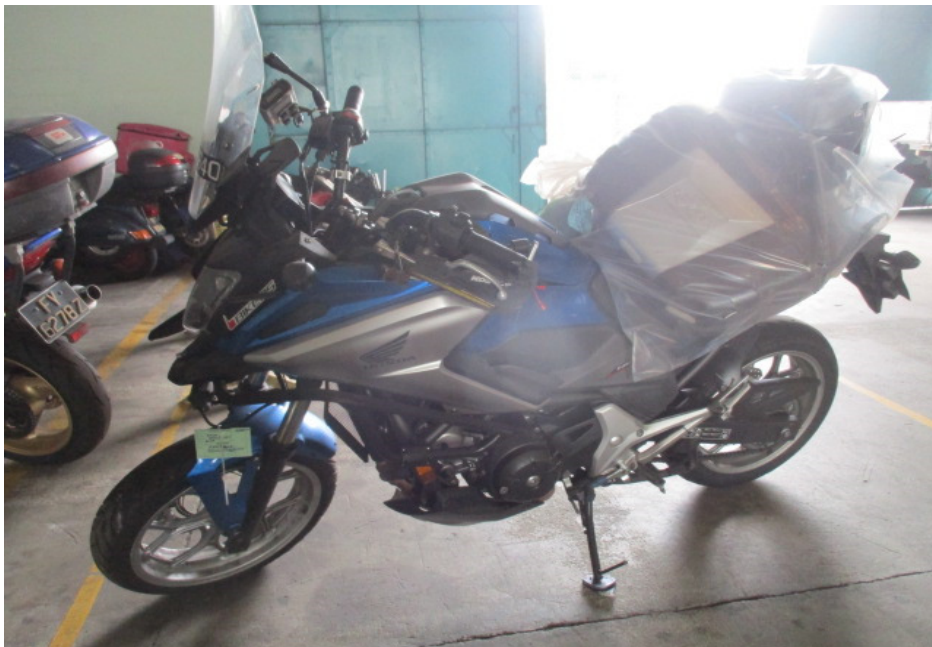
Photo 4 shows a general view of the left body of the Motorcycle at the time of our inspection. The Motorcycle was observed to have sustained damages all around. Amongst the body parts that were found to have been damaged include its headlight assembly, side covers, handlebar ends, front cowling, front mudguard, engine crash bars, handlebar ends, front brake lever, clutch lever, clutch lever guard, side stand enlarger, fuel tank cover, rear brake pedal, right front footrest, exhaust muffler and exhaust muffler slider, amongst others.
