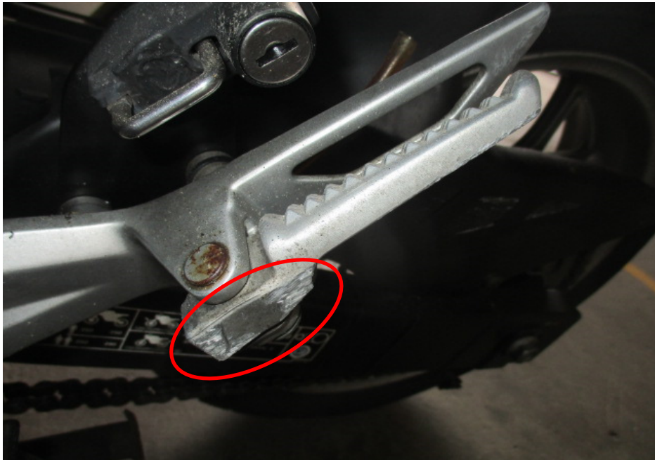
Photo 11 shows a closer view of the left pillion foot peg (circled) which was amongst the body parts of the Motorcycle that had sustained damage as a result of the accident.
