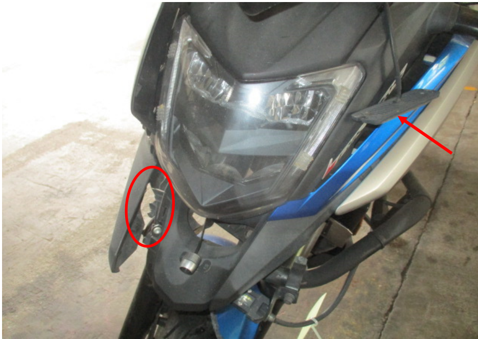
Photo 5 shows a closer view of the damaged headlight assembly (arrowed) and front cowling (circled) of the Motorcycle as a result of the accident.
