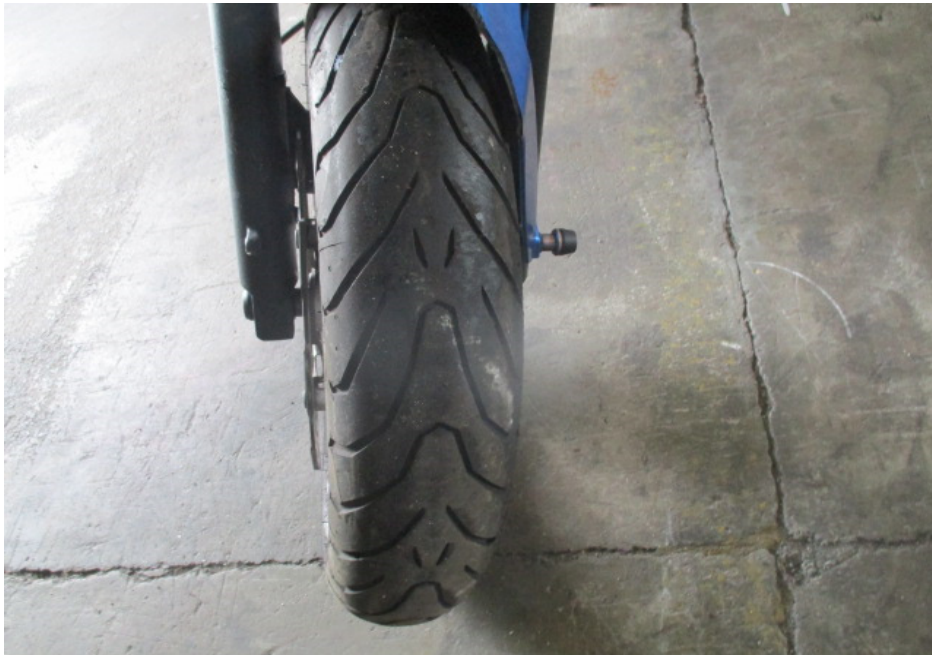
Photo 17 shows the condition of the Motorcycle's front tyre. The front tyre was observed to be in serviceable condition with remaining tread depth of approximately 3mm. There was no tear, burst mark(s) and/or punctured hole(s) on the sidewalls as well as across the tread of the front tyre.
