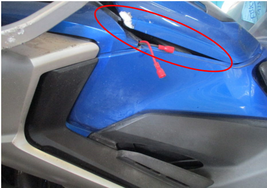
Photo 12 shows the damaged fuel tank cover Motorcycle as a result of the accident (circled).
