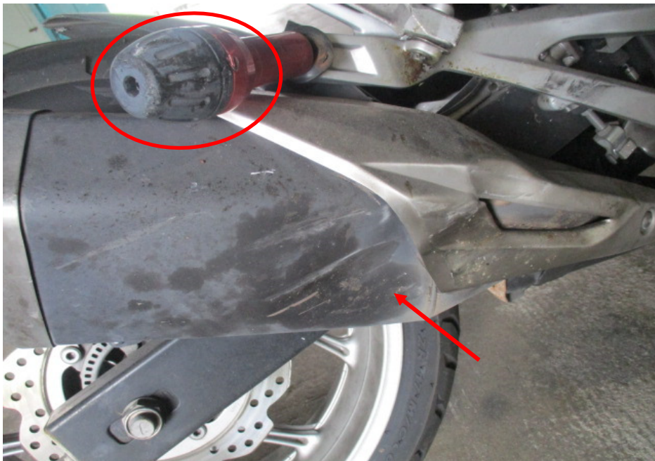
Photo 16 shows a closer view of the bent exhaust muffler slider (circled) and the damaged exhaust muffler (arrowed) which were amongst the body parts of the Motorcycle that had sustained damage as a result of the accident.
