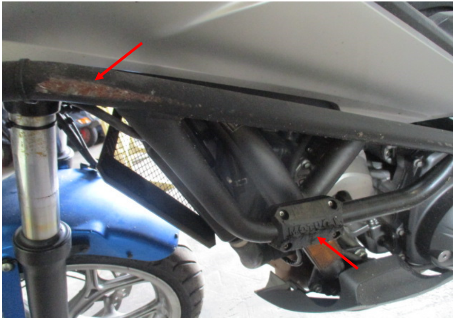
Photo 14 shows a closer view of the left crash bar of the Motorcycle that had sustained damages of grazing nature as a result of the accident (arrowed).
