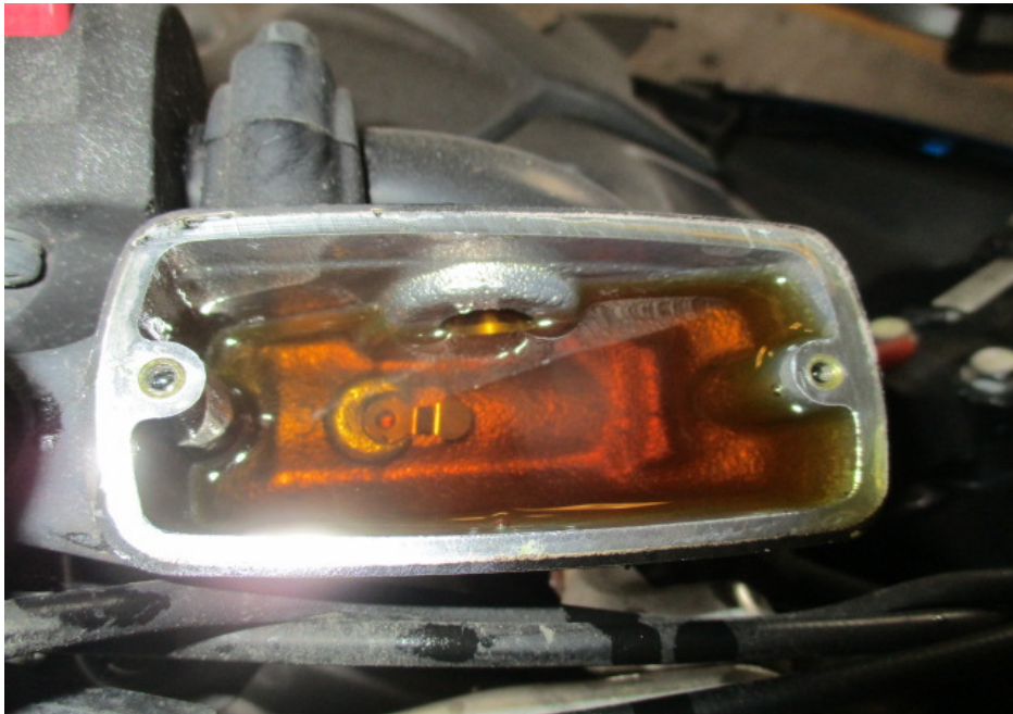
Photo 27 shows the brake fluid reservoir for the front brake of the Motorcycle. The brake fluid was observed to be of sufficient level and without contamination for operational purposes.
