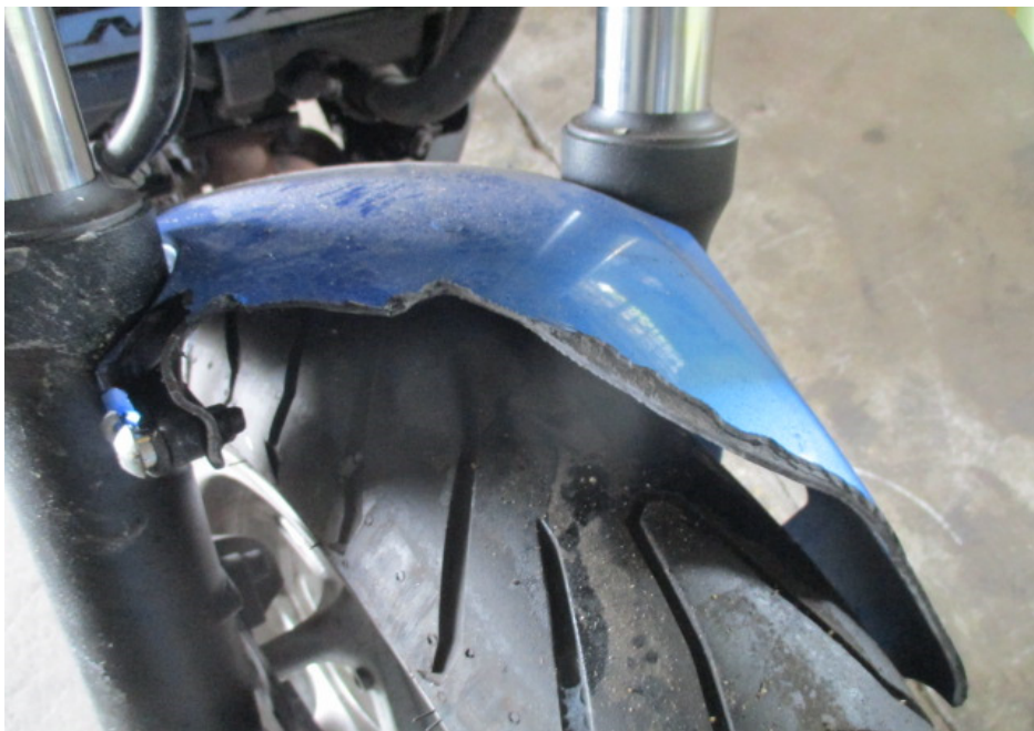
Photo 6 shows a close up view of the cracked front mudguard of the Motorcycle as a result of the accident.
