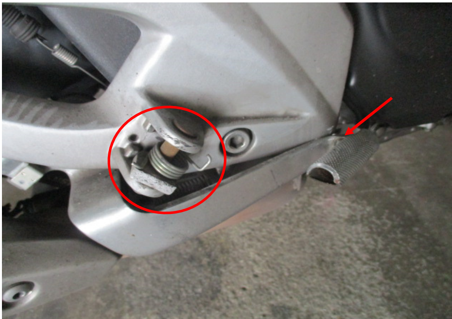
Photo 10 shows a closer view of the bent rear brake pedal (arrowed) and broken right front footrest (circled) which were amongst the body parts of the Motorcycle that had sustained damage as a result of the accident.
