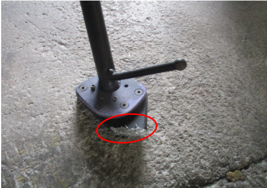
Photo 9 shows a closer view of the side stand enlarger of the Motorcycle which sustained damages of grazing nature as a result of the accident (circled).
