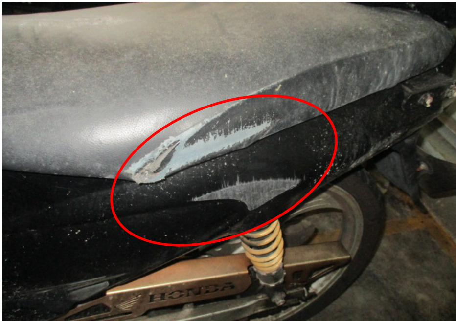
Photo 10 shows a closer view of the seat and left rear side cover, which was amongst the body parts of the Motorcycle that had sustained damages of grazing nature as a result of the accident
