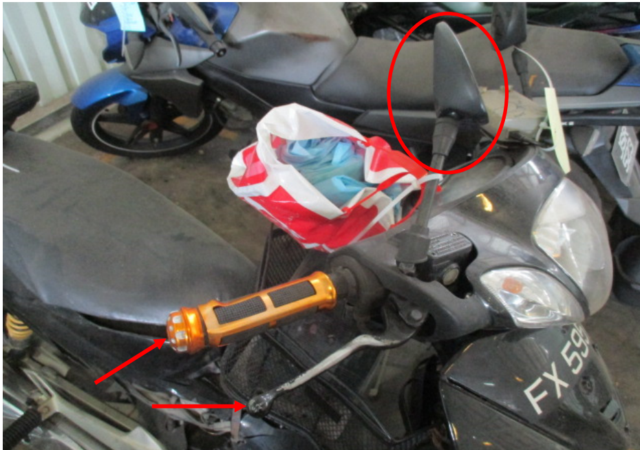
Photo 8 shows a close up view of the right handlebar end and front brake lever (arrowed) as well as the right side mirror (circled) of the Motorcycle. These parts were amongst the body parts of the Motorcycle which were damaged as a result of the accident.
