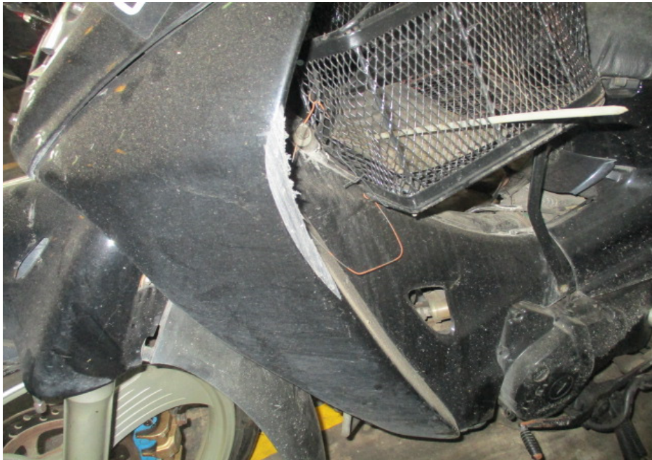
Photo 5 shows the general view of the left cowling of the Motorcycle which was amongst the body parts of the Motorcycle that had sustained damage as a result of the accident.
