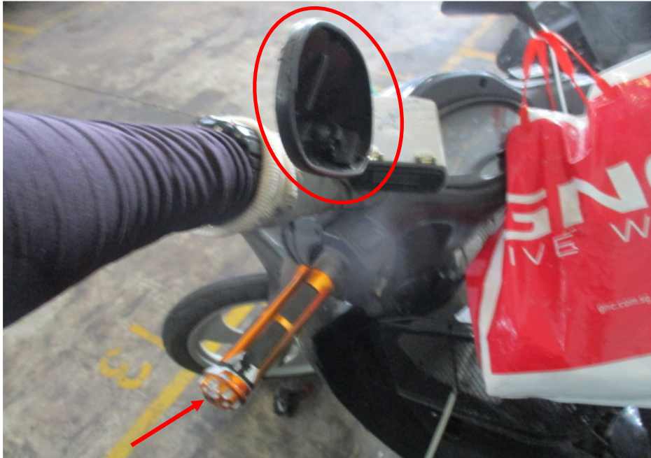
Photo 7 shows a close up view of the left handlebar end as well as the left side mirror (circled) of the Motorcycle. These parts were amongst the body parts of the Motorcycle which were damaged as a result of the accident.
