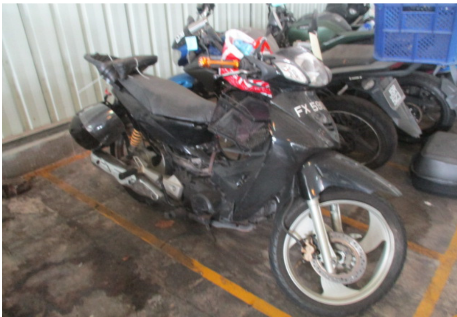
Photo 2 shows a general view of the right body of the Motorcycle at the time of our inspection. Body parts that were found to have been damaged include its front wheel, front mudguard, side mirrors, handlebar ends, front brake lever, side cowlings, left rear side cover, rear brake pedal, gear shift pedal, left front footrest, right front footrest, seat, exhaust muffler and exhaust muffler heat shield, amongst others.
