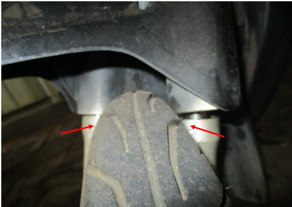
Photo 21 shows the front wheel of the Motorcycle. The front wheel (arrowed) was observed to be misaligned as a result of the accident. We were hence not able to conduct any tests on the steering system of the Motorcycle.
