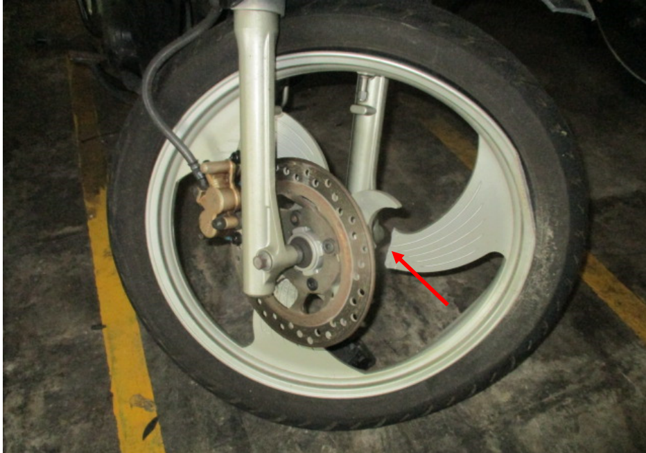
Photo 14 shows a closer view of the broken front wheel rim of the Motorcycle as a result of the accident (arrowed).
