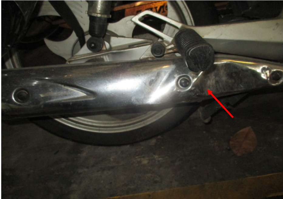
Photo 13 shows the dented exhaust muffler and exhaust muffler heat shield (arrowed) of the Motorcycle as a result of the accident.
