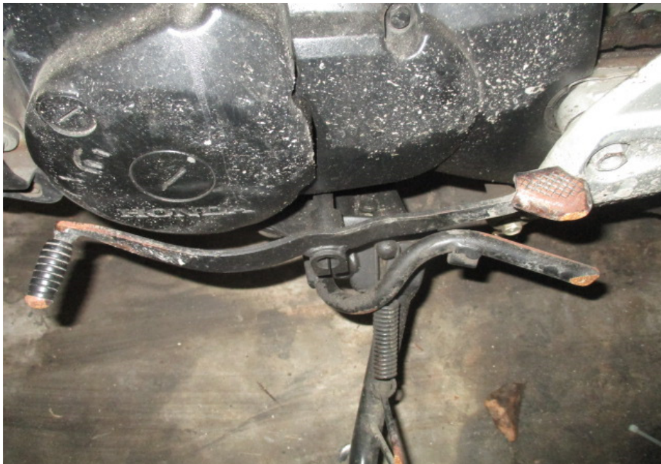
Photo 12 shows the damaged gear shift pedal and left front footrest which were amongst the body parts of the Motorcycle that had sustained damage as a result of the accident.
