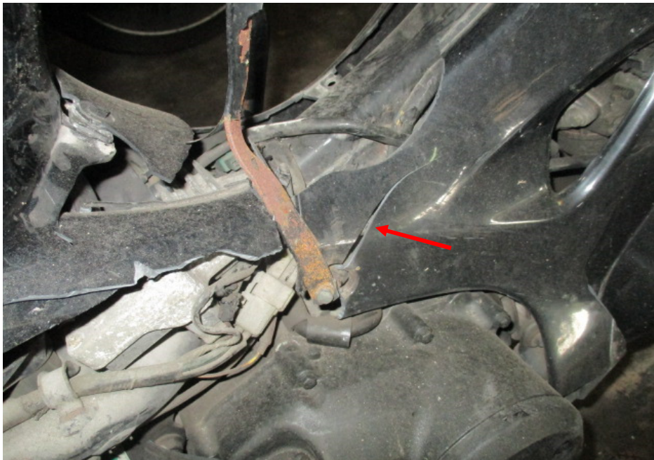
Photo 6 shows the cracked right side cover of the Motorcycle as a result of the accident (arrowed).
