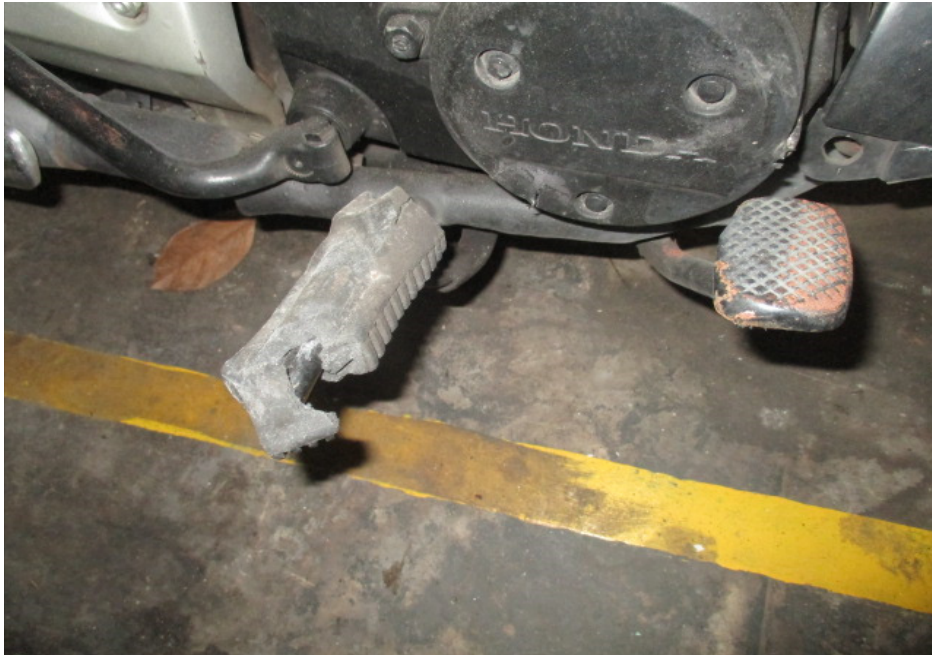
Photo 11 shows the damaged rear brake pedal and right front footrest which were amongst the body parts of the Motorcycle that had sustained damage as a result of the accident.
