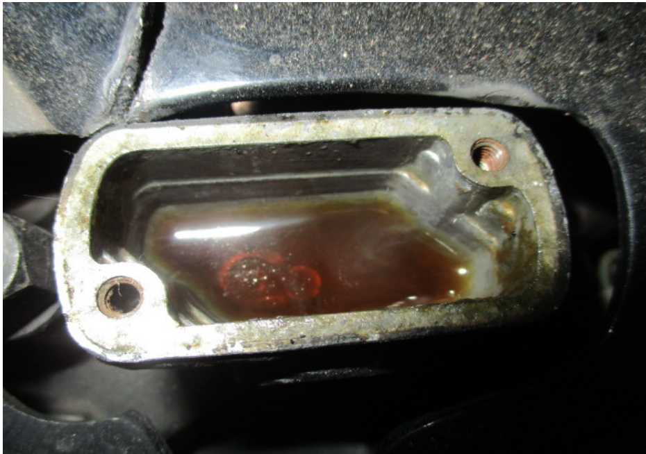
Photo 23 shows the brake fluid reservoir for the front brake of the Motorcycle. The brake fluid was observed to be of sufficient level for operational purposes and without contamination for.
