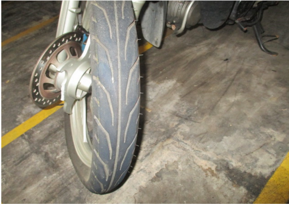
Photo 15 shows the condition of the Motorcycle's front tyre. The front tyre was observed to be in serviceable condition with remaining tread depth of approximately 4mm. The tyre was also observed to be sufficiently inflated for vehicular operation. We did not observe any tear, burst mark(s) and/or punctured hole(s) on the sidewalls as well as across the tread of the front tyre.
