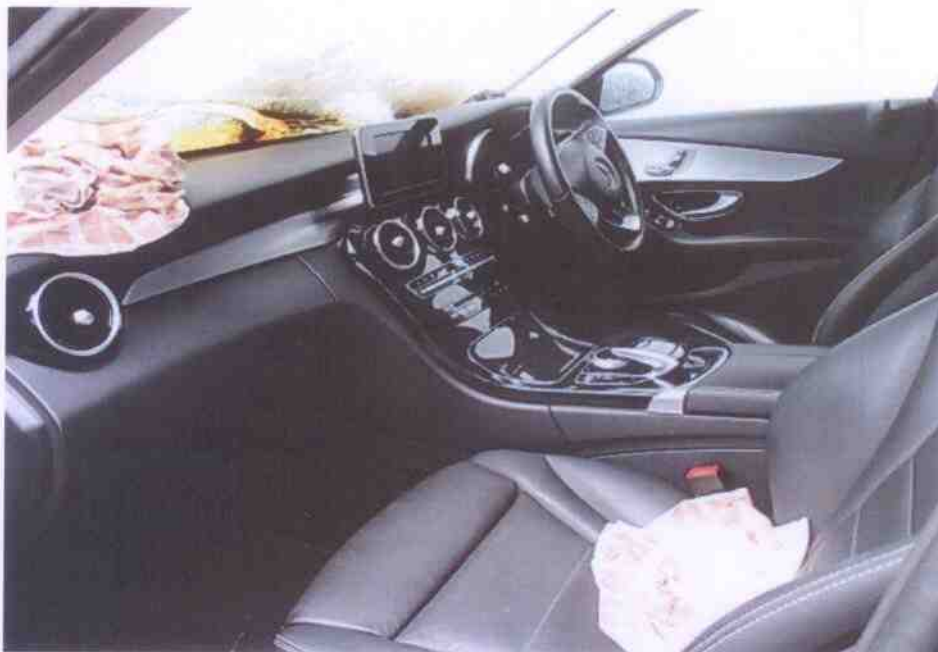
Photo 6 shows the interior compartment of the Insured Vehicle, which was observed to be relatively unaffected by the fire.
