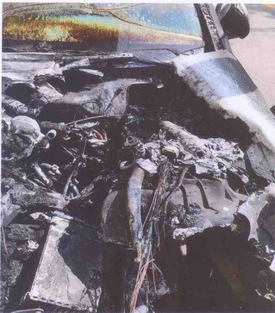
Photo 15 shows the Insured Vehicle at the incident scene after the fire was extinguished. In general, the information that could be gathered from this photograph had corresponded to the events that were related to us by Ms Florence. The extent of damage indicates that the fire had started in the left portion of the engine compartment.
