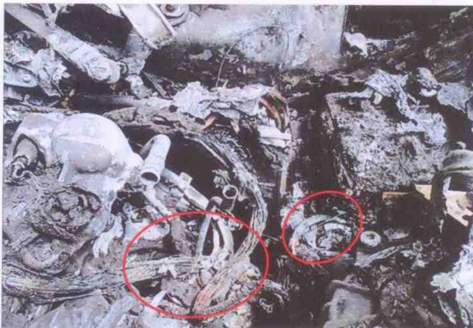
Photo 11 shows a closer view of the burnt wirings around the left portion of the engine compartment, which is in the immediate vicinity where the fire to the Insured Vehicle had likely started. We noticed greenish residue on several stretches of burnt wirings (circled). The presence of greenish residue indicates internal heating of copper wires, a sign of an electrical short circuit occurring. The greenish residue is normally left behind from oxidation as a result of chemical reaction involving the copper wires.
