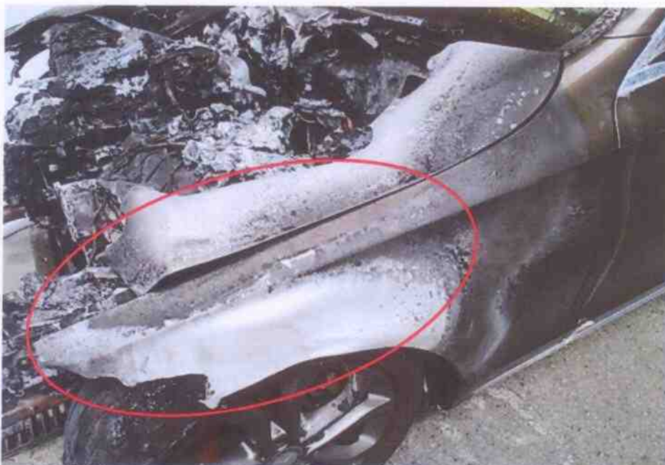
Photo 9 shows the whitish burn marks that were found on the left front fender of the Insured Vehicle (circled). Such whitish burn marks are a result of exposure to prolonged heat intensity, which may indicate where the fire had started. Rust would also begin to develop on these areas soon after the fire.
