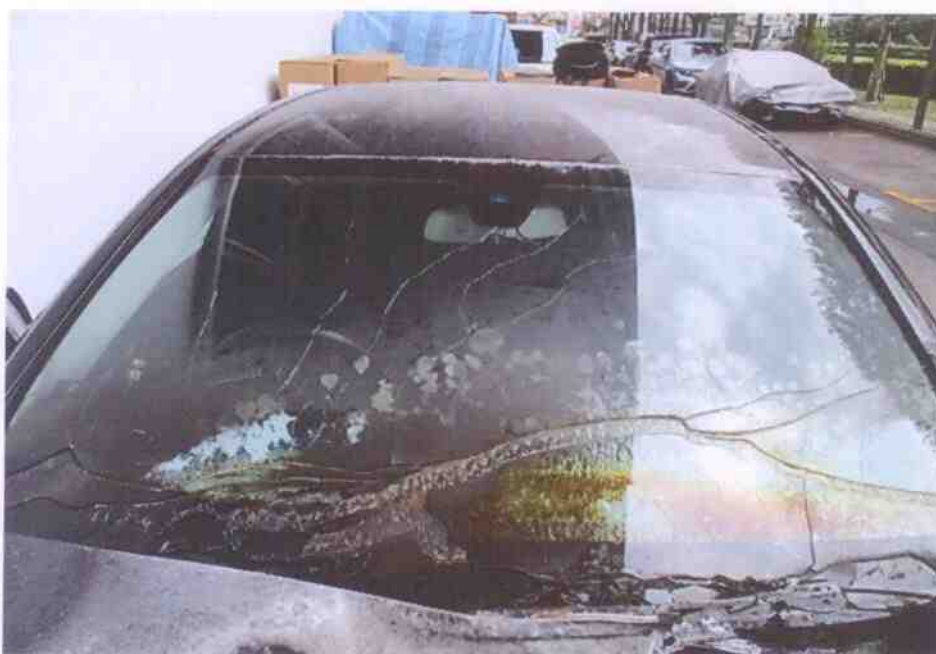
Photo 4 shows a closer view of the front windscreen of the Insured Vehicle at the time of our inspection. The front windscreen had sustained extensive fire damage.
