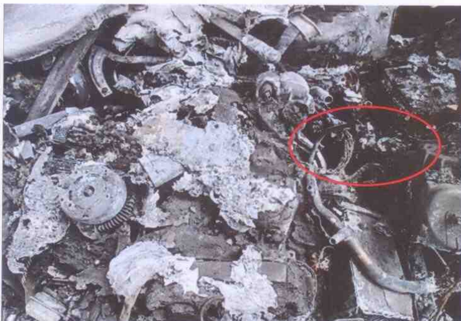
Photo 10 shows the burnt wirings around the left portion of the engine compartment (circled), which is in the immediate vicinity where the fire to the Insured Vehicle had likely started.
