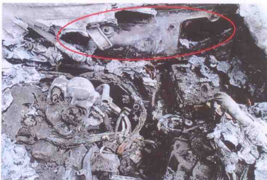
Photo 8 shows a closer view of the rust that had developed on the left rear portion of the engine compartment (circled). The development of rust is an indication that this area was subjected to prolonged exposure to high heat intensity, which had caused the steel/metal material of the front bonnet to be exposed to natural environmental condition. Hence the fire to the Insured Vehicle can be determined to have originated towards the left portion of the engine compartment.
