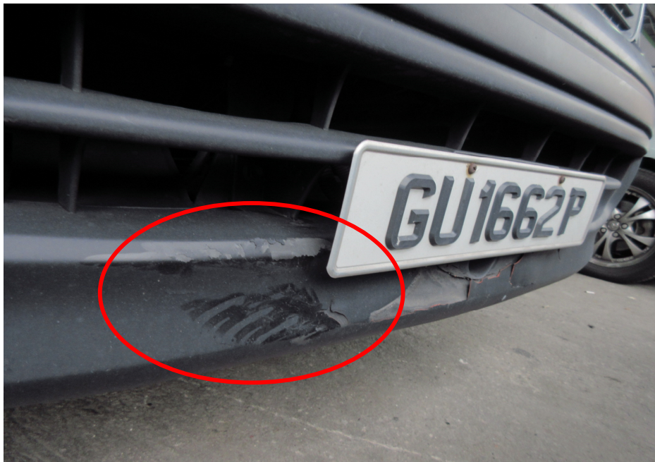
Photo 13 shows a closer view of the damage at the lower part of the Motor Van's front bumper (circled), at or below the area where its front number plate was fixed on. The part(s) at the entire front portion of the Motor Van above this area did not sustain any damage. The Motor Van had sustained a single area of damage at its front portion.
