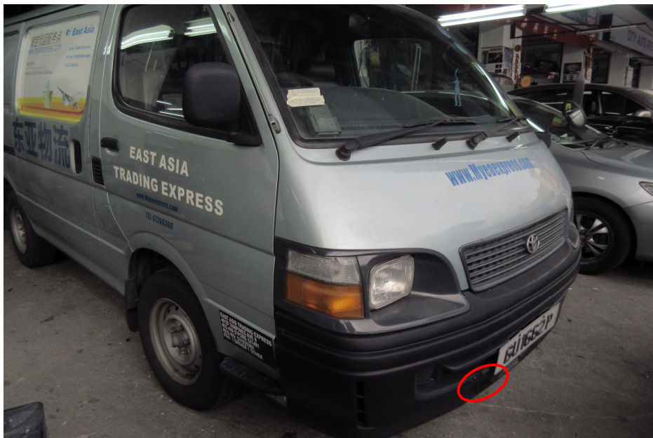
Photo 12 shows the front portion of the Motor Van. From the photographs showing the Motor Van prior to any repairs, I had observed damage at the lower part of its front bumper (circled), at or below the area where its front number plate was fixed on. There was no damage observed to the part(s) at the entire front portion of the Motor Van above the front number plate.
