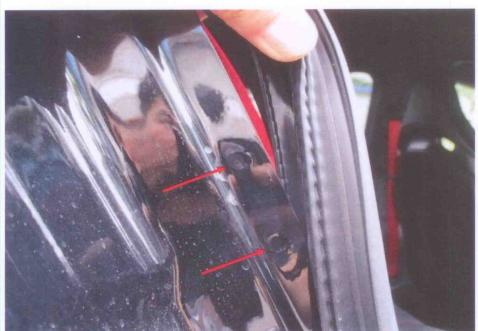
Photo 17 shows the right "C" pillar of the Motor Car. I did not find any weld marks other than original spot weld marks (arrowed) on the non-detachable body panels of the Motor Car, indicating that there was no re-welding works carried out; and that the non-detachable body panels of the Motor Car were originally fitted.
