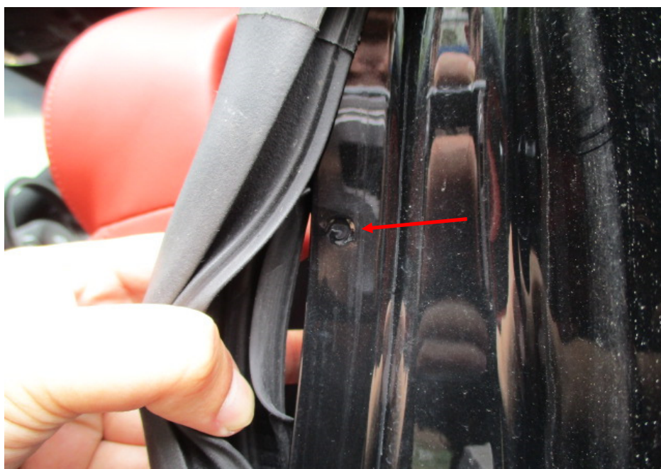
Photo 16 shows the rear left body panel of the Motor Car. I did not find any weld marks other than original spot weld marks (arrowed) on the non-detachable body panels of the Motor Car, indicating that there was no re-welding works carried out; and that the non-detachable body panels of the Motor Car were originally fitted.
