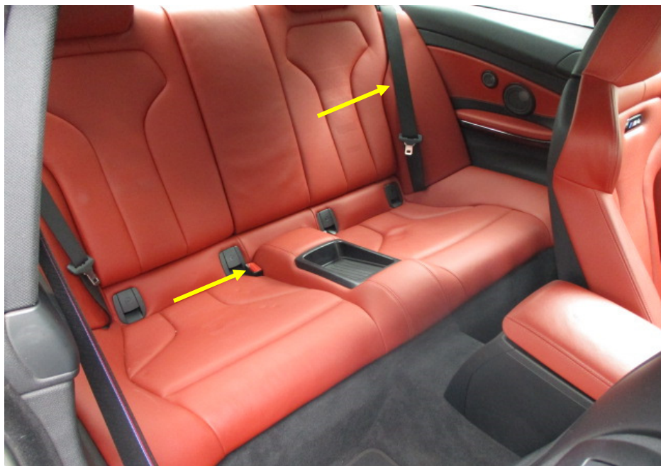
Photo 5 shows the rear seats of the Motor Car. All the seats of the Motor Car were secured via seat rails to the floor board. They were also fitted with a retractable seat belt reel and a pre-tensioner (arrowed). The seat belts were checked and able to be fastened securely to the respective pretension that was fitted on the side of each individual seat.
