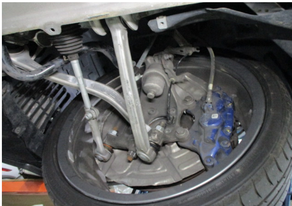
Photo 11 shows the various undercarriage components at the front right wheel of the Motor Car. The mechanical components, control arms and linkages were all found to be intact and secured in an appropriate manner. All of the Motor Car's undercarriage components were observed to be intact and secured in an appropriate manner.
