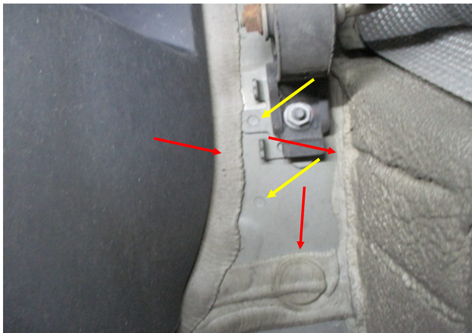
Photo 13 shows the chassis/structural body at the underside rear left of the Motor Car. Visually, I did not find any weld marks other than original spot weld marks (yellow arrow) on the chassis/structural body of the Motor Car. The original factory sealant (red arrow) at the joints along the chassis/structural body was also untouched, indicating no work was done on the chassis/structural body of the Motor Car and that the chassis/structural body was originally fitted.
