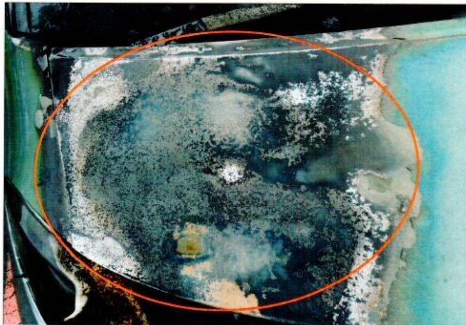
Photo 19 shows the exterior front bonnet of the Insured Vehicle, which is situated above the burnt headlamp at the time of our inspection. Due to heat rises, the prolonged high heat intensity confined to this area caused high heat intensity burn marks (whitish burn marks) and rust development on the surface of the metal bonnet of the Insured Vehicle. (circled).
