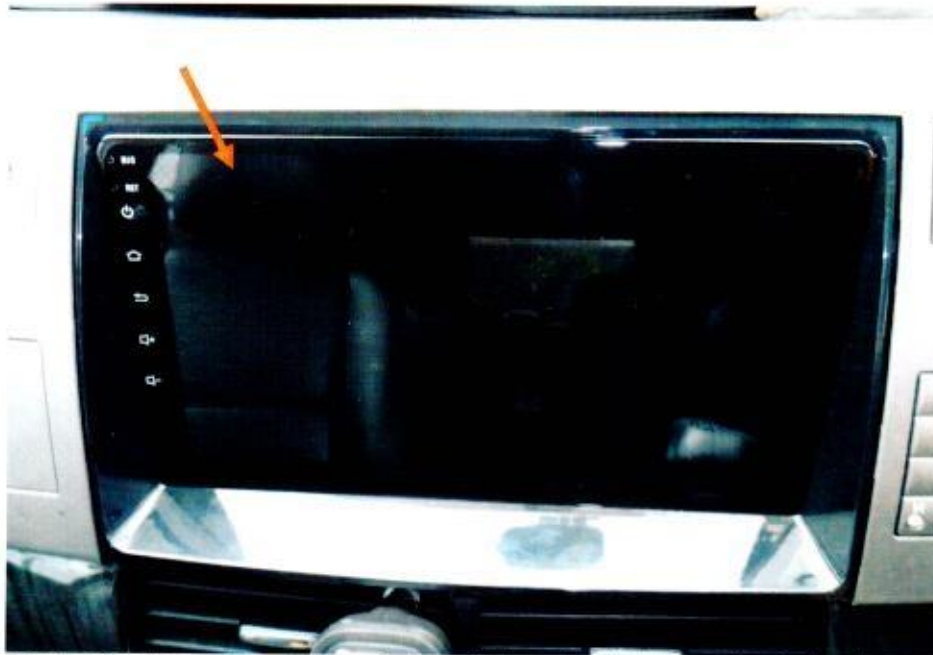
Photo 13 shows the aftermarket audio head unit (arrowed) of the Insured Vehicle, which was observed to be unaffected by the fire.
