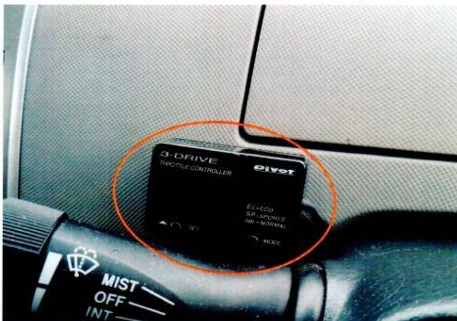
Photo 16 shows aftermarket electronic throttle pedal controller unit of the Insured Vehicle, which was observed to be unaffected by the fire.
