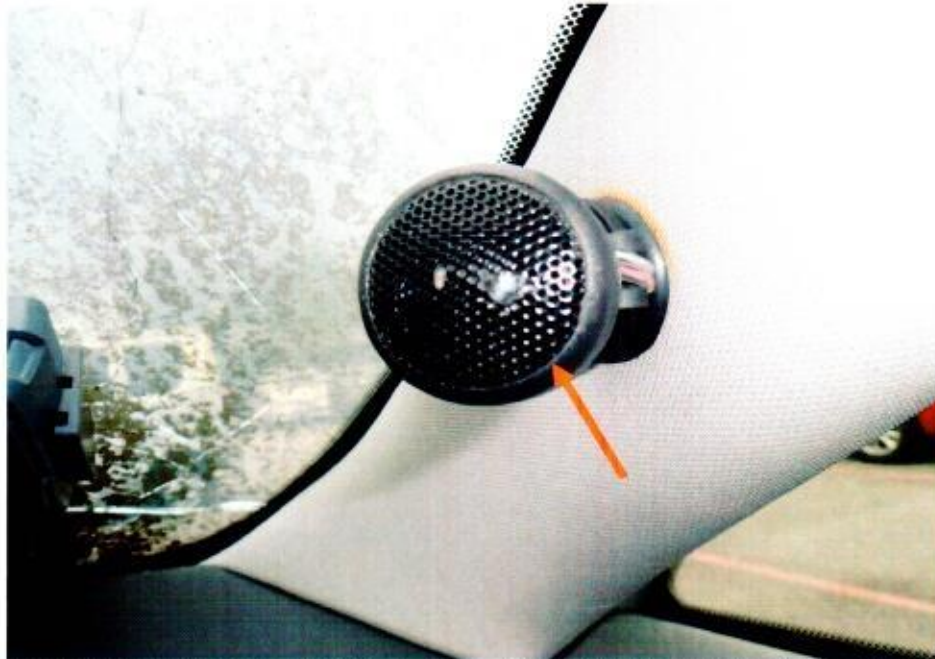
Photo 15 shows pair of audio tweeter (right side) (arrowed) of the Insured Vehicle, which was observed to be unaffected by the fire.
