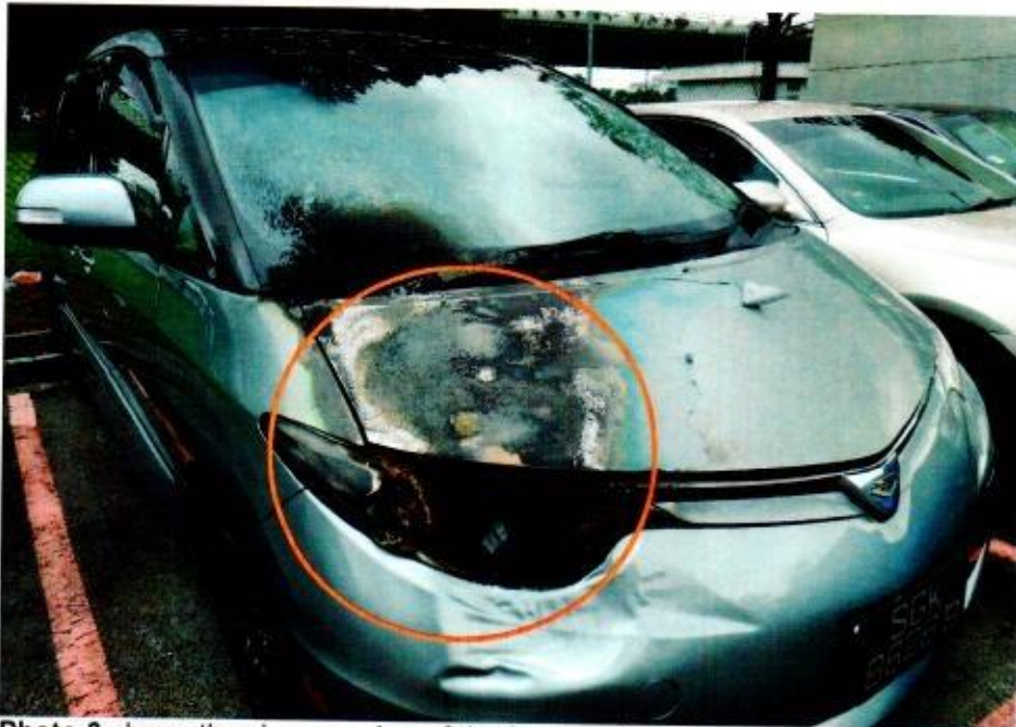
Photo 3 shows the close-up view of the front portion of the Insured Vehicle at the time of our inspection. The fire damage to the Insured Vehicle was confined to its front right portion. As observed whitish burn marks (circled) on the surface are a result of exposure to prolonged heat intensity as a result of the fire.
