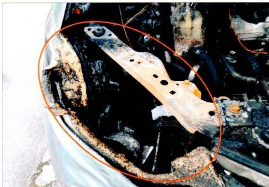
Photo 21 shows a general view of the front right headlamp assembly (circled) and the various surrounding components. The headlamp assembly and various components was observed to be melted from the high heat intensity. Rust development was also observed on the metal brackets of the Insured Vehicle.
