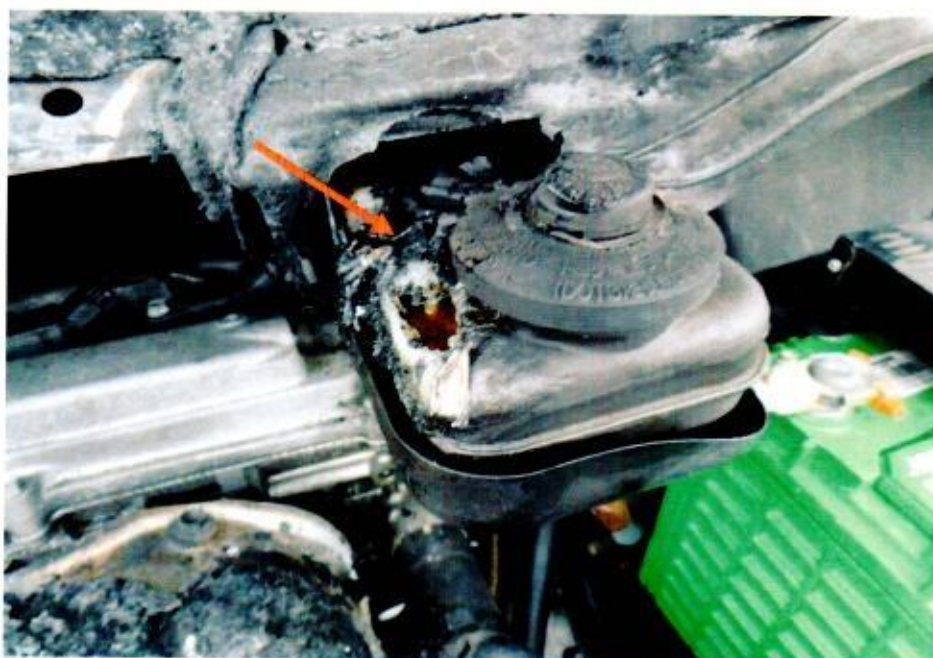
Photo 6 shows the close-up view of the front engine compartment portion of the Insured Vehicle at the time of our inspection. Its brake fluid reservoir (arrowed) was damaged as a result of the fire.
