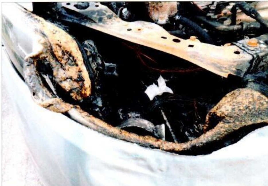
Photo 22 shows general view of the wirings leading from the halogen light bulb to the fuse box. Both the halogen light bulb and fuse box were factory fitted. The presence of greenish residue indicates internal heating of copper wires, a sign of an electrical short circuit occurring. The greenish residue is normally left behind from oxidation as a result of chemical reaction involving the copper wires.
