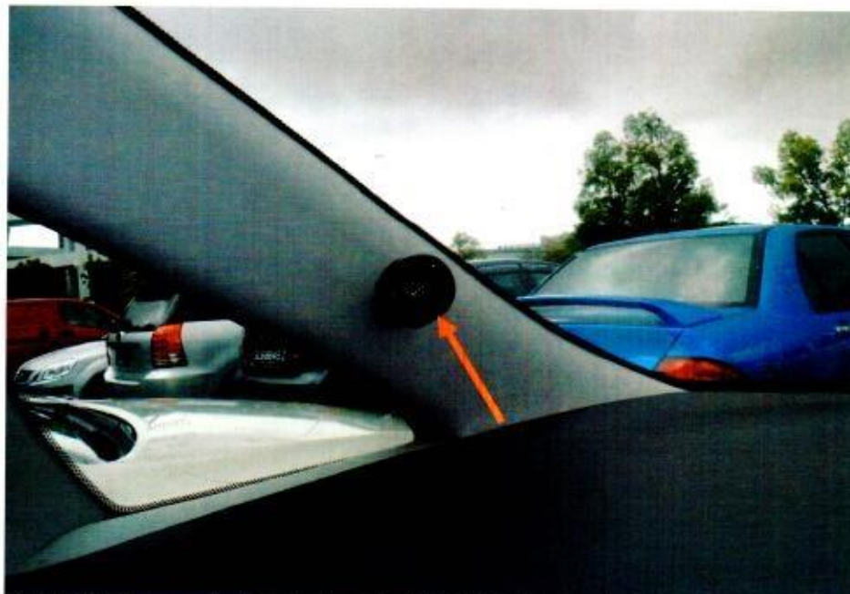
Photo 14 shows pair of audio tweeter (left side) (arrowed) of the Insured Vehicle, which was observed to be unaffected by the fire.
