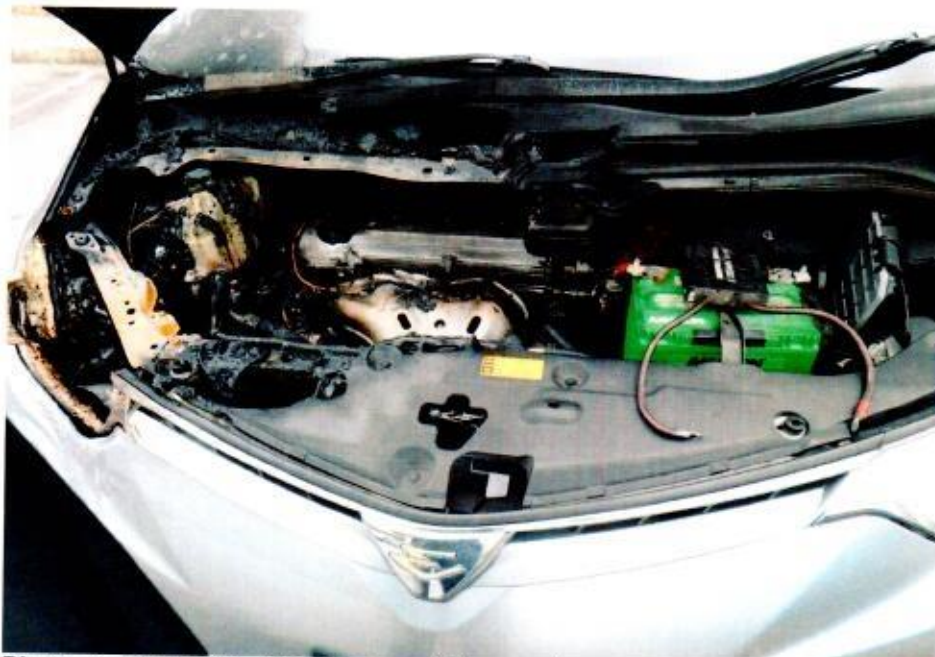
Photo 4 shows the general view of the engine compartment of the Insured Vehicle at the time of our inspection. The fire damage to the Insured Vehicle was confined to its front right portion. Its front windscreen, right headlamp, bonnet, bumper and several parts inside the engine compartment were also observed to sustain heat damage. These includes the timing cover, fuse box, coolant fluid reservoir, brake fluid reservoir and its factory wiring harness, are amongst the body parts that were found to have been affected as a result of the fire.
