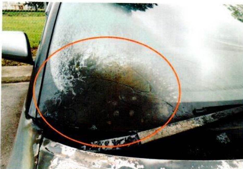
Photo 2 shows the close-up view of the front portion of the Insured Vehicle at the time of our inspection. The fire damage to the Insured Vehicle was confined to its front right portion. As observed its front windscreen (circled) had suffered heat and smoke damage as a result of the fire.
