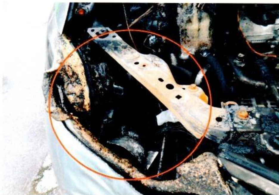
Photo 8 shows the close-up view of the front right head lamp portion of the Insured Vehicle at the time of our inspection. The whole of the head lamp including its housing and its factory wiring harness (circled) were damaged and melted down as a result of the fire.
