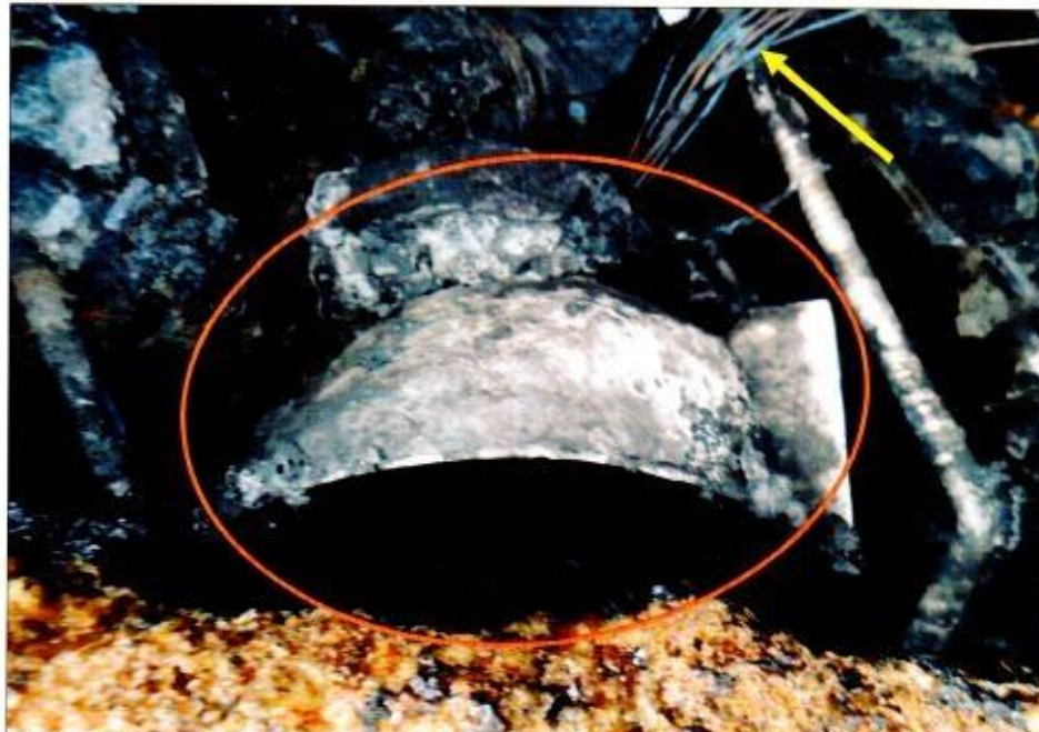
Photo 23 shows the close-up view of the headlamp. Observed was greenish residue on the wiring harness leading (arrowed) from the headlamp light bulb (circled). to the fuse box Observed was greenish residue on the wiring harness. The presence of greenish residue indicates internal heating of copper wires, a sign of an electrical short circuit occurring. The greenish residue is normally left behind from oxidation as a result of chemical reaction involving the copper wires.
