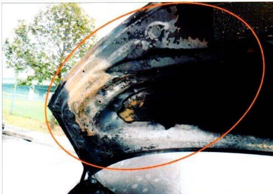
Photo 20 shows the interior front bonnet of the Insured Vehicle, which is situated above the burnt headlamp at the time of our inspection. Due to heat rises, the prolonged high heat intensity confined to this area caused high heat intensity burn marks (whitish burn marks) and rust development on the surface of the metal bonnet of the Insured Vehicle. Rust had also developed on the surface. (circled).
