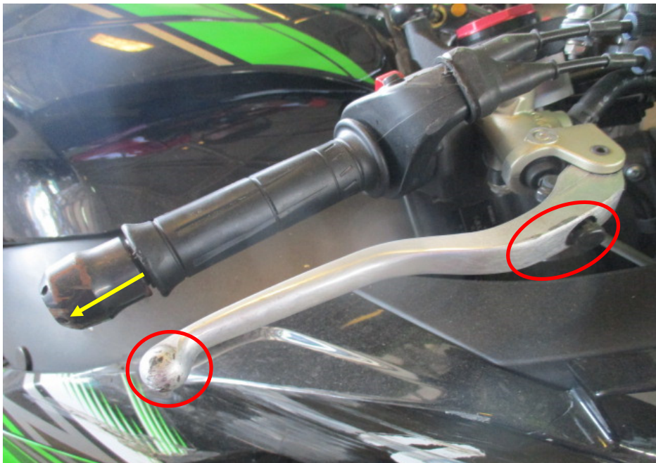
Photo 9 shows a closer view of the right handlebar end (yellow arrow) and front brake lever (circled) which were amongst the body parts of the Motorcycle that had sustained damage as a result of the accident.
