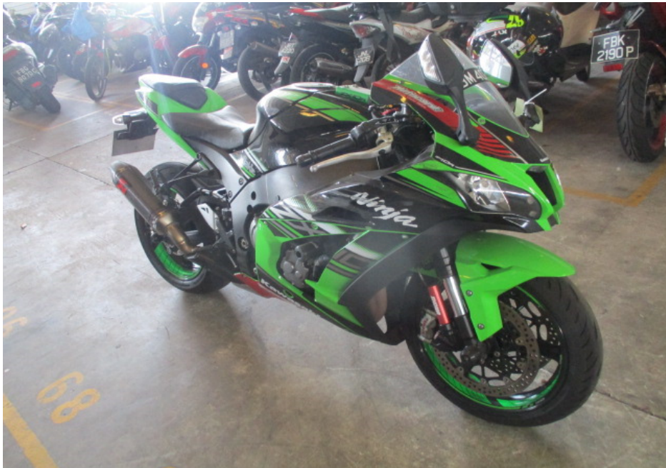
Photo 4 shows a general view of the right body of the Motorcycle at the time of our inspection. The Motorcycle was observed to have sustained damages at its frontal portion and right body. Amongst the body parts that were found to have been damaged include its headlight, head cowling, right cowling, right handlebar end, front brake lever, rear brake pedal, right front footrest, petrol tank, right frame and exhaust muffler, amongst others.
