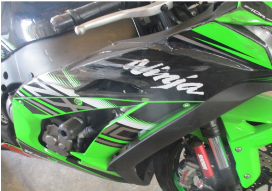
Photo 7 shows a closer view of the right cowl which was amongst the body parts at the front body of the Motorcycle that had sustained damage as a result of the accident.
