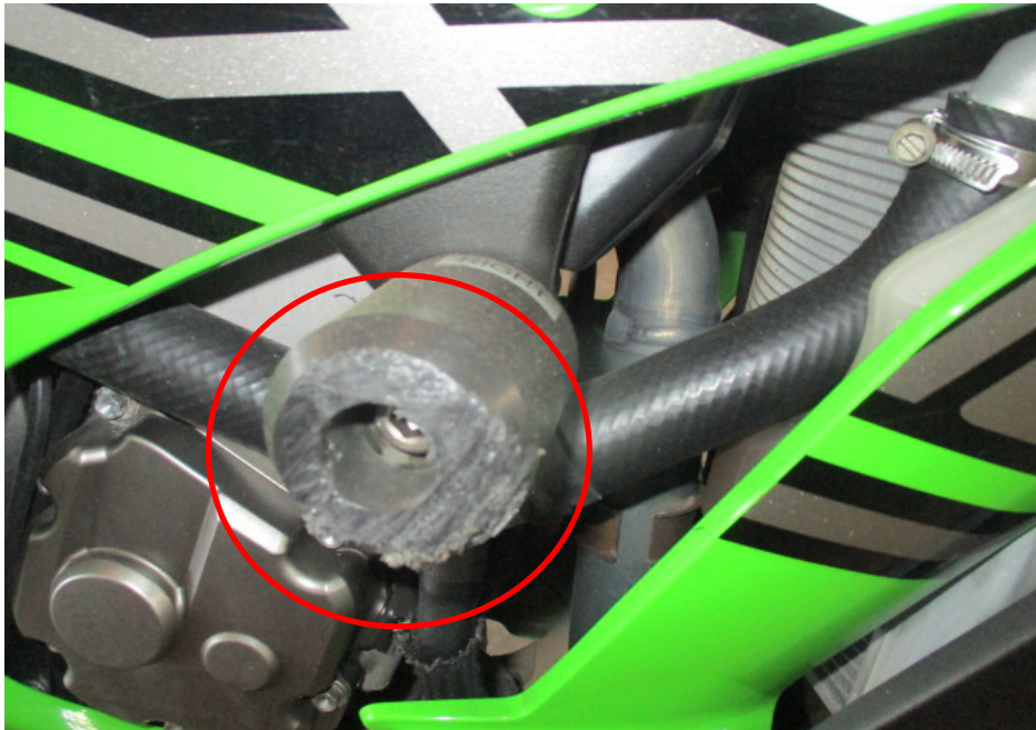
Photo 8 shows a closer view of the right frame slider of the Motorcycle that had sustained damages of grazing nature as a result of the accident (circled).
