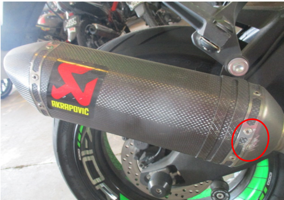
Photo 13 shows a closer view of the rear exhaust muffler of the Motorcycle that had sustained damages of grazing nature as a result of the accident (circled).
