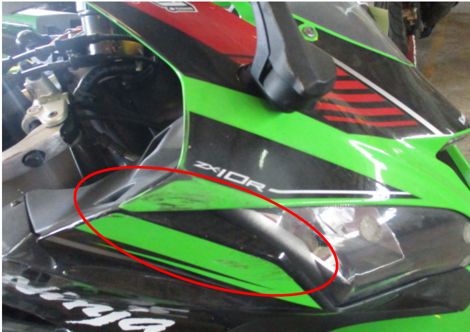
Photo 6 shows a closer view of the head cowl which was amongst the body parts at the front body of the Motorcycle that had sustained damage as a result of the accident (circled).
