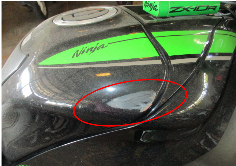
Photo 12 shows a closer view of the petrol tank which was amongst the body parts of the Motorcycle that had sustained damages of grazing nature as a result of the accident (circled).
