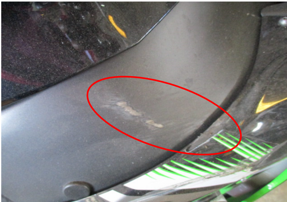
Photo 11 shows a closer view of the right frame which was amongst the body parts of the Motorcycle that had sustained damages of grazing nature as a result of the accident (circled).
