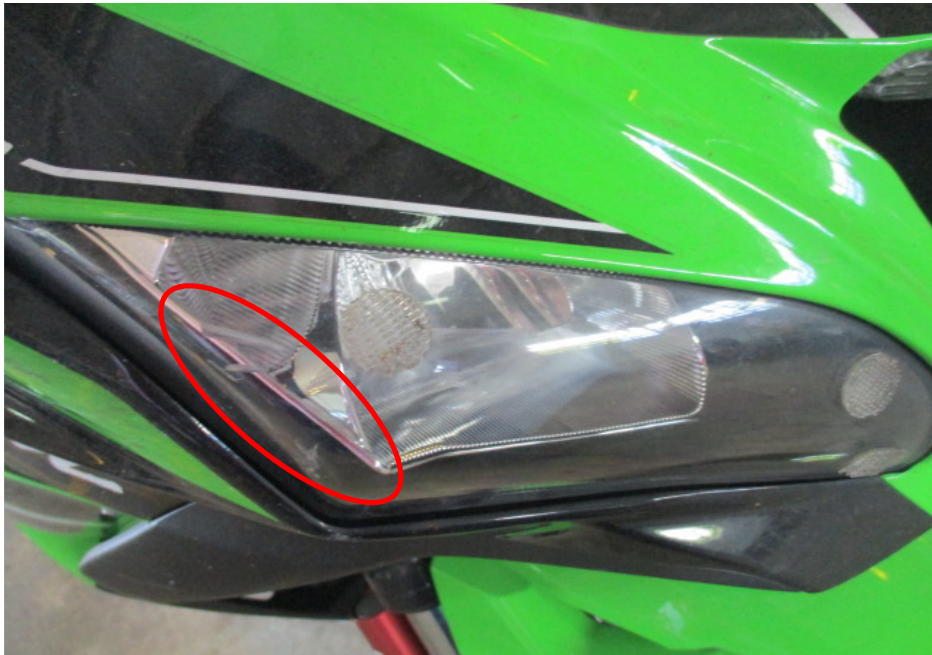
Photo 5 shows a close up view of the right front signal lamp which was amongst the body parts of the Motorcycle that had sustained damage as a result of the accident (circled).
