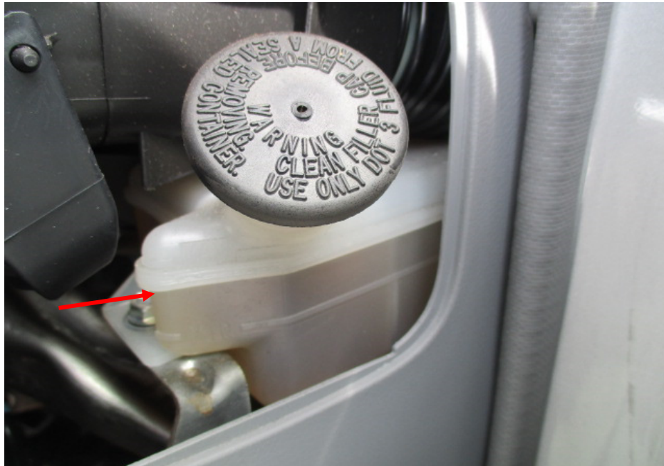
Photo 9 shows the brake fluid reservoir of the Motor Lorry at the time of our inspection. The brake fluid was observed to be of sufficient level and without any visible contamination (arrowed).
