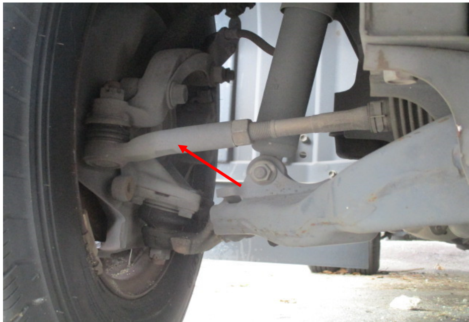
Photo 17 shows the various undercarriage components at the front right wheel of the Motor Lorry, in particular the steering tie rod end (arrowed). The various steering components were all found to be intact, suggesting that the steering system of the Motor Lorry was likely to be in serviceable condition at the material time of accident. There was also no sign of fluid stain(s) observed on the various undercarriage components.
