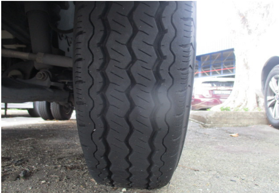
Photo 4 shows the condition of the front left tyre of the Motor Lorry, which was observed to be in serviceable condition with remaining tread depth of approximately 6mm. The tyre, which was wrapped around standard alloy wheel rim, was also observed to be sufficiently inflated for vehicular operation. There was no tear, cut or burst mark(s) on the outer and the inner sidewalls as well as across the tread of the 6 tyres that were fitted on the Motor Lorry.
