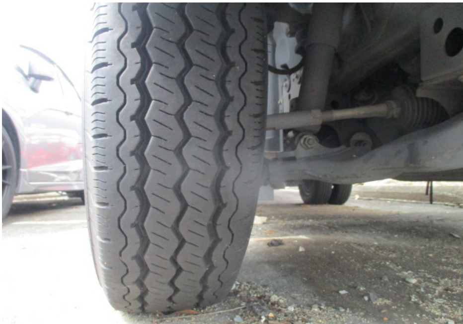
Photo 5 shows the condition of the front right tyre of the Motor Lorry, which was observed to be in serviceable condition with remaining tread depth of approximately 6mm. The tyre, which was wrapped around standard alloy wheel rim, was also observed to be sufficiently inflated for vehicular operation.
