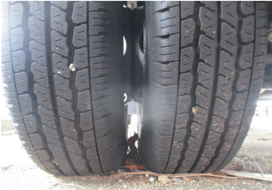
Photo 6 shows the condition of the rear left tyres of the Motor Lorry, which was observed to be in serviceable condition with remaining tread depth of approximately 6mm. The tyres, which were wrapped around standard alloy wheel rim, were also observed to be sufficiently inflated for vehicular operation. There was also no damage found on all 6 alloy wheel rims of the Motor Lorry.
