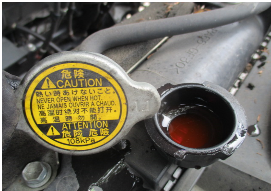
Photo 10 shows the engine coolant of the Motor Lorry at the time of our inspection. The engine coolant was observed to be of sufficient level and without any visible contamination.
