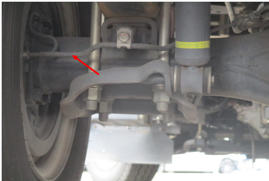
Photo 13 shows the brake pipe (arrowed) at the rear left wheel of the Motor Lorry. We did not observe any leakage of brake fluid at the time of our inspection of the Motor Lorry. Our static tests of the Motor Lorry's braking system, along with our visual examination of the various mechanical components in the braking system, had indicated that there was no internal leakage of pressure/vacuum. Hence the braking system of the Motor Lorry was likely to be in serviceable condition at the material time of accident.
