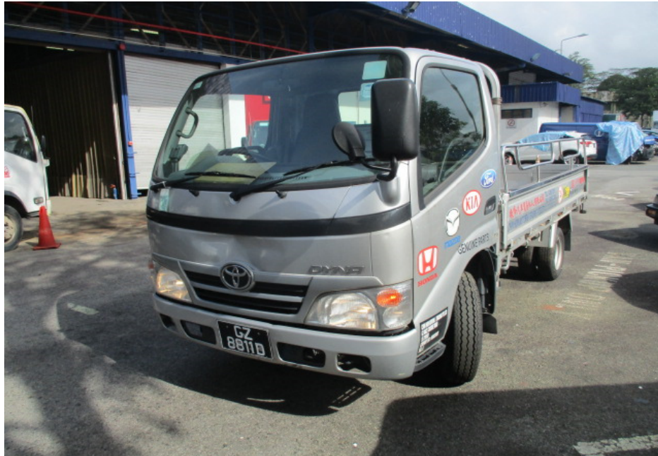
Photo 16 shows the front left wheel of the Motor Lorry turned to its full left. During our steering system test, we did not experience any abnormal free play and/or resistance when we had turned the steering wheel towards full left and full right. This would suggest that the steering system of the Motor Lorry was likely to be in serviceable condition at the material time of accident.
