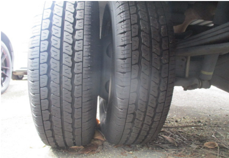
Photo 7 shows the condition of the rear right tyres of the Motor Lorry, which were observed to be in serviceable condition with remaining tread depth of approximately 6mm. There was also no tear, cut or burst mark(s) on the outer and the inner sidewalls as well as across the tread of the 6 tyres that were fitted on the Motor Lorry.
