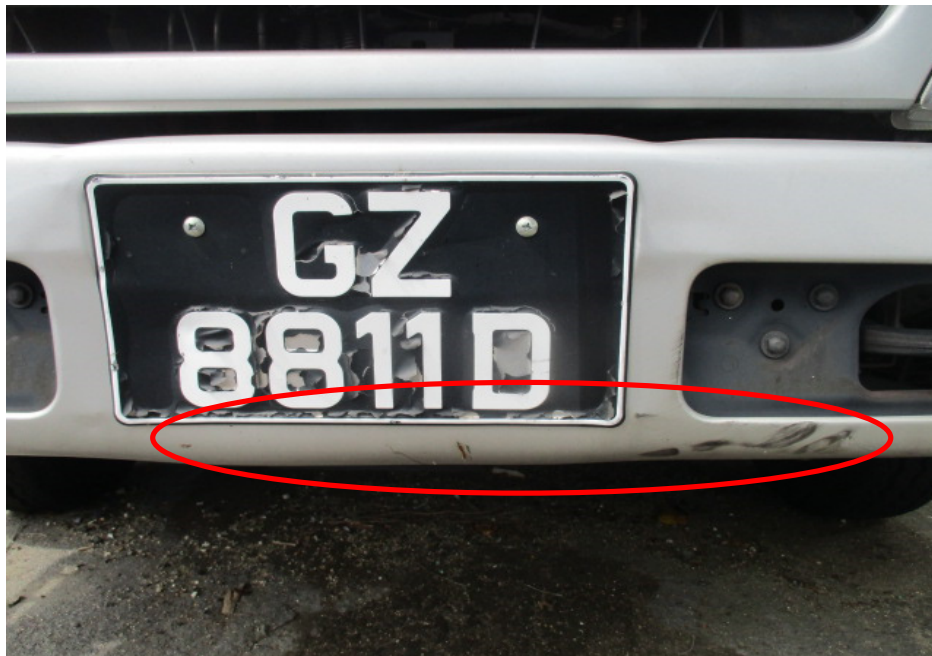
Photo 3 shows a closer view of the black marks observed on the front bumper (circled) of the Motor Lorry at the time of our inspection.
