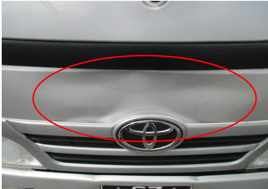
Photo 2 shows a closer view of the dented front panel (circled) of the Motor Lorry at the time of our inspection.
