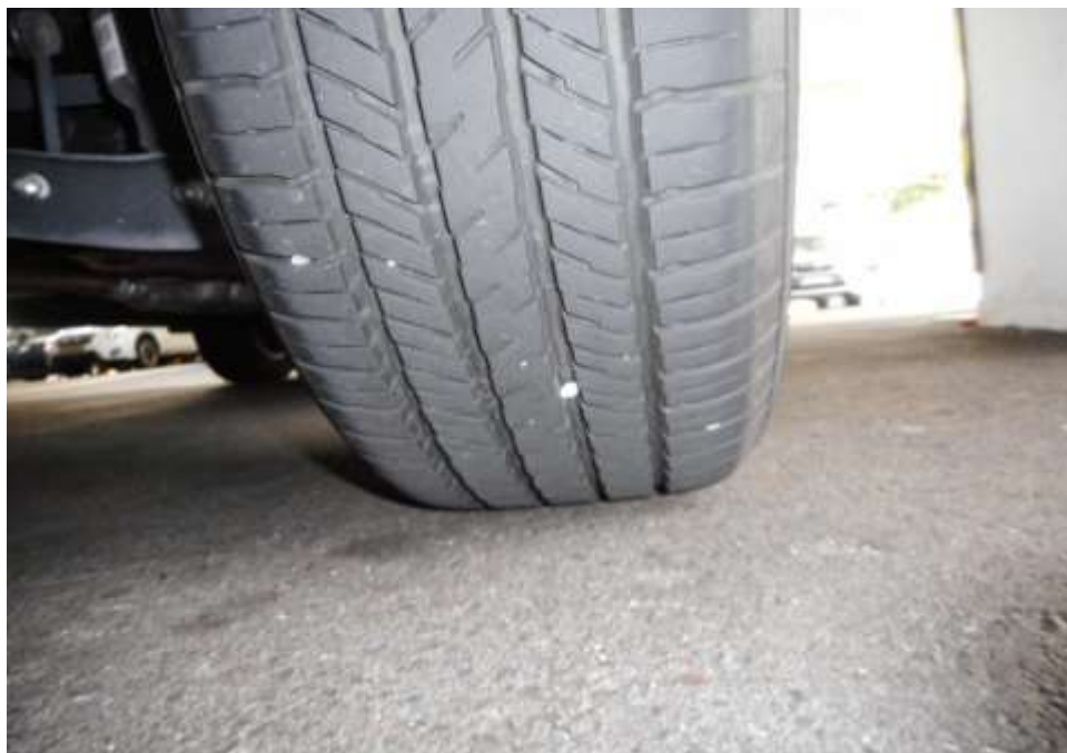
Photo 7 shows the condition of the rear right tyre of the Motor Car, which was observed to be in serviceable condition with remaining tread depth of approximately 6.4mm. The tyre, which was wrapped around standard alloy wheel rim, was also observed to be sufficiently inflated for vehicular operation.
