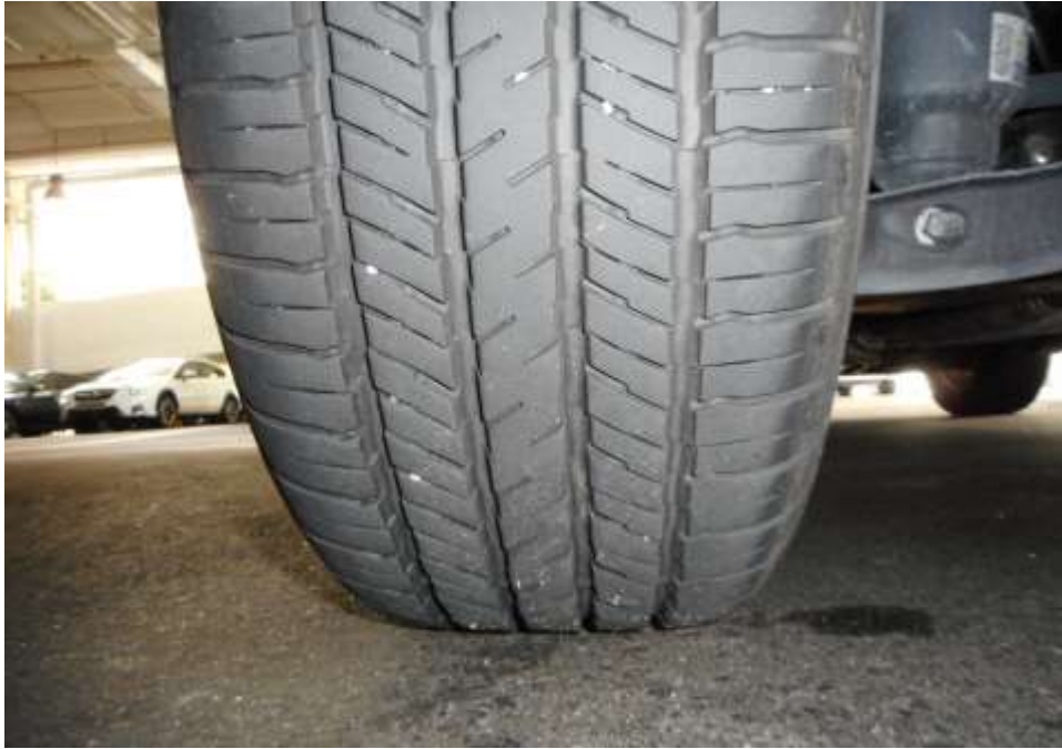
Photo 8 shows the condition of the rear left tyres of the Motor Car, which was observed to be in serviceable condition with remaining tread depth of approximately 6.3mm. The tyres, which were wrapped around standard alloy wheel rim, were also observed to be sufficiently inflated for vehicular operation. There was also no damage found on all 4 alloy wheel rims of the Motor Car.
