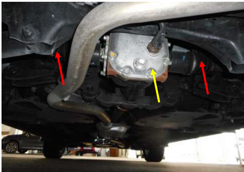
Photo 21 shows the various undercarriage components at the rear transfer case (yellow arrow) and rear driveshaft (red arrow) both for the AWD system of the Motor Car. The various components were all found to be intact, suggesting that the steering system of the Motor Car was likely to be in serviceable condition at the material time of accident. There was also no sign of fluid stain(s) observed on the various undercarriage components.
