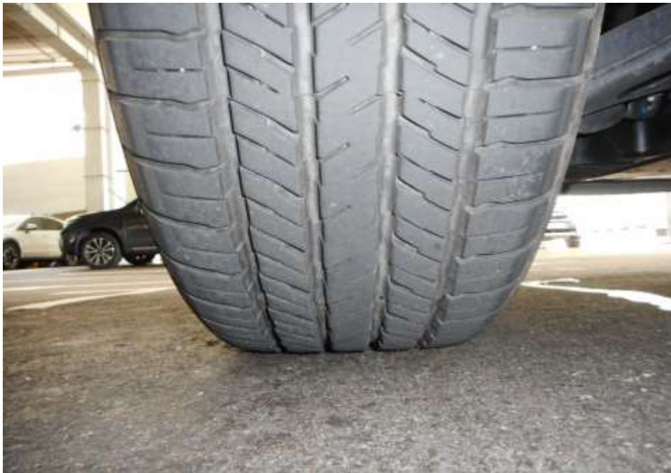
Photo 9 shows the condition of the rear right tyres of the Motor Car, which were observed to be in serviceable condition with remaining, tread depth of approximately 6.3mm. There was also no tear, cut or burst mark(s) on the outer and the inner sidewalls as well as across the tread of the 4 tyres that were fitted on the Motor Car.
