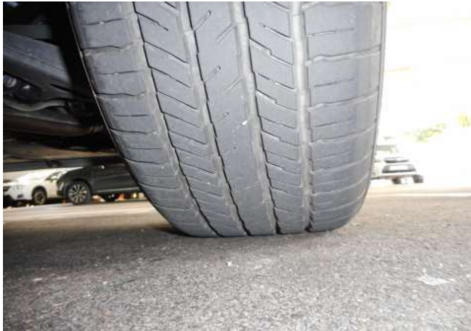
Photo 6 shows the condition of the front right tyre of the Motor Car, which was observed to be in serviceable condition with remaining tread depth of approximately 5.9mm. The tyre, which was wrapped around standard alloy wheel rim, was also observed to be sufficiently inflated for vehicular operation. There was no tear, cut or burst mark(s) on the outer and the inner sidewalls as well as across the tread of the 4 tyres that were fitted on the Motor Car.
