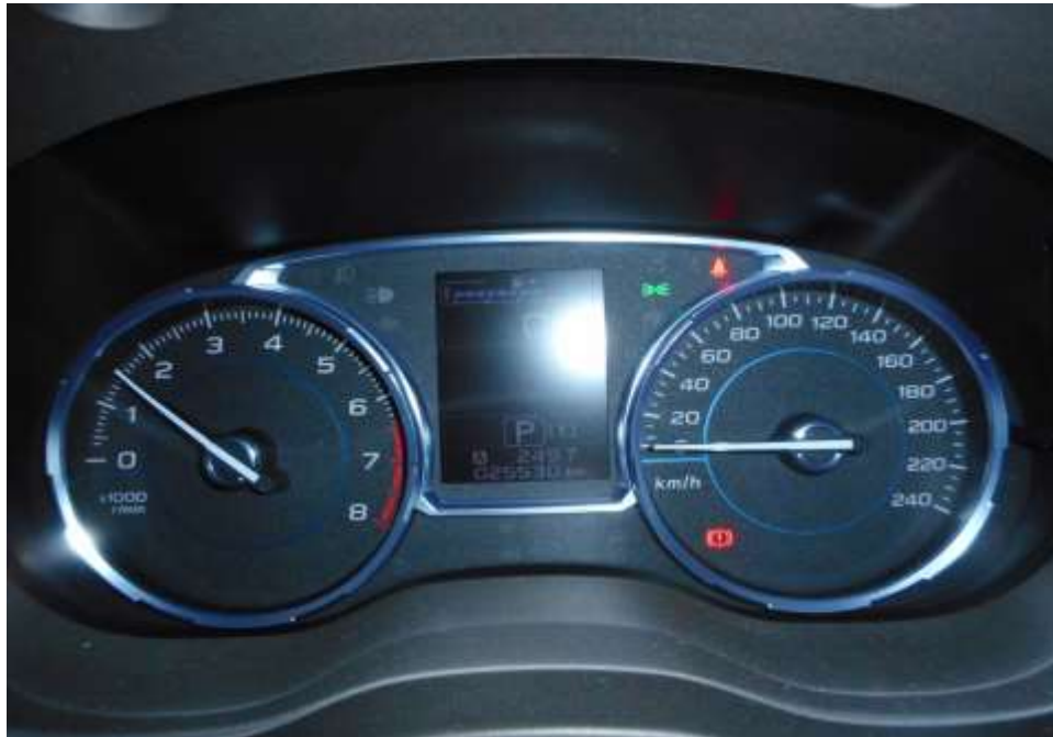
Photo 24 shows no warning lights illuminated on the instrument panel of the Motor Car after the engine was cranked. This would suggest that there was no abnormality to the various electronic operating systems of the Motor Car, like the ABS, TC, SRS and EPS.
