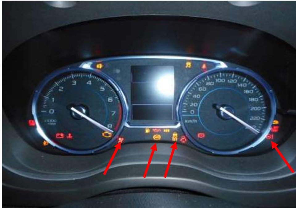
Photo 23 shows the warning light for Anti-Lock Brake System (ABS), Traction Control (TC), Supplemental Restraint System (SRS) and Electric Power Steering System (EPS) appearing on the instrument panel of the Motor Car during the self-test of its various electronic operating systems when its engine was cranked.
