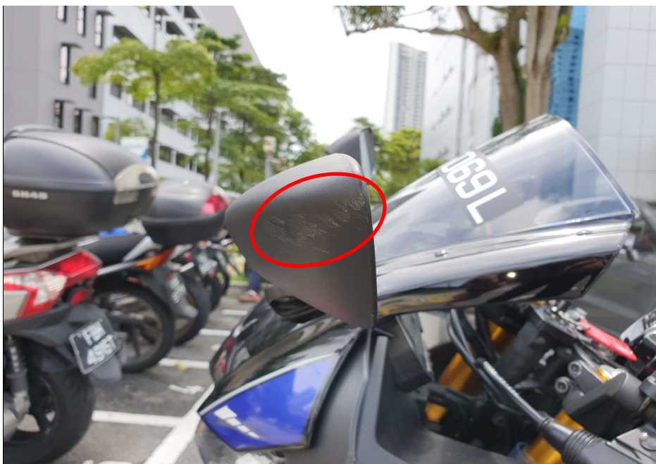
Photo 8 shows a closer view of the left side mirror of the Yamaha at the time of reporting, which was about 2 days after the accident. We observed scratches on the back portion (circled).
