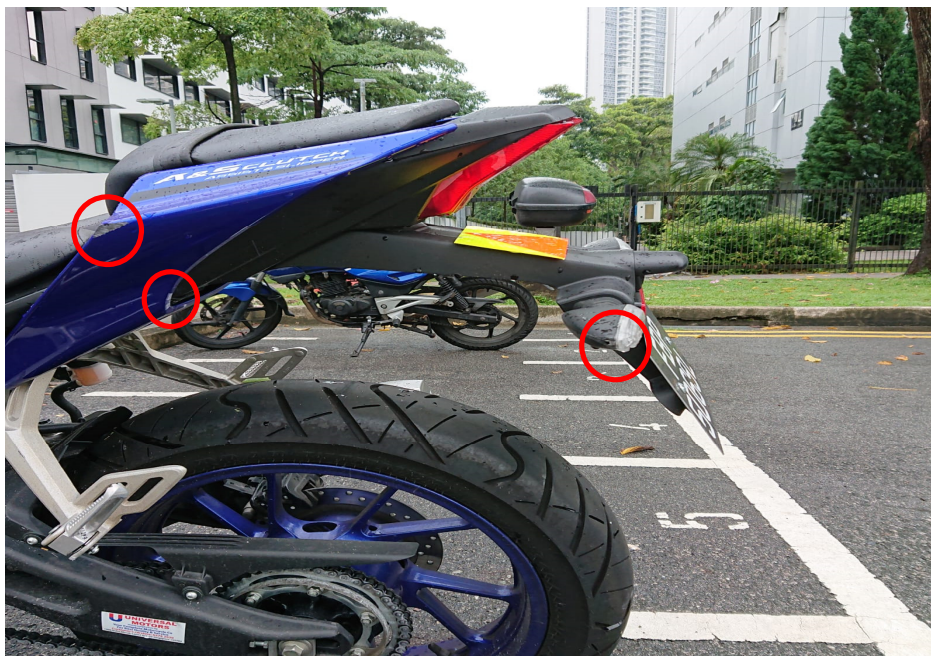
Photo 10 shows a closer view of the damages of grazing nature observed on the left rear side cover and left rear signal lamp of the Yamaha (circled) at the time of reporting, which was about 2 days after the accident.
