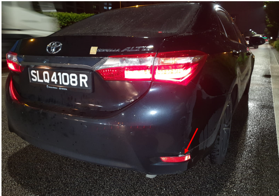
Photo 12 shows a closer view of the bottom right portion of the rear bumper of the Toyota post- accident. We observed paint cracks on the bottom right portion of the rear bumper of the Toyota (arrowed).
