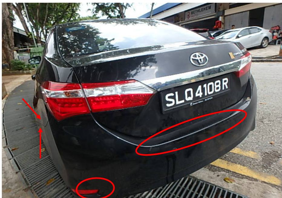
Photo 1 shows the general view of the rear left portion of the Toyota at the time of the Pre- Repair Survey conducted by LKK Auto Consultants Pte. Ltd. The damage to the Toyota was observed to be confined to its rear portion, at the rear bumper (circled). We also noted that the rear bumper was not misaligned at its left corner edges (arrowed).
