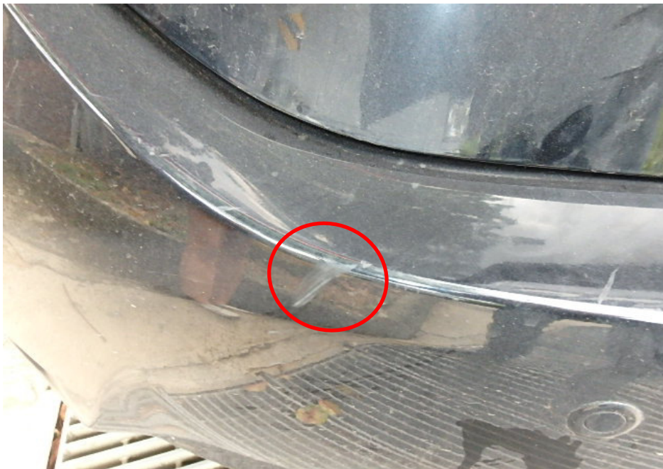
Photo 4 shows closer view of the left top portion of the rear bumper. Paint graze marks were observed (circled).
