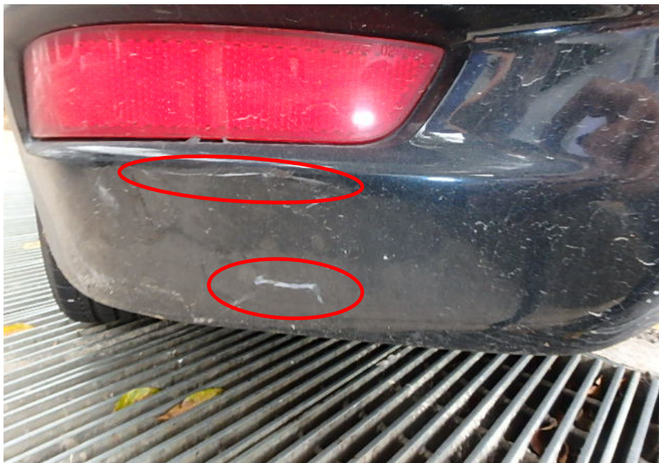
Photo 5 shows a closer view of the bottom left portion of the rear bumper of the Toyota at the time of the Pre- Repair Survey conducted by LKK Auto Consultants Pte. Ltd. We observed horizontal paint graze marks below the left rear bumper reflector (circled).
