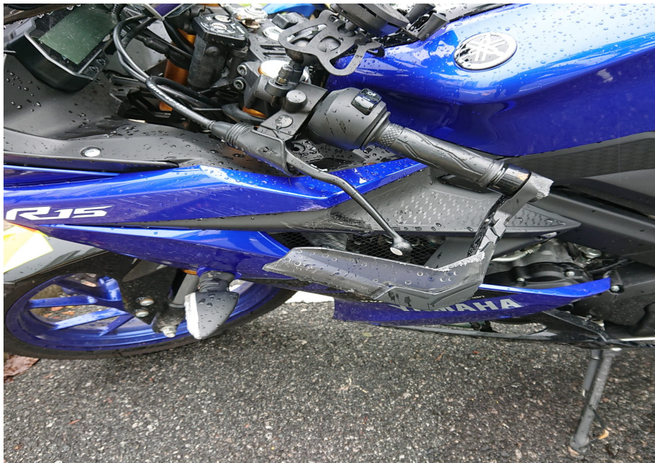
Photo 9 shows a closer view of the damages of grazing nature observed on the left cowling of the Yamaha at the time of reporting, which was about 2 days after the accident.
