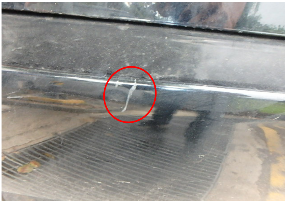
Photo 3 shows a closer view of the centre top portion of the rear bumper. Paint graze marks were observed (circled).
