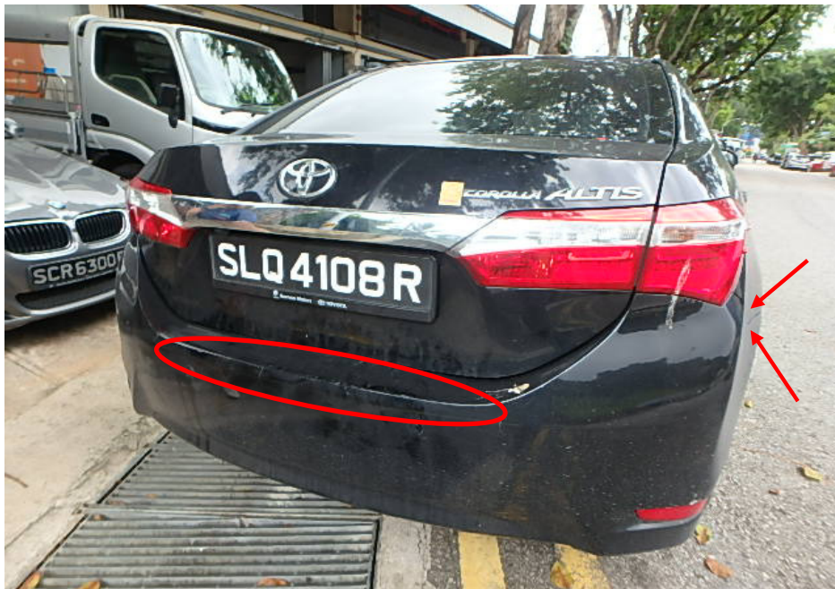
Photo 2 shows the general view of the rear right portion of the Toyota at the time of the Pre- Repair Survey conducted by LKK Auto Consultants Pte. Ltd. The damage to the Toyota was observed to be confined to its rear portion, at the rear bumper (circled). We also noted that the rear bumper was not misaligned at its right corner edges (arrowed).
