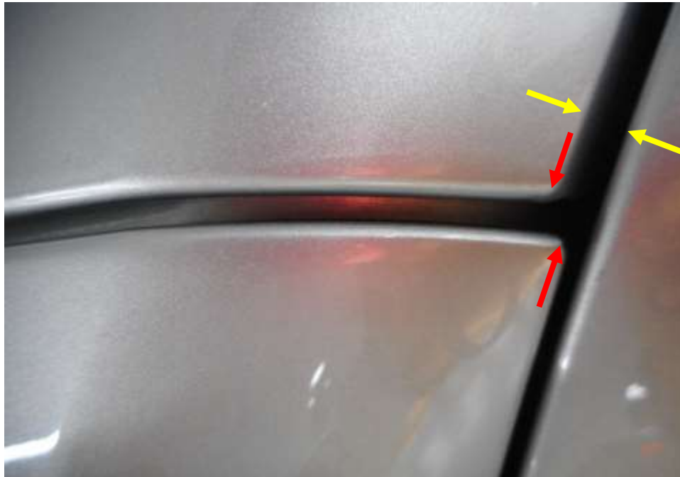
Photo 7 shows the close up view of the front left bumper portion and left fender and left bonnet portion of the Insured Vehicle at the time of our inspection. A alignment differences between the front left bonnet, front left bumper (red arrow) and front left fender, front left bonnet (yellow arrow) as observed.
