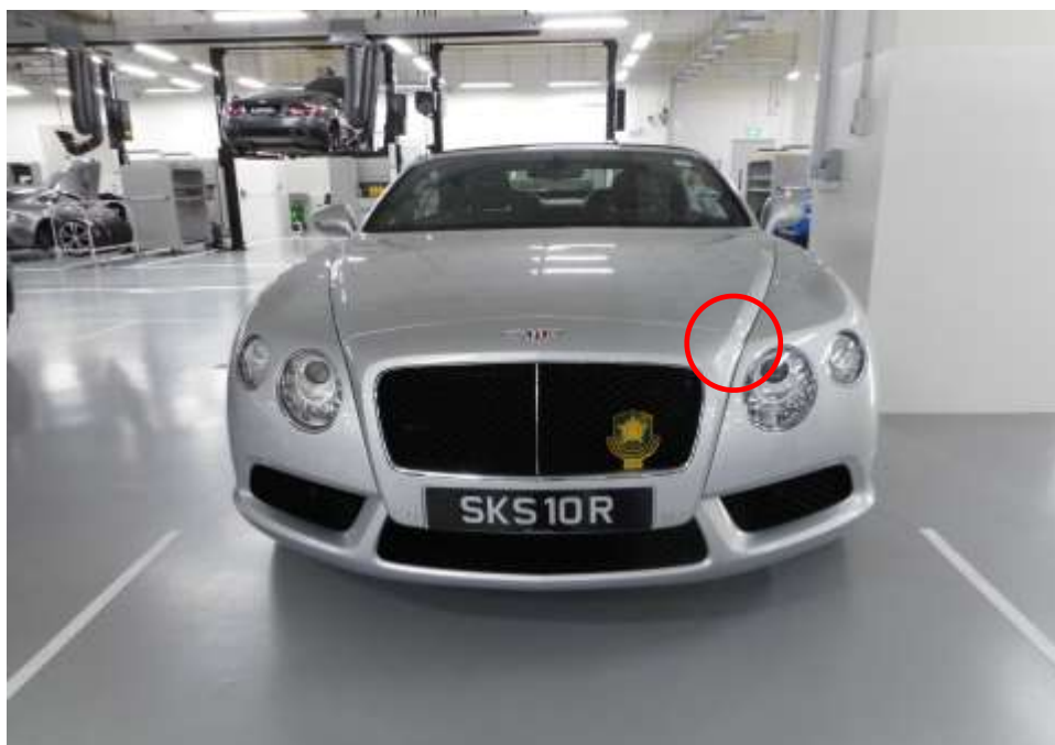
Photo 4 shows the general view of the front portion of the Insured Vehicle at the time of our inspection. The alignment of the front left bumper, front left fender and front bonnet (circled) was found to be misaligned at the time of our inspection.
