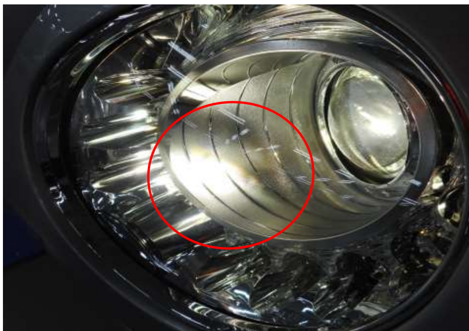
Photo 12 shows the close up view of the left portion of the Insured Vehicle at the time of our inspection. The front left headlight inner cover surface (circled) of the Insured Vehicle was observed to be clear as compared to the front right headlight (Refer to photo 10 above).
