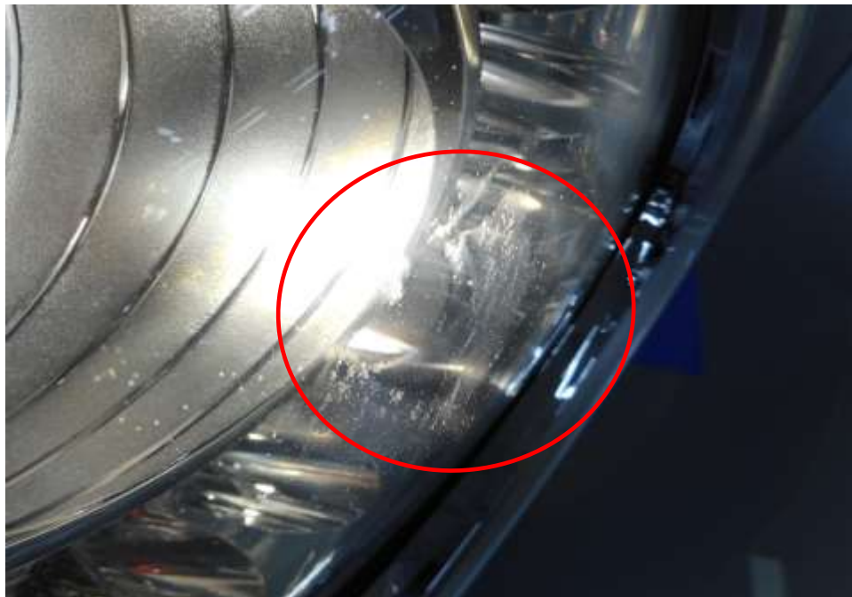
Photo 10 shows the close up view of the right portion of the Insured Vehicle at the time of our inspection. The front right headlight inner cover surface (circled) of the Insured Vehicle was observed with hazy stain marks.
