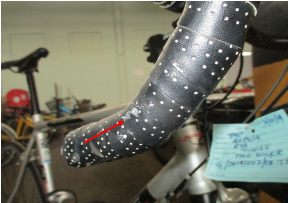
Photo 7 shows the damaged right handlebar (arrowed) of the Bicycle at the time of our inspection.
