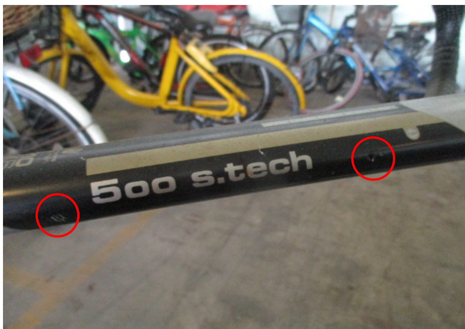
Photo 9 shows the damages of grazing nature on the right frame (circled) of the Bicycle at the time of our inspection.
