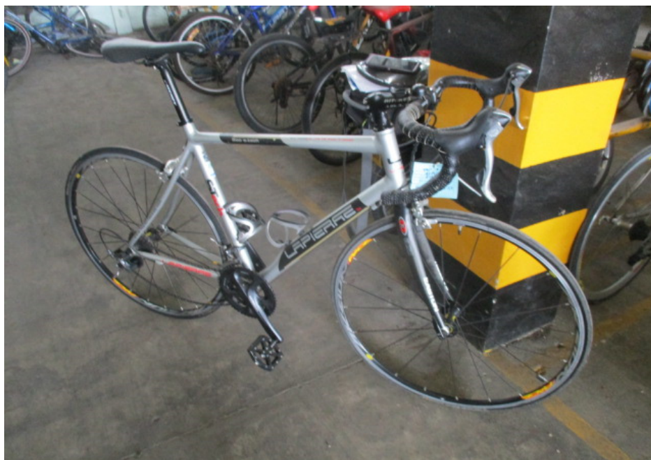
Photo 4 shows the right body of the Bicycle at time of our inspection. The bicycle had sustained damages to its right body. The body parts that were found to have been damaged include its rear brake lever, right handlebar, right pedal and right frame, amongst others as a result of the accident.
