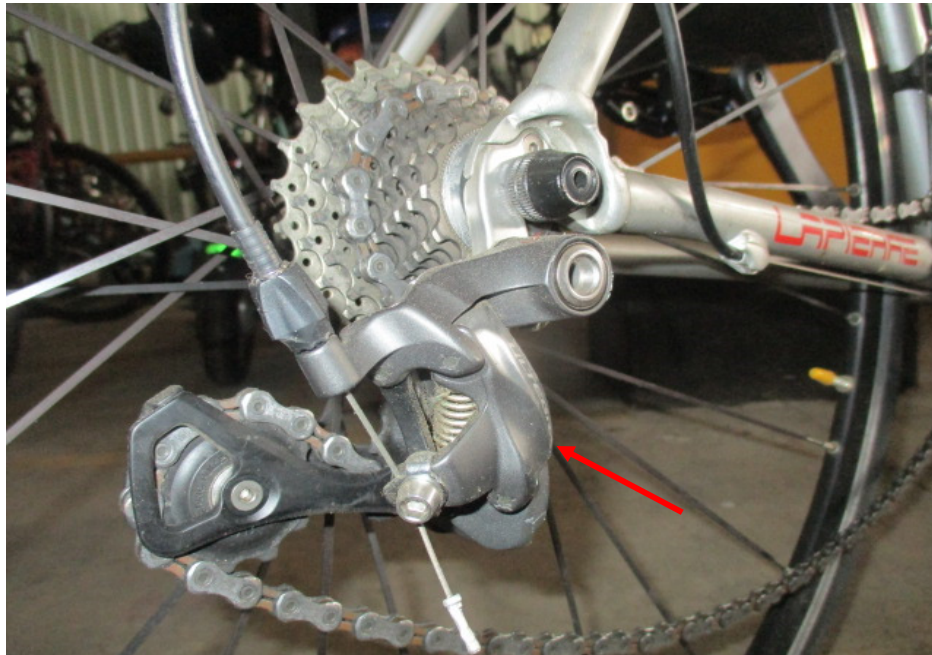
Photo 14 shows a closer view of the gear train (arrowed) of the Bicycle, which was observed to be intact with no misalignment. It was also adequately lubricated for operating purposes.
