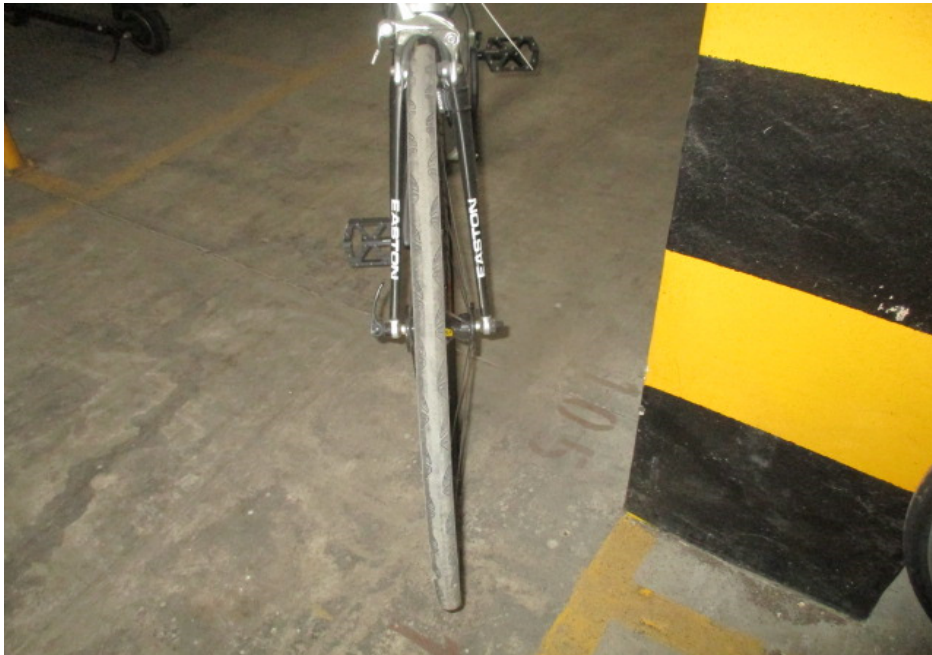
Photo 11 shows the front tyre of the Bicycle. The pattern of the tread was clearly visible. There was no tear, burst mark(s) and/or punctured hole(s) on the sidewalls as well as across the tread of the front tyre. However the front tyre was observed to be deflated.
