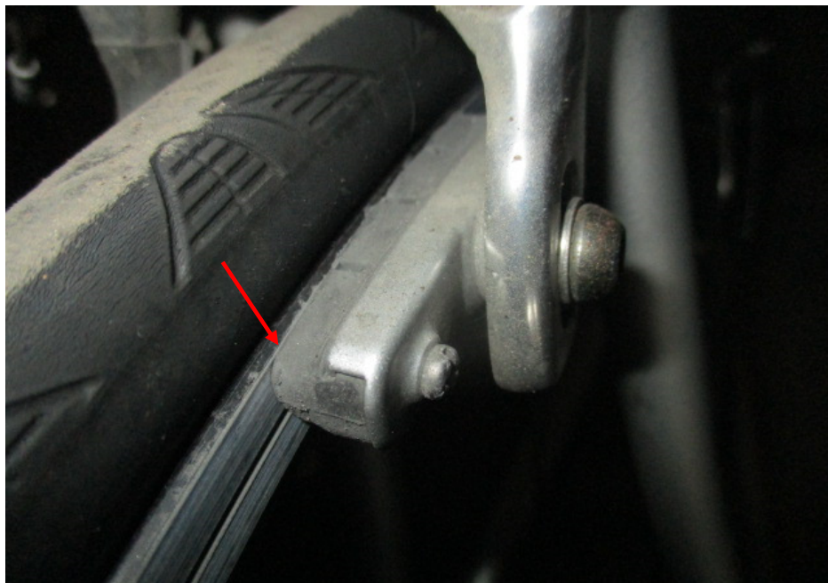
Photo 21 shows a close up view of the rear brake clamps responding to the gripping action. The rubber brake blocks pressed against the rear wheel rim upon depressing the right hand brake lever (arrowed). This had appeared to indicate that the rear brake was in serviceable condition.
