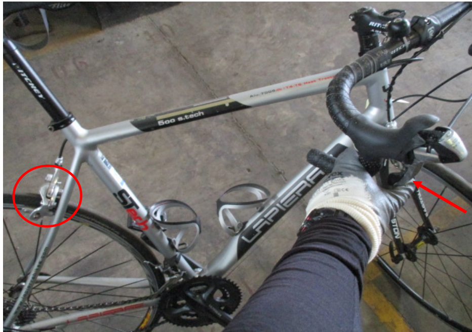
Photo 20 shows a static brake test conducted on the Bicycle's rear brake. There was some resistance felt upon pressing the right hand brake lever (arrowed). It also shows that the rear brake clamps responded to the gripping action (circled) after depressing the right hand brake lever.
