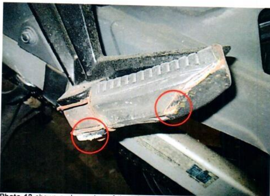
Photo 12 shows a closer view of the left pillion footrest bracket and left pillion foot peg, which were amongst the body parts of the Motorcycle that had sustained damage as a result of the accident (circled).
