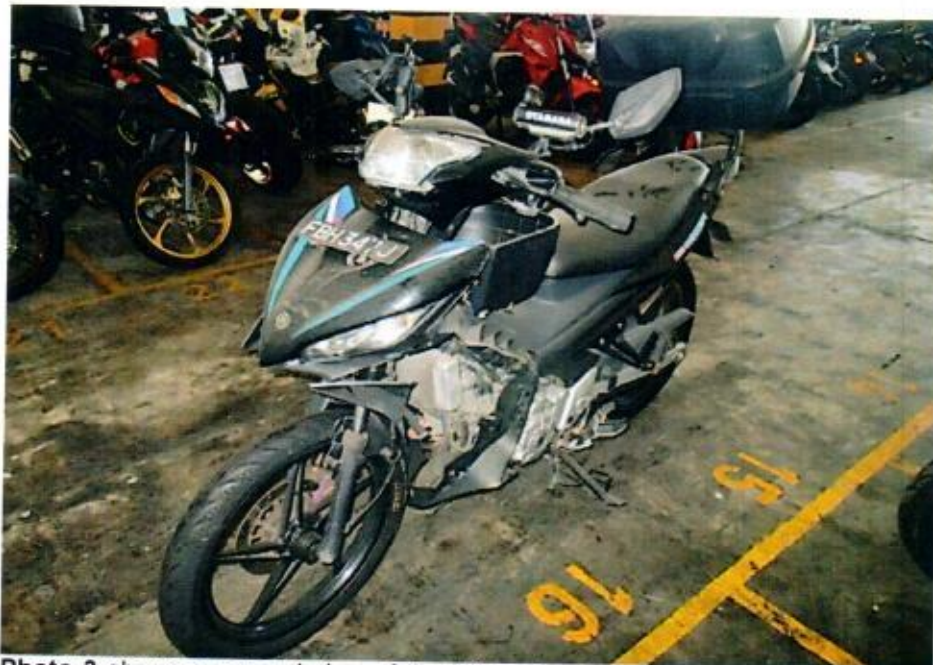
Photo 3 shows a general view of the left body of the Motorcycle at the time of our inspection. Body parts that were found to have been damaged include its headlight, head cowl, front fork assembly, steering stem, side cowlings, left side mirror, clutch lever, gear shift pedal, left front footrest, left pillion footrest bracket and rear number plate, amongst others.
