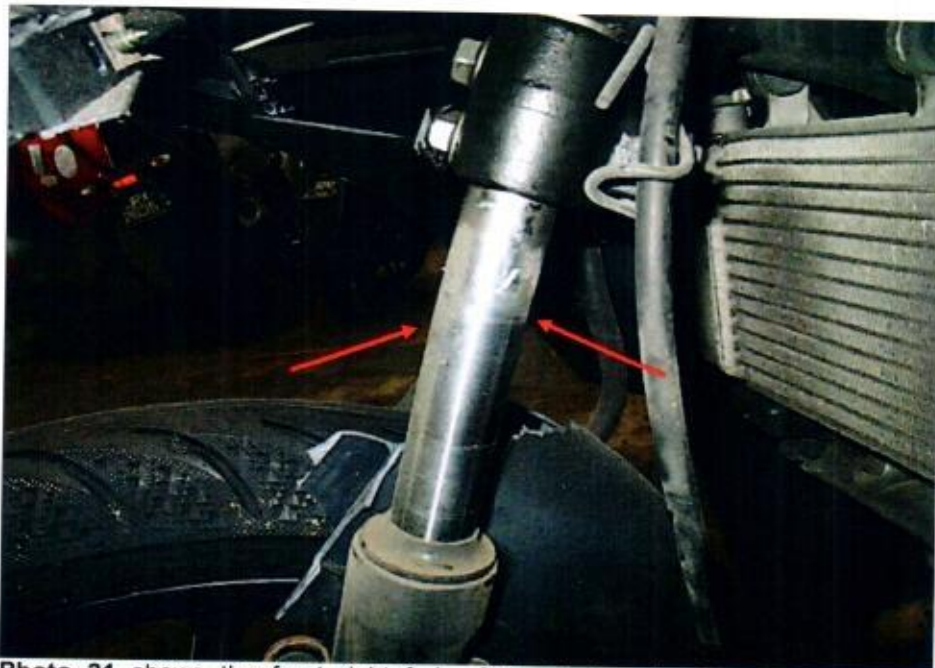
Photo 21 shows the front right fork of the Motorcycle. The front right fork (arrowed) was observed to be bent inwards as a result of the accident. We were hence not able to conduct any tests on the steering system of the Motorcycle.
