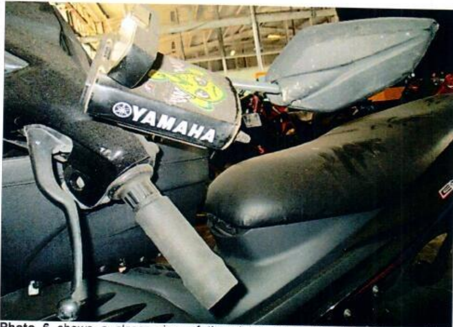
Photo 6 shows a closer view of the clutch lever, left side mirror and left handlebar grip of the Motorcycle. These parts were amongst the body parts of the Motorcycle which were damaged as a result of the accident.
