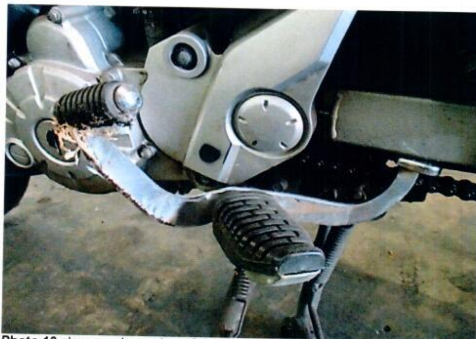
Photo 13 shows a closer view of the gear shift pedal and left front footrest which were amongst the body parts of the Motorcycle that had sustained damage as a result of the accident.
