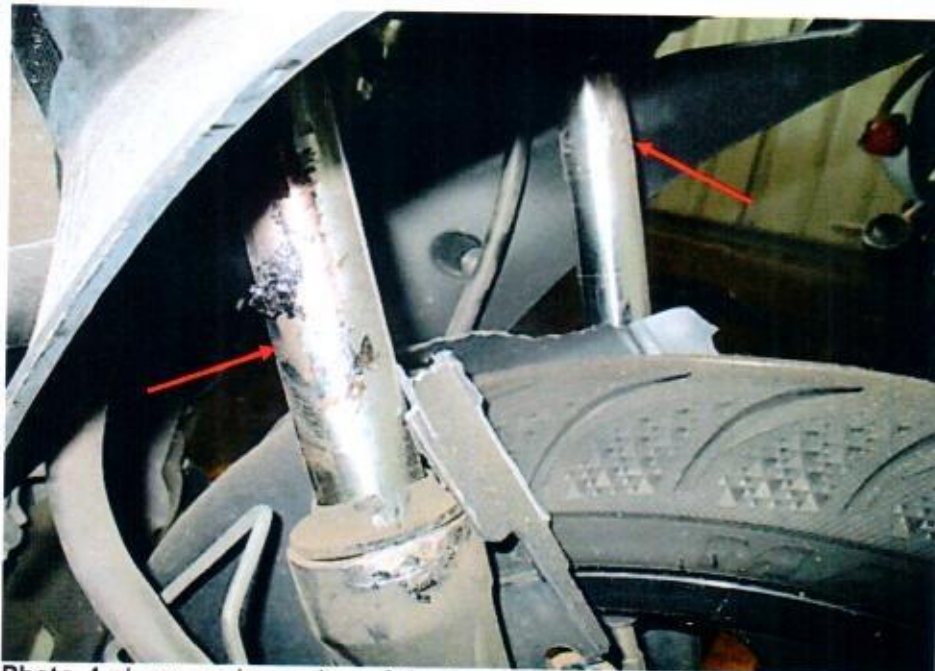
Photo 4 shows a closer view of the front fork assembly (arrowed) which was amongst the body parts at the front body of the Motorcycle that had sustained damage as a result of the accident.
