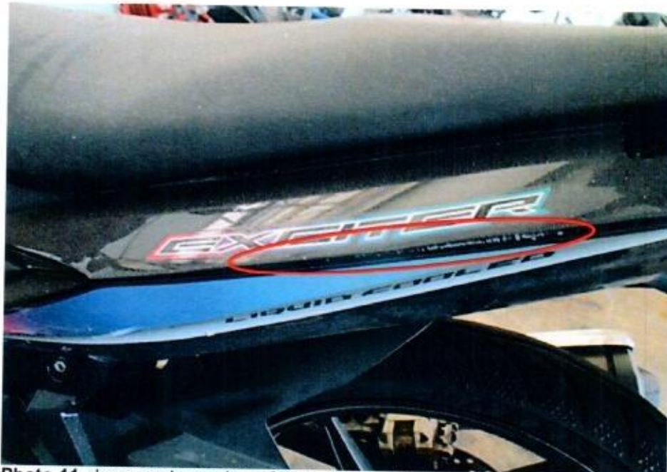
Photo 11 shows a closer view of the left rear side cover which was amongst the body parts of the Motorcycle that had sustained damages of grazing nature as a result of the accident (circled).
