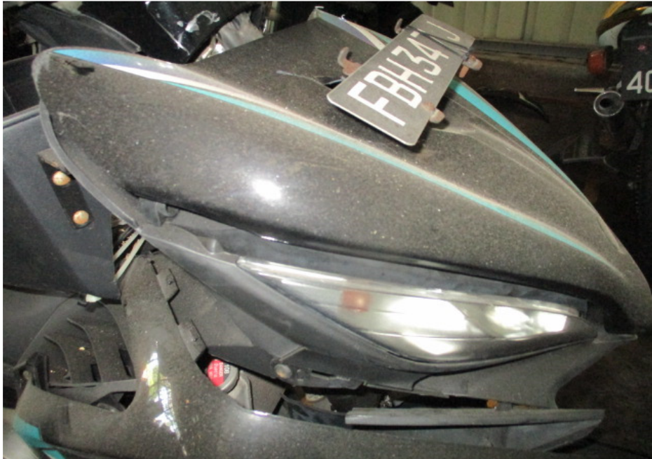
Photo 8 shows a closer view of the head cowl which was amongst the body parts at the front body of the Motorcycle that had sustained damages as a result of the accident.
