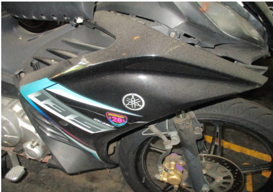
Photo 9 shows a closer view of the right cowl which was amongst the body parts at the front body of the Motorcycle that had sustained damages as a result of the accident.
