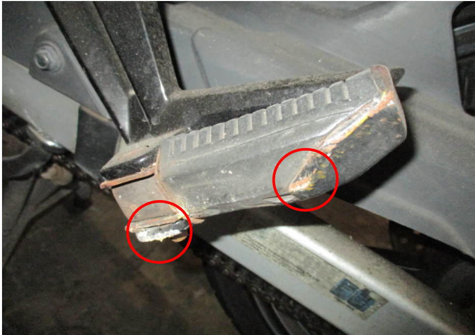
Photo 12 shows a closer view of the left pillion footrest bracket and left pillion foot peg, which were amongst the body parts of the Motorcycle that had sustained damage as a result of the accident (circled).
