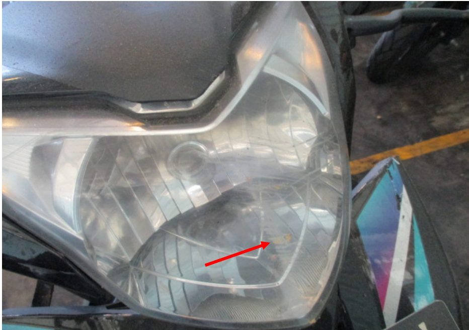
Photo 5 shows a closer view of the headlight which was amongst the body parts at the front body of the Motorcycle that had sustained damages as a result of the accident (arrowed).
