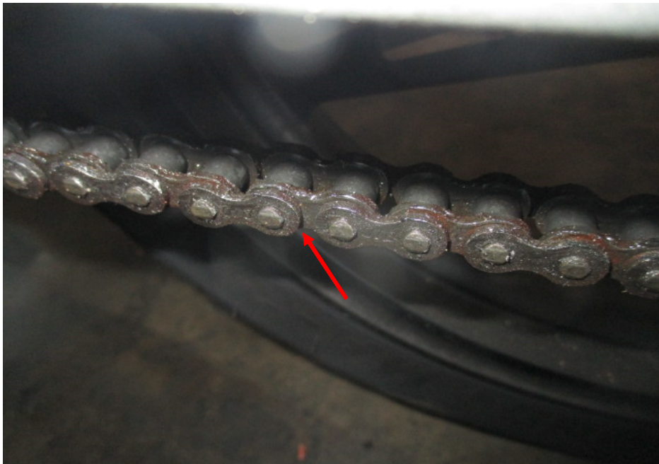
Photo 20 shows the closer view of the gear chain (arrowed) of the Motorcycle, which was observed to be intact with no misalignment. It was also adequately lubricated for operating purposes.
