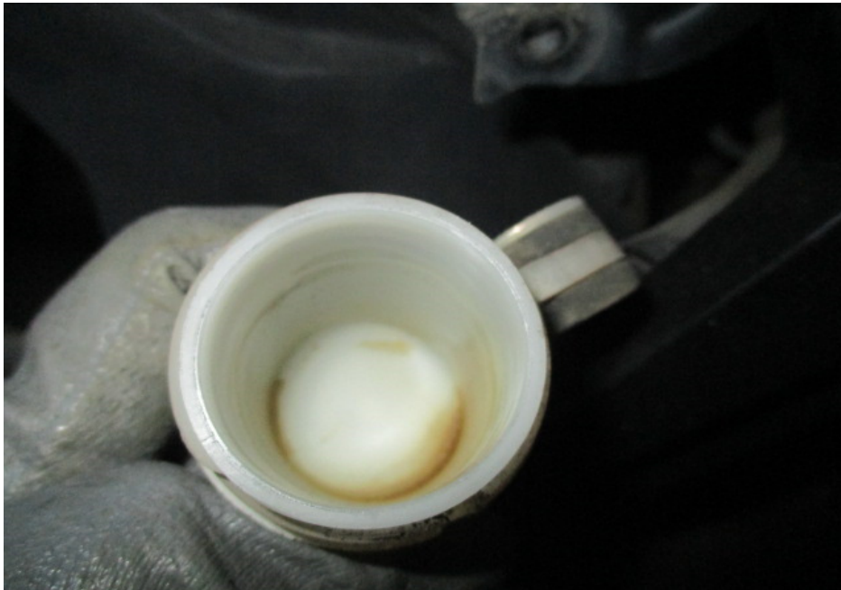
Photo 27 shows the brake fluid reservoir for the rear brake of the Motorcycle. The rear brake fluid reservoir was observed to be empty at the time of our inspection.
