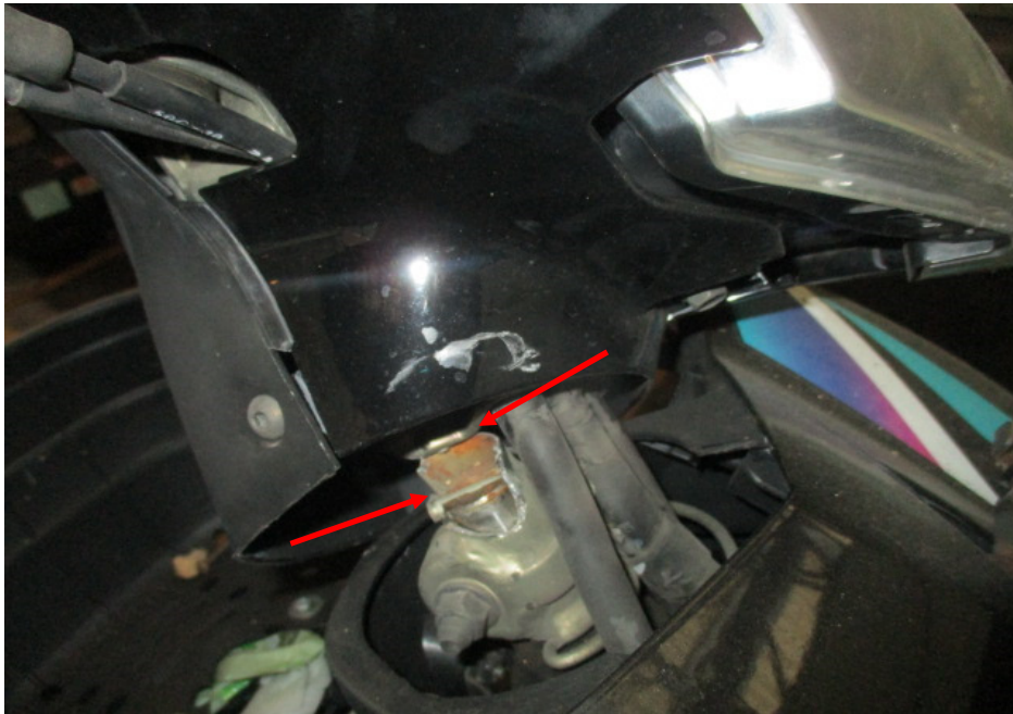
Photo 22 shows the steering stem of the Motorcycle. The steering stem (arrowed) was observed to be broken as a result of the accident. We were hence not able to conduct any tests on the steering system of the Motorcycle.
