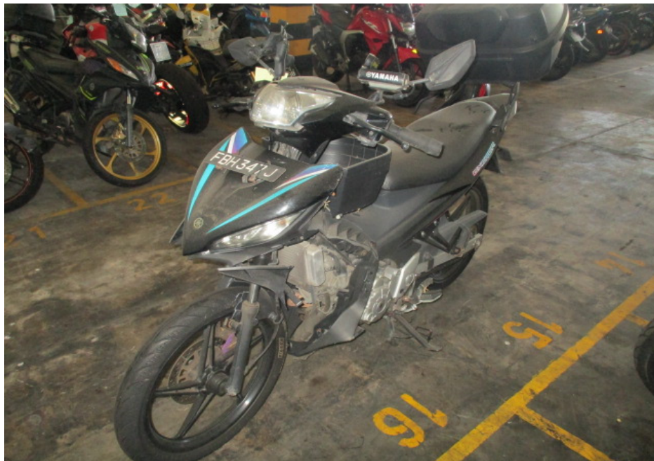
Photo 3 shows a general view of the left body of the Motorcycle at the time of our inspection. Body parts that were found to have been damaged include its headlight, head cowlings, front fork assembly, steering stem, side cowlings, left side mirror, clutch lever, gear shift pedal, left front footrest, left pillion footrest bracket and rear number plate, amongst others.
