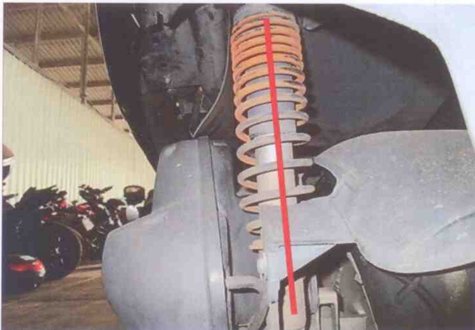
Photo 16 shows the left shock absorber of the motorcycle which was found to be intact however slightly misaligned as a result of the accident.
