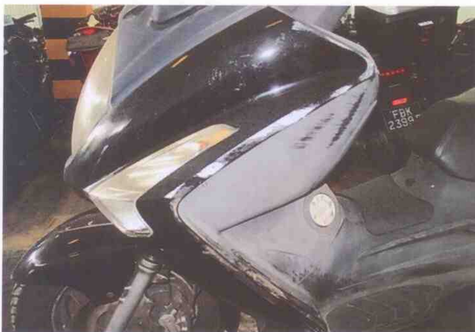
Photo 6 shows a closer view of the left cowling which was amongst the body parts at the front body of the Motorcycle that had sustained damage as a result of the accident.
