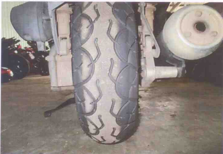
Photo 13 shows the condition of the Motorcycle's rear tyre. The rear tyre was observed to be in serviceable condition with remaining tread depth of approximately 4mm. The tyre was also observed to be sufficiently inflated for vehicular operation. We did not observe any tear, burst mark(s) and/or punctured hole(s) on the sidewalls as well as across the tread of the rear tyre.
