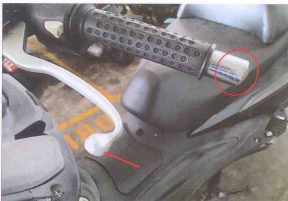
Photo 5 shows a closer view of the rear brake lever (arrowed) and left handlebar end (circled) of the Motorcycle which were observed to be damaged due to the accident.
