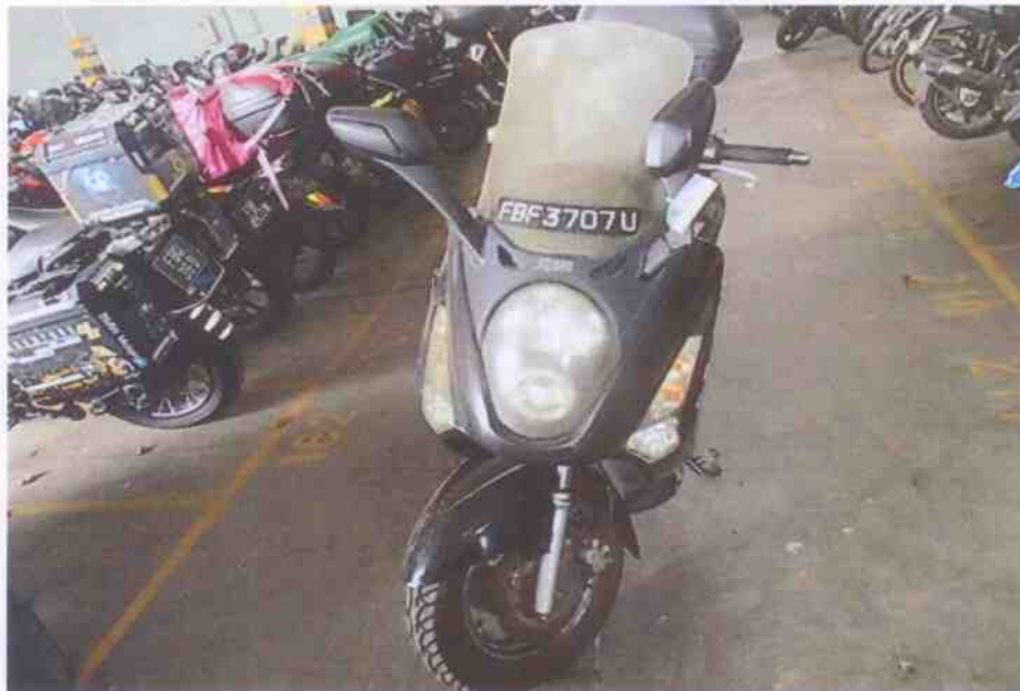
Photo 19 shows the front wheel of the Motorcycle turned towards its full right. Turning the Motorcycle's handle bar towards the left and right did not produce any abnormal free play and/or resistance. This would indicate that the steering system of the Motorcycle was in serviceable condition at the time of our inspection.
