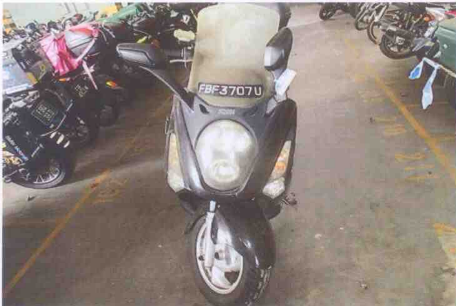
Photo 20 shows the front wheel of the Motorcycle turned towards its full left. Turning the Motorcycle's handle bar towards the left and right did not produce any abnormal free play and/or resistance. This would indicate that the steering system of the Motorcycle was in serviceable condition at the time of our inspection.
