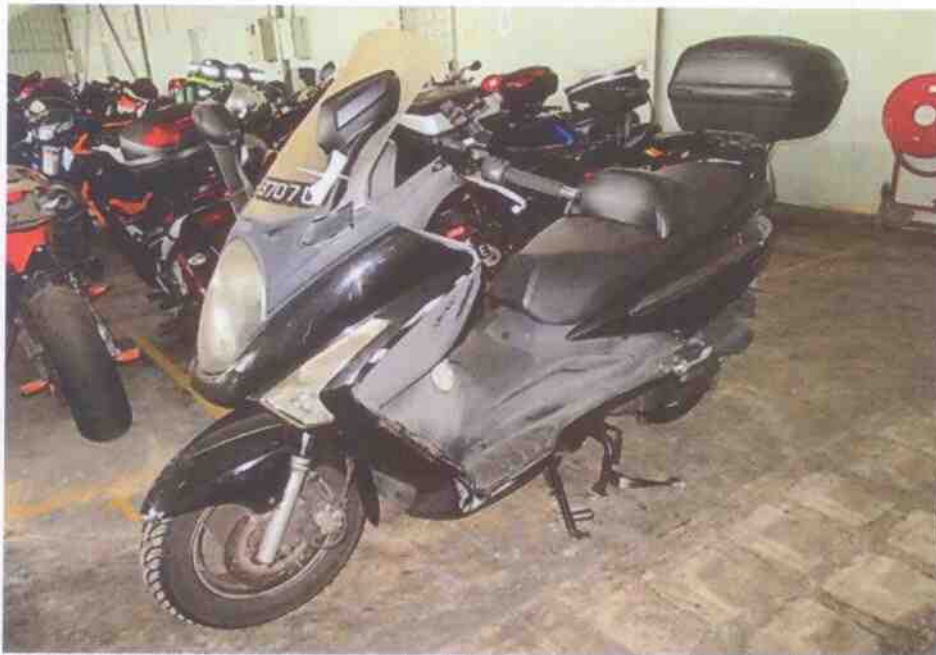
Photo 3 shows a general view of the left front body of the Motorcycle at the time of our inspection. The Motorcycle was observed to have sustained minor damages at the frontal and left portion. The body parts that were found to have been damaged include its front mudguard, rear brake lever, left side mirror, left cowl, left rear side cover, left pillion foot rest, main stand and top box, amongst others as a result of the accident.
