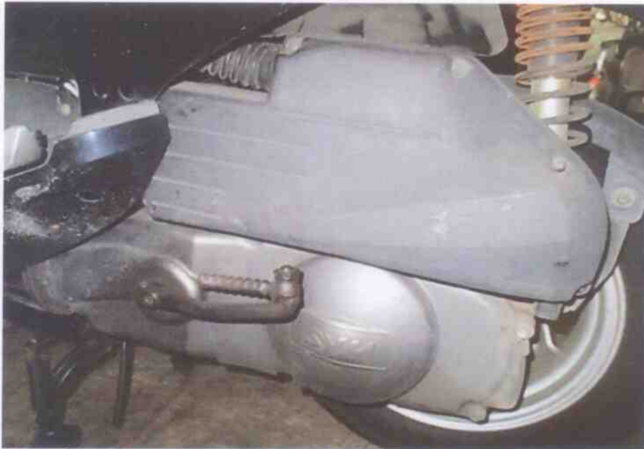
Photo 15 shows the drive train of the Motorcycle which was found to be intact without any misalignment.
