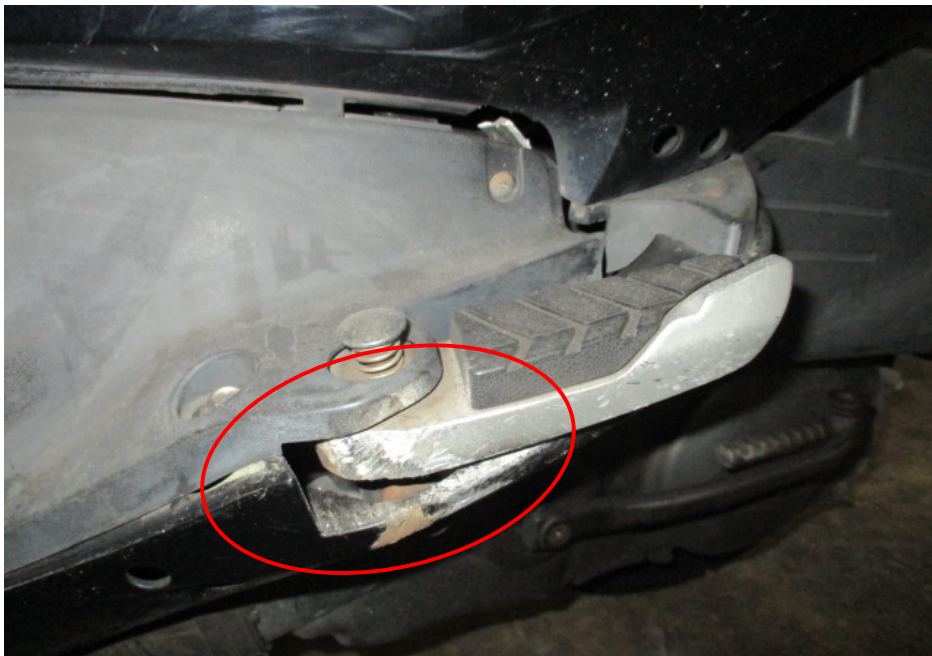
Photo 8 shows a closer view of the damaged left pillion footrest (circled) of the Motorcycle at the time of our inspection.
