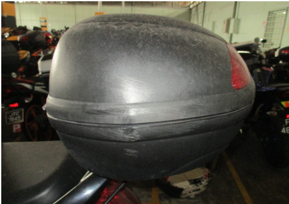
Photo 11 shows a closer view of the top box of the Motorcycle which was observed to have sustained damages of grazing nature due to the accident.
