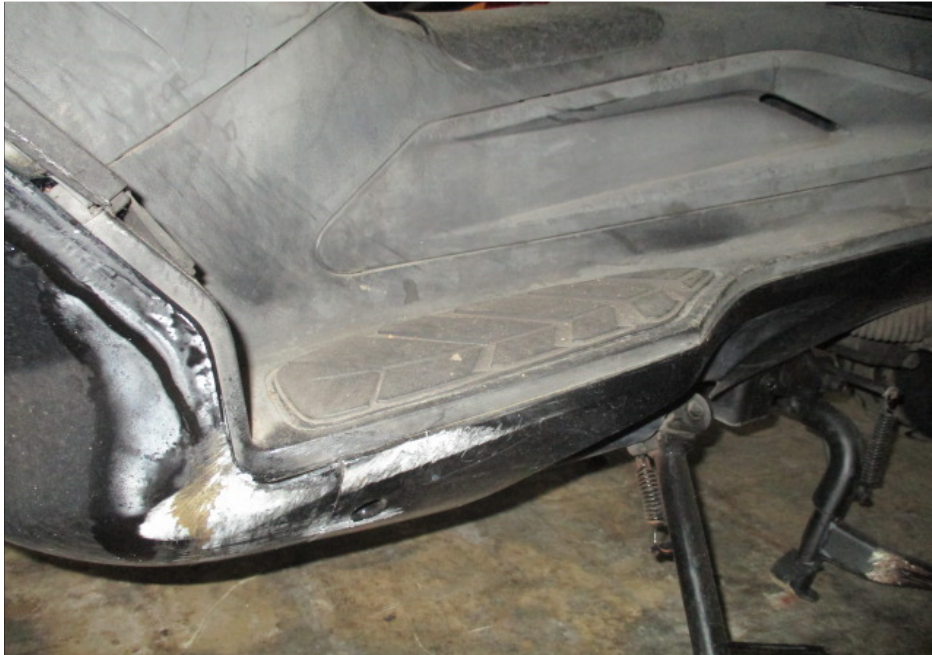
Photo 7 shows a closer view of the left bottom cowling of the Motorcycle which was observed to be damaged due to the accident.
