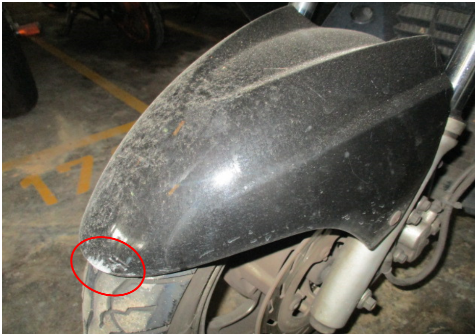
Photo 4 shows a closer view of the front mudguard (circled) which was amongst the body parts at the front body of the Motorcycle that had sustained damage as a result of the accident.
