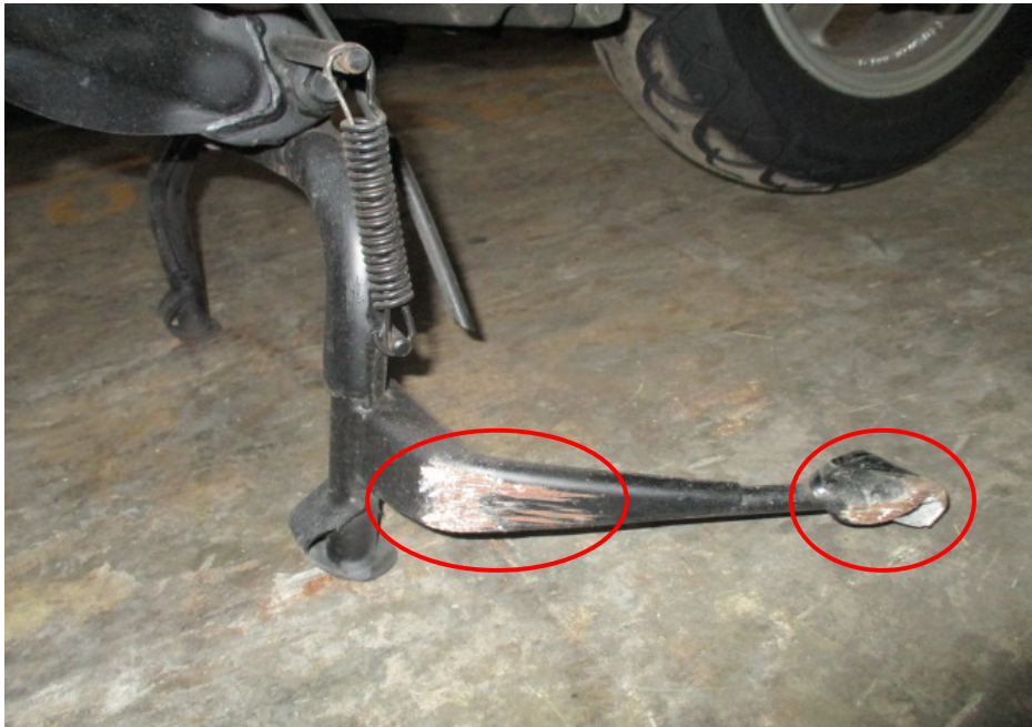
Photo 11 shows a closer view of the main stand of the Motorcycle which was observed to have sustained damages of grazing nature due to the accident (circled).
