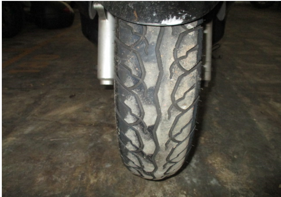
Photo 12 shows the condition of the Motorcycle's front tyre. The front tyre was observed to be in serviceable condition with remaining tread depth of approximately 4mm. There was no tear, burst mark(s) and/or punctured hole(s) on the sidewalls as well as across the tread of the front tyre.
