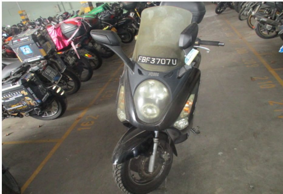
Photo 19 shows the front wheel of the Motorcycle turned towards its full right. Turning the Motorcycle's handle bar towards the left and right did not produce any abnormal free play and/or resistance. This would indicate that the steering system of the Motorcycle was in serviceable condition at the time of our inspection.
