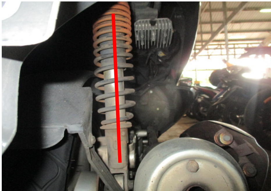
Photo 17 shows the right shock absorber of the motorcycle which was found to be intact without any misalignment.
