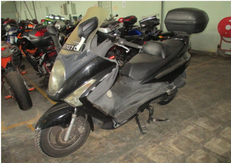
Photo 3 shows a general view of the left front body of the Motorcycle at the time of our inspection. The Motorcycle was observed to have sustained minor damages at the frontal and left portion. The body parts that were found to have been damaged include its front mudguard, rear brake lever, left side mirror, left cowling, left rear side cover, left pillion foot rest, main stand and top box, amongst others as a result of the accident.
