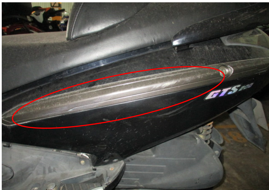
Photo 10 shows a closer view of the damaged left rear side cover of the Motorcycle which was observed to have sustained scratches due to the accident (circled).
