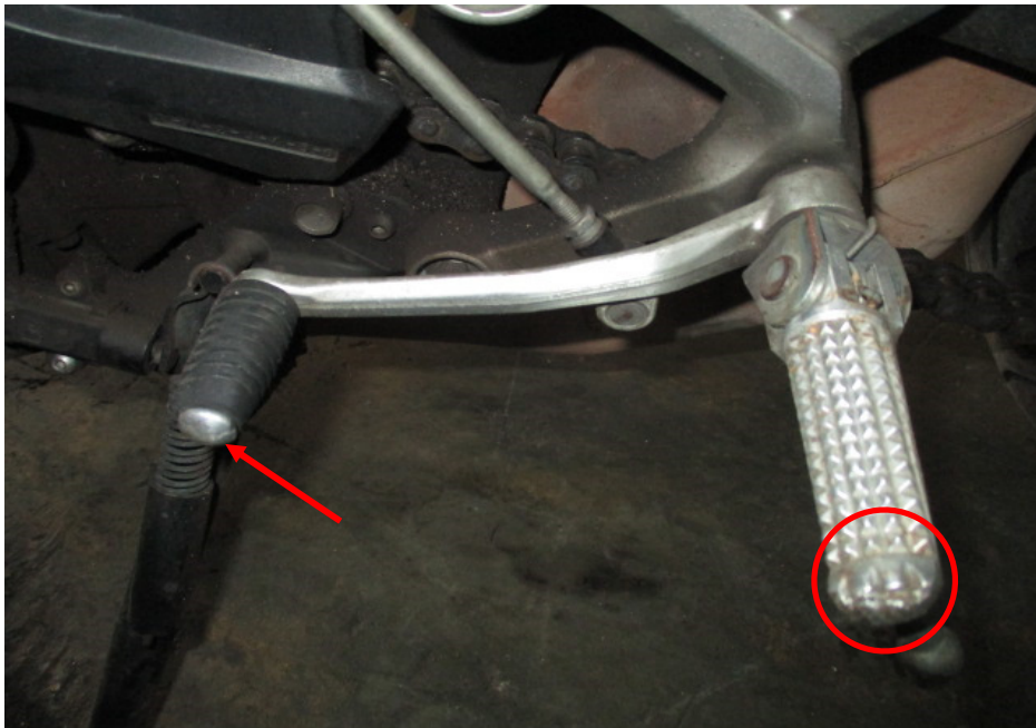
Photo 9 shows a closer view of the gear shift pedal (arrowed) and left front footrest (circled) which were amongst the body parts of the Motorcycle that had sustained damage as a result of the accident.
