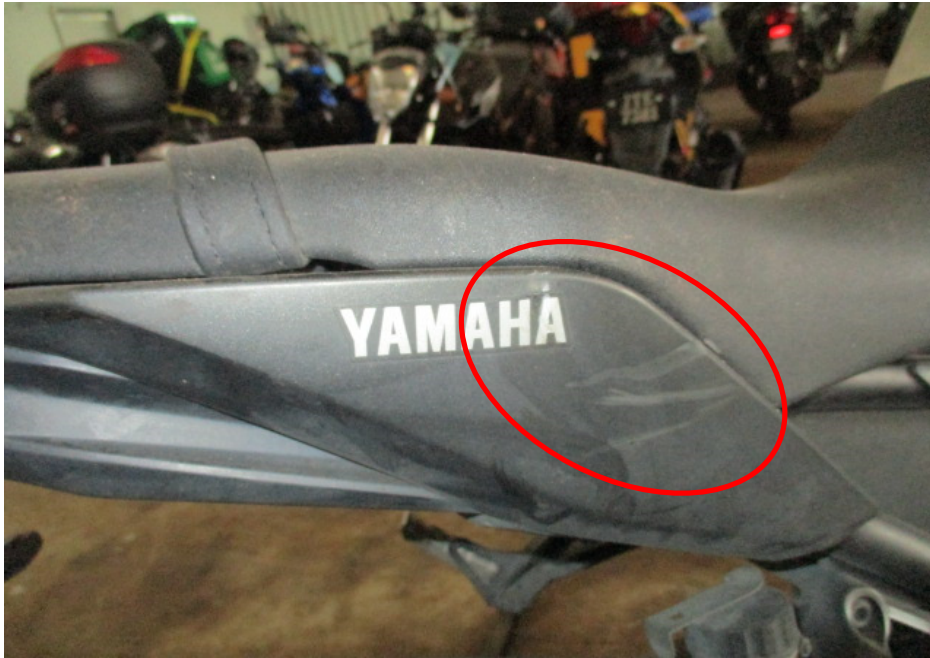
Photo 10 shows a closer view of the right rear side cover which was amongst the body parts of the Motorcycle that had sustained damages of grazing nature as a result of the accident (circled).
