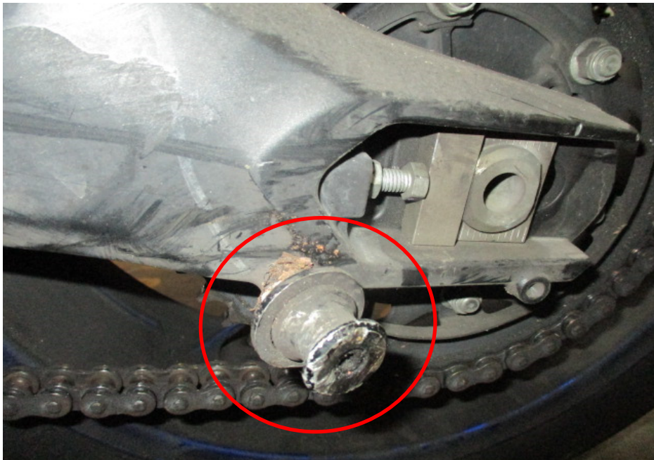
Photo 11 shows a closer view of the swingarm and left swingarm spool which were amongst the body parts of the Motorcycle that had sustained damages of grazing nature as a result of the accident (circled).
