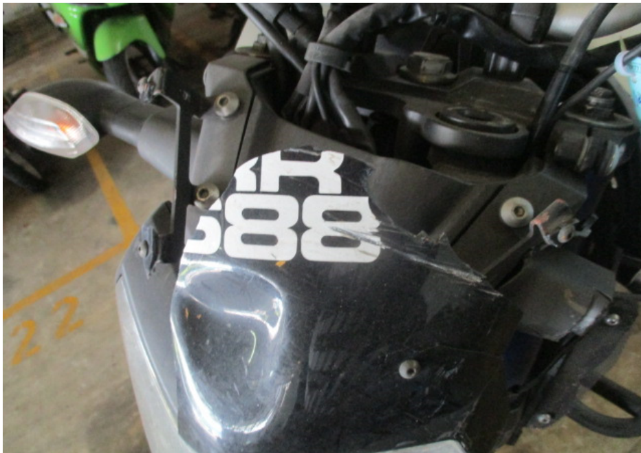
Photo 5 shows a close up view of the cracked windshield which was amongst the body parts of the Motorcycle that had sustained damage as a result of the accident.
