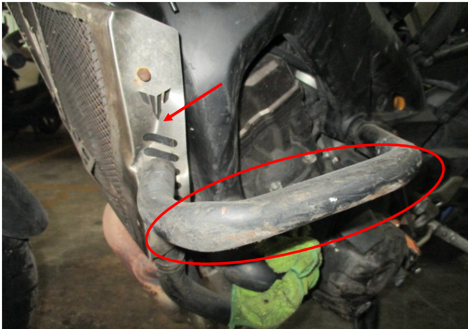
Photo 7 shows a closer view of the left engine crash bar (circled) and radiator guard (arrowed) of the Motorcycle that had sustained damage as a result of the accident.
