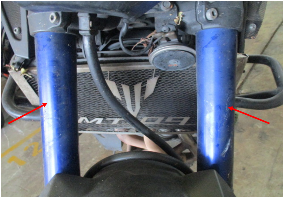
Photo 19 shows the front fork (arrowed) of the Motorcycle. The front fork and fork bracket of the Motorcycle were both found to be intact and undamaged. Turning the Motorcycle's handle bar towards the left and right did not produce any abnormal free play and/or resistance. The steering system of the Motorcycle was in serviceable condition at the time of our inspection.
