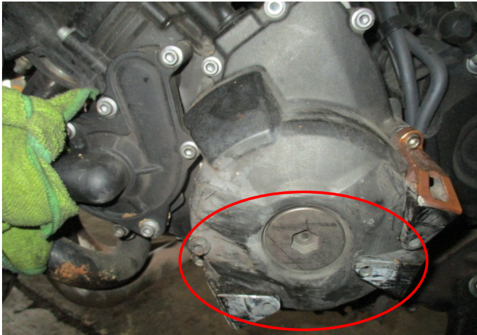
Photo 15 shows the left side of the engine of the Motorcycle at the time of our inspection. The various left engine components had sustained damage of grazing nature as a result of the accident (circled) however the engine components were still intact. There was also no fluid leak and/or fluid stain found around the left engine area of the Motorcycle.
