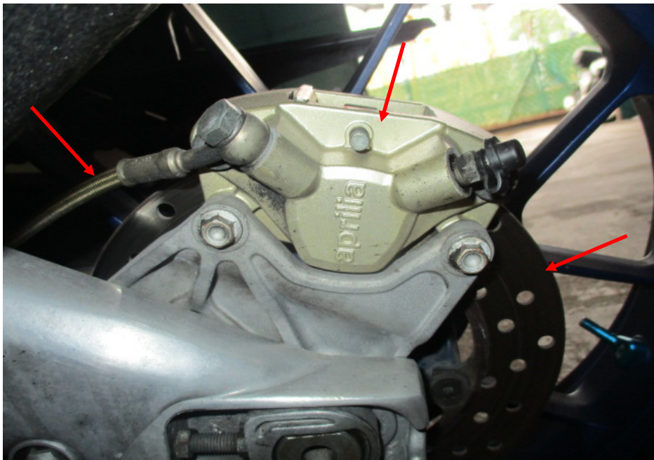
Photo 28 shows a close up view of the rear brake caliper, rear brake disc and rear brake hose (arrowed) of the Motorcycle, which are all part of the components in the hydraulic rear brake system of the Motorcycle. Our visual checks of these various components had revealed all to be intact with no visible damage. No leakage of brake fluid was also observed.
