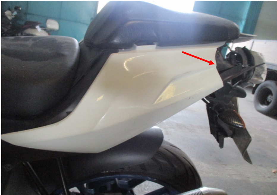
Photo 10 shows a closer view of the cracked left rear side cover (arrowed) of the Motorcycle as a result of the accident.
