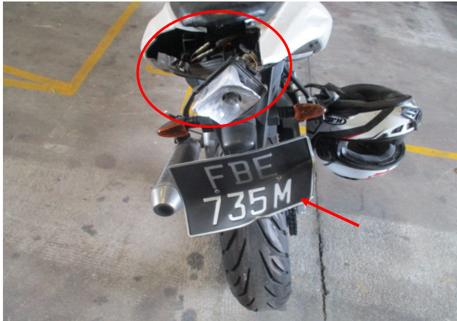
Photo 12 shows the cracked rear cover and tail light (circled) as well as the dented rear number plate (arrowed) of the Motorcycle as a result of the accident.
