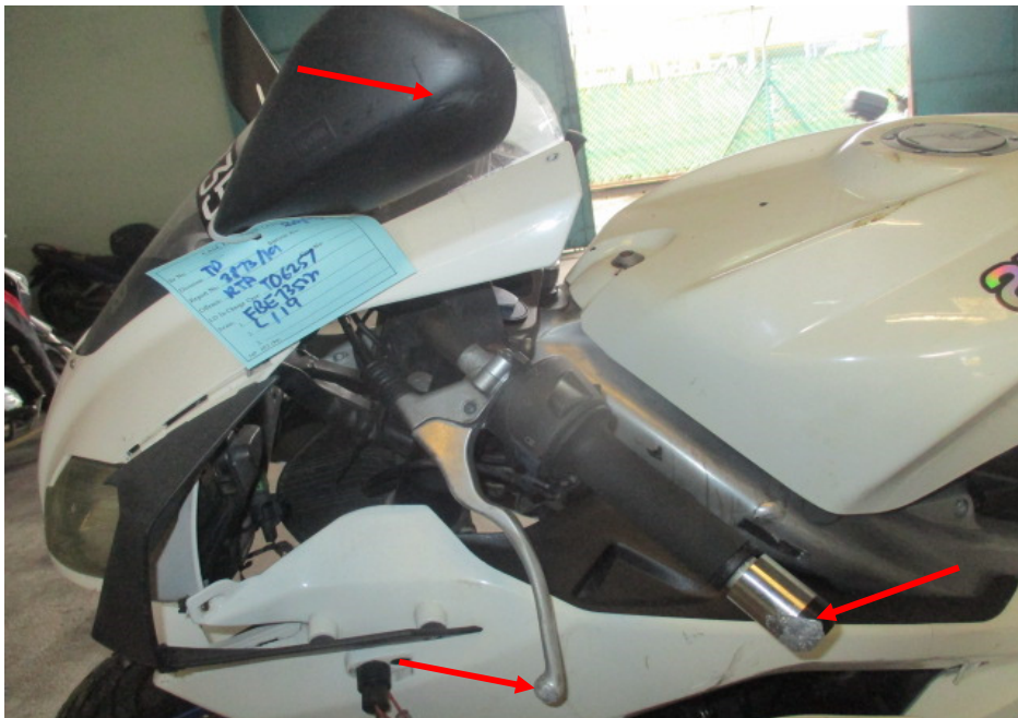
Photo 9 shows a closer view of the left handlebar end, clutch lever as well as left side mirror (arrowed) which were amongst the body parts of the Motorcycle that had sustained damage as a result of the accident.
