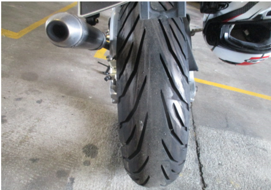
Photo 17 shows the condition of the Motorcycle's rear tyre. The rear tyre was observed to be in serviceable condition with remaining tread depth of approximately 5mm. The tyre was also observed to be sufficiently inflated for vehicular operation. We did not observe any tear, burst mark(s) and/or punctured hole(s) on the sidewalls as well as across the tread of the rear tyre.
