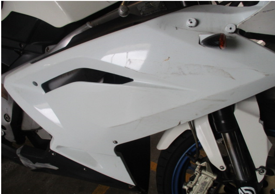
Photo 14 shows a closer view of the right cowling of the Motorcycle that had sustained damages of grazing nature as a result of the accident.
