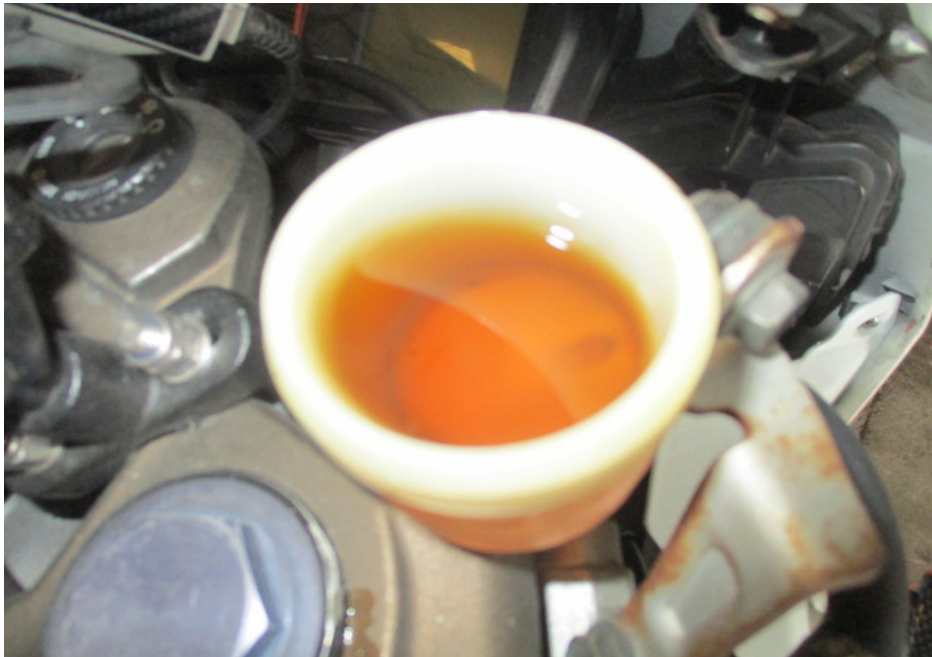
Photo 26 shows the brake fluid reservoir for the front brake of the Motorcycle. The brake fluid was observed to be of sufficient level and without contamination for operational purposes.
