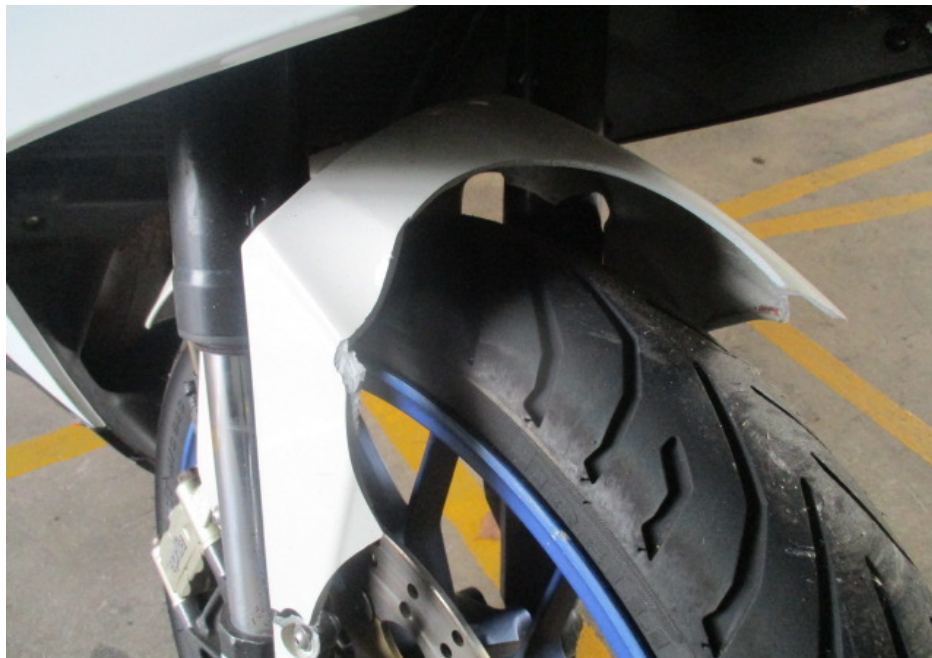
Photo 7 shows a closer view of the cracked front mudguard which was amongst the body parts at the front body of the Motorcycle that had sustained damage as a result of the accident.
