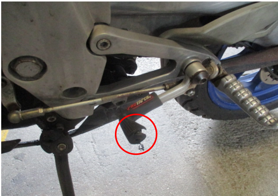
Photo 11 shows a closer view of the gear shift pedal (circled) which was amongst the body parts of the Motorcycle that had sustained damage as a result of the accident.
