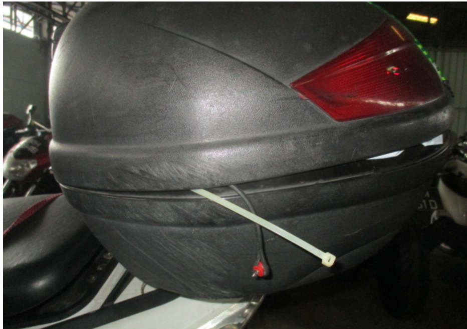
Photo 9 shows a closer view of the top box of the Motorcycle which was observed to have sustained scratches due to the accident.
