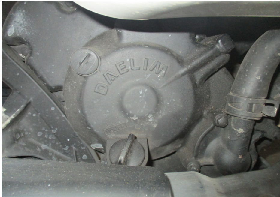
Photo 12 shows the right side of the engine of the Motorcycle at the time of our inspection. The various engine related parts and components were found to be intact with no visible damage. There was also no sign(s) or indication(s) of fluid leak observed around the right engine area of the Motorcycle.
