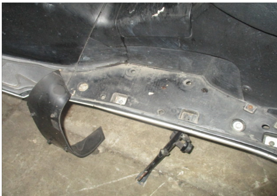
Photo 7 shows a closer view of the left rider step plate of the Motorcycle which was observed to be damaged due to the accident.
