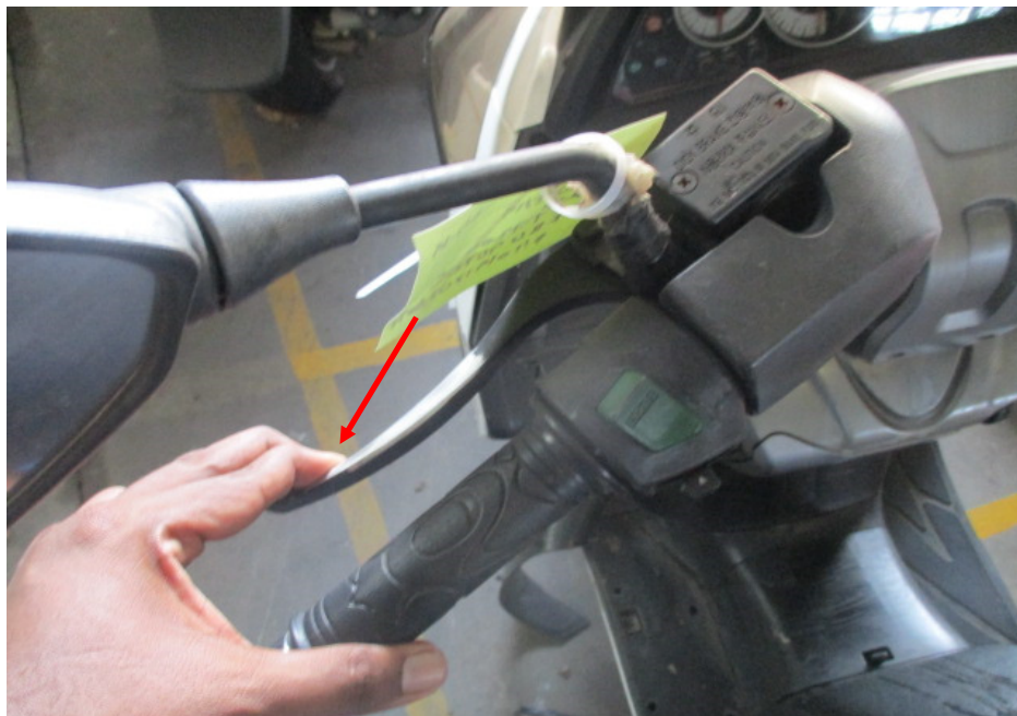
Photo 21 shows the rear brake lever being depressed. There was some resistance felt (spongy like feel) upon pressing the rear brake lever (arrowed). This would indicate that there is no leakage of pressure/vacuum in the brake system.
