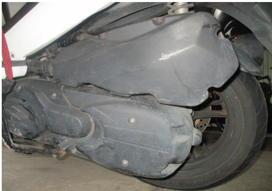
Photo 13 shows the drive train of the Motorcycle which was found to be intact without any misalignment.
