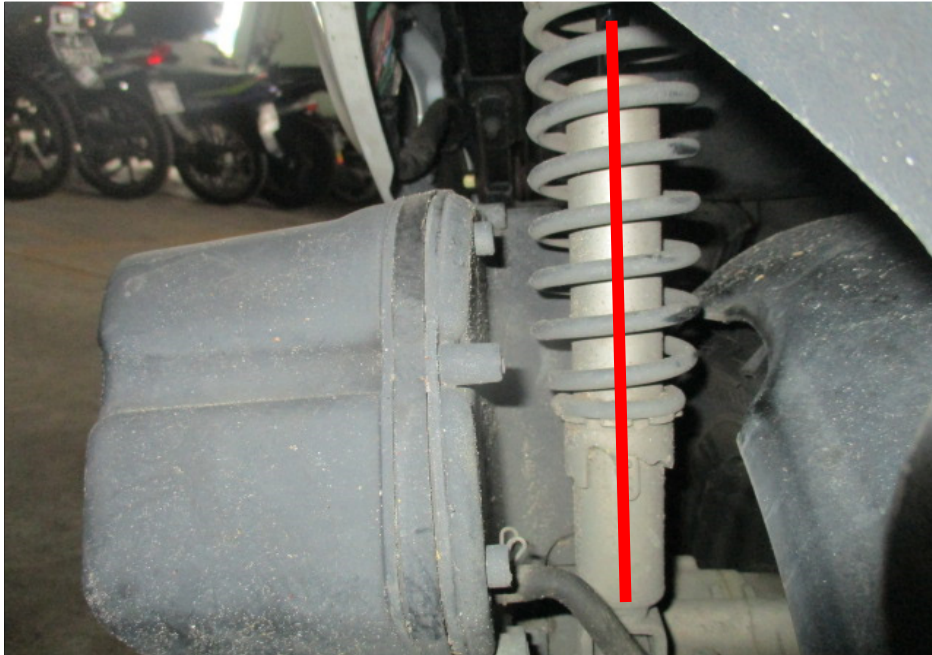
Photo 14 shows the left shock absorber of the motorcycle which was found to be intact without any misalignment.
