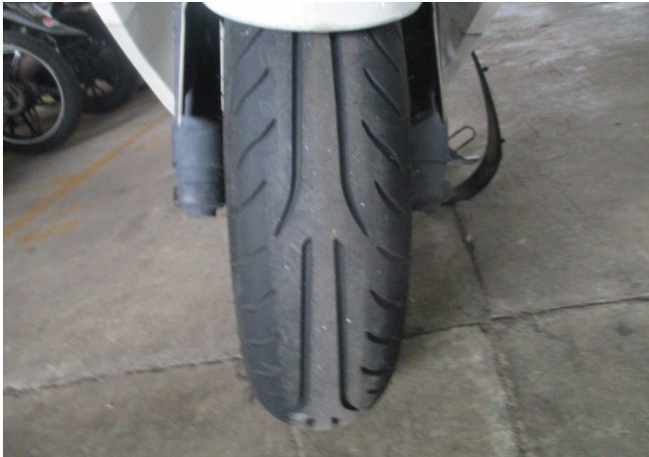
Photo 10 shows the condition of the Motorcycle's front tyre. The front tyre was observed to be in serviceable condition with remaining tread depth of approximately 4mm. There was no tear, burst mark(s) and/or punctured hole(s) on the sidewalls as well as across the tread of the front tyre.
