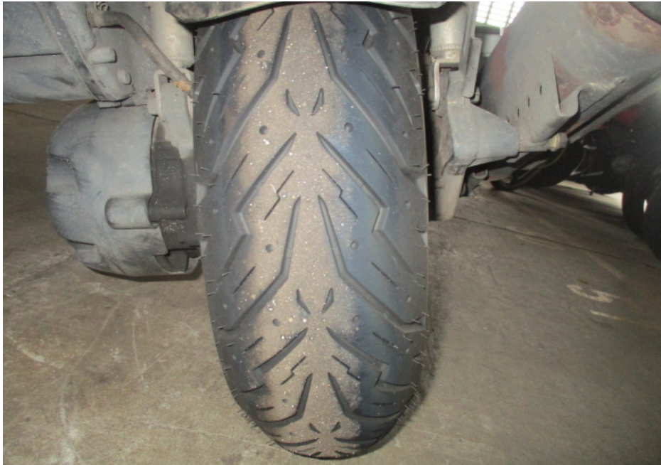
Photo 11 shows the condition of the Motorcycle's rear tyre. The rear tyre was observed to be in serviceable condition with remaining tread depth of approximately 5mm. The tyre was also observed to be sufficiently inflated for vehicular operation. We did not observe any tear, burst mark(s) and/or punctured hole(s) on the sidewalls as well as across the tread of the rear tyre.
