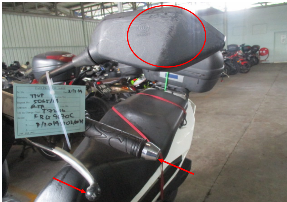
Photo 5 shows a closer view of the rear brake lever and left handlebar end (arrowed) as well as the left side mirror (circled) of the Motorcycle which were observed to be damaged due to the accident
