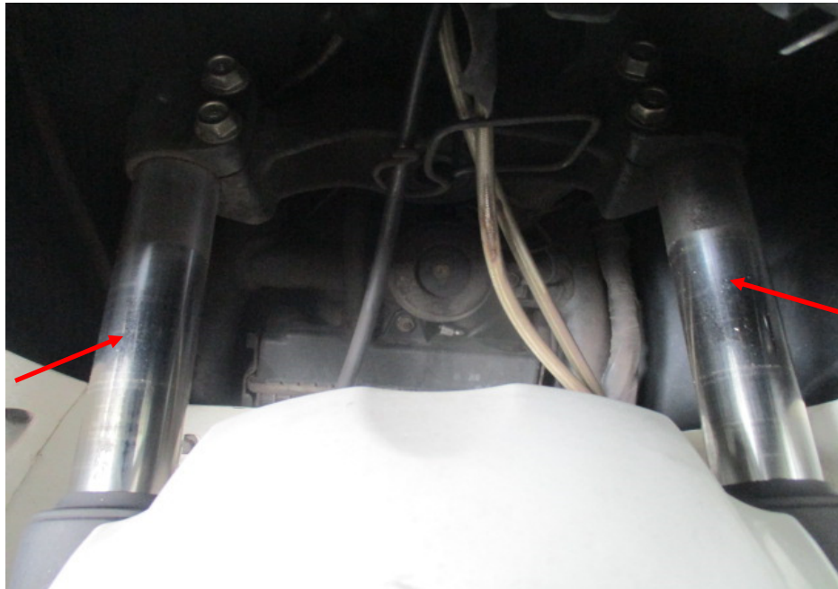
Photo 16 shows the front forks (arrowed) of the Motorcycle. The front forks and fork brackets of the Motorcycle were both found to be intact and undamaged. Turning the Motorcycle's handle bar towards the left and right did not produce any abnormal free play and/or resistance. The steering system of the Motorcycle was in serviceable condition at the time of our inspection.
