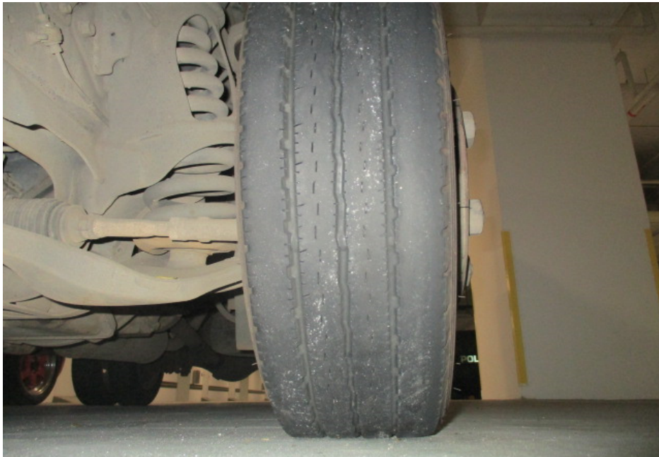
Photo 4 shows the condition of the front left tyre of the Motor Lorry, which was observed to be in serviceable condition with remaining tread depth of approximately 4mm. The tyre, which was wrapped around standard alloy wheel rim, was also observed to be sufficiently inflated for vehicular operation. There was no tear, cut or burst mark(s) on the outer and the inner sidewalls as well as across the tread of the 6 tyres that were fitted on the Motor Lorry.
