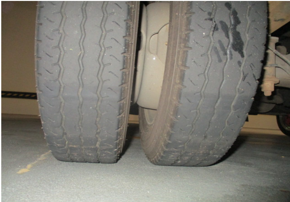
Photo 6 shows the condition of the rear left tyres of the Motor Lorry, which was observed to be in serviceable condition with remaining tread depth of approximately 4mm. The tyres, which were wrapped around standard alloy wheel rim, were also observed to be sufficiently inflated for vehicular operation. There was also no damage found on all 6 alloy wheel rims of the Motor Lorry.
