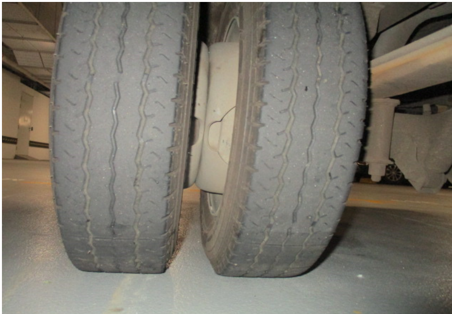
Photo 7 shows the condition of the rear right tyres of the Motor Lorry, which were observed to be in serviceable condition with remaining tread depth of approximately 4mm. There was also no tear, cut or burst mark(s) on the outer and the inner sidewalls as well as across the tread of the 6 tyres that were fitted on the Motor Lorry.
