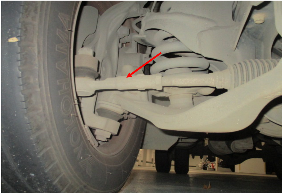
Photo 16 shows the various undercarriage components at the front right wheel of the Motor Lorry, in particular the steering tie rod end (arrowed). The various steering components were all found to be intact, suggesting that the steering system of the Motor Lorry was likely to be in serviceable condition at the material time of accident. There was also no sign of fluid stain(s) observed on the various undercarriage components.
