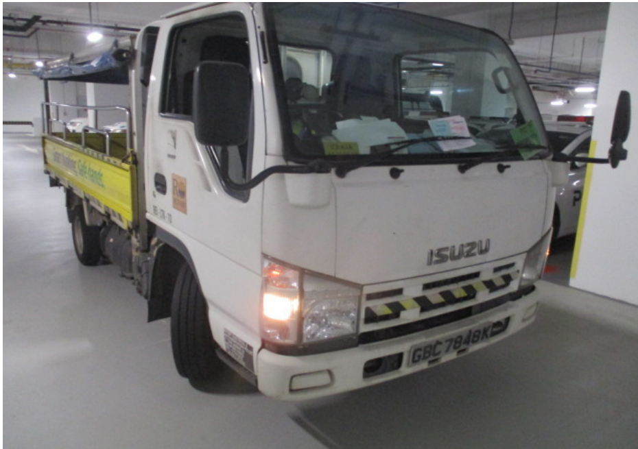
Photo 14 shows the front right wheel of the Motor Lorry turned to its full right. During our steering system test, we did not experience any abnormal free play and/or resistance when we had turned the steering wheel towards full left and full right. This would suggest that the steering system of the Motor Lorry was likely to be in serviceable condition at the material time of accident.
