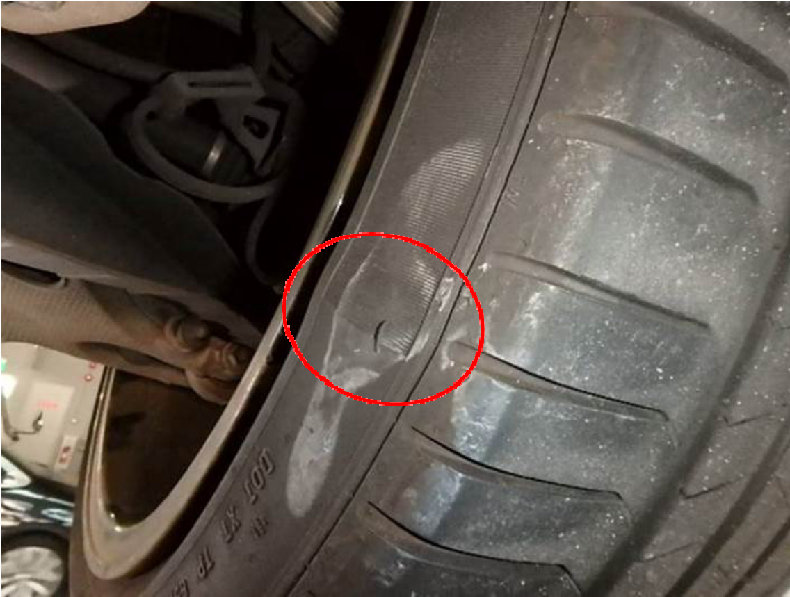
Rear left tyre with the bulged area circled.
