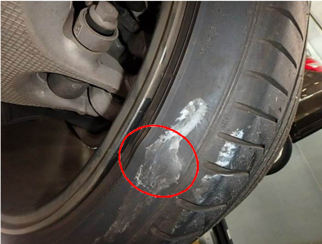
Rear right tyre with the bulged area circled.
