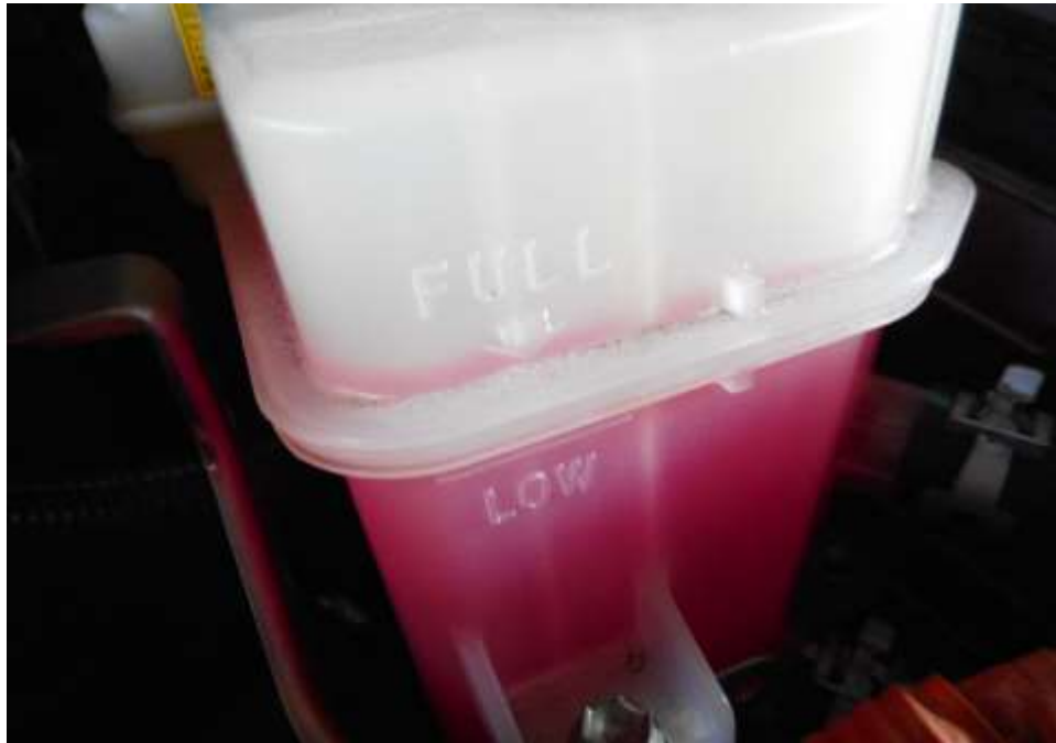
Photo 15 shows the engine coolant reservoir of the Motor Car at the time of my inspection. The engine coolant was observed to be of sufficient level and without any visible contamination.
