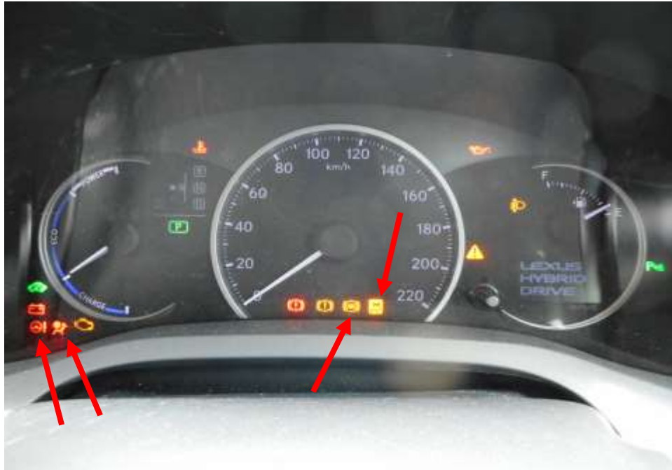
Photo 25 shows the warning light for Anti-Lock Brake System (ABS) and Supplemental Restraint System (SRS) and Electric Power Steering System (EPS) and Traction Control (TC) appearing on the instrument panel of the Motor Car during the self-test of its various electronic operating systems when its engine was cranked.
