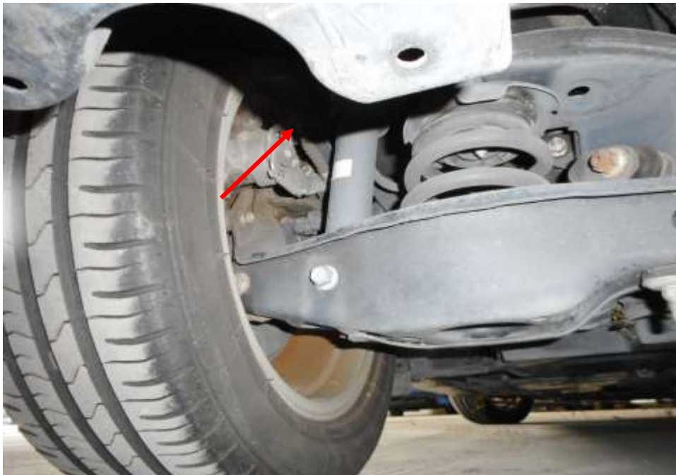
Photo 21 shows the brake pipe (arrowed) at the rear left wheel of the Motor Car. I did not observe any leakage of brake fluid at the time of my inspection of the Motor Car. My static tests of the Motor Car's braking system, along with my visual examination of the various mechanical components in the braking system had indicated that there was no internal leakage of pressure/vacuum. Hence the braking system of the Motor Car was likely to be in serviceable condition at the material time of accident.
