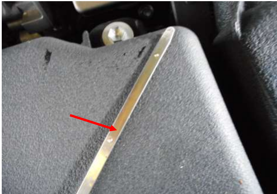
Photo 16 shows the engine oil dip stick of the Motor Car at the time of my inspection. The engine oil was observed to be of sufficient level (arrowed) and without any visible contamination.
