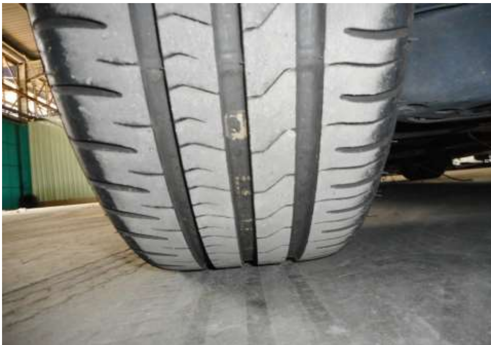
Photo 11 shows the condition of the rear left tyres of the Motor Car, which was observed to be in serviceable condition with remaining tread depth of approximately 6.6mm. The tyres, which were wrapped around standard alloy wheel rim, were also observed to be sufficiently inflated for vehicular operation. There was also no damage found on all 4 alloy wheel rims of the Motor Car.
