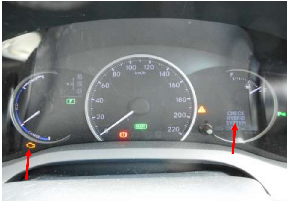
Photo 26 shows only the engine check lights remained on due to a fault in the Motor Car's hybrid system (arrowed) as a result of the accident. No other warning lights illuminated on the instrument panel of the Motor Car after the engine was cranked. This would suggest that there was no abnormality to the various electronic operating systems of the Motor Car, like the ABS, SRS, EPS and TC.
