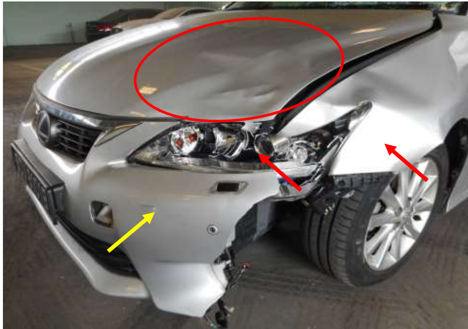
Photo 4 shows a close up view of the Motor Car's frontal portion at the time of my inspection. Its front bonnet (circled), front bumper (yellow arrow), front left fender and front right headlamp (red arrow) were damage at the time of my inspection.
