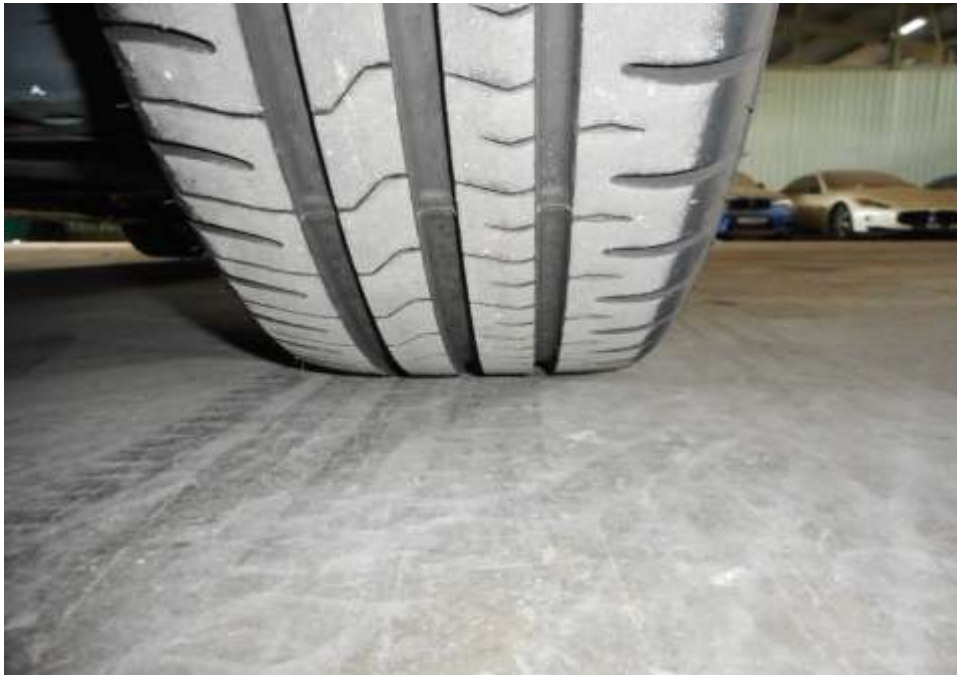
Photo 10 shows the condition of the rear right tyre of the Motor Car, which was observed to be in serviceable condition with remaining tread depth of approximately 6.7mm. The tyre, which was wrapped around standard alloy wheel rim, was also observed to be sufficiently inflated for vehicular operation.
