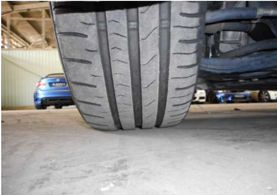
Photo 12 shows the condition of the rear right tyres of the Motor Car, which were observed to be in serviceable condition with remaining, tread depth of approximately 5.1mm. There was also no tear, cut or burst mark(s) on the outer and the inner sidewalls as well as across the tread of the 4 tyres that were fitted on the Motor Car.
