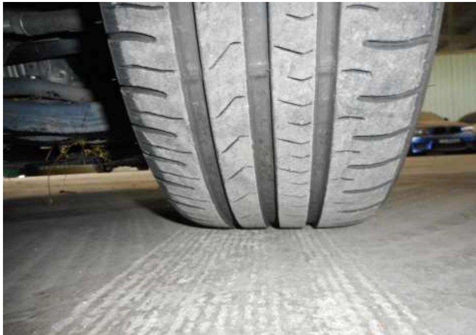
Photo 9 shows the condition of the front right tyre of the Motor Car, which was observed to be in serviceable condition with remaining tread depth of approximately 5.1mm. The tyre, which was wrapped around standard alloy wheel rim, was also observed to be sufficiently inflated for vehicular operation. There was no tear, cut or burst mark(s) on the outer and the inner sidewalls as well as across the tread of the 4 tyres that were fitted on the Motor Car.
