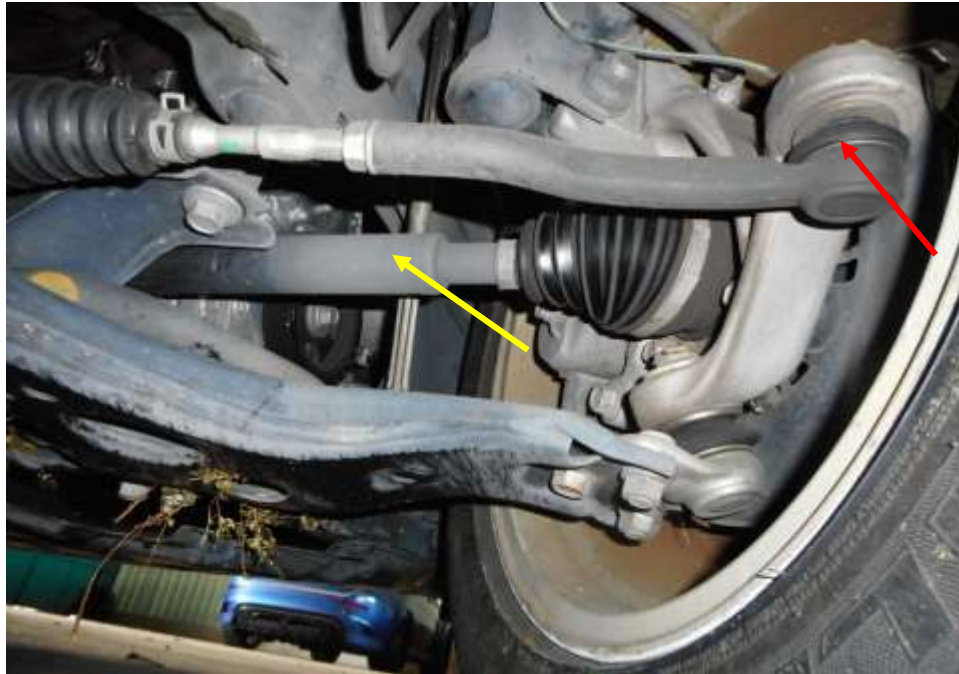
Photo 18 shows the various undercarriage components at the front right wheel of the Motor Car, in particular the steering tie rod end (arrowed) and drive shaft (yellow arrow). The various steering components were all found to be intact, suggesting that the steering system of the Motor Car was likely to be in serviceable condition at the material time of accident. There was also no sign of fluid stain(s) observed on the various undercarriage components.
