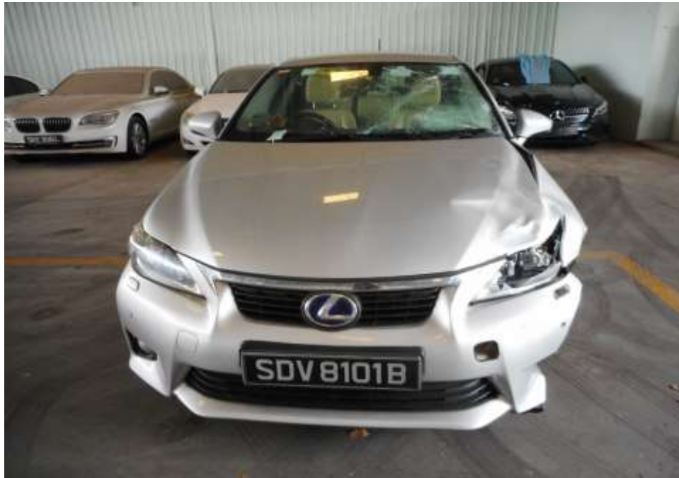
Photo 2 shows a general view of the Motor Car's frontal portion at the time of my inspection. It appeared to have sustained damage at its frontal portion. Its front windscreen, front bonnet, front bumper, left fender, front left headlamp and left rear mirror were damage at the time of my inspection.
